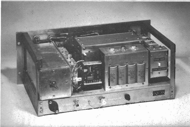
Rear view of the receiver, showing block construction and heavy shielding. The large compartment at the left of the chassis is the rf assembly. To the right of center may be seen the four electrolytic capacitors in the power supply. The assembly forward of the supply is the LMO.
