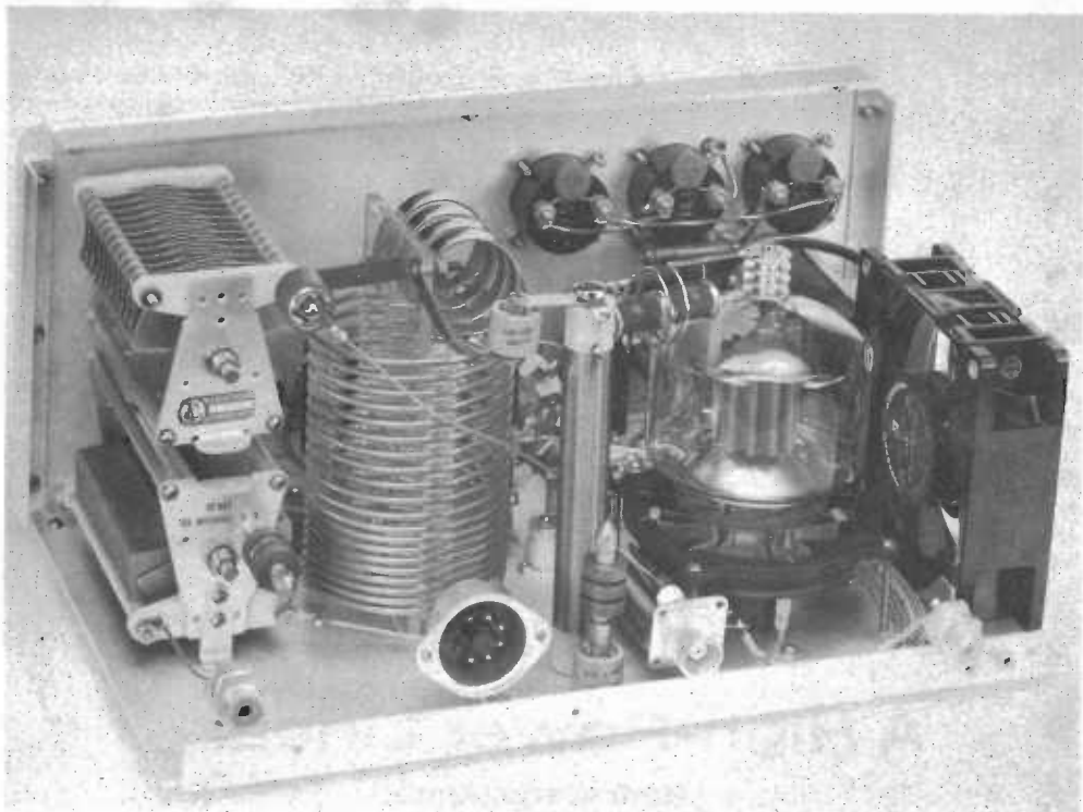
FIG. 3—The rear wall of the compact kilowatt has been removed to reveal the "works." Coaxial receptacles at left are output and input jacks; receptacle at center (near tube) is high-voltage connector. A 50-pf 3.5-Mc. plate loading capacitor can be seen mounted on the plate tuning capacitor (upper left); the 500-pf. 3.5-Mc. output loading capacitor is mounted on the base behind the coil (just visible to right of variable loading capacitor).
