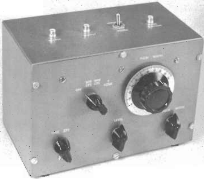
Front view of the two-tone test oscillator. The generator is completely self-contained. Battery drain is only 4 ma.
