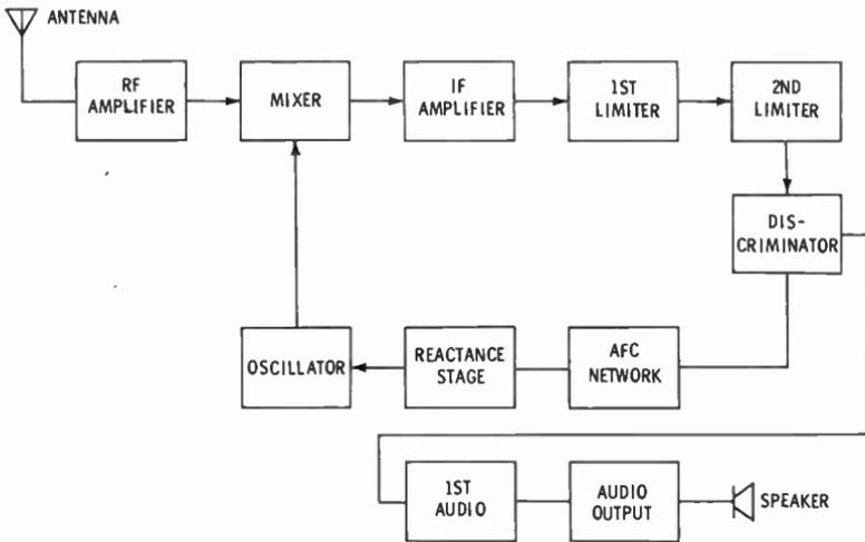
**Fig. 49. Block diagram of a superheterodyne FM receiver with automatic frequency control.**
