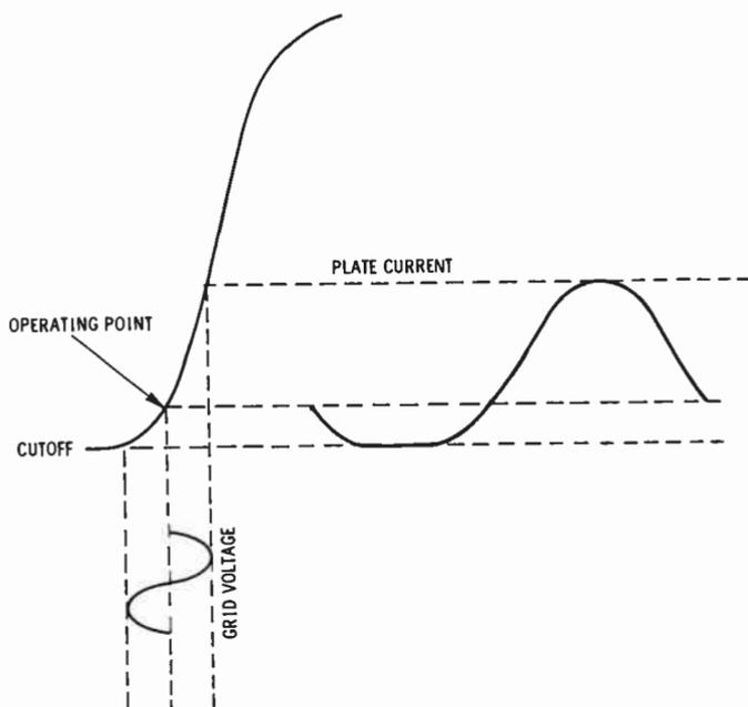
Fig. 9. The effect of biasing a tube near the cutoff point.
