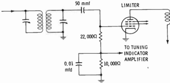
Fig. 40. One type of limiter used in FM receivers.
