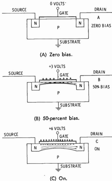
Fig. 25. N-channel enhancement MOSFET.
