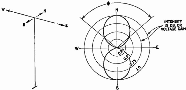
Fig. 11. Directional response pattern of a dipole antenna.
