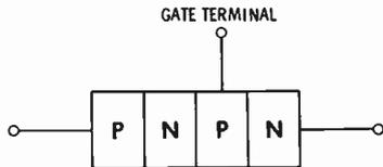
semiconductor acts as an open circuit to electron flow until an appropriate gate signal is applied to the third terminal. When this occurs the device is triggered into conduction and from then on operates as a conventional semiconductor diode. The action of this rectifier is similar to that of a thyatron tube.
