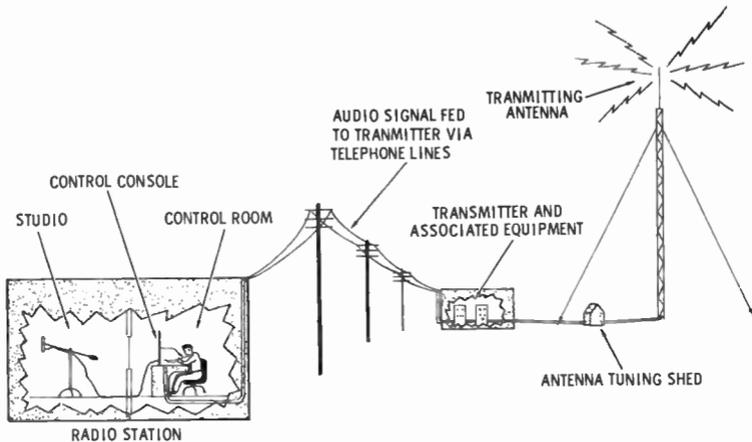
Fig. 5. Hookup of a typical radio broadcasting station.
