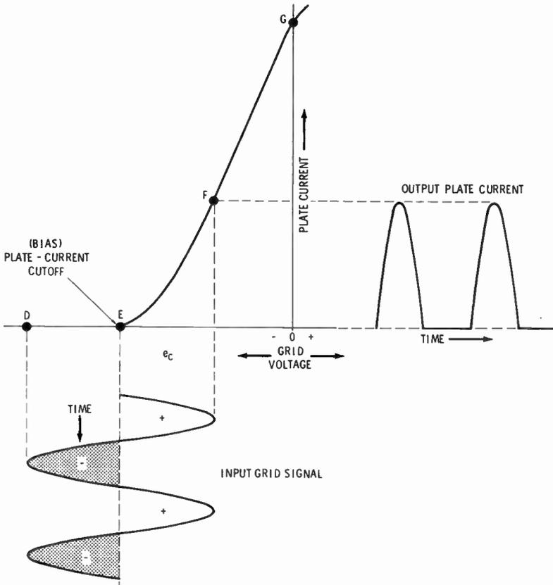
**Fig. 10. Characteristic curve with class-B operation.**
