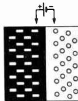
Fig. 5. Action of the carriers at a junction.
