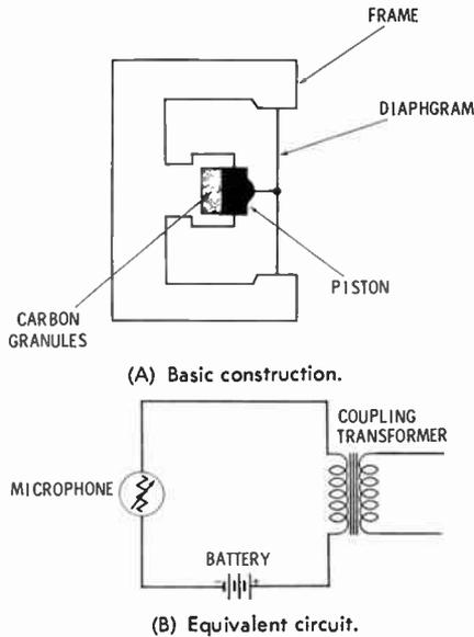
**Fig. 9. Principles of a carbon microphone.**
