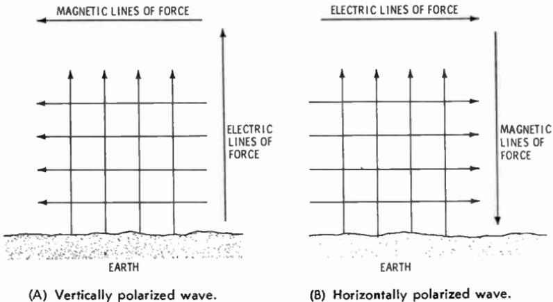
Fig. 1. Relationship between the electric and magnetic fields in a radio wave.
