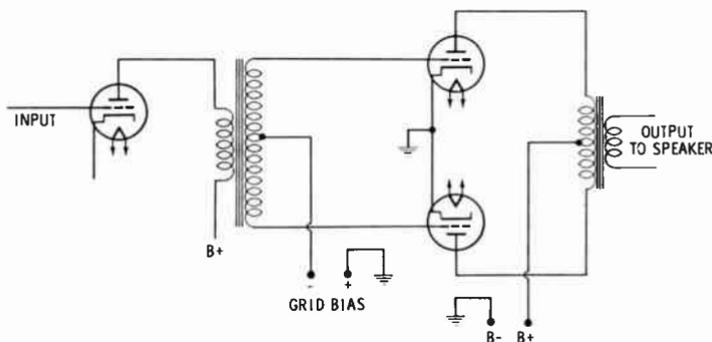
Fig. 7. A push-pull amplifier circuit. This type of amplification requires two identical tubes in the stage.
