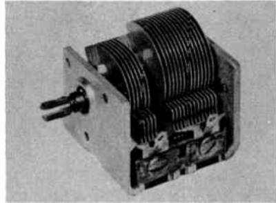
with those of the stationary (stator) plates, and the maximum capacity is obtained when the full areas of the two sets of plates are exposed to each other. For various other positions, some intermediate value of capacitance exists (see Fig. 10). The shape of the movable plates determines the amount of capacitance variation with rotation.
