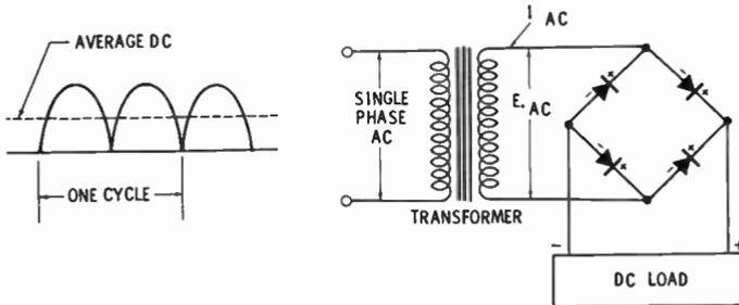
Fig. 3. A full-wave-bridge rectifier circuit.
