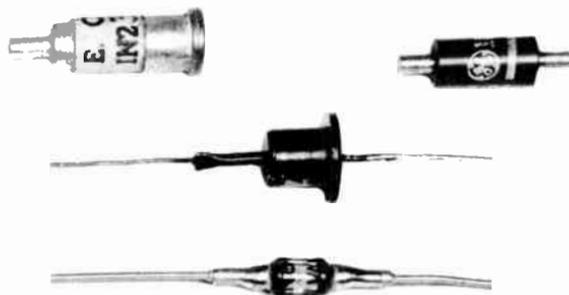
Fig. 1. Typical examples of crystal diodes.
