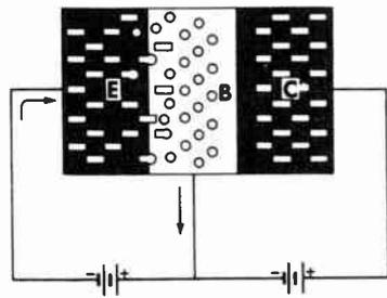
(B) Action caused by connecting a second battery in the reverse bias direction of an NPN-type of transistor.
