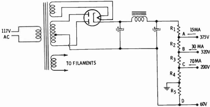
Fig. 11. A voltage divider network.
