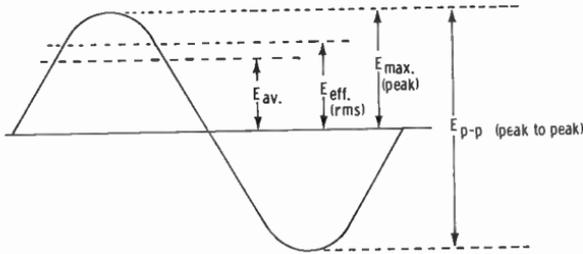
**Fig. 12.** Relationship between average, effective (rms), maximum (peak), and peak-to-peak voltages and current.
