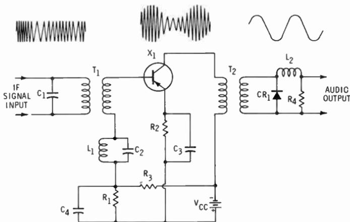
Fig. 48. A transistor slope detector and diode detector.
