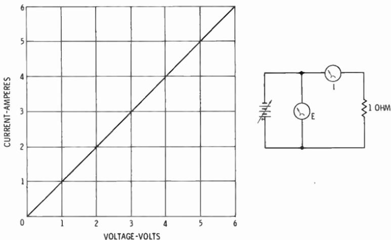
Fig. 20. Current vs voltage, with resistance constant.
