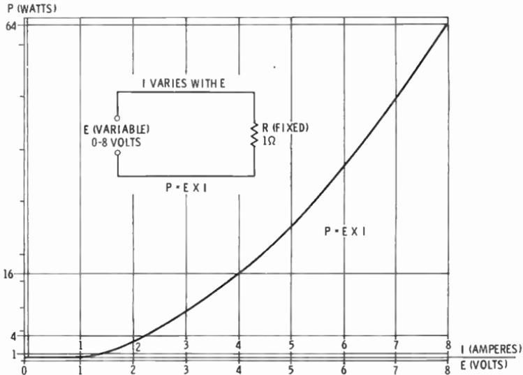
Fig. 26. Graph of power related to changing voltage and current.
