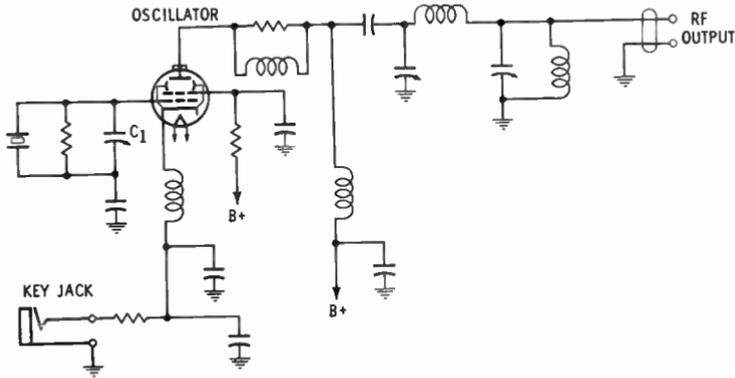
Fig. 1. A simple tube-type radio transmitter.
