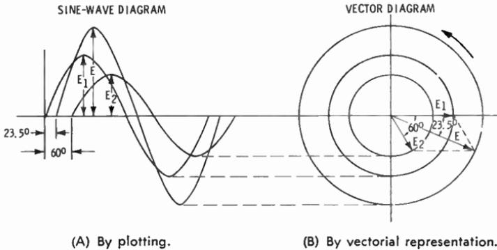
Fig. 17. Addition of two sine waves.
