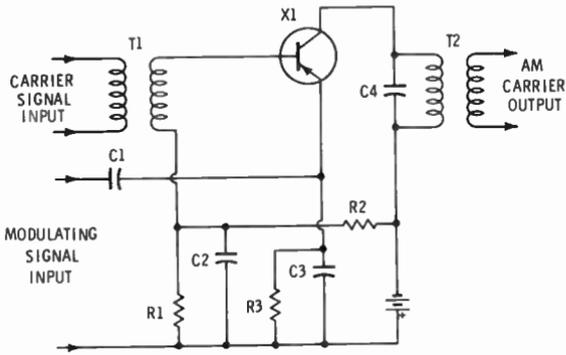
**Fig. 10. An amplitude-modulated amplifier with emitter injection.**
