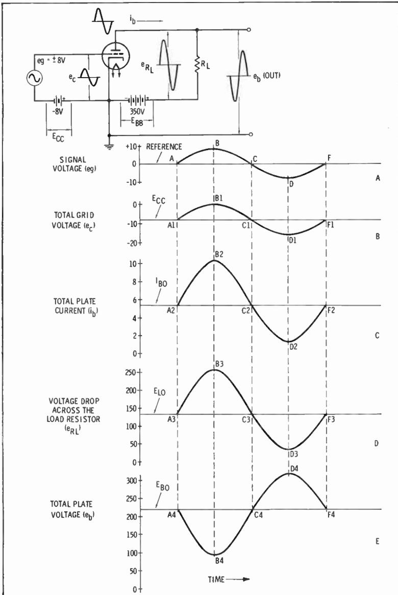
Fig. 16. Waveforms in a triode amplifier circuit.
