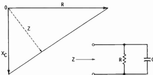
Fig. 8. Graphical solution of an RC parallel circuit.
