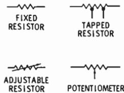
flow is about 17 ma., which means that the top half of the potentiometer must dissipate about 4.5 watts. This will cause the unit to overheat badly and be damaged. This example shows that a potentiometer must be derated accordingly when it is required to supply current to a load.
