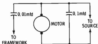
Fig. 3: Schematic diagram showing connection of interference suppressors to a vacuum cleaner.
