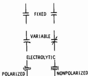
Fig. 15. Common schematic symbols for capacitors.
