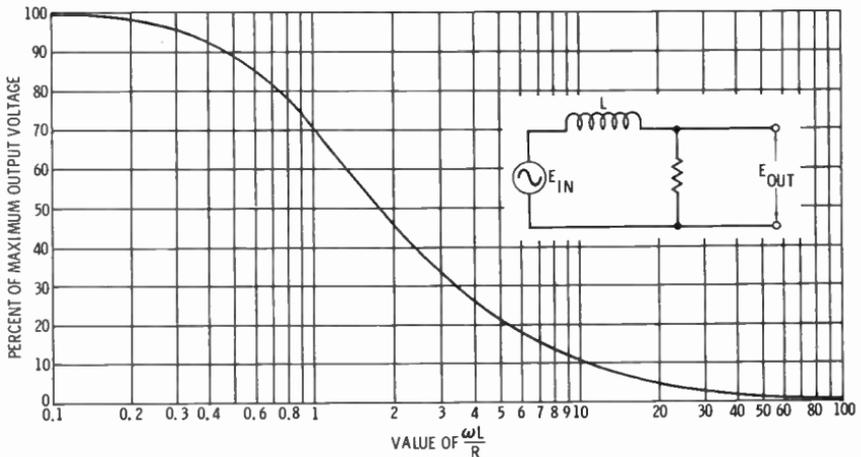
Fig. 3. Universal frequency-response curve for RL series circuits.
