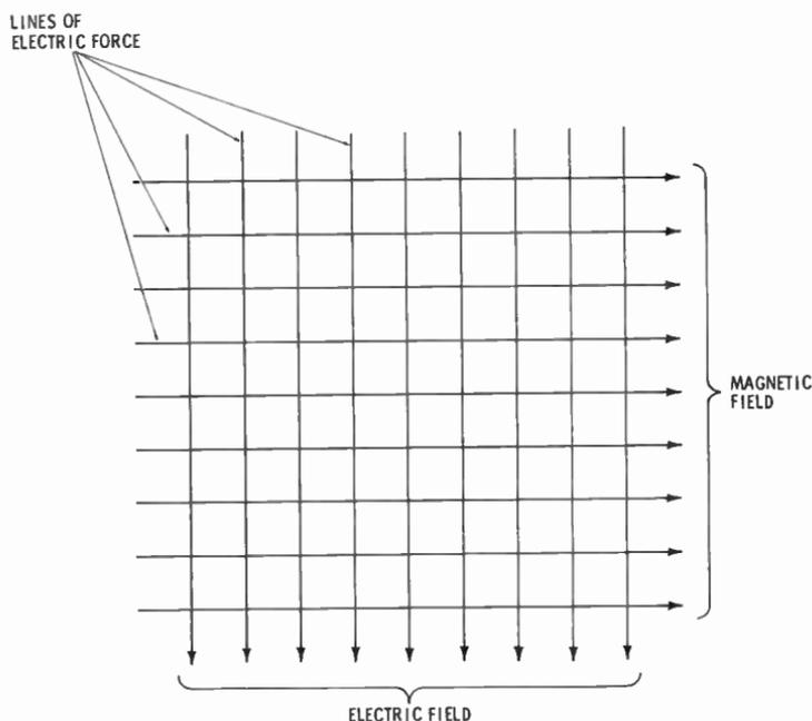
Fig. 4. Electric and magnetic lines of force in a radio wave.
