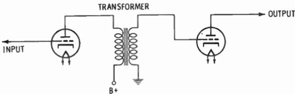
**Fig. 34. Interconnection of a transformer-coupled AF amplifier.**
