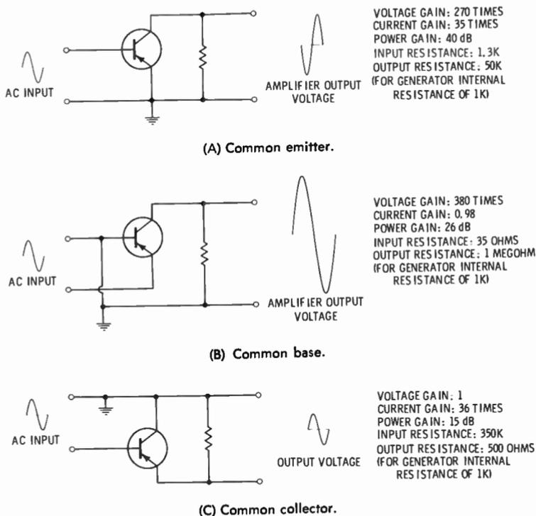
Fig. 20. Transistor circuit parameters.
