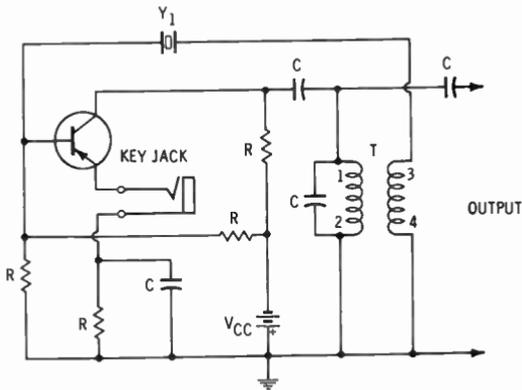
Fig. 2. A simple transistor-type radio transmitter.
