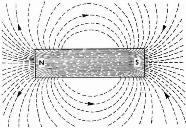
Fig. 10. Theoretical concept of lines of force surrounding the poles of a bar magnet.
