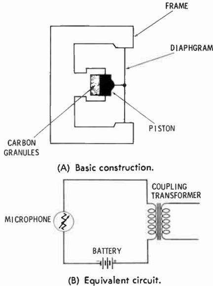
**Fig. 9. Principles of a carbon microphone.**
