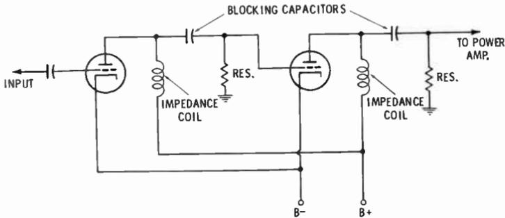
**Fig. 33. An impedance-coupled AF amplifier.**
