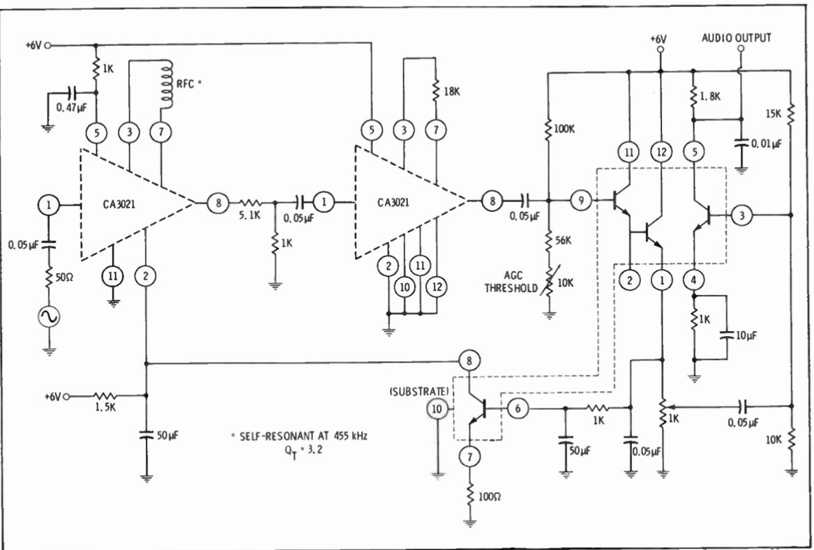
Fig. 39. Connections of the RCA CA3021 IC in a 455-kHz amplifier.
