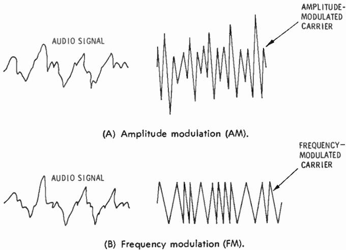
Fig. 2. Two types of modulation presently employed in radiocommunications.
