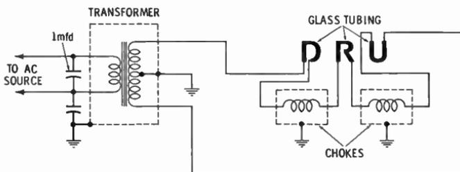
Fig. 8. Interference suppressors added to a neon sign.
