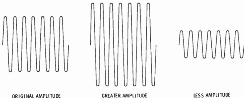
(B) Sine waveforms with same frequency (or wavelength).
