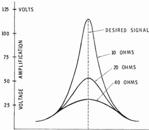
**Fig. 14.** Typical voltage characteristics indicating the effect of varying the effective resistance of a circuit at resonance.
