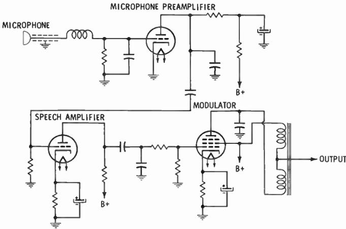
Fig. 5. One type of audio modulator circuit.
