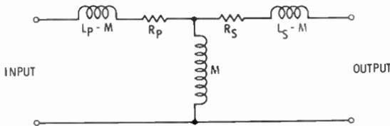
Fig. 15. A more complete equivalent circuit of a basic transformer.
