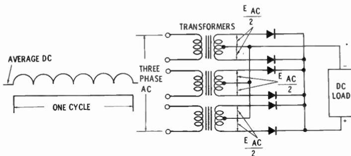
Fig. 7. A center-tapped, three-phase rectifier circuit.
