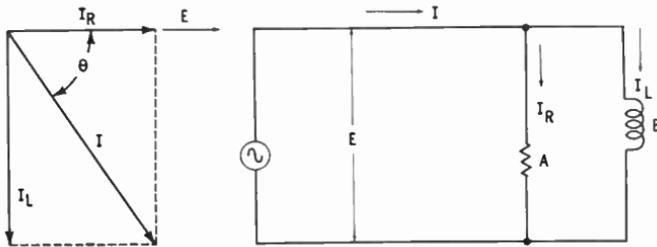
Fig. 6 Parallel connection of resistance (R) and inductive reactance ( $X_L$ ).
