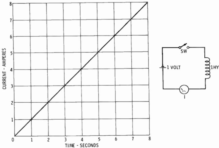
Fig. 1. Current increase in a pure inductance of 1 henry.
