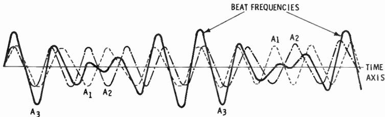
Fig. 17. How beat frequencies are generated. Observe how frequencies  $A_1$  and  $A_2$  are alternately in and out of phase with each other. The frequency with which these two are in phase is equal to the difference between their frequencies.
