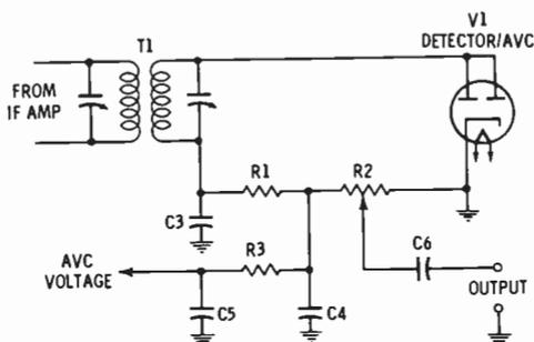
Fig. 5. A typical detector/AVC circuit.
