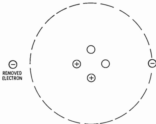
Fig. 4. Structure and electron orbit of a positively charged helium atom.
