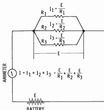
Fig. 23. Simple circuit with three resistances connected in parallel.
