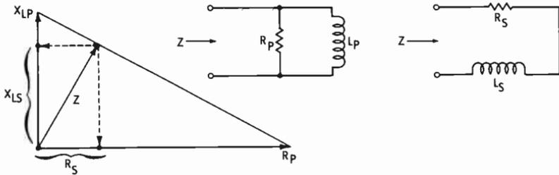
Fig. 9. Graphical solution for finding equivalent series and parallel circuits.
