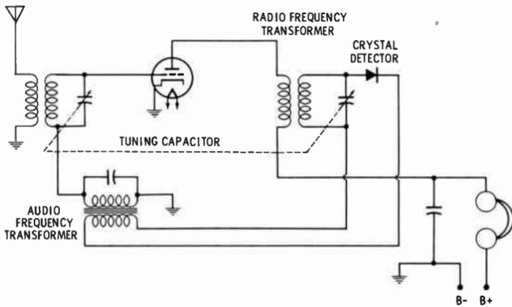
Fig. 28. A typical reflex circuit.
