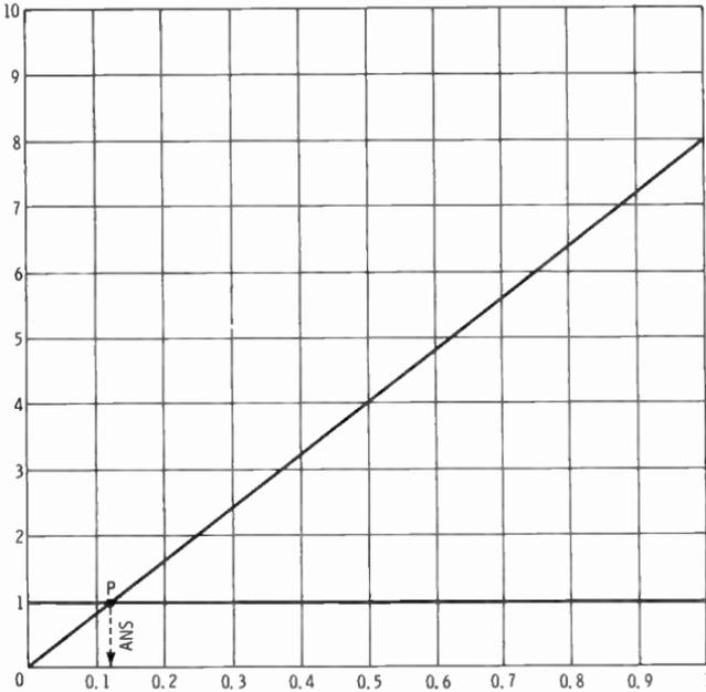
Fig. 9. Graphical method for finding a reciprocal.
