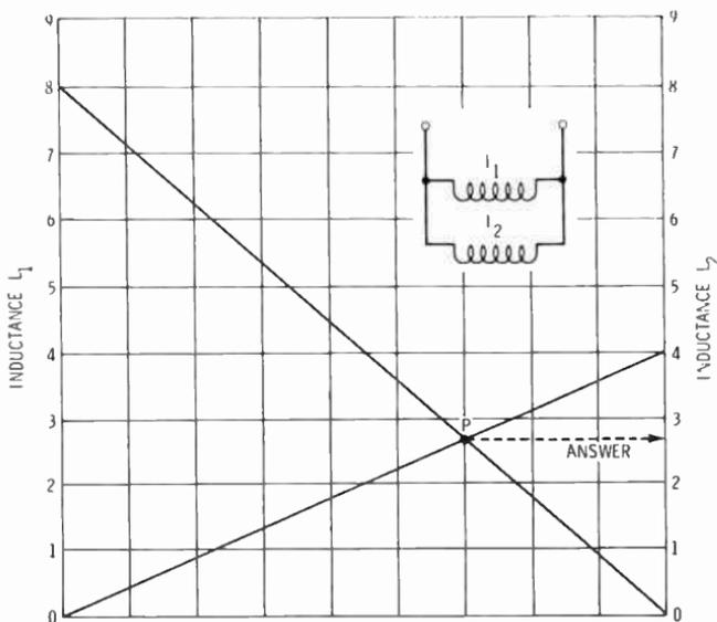
Fig. 10. Graphical method for finding total inductance of inductors in parallel.
