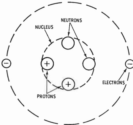
Fig. 3. Structure and electron orbit of a neutral helium atom.
