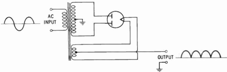
Fig. 3. Full-wave rectifier circuit.
