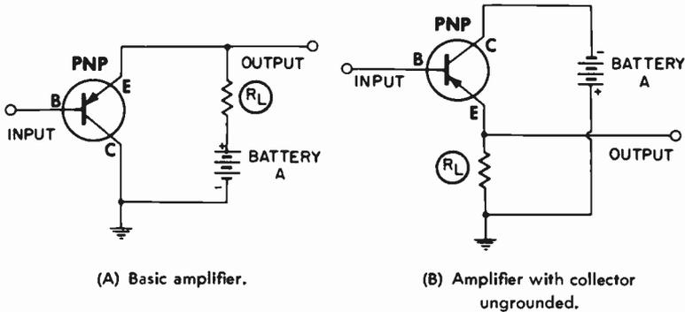
Fig. 19. The common-collector amplifier.
