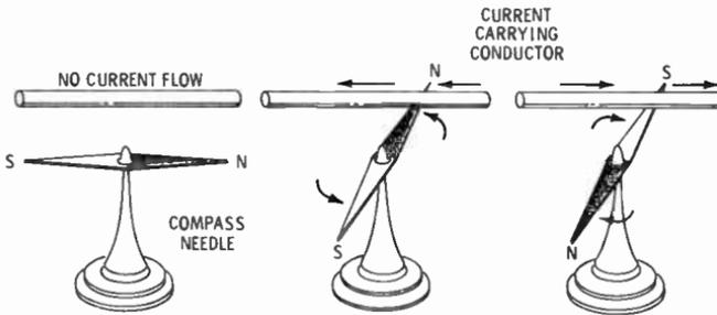
Fig. 31. Deflection of a compass needle when held near a current-carrying conductor.
