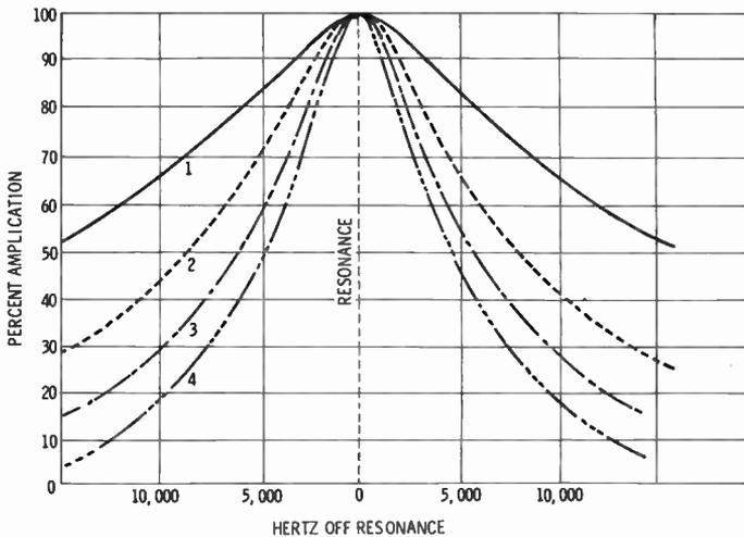
Fig. 13. How several stages of RF amplification increase the selectivity of a receiver by reducing undesired signal strength.
