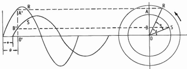
Fig. 16. Vectorial representation of two alternating-current sine waves.
