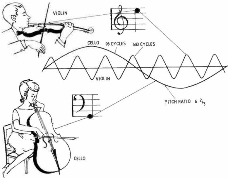
Fig. 10. Properties of wave motion illustrating pitch.
