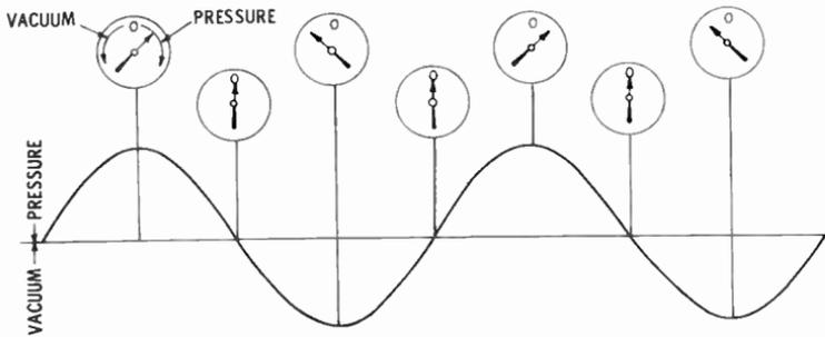
Fig. 5. Diagram illustrating pressure variations due to sound waves.
