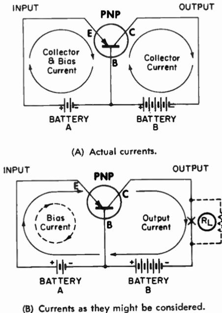
Fig. 18. Current paths in a common-base amplifier.
