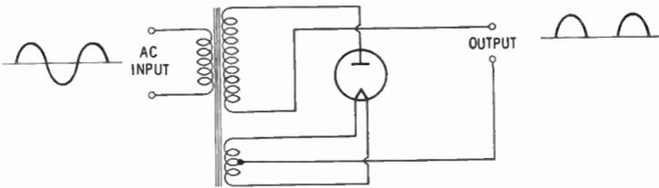
Fig. 2. Basic half-wave rectifier circuit.
