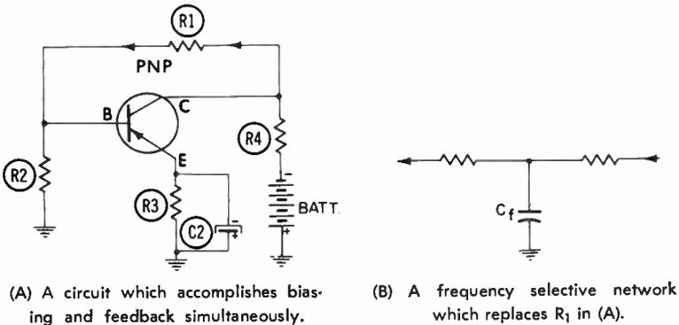
Fig. 27. Bias stabilization and signal feedback.
