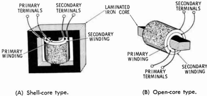
Fig. 14. Two types of transformers having the primary and secondary windings placed directly on top of each other.
