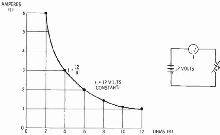
**Fig. 21. Relation between current and resistance, with voltage constant.**
