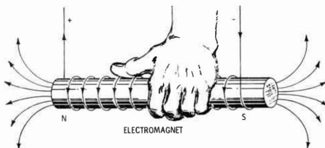
Fig. 35. Method of finding the polarity of a coil by means of the left-hand rule.
