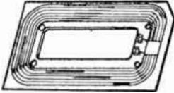
Fig. 12. A typical built-in loop antenna.
