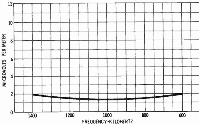
Fig. 5. Sensitivity characteristics of a typical radio receiver.
