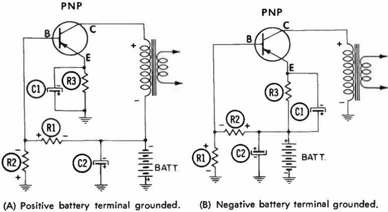
Fig. 26. A common-emitter amplifier using a PNP transistor.
