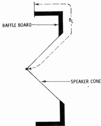
Fig. 6. A speaker baffle.
