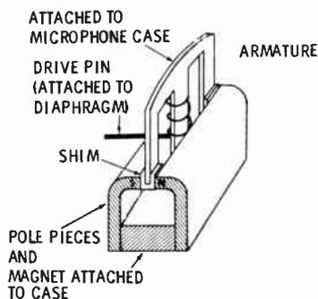
Fig. 10. Basic construction of a variable-reluctance microphone.
