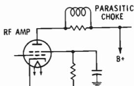
Fig. 4. A parasitic choke in the plate lead of an RF power amplifier.
