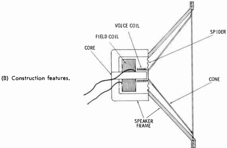
Fig. 2. An electrodynamic speaker. Notice that this speaker has an electromagnet instead of a permanent magnet.
