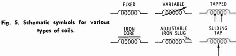
Fig. 5. Schematic symbols for various types of coils.
