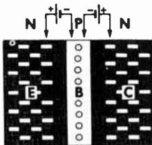
Fig. 8. Arrangement of an NPN-type of transistor.
