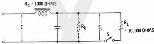
Fig. 12. Application of a bleeder resistor across a power supply.
