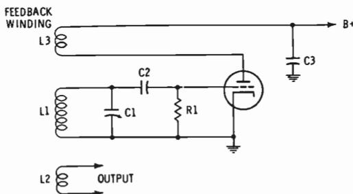
Fig. 17. "Tickler coil" oscillator circuit.
