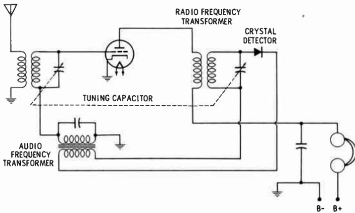
Fig. 28. A typical reflex circuit.
