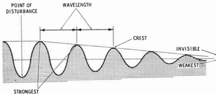
Fig. 2. Cross-sectional view of waves produced by throwing a stone in still water.
