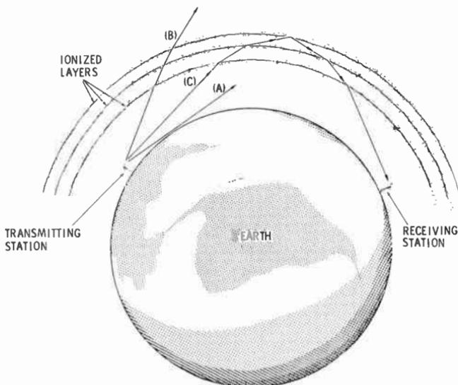
Fig. 8. The effect of frequency on sky-wave propagation.
