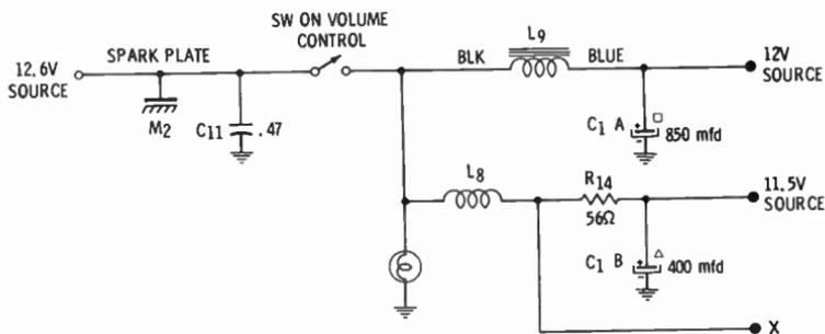
Fig. 51. Power supply for automobile receiver using low-voltage tubes.
