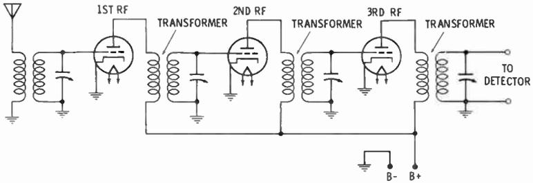
Fig. 12. A three-stage transformer-coupled RF amplifier.
