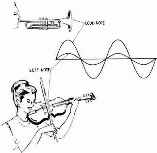
Fig. 8. Properties of wave motion illustrating the causes of loudness of tone.
