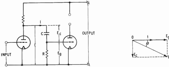
Fig. 15. Interstage coupling with vector diagram.
