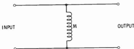
Fig. 4. Equivalent circuit for a basic transformer when magnetic coupling is complete.
