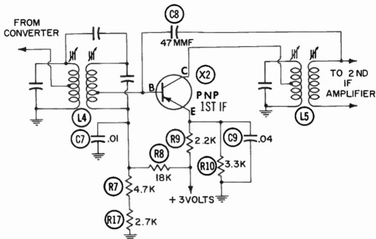
Fig. 37. An IF amplifier with double-tuned transformers.
