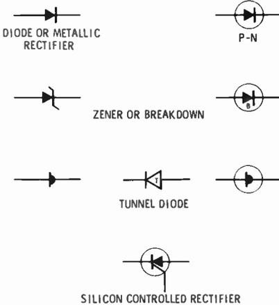
Fig. 9. Common schematic symbols for semiconductors.
