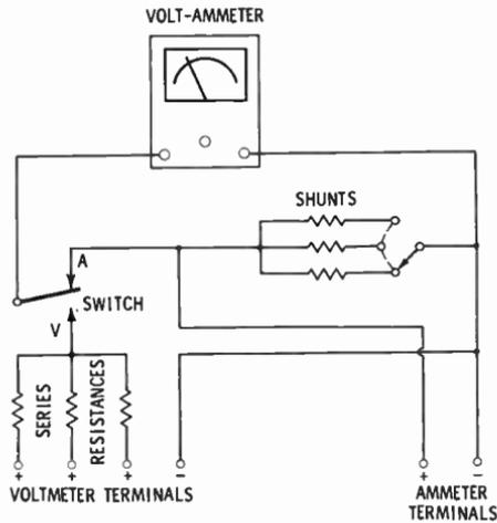
**Fig. 8. Switching arrangement used to permit voltage and current measurements with the same meter.**
