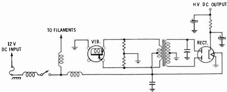
Fig. 16. A DC-to-DC converter using a vibrator.
