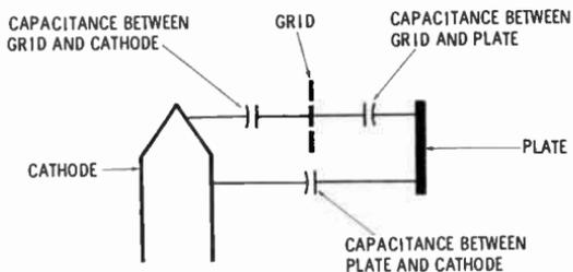
Fig. 13. Interelectrode capacities in a triode.
