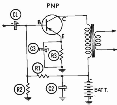
Fig. 28. A very common RC-coupled amplifier circuit.
