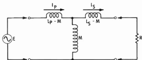
Fig. 11. Illustrating voltage decrease under load.
