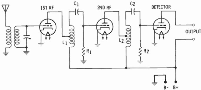
Fig. 11. A two-stage impedance-coupled RF amplifier.
