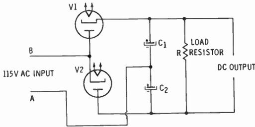
Fig. 13. A voltage-doubler circuit using vacuum tubes.
