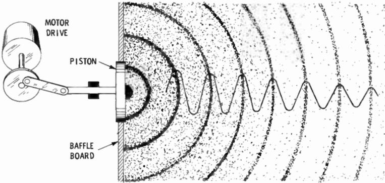
Fig. 3. Generation of sound waves by the oscillation of a piston.
