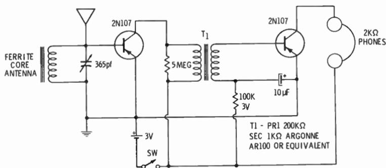
Fig. 21. A two-transistor receiver.
