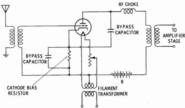
**Fig. 24.** A grid-bias detector circuit.
