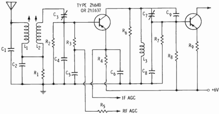
Fig. 10. A transistor "front-end" for a radio receiver.
