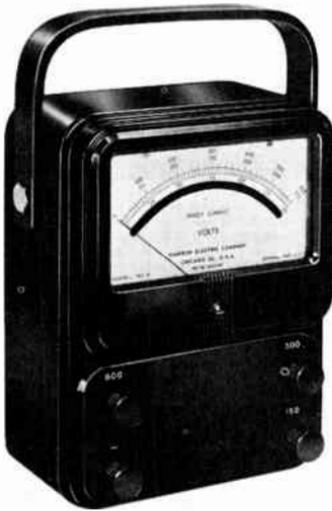
Fig. 6. A high-accuracy DC voltmeter.
