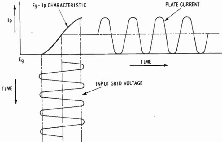
Fig. 39. Action of limiter in clipping modulation peaks beyond linear portion of the characteristic curve.
