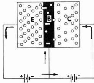
(D) A PNP-type of transistor showing reversed action.
