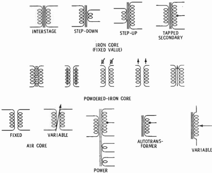
Fig. 19. Schematic symbols for transformers.
