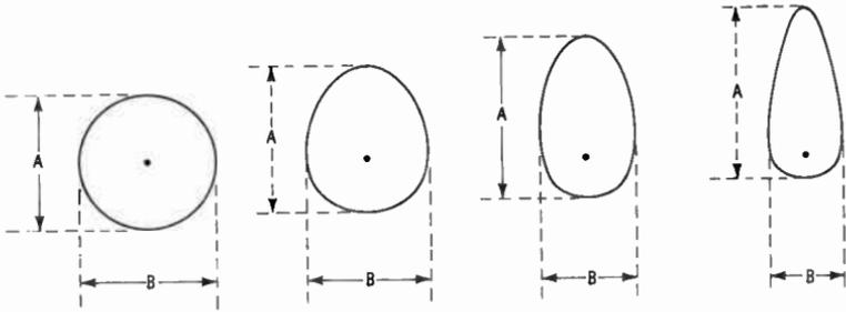
**Fig. 3. Radiation patterns showing how increasing the field strength in one direction decreases the strength in other directions.**
