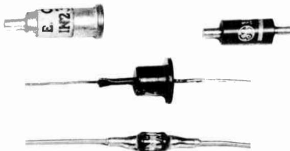
Fig. 1. Typical examples of crystal diodes.
