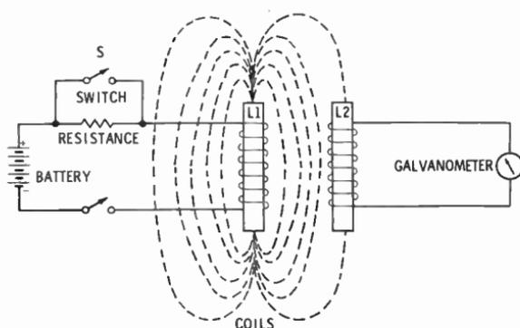
Fig. 36. Circuit showing how the effect of mutual induction may be measured by a galvanometer.
