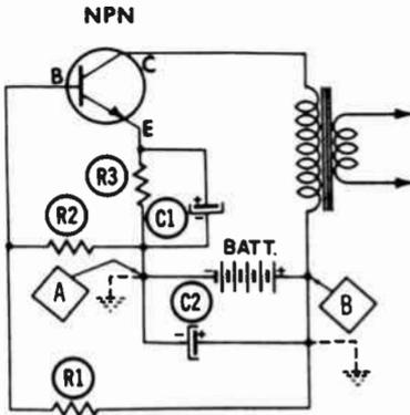
(C) Circuit of (A) and (B) showing alternate points of grounding.
