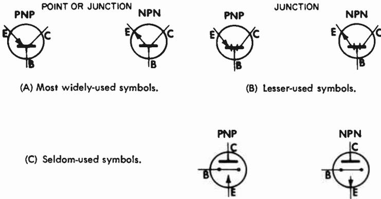
Fig. 11. Commonly accepted transistor symbols.
