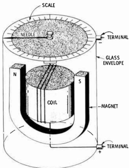
Fig. 1. Essential features of a D'Arsonval galvanometer.
