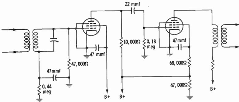
Fig. 44. A dual limiter circuit.
