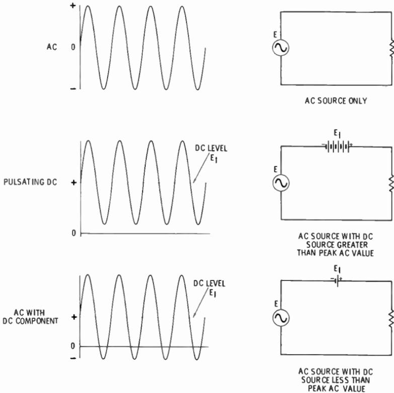
Fig. 7. Three basic combinations of AC and DC values.
