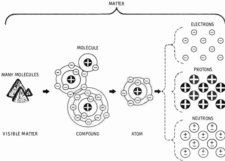
Fig. 1. Breakdown of visible matter to electrical particles.
