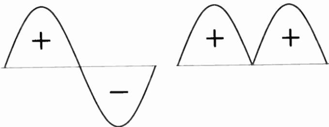
**Fig. 13.** The average and effective values of these waveforms are the same.
