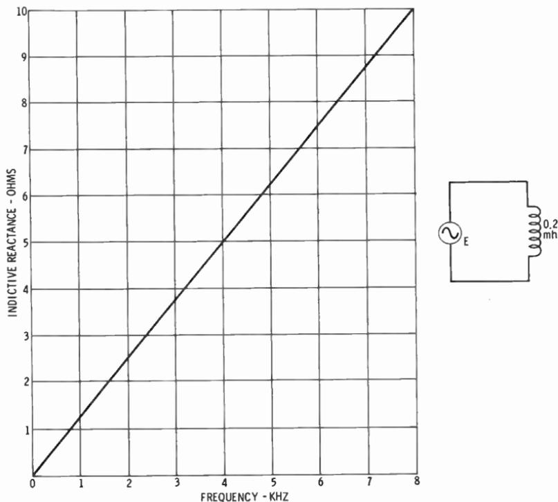
Fig. 4. Inductive reactance versus frequency.
