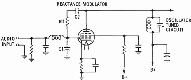
Fig. 12. Reactance modulator used to produce frequency modulation.
