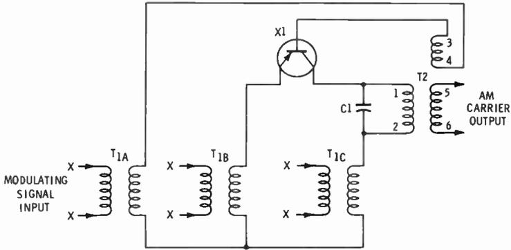
Fig. 7. Methods of injecting an amplitude-modulating signal into an oscillator circuit.
