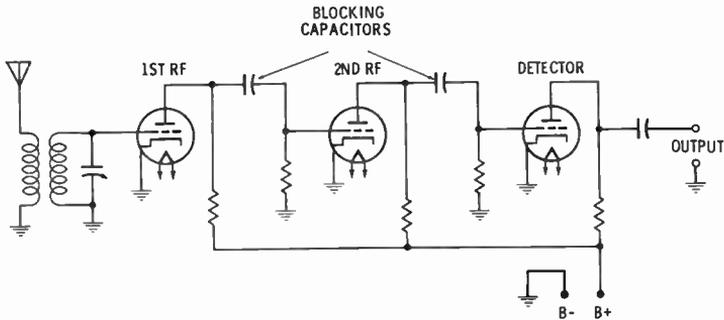
Fig. 9. A typical two-stage resistance-coupled RF amplifier.
