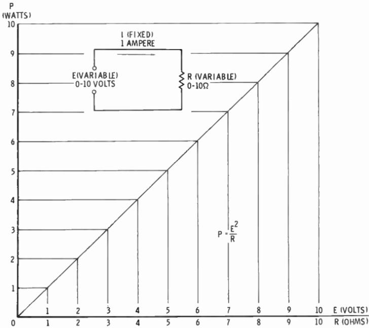
**Fig. 28. Graph of power related to changing voltage and resistance.**
