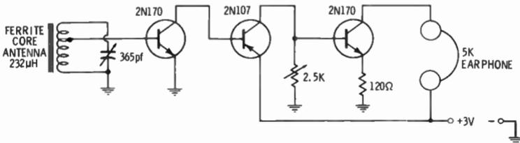
Fig. 25. A three-transistor receiver.
