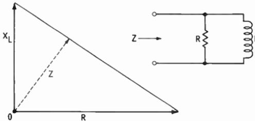
Fig. 7. Graphical solution of an RL parallel circuit.
