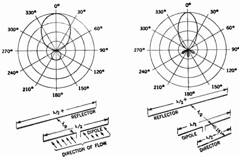
Fig. 10. The effect on the radiation pattern of adding director and reflector elements to a dipole.
