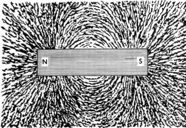
Fig. 11. The magnetic lines of force as exerted by a bar magnet on iron filings.
