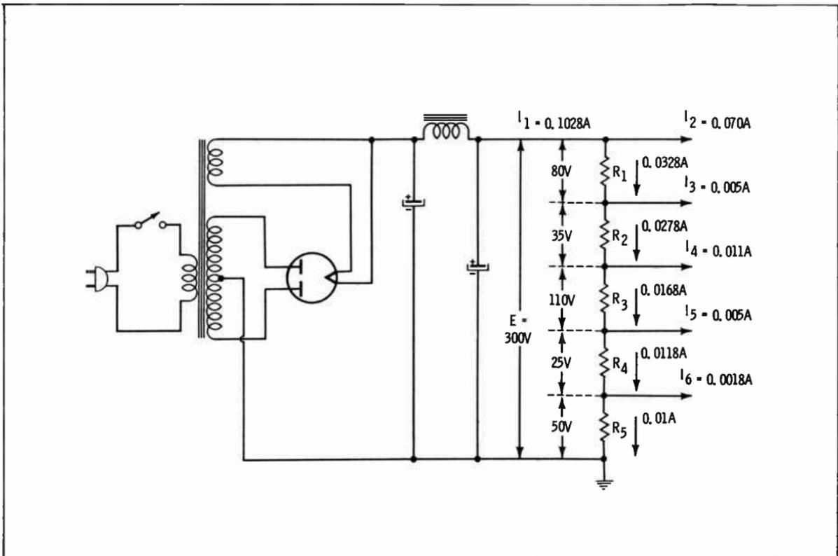
mainder or  $0.1028 - 0.07 = 0.0328$  amperes must pass through resistance  $R_1$ . The value of resistance  $R_1$  may now be calculated by applying Ohm's law to this part of the circuit. We have:
