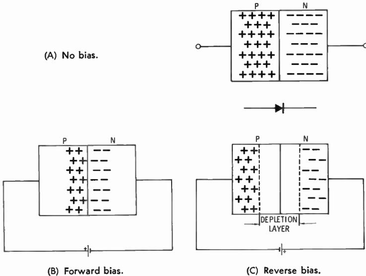
Fig. 21. PN junction characteristics.
