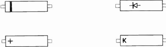
Fig. 8. Various methods of indicating the polarity of semiconductor devices.
