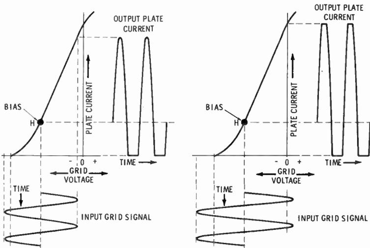
Fig. 13. Dynamic characteristic with class-AB operation.
