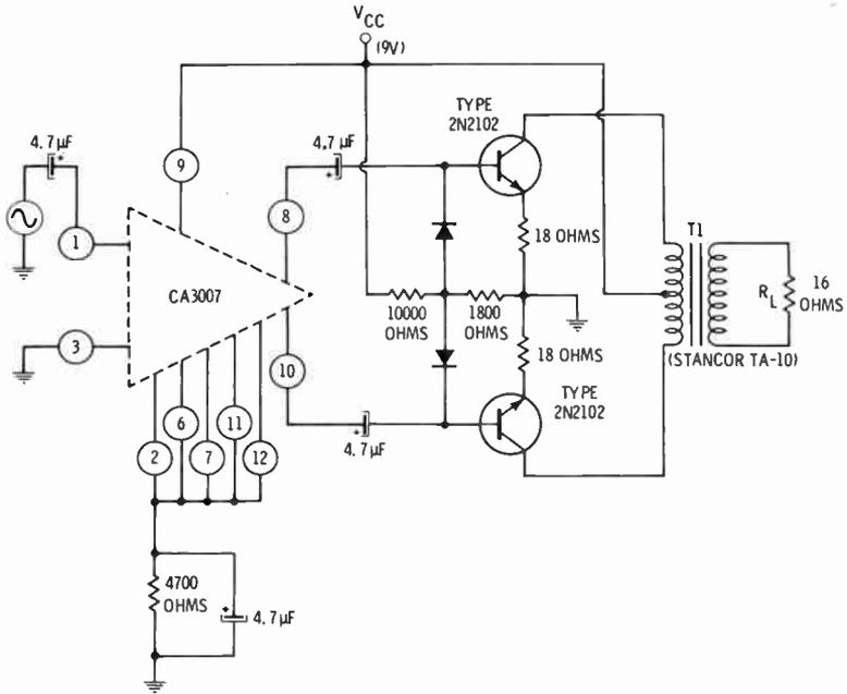
Fig. 31. The RCA CA3007 used as an audio driver for a 30-milliwatt audio amplifier.
