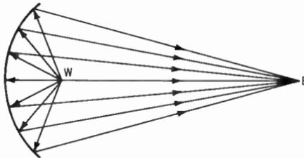
Fig. 4. Focusing of sound waves by a large reflector.
