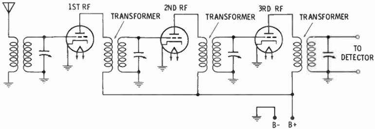
Fig. 12. A three-stage transformer-coupled RF amplifier.
