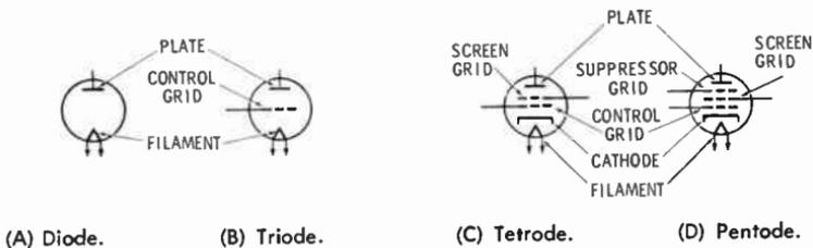
Fig. 6. Vacuum tube schematic representation.
