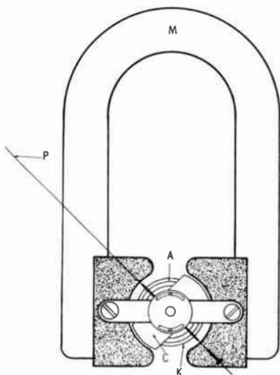
**Fig. 3.** The essential parts of a DC meter are: A, spiral spring; C, coil; K, soft-iron core; M, permanent magnet; and P, pointer. Current passing through the coil causes the moving system to turn against the restraining force of the spiral spring.
