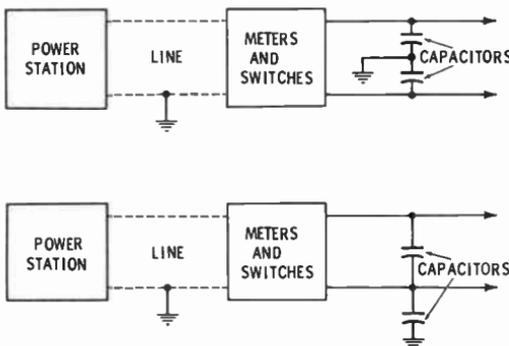
Fig. 5. Method of connecting interference suppressors to prevent noise in an AC wiring system.
