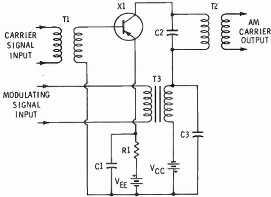
Fig. 11. An amplitude-modulated amplifier with collector injection.
