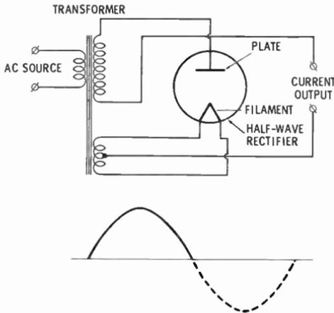
Fig. 8. A half-wave rectifier circuit.
