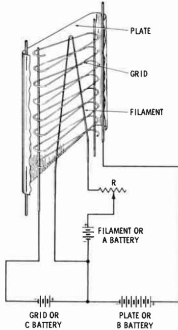
Fig. 11. Triode connected to batteries.
