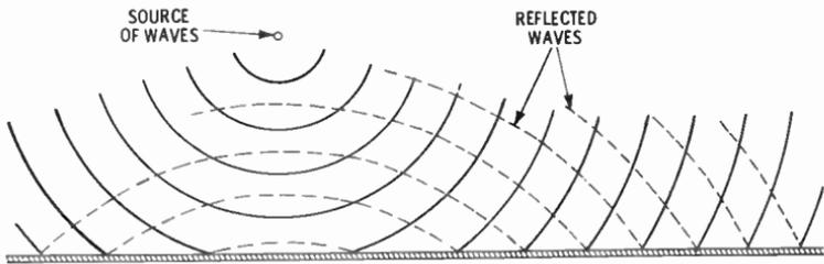
Fig. 6. Reflection of waves from a plane surface.
