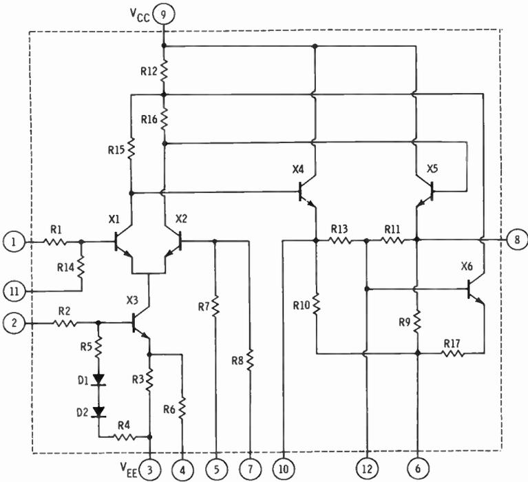
Fig. 30. Schematic diagram of the RCA CA3007 audio driver.
