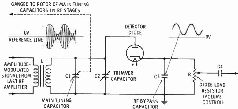
Fig. 4. Circuit action of a diode detector.
