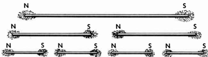
Fig. 7. Effects of breaking a magnet into several pieces.
