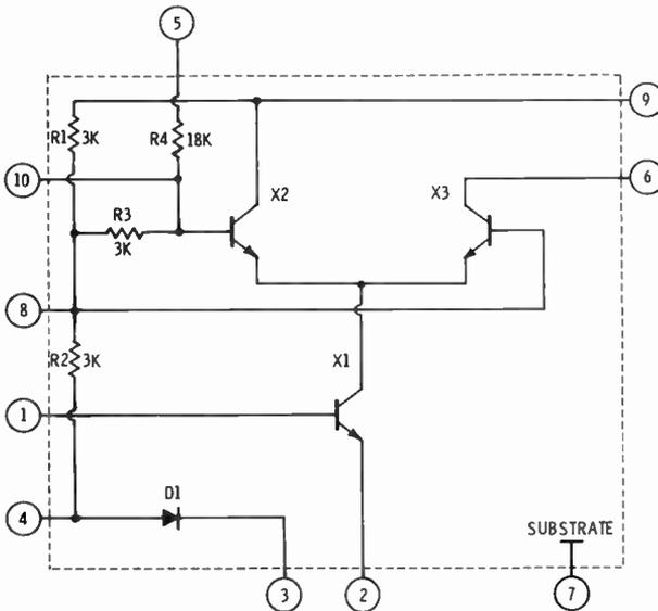
Fig. 26. An integrated amplifier package.
