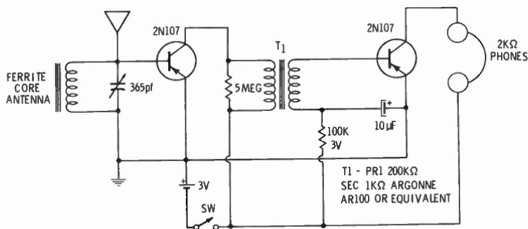
Fig. 21. A two-transistor receiver.
