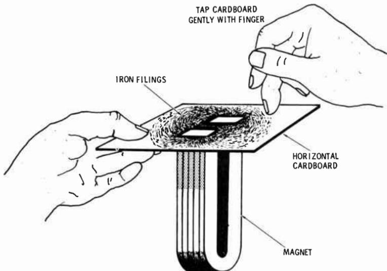
Fig. 9. Results obtained by placing iron filings on cardboard above a horseshoe magnet.
