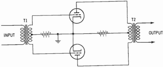
Fig. 11. A basic class-B push-pull amplifier circuit.
