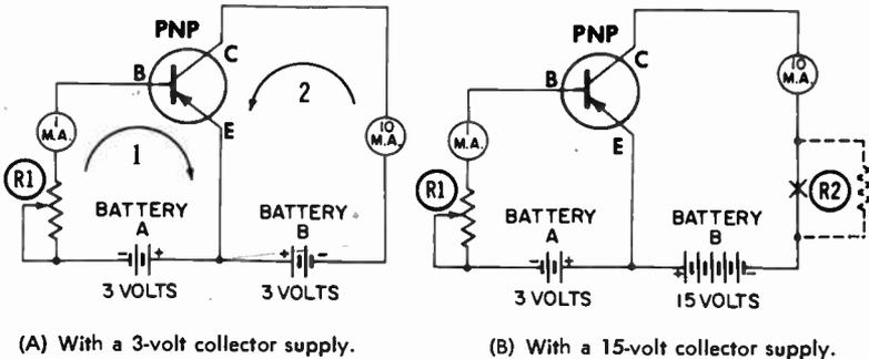
Fig. 17. The common-emitter amplifier.
