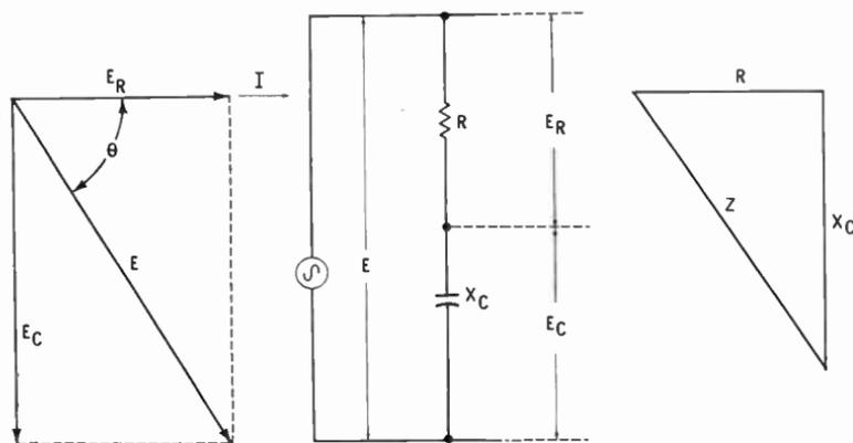
Fig. 4. Combination of resistance ( $R$ ) and capacitive reactance ( $X_C$ ).
