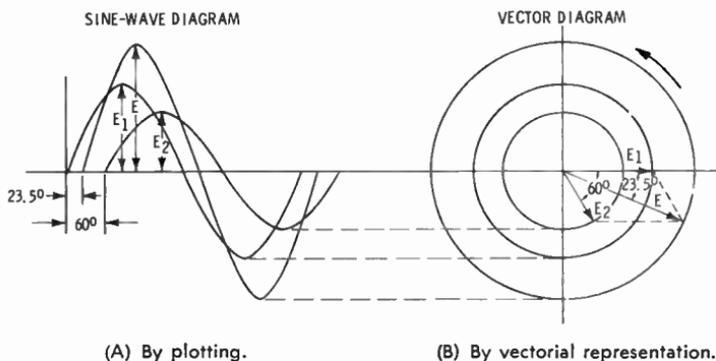
Fig. 17. Addition of two sine waves.
