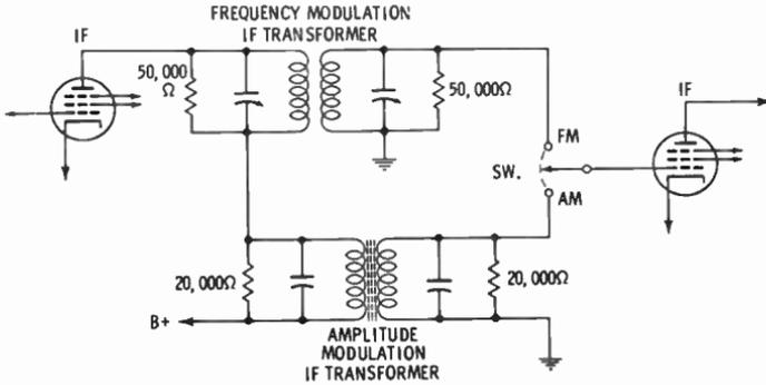
Fig. 38. Use of resistive loading to broaden response characteristics.
