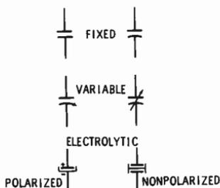
Fig. 15. Common schematic symbols for capacitors.
