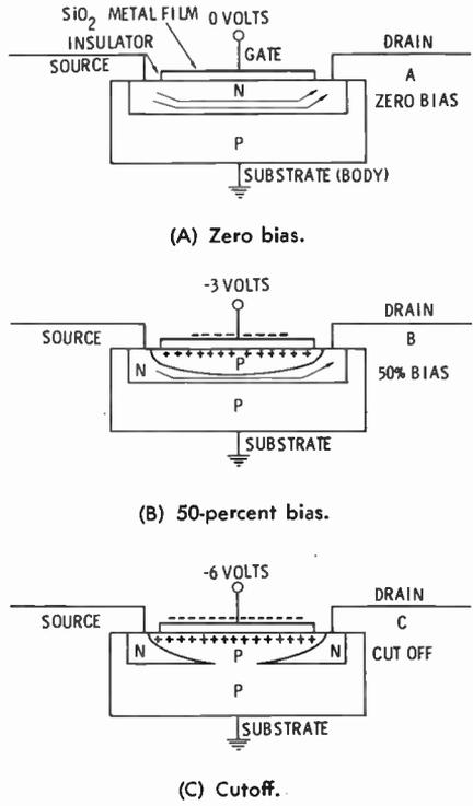
Fig. 24. N-channel depletion MOSFET.
