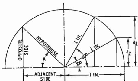
Fig. 14. Diagram illustrating the sine of an angle.
