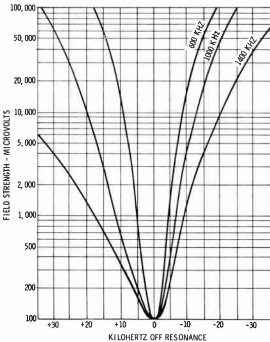
**Fig. 3. Selectivity curve of a typical radio receiver.**
