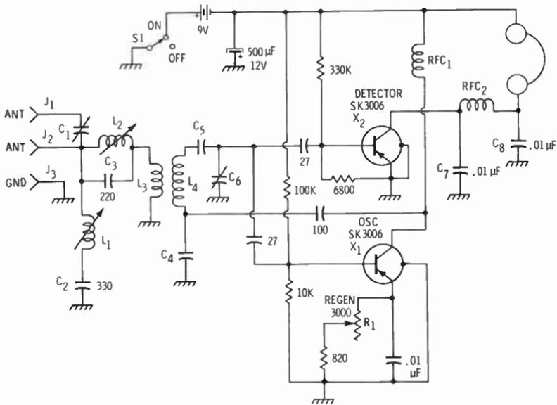
Fig. 16. A simple transistor regenerative receiver.
