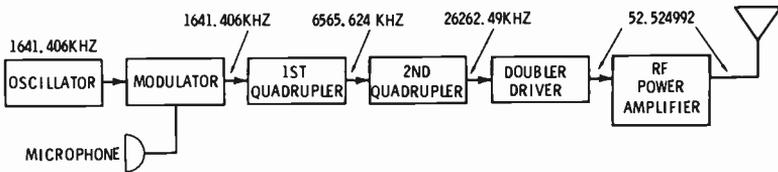
Fig. 13. Block diagram of an FM transmitter using frequency multipliers.
