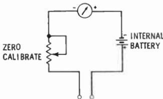
Fig. 16. A basic ohmmeter circuit.
