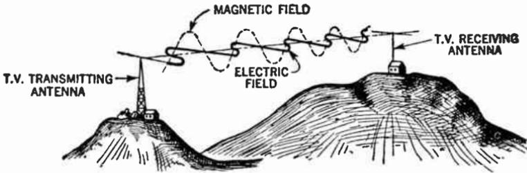
Fig. 2. Electric and magnetic fields of a horizontally polarized wave in relation to transmitting and receiving antennas having the same polarization.
