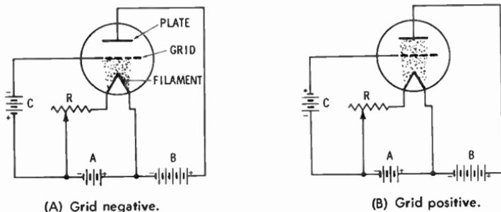
Fig. 12. Effect of grid polarity on plate current.
