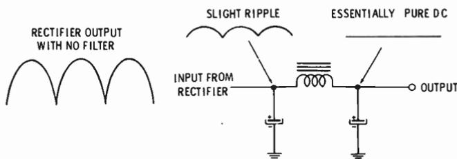
Fig. 10. Smoothing action of a power-supply filter.
