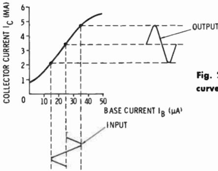
Fig. 22. Dynamic transfer characteristic curve showing linear (class-A) operation.
