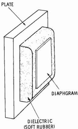
**Fig. 4. Elements of an electrostatic speaker.**
