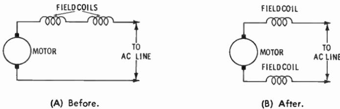
Fig. 4. Diagram illustrating how the internal connections of a universal motor may be altered to reduce interference.
