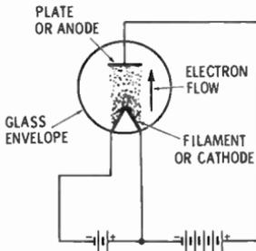
**Fig. 3. The flow of electrons in a vacuum tube.**
