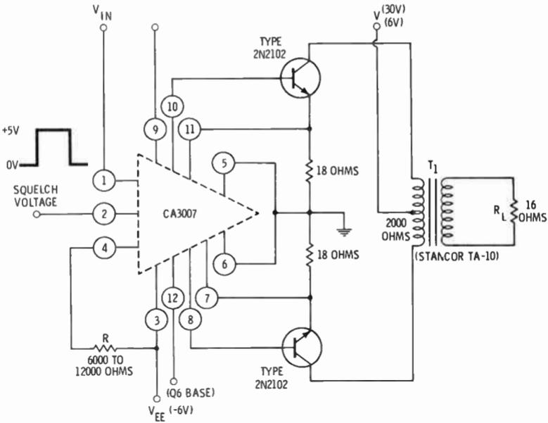
**Fig. 32. The RCA CA3007 used as an audio driver for a direct-coupled 300-milliwatt audio amplifier.**
