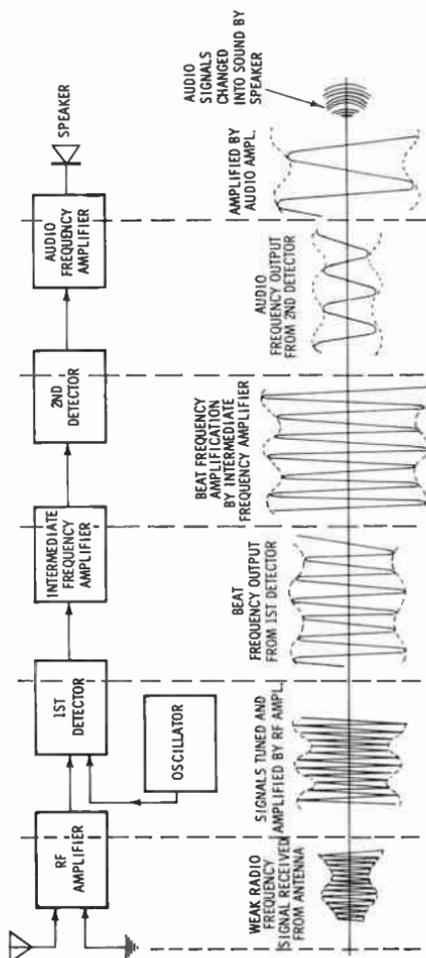
**Fig. 35.** Combination diagram showing arrangement of the different stages of a typical superheterodyne receiver, with charts indicating how the radio signals are modified by each unit.
