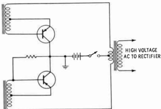
Fig. 17. A transistorized power-supply circuit.
