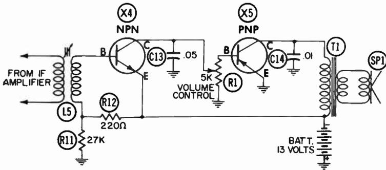
Fig. 35. A DC-coupled amplifier employed in a receiver.
