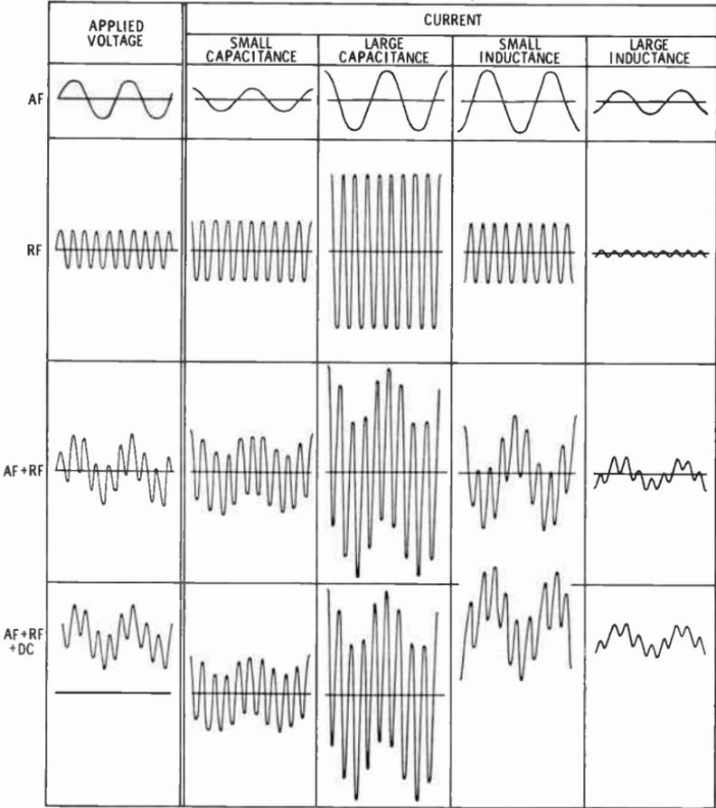
Fig. 12. Filter action of individual series capacitors and inductors.
