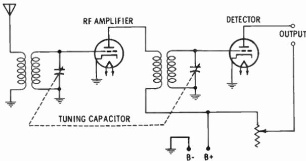
Fig. 27. The principle of a TRF receiver.
