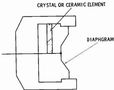
Fig. 8. Basic construction of a crystal and ceramic microphone.
