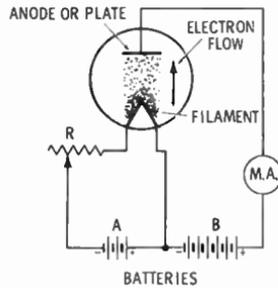
and return through the external plate-supply circuit to the cathode, thus completing the circuit. This flow of electrons is known as the plate current and may be measured by a sensitive current indicator such as a galvanometer.
