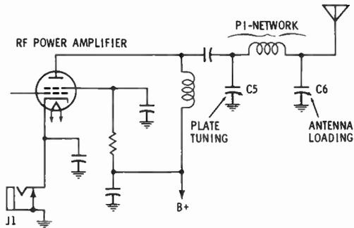
Fig. 3. An RF power amplifier stage using a pi-network to couple the signal to the antenna.
