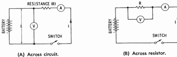
Fig. 15. Two different connections to obtain resistance values.
