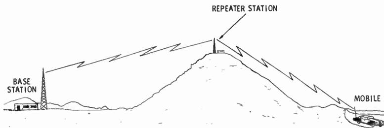
Fig. 4. Two-way radio system using repeater station to extend coverage.
