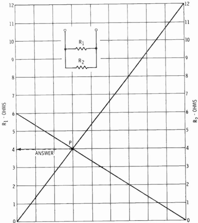
Fig. 24. Graphical solution for two resistors connected in parallel.
