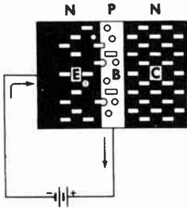
(A) The proper base-to-emitter bias for an NPN-type of transistor.
