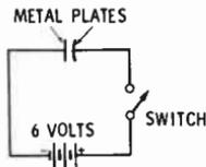
Fig. 2. Direct current applied across a capacitor.
