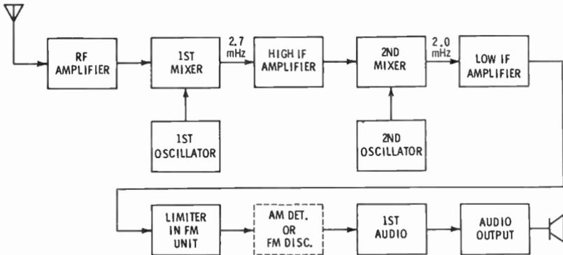
Fig. 50. Block diagram of a dual-conversion superheterodyne receiver.
