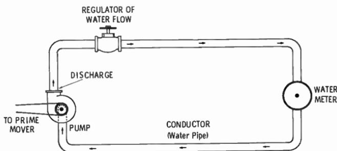
Fig. 8. Water system analogy to an electrical circuit.
