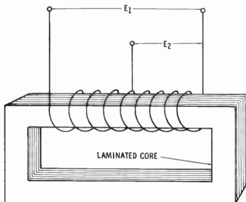
**Fig. 16. Typical autotransformer arrangement.  $E_1$  is the primary voltage and  $E_2$  is the secondary voltage for a step-down voltage ratio.**
