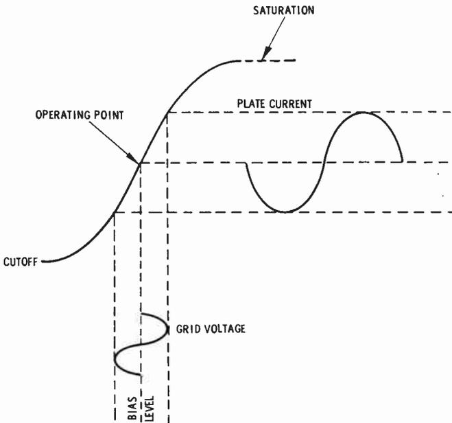
Fig. 8. Characteristic curve of a vacuum tube.
