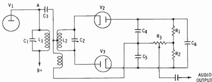
Fig. 46. A ratio detector.
