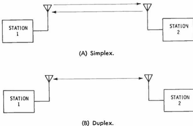
**Fig. 1. Methods of two-way radio operation.**
