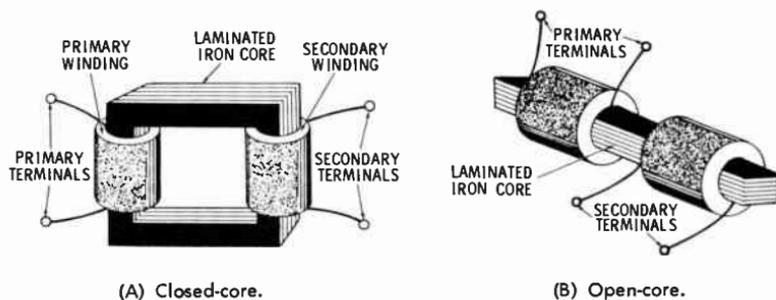
Fig. 13. Two core-type transformers.
