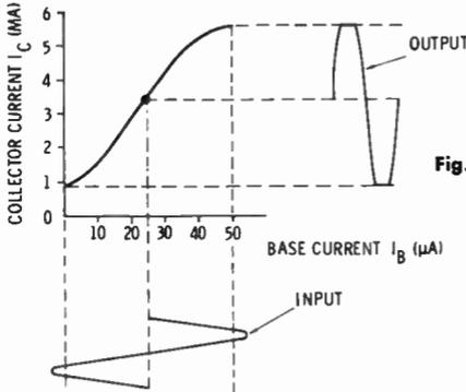
Fig. 23. Dynamic transfer characteristic curve showing overdriving.
