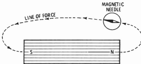
Fig. 33. Method of tracing the direction of magnetic lines of force by means of a magnetic needle.
