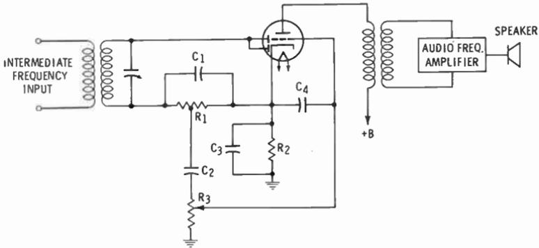
**Fig. 23.** A typical diode-detector circuit using a duplex-diode tube.  $R_1$  is the diode-load resistor. In a typical circuit,  $R_1$  may be tapped so that 80% of the total AF voltage across it is applied to the volume control. This reduces audio distortion and improves the RF filtering.
