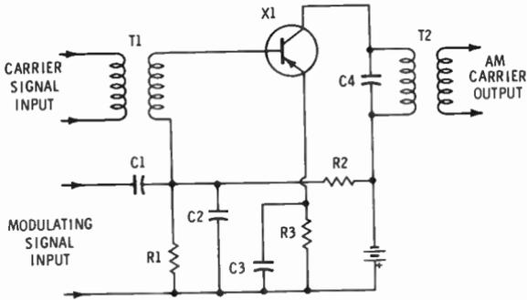
**Fig. 9. An amplitude-modulated amplifier with base injection.**
