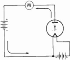
Fig. 1. Circuit connections for current flow through a diode vacuum tube.
