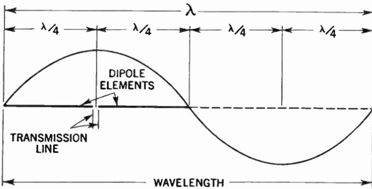
Fig. 5. Relation between wavelength and physical length of dipole elements.
