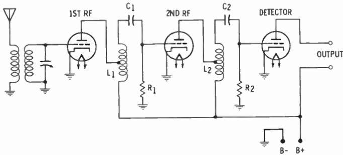
Fig. 11. A two-stage impedance-coupled RF amplifier.
