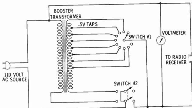
Fig. 1. Schematic diagram of a voltage-compensating circuit.
