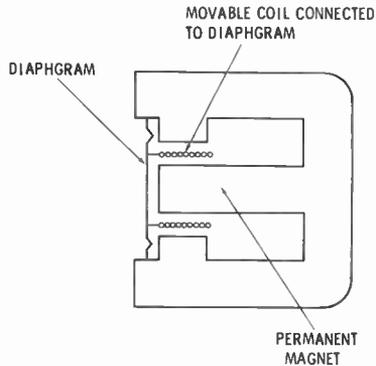
Fig. 7. Basic construction of a dynamic microphone.
