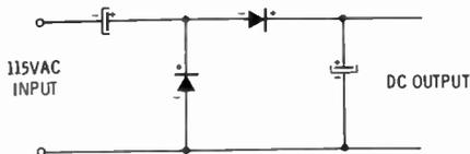
Fig. 14. A voltage-doubler circuit using semiconductor diodes.
