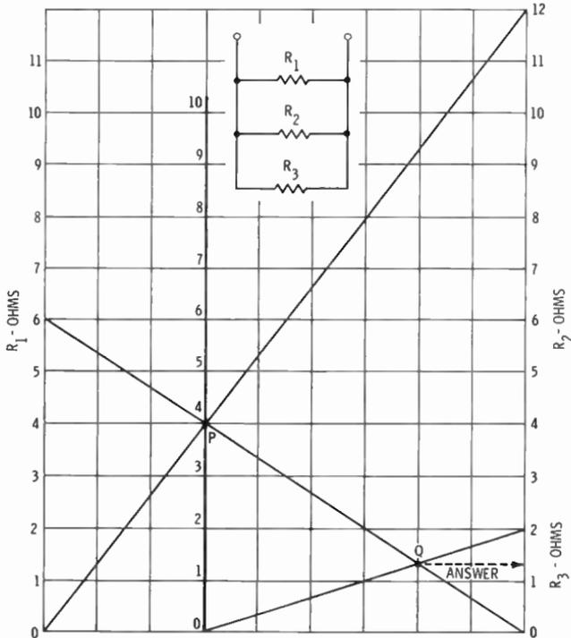
Fig. 25. Graphical solution for three resistors connected in parallel.
