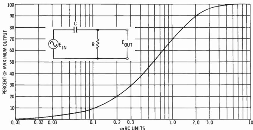
Fig. 5. Universal frequency-response curve for RC series circuits.
