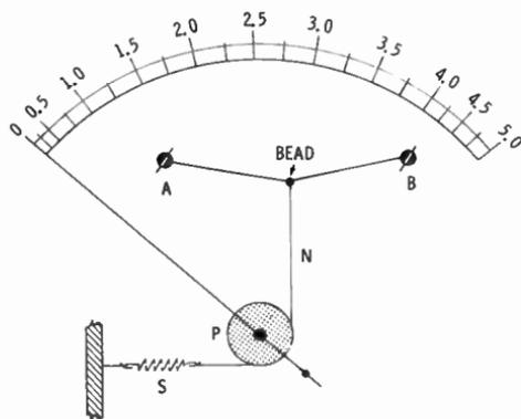
Fig. 10. Simplified diagram showing the construction of a hot-wire instrument.
