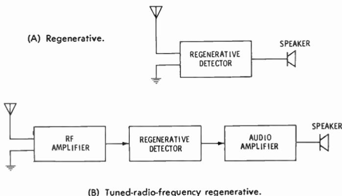
Fig. 2. Block diagrams of two regenerative-type receivers.
