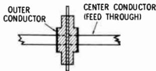
pacitors are generally employed to bring connections through a chassis. The metal portion of the capacitor body is usually soldered to the chassis or fastened with lock nuts to provide good contact.
