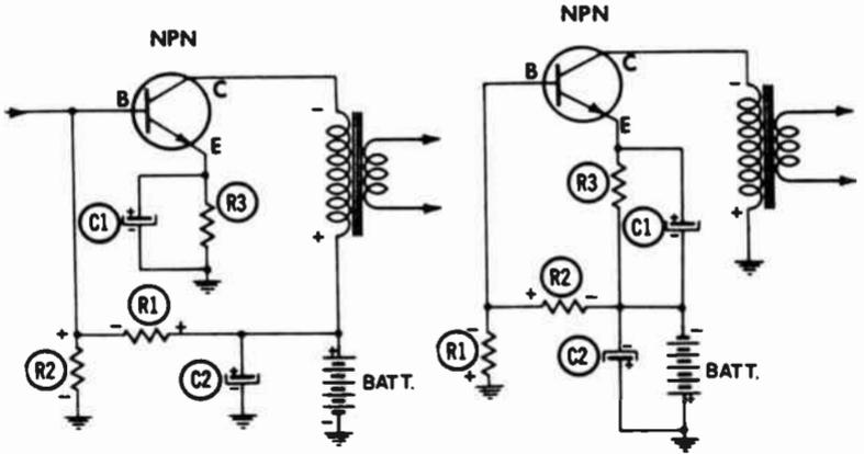
(A) Circuit with negative battery lead grounded.
