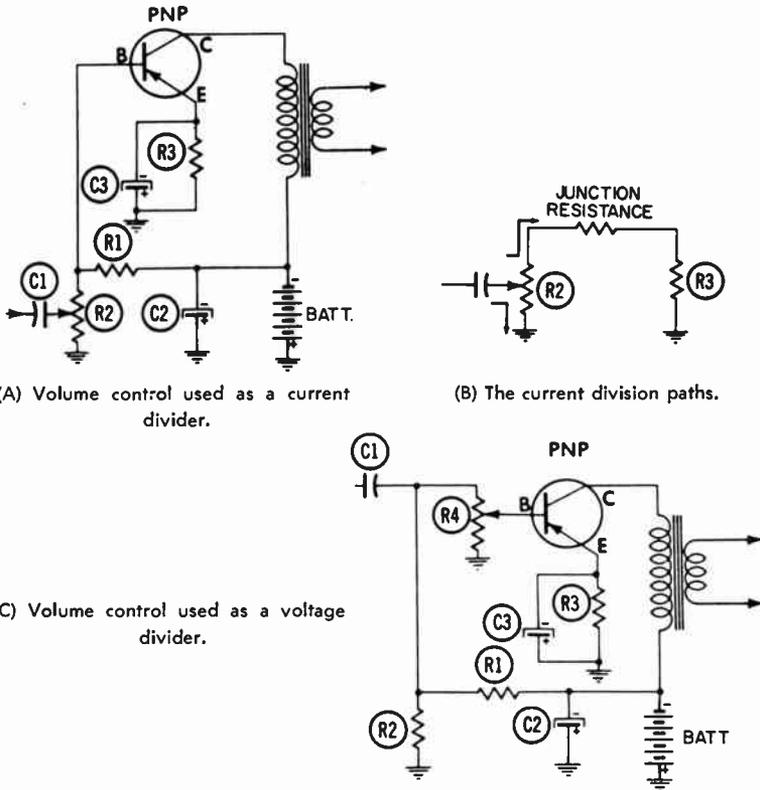
Fig. 29. Different types of volume-control circuits.
