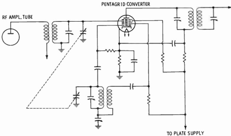
Fig. 30. A pentagrid converter tube employed as an oscillator-mixer in a superheterodyne receiver.
