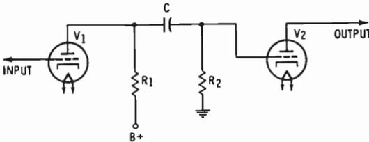
Fig. 32. A resistance-coupled AF amplifier.
