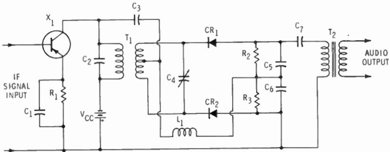
**Fig. 47. A transistor IF amplifier and discriminator stage.**
