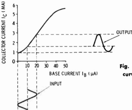
Fig. 24. Dynamic transfer characteristic curve showing nonlinear operation.
