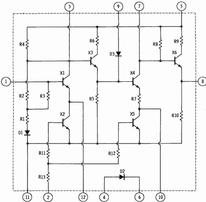
Fig. 38. Schematic diagram of the RCA CA3021 integrated circuit.
