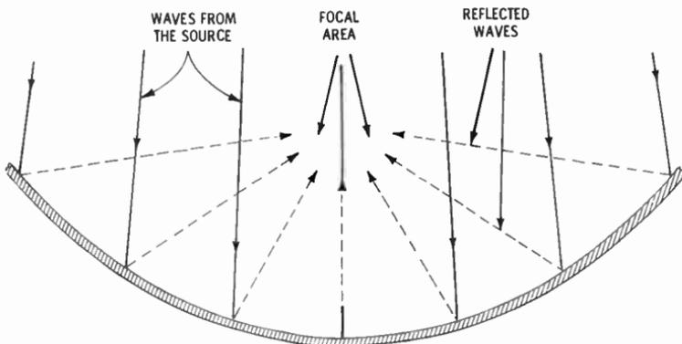
Fig. 7. Reflection of waves from a curved surface. The solid lines show the direction of the original waves, and the dotted lines show the direction and focusing of the reflected waves.
