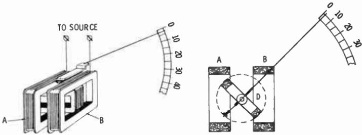
**Fig. 12. Construction of an electrodynamic instrument.**
