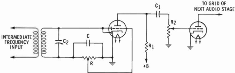
Fig. 22. A diode-biased detector circuit.
