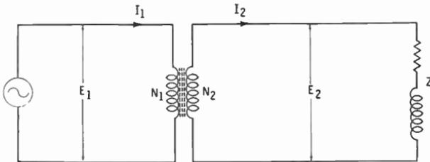
Fig. 12. Simple schematic of a typical transformer.
