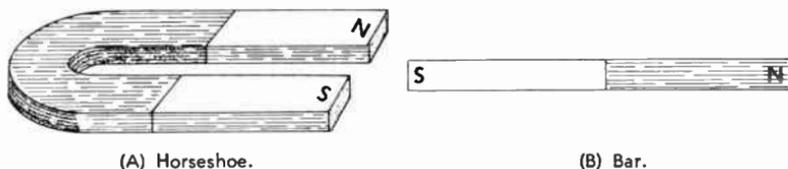
Fig. 8. Two types of permanent magnets.
