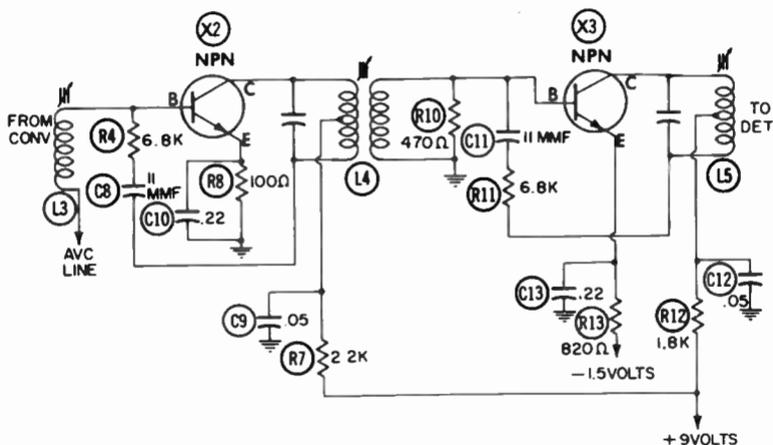
Fig. 36. An IF amplifier with single-tuned transformers.
