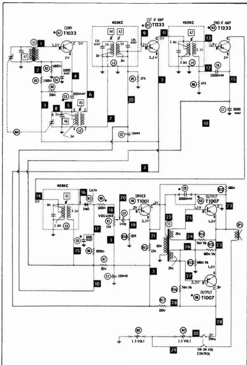
Fig. 31. A transistor superheterodyne receiver.
