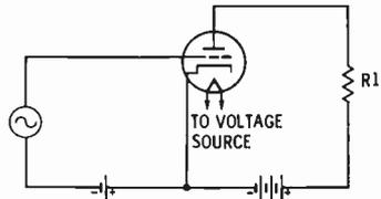
amount of current passing through it. Under the present condition let us assume that 15 volts DC appears across  $R_1$ . At the same time assume that an increase of 50 volts on the plate results in a voltage drop of 25 volts across  $R_1$ , an increase of 10 volts. This is one way of changing the plate current.
