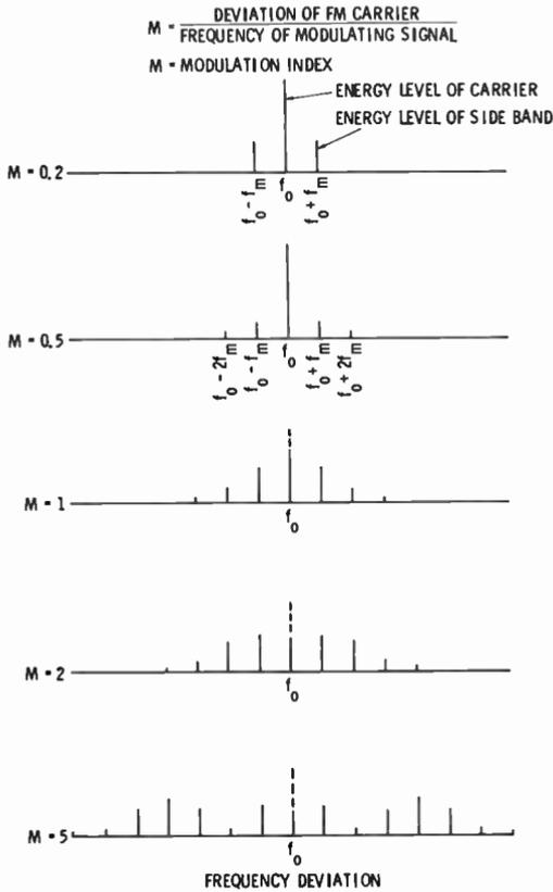
**Fig. 14. Sidebands in frequency-modulated waves.**
