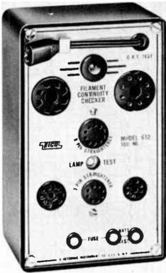
Fig. 21. A filament continuity checker.
