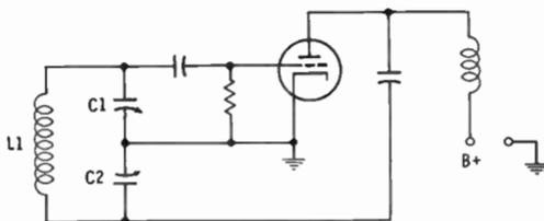
Fig. 19. Colpitts oscillator circuit.
