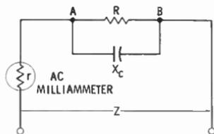
Fig. 3. Connections for measurement of capacity when the capacitor is shunted by a noninductive resistor.
