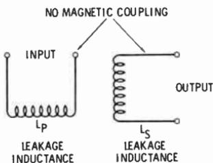
Fig. 5. Representation of a basic transformer with zero magnetic coupling.
