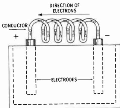
Fig. 6. The movement of electrons from the positive to the negative terminal of a battery.
