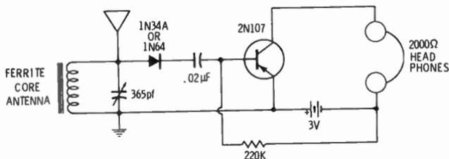
Fig. 20. A one-transistor receiver.
