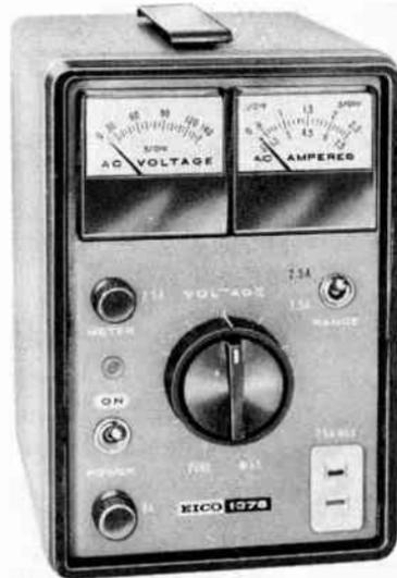
Fig. 2. A metered variable AC bench power supply.
