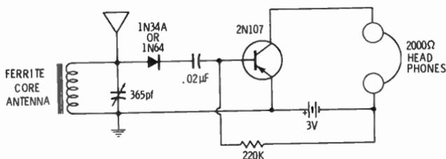
Fig. 20. A one-transistor receiver.
