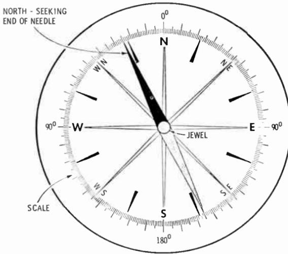
Fig. 3. A typical compass card.
