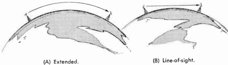
**Fig. 7. Two types of ground-wave propagation.**
