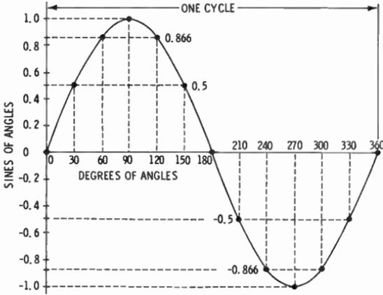
Fig. 15. Relationship between angles in 30° steps and the respective sines. The complete curve, covering angles from 0° to 360°, represents one complete cycle of an alternating current.
