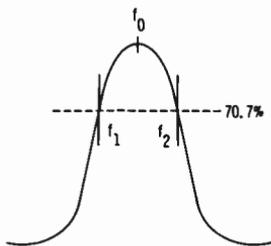
Fig. 4. Bandwidth is measured between the 70.7% maximum voltage points.
