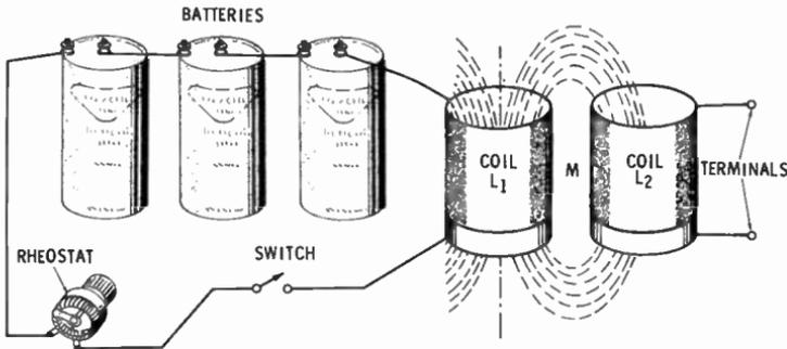
Fig. 6. Illustrating the degree of coupling between two coils.
