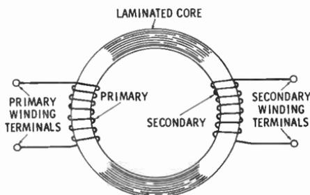
**Fig. 7. A transformer, in its simplest form, consists of two separate and distinct coils of insulated wire wound around a common, laminated iron core.**
