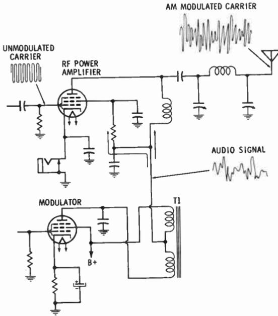
Fig. 6. A transmitter PA stage using plate modulation.
