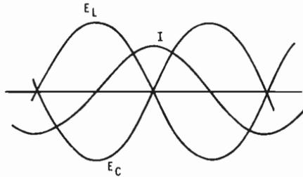
Fig. 13. Voltage and current in a series-resonant circuit.
