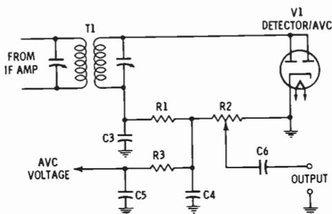
Fig. 5. A typical detector/AVC circuit.
