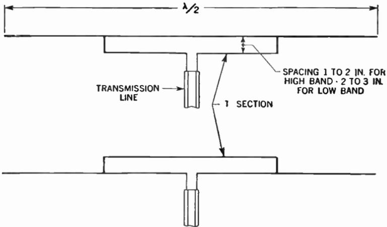
Fig. 8. A T-matched dipole antenna.
