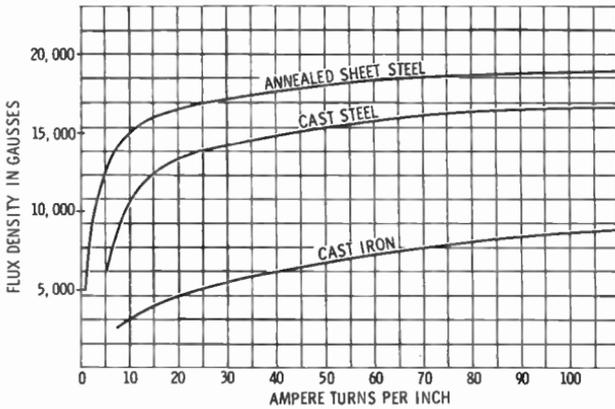
Fig. 37. Typical magnetization curves for cast iron, cast steel, and annealed sheet steel.
