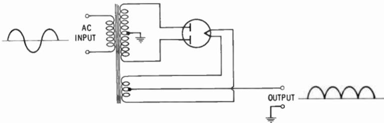
Fig. 3. Full-wave rectifier circuit.
