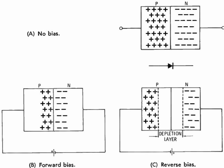
Fig. 21. PN junction characteristics.
