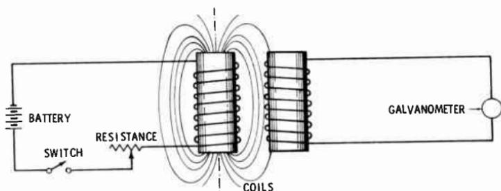
Fig. 1. Diagram showing the action of mutual induction between two coils. One circuit includes a source of electrical energy and a switch; the other includes an instrument to measure current but has no energy source. During an increase or decrease in current, as when the switch is closed, current is induced in the secondary. This current in the secondary flows in a direction opposite to that of the current in the primary.
