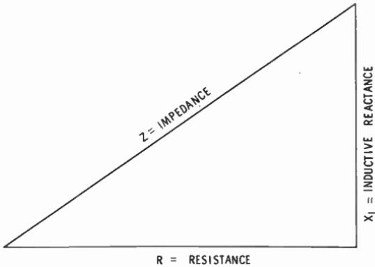
Fig. 2. Vector relationship between inductive reactance and resistance.
