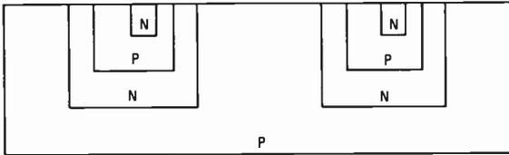
Fig. 27. A pair of NPN transistors diffused into a P-type substrate.
