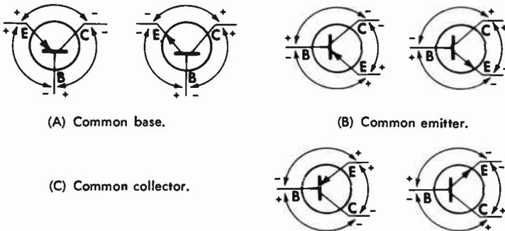
Fig. 12. The polarities of transistor voltages in the three circuit configurations.
