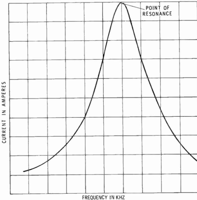
Fig. 11. Current versus frequency variations in a resonant circuit.
