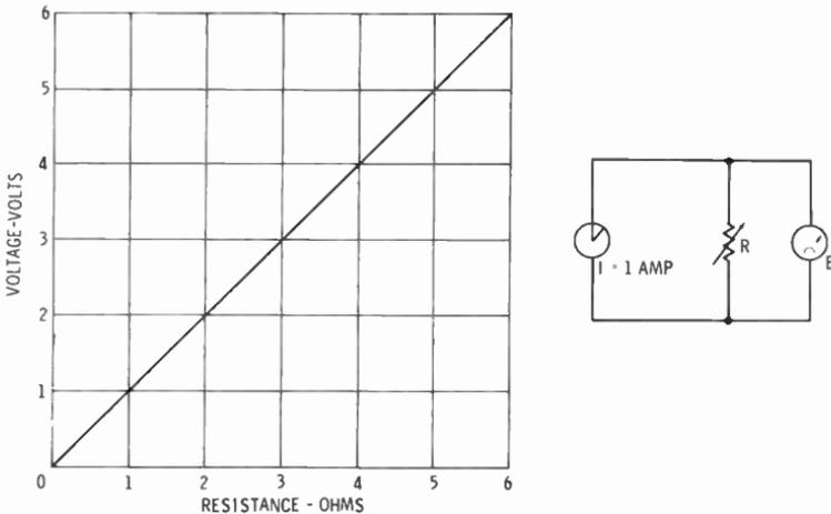
**Fig. 22. Relation between voltage and resistance, with current constant.**
