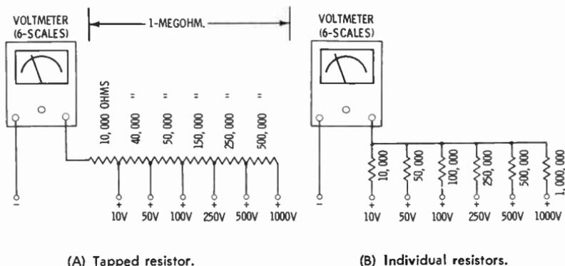
Fig. 7. Two methods of connecting multipliers to a voltmeter.
