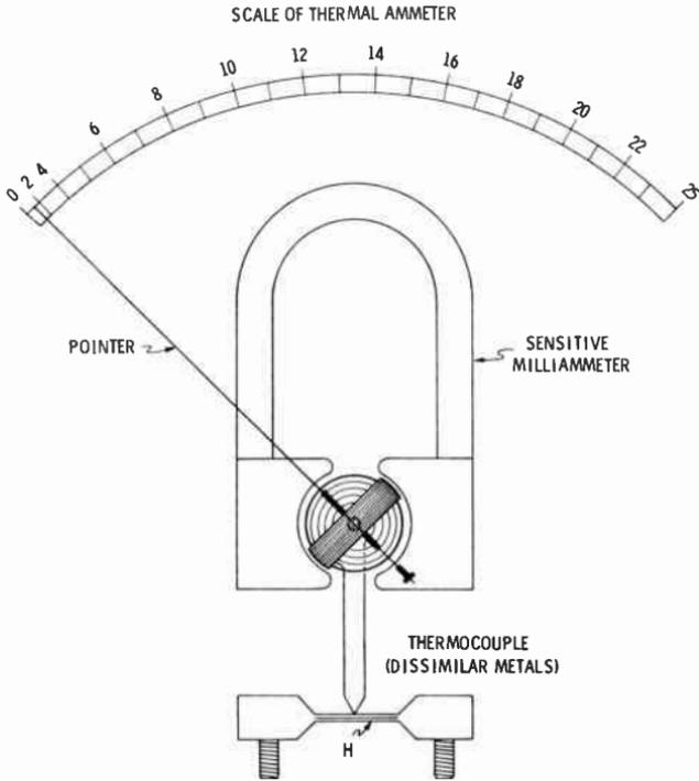
Fig. 11. Thermocouple arrangement and connection to a milliammeter.
