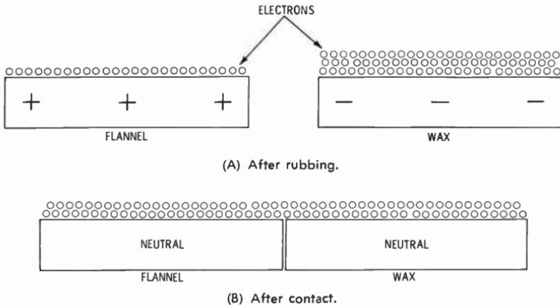
Fig. 5. Distribution of electrons in flannel and wax.
