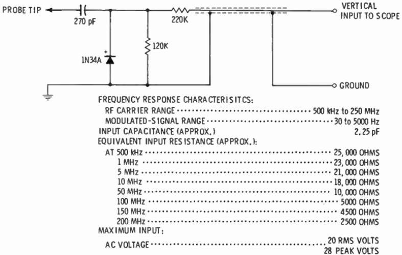
**Fig. 9 Typical demodulator probe and specifications.**
