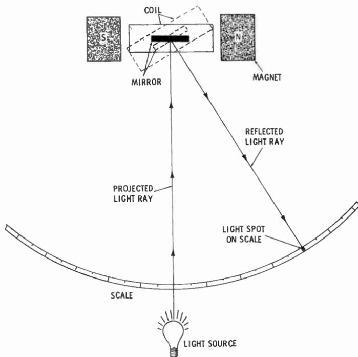
Fig. 2. Method used to obtain an enlarged view of a meter indication.
