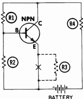
(C) Voltage-divider biasing with DC compensation.
