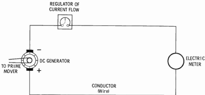
Fig. 9. Equivalent electrical circuit of the water system in Fig. 8.
