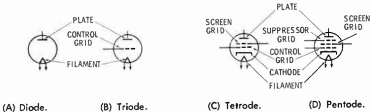
Fig. 6. Vacuum tube schematic representation.
