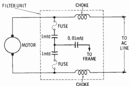
Fig. 6. Interference-suppressor filter added to a washing machine.
