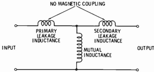
Fig. 2. Equivalent circuit for a basic transformer.
