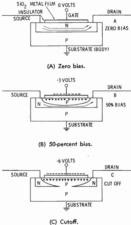
Fig. 24. N-channel depletion MOSFET.
