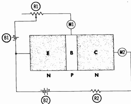
Fig. 10. Circuit illustrating basic operation of the NPN-type of transistor as an amplifier.
