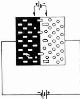
Fig. 7. Result of connecting a battery to reduce the potential hill (forward biasing).
