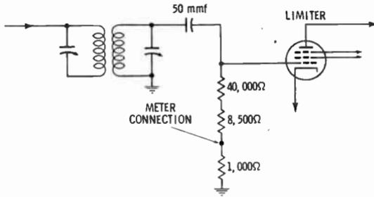
Fig. 43. A limiter circuit in which an indicating meter may be connected.
