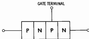
semiconductor acts as an open circuit to electron flow until an appropriate gate signal is applied to the third terminal. When this occurs the device is triggered into conduction and from then on operates as a conventional semiconductor diode. The action of this rectifier is similar to that of a thyatron tube.
