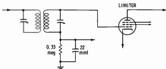
Fig. 42. Another type of limiter circuit employed in FM receivers.
