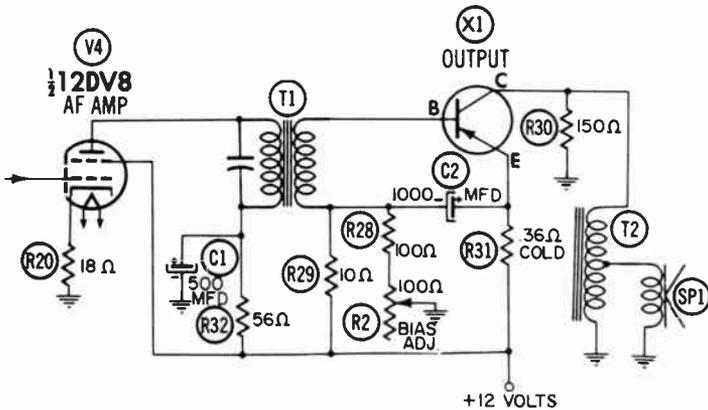
Fig. 33. An example of a vacuum-tube stage driving a transistor stage.
