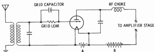
Fig. 26. A grid-leak and capacitor detector circuit.
