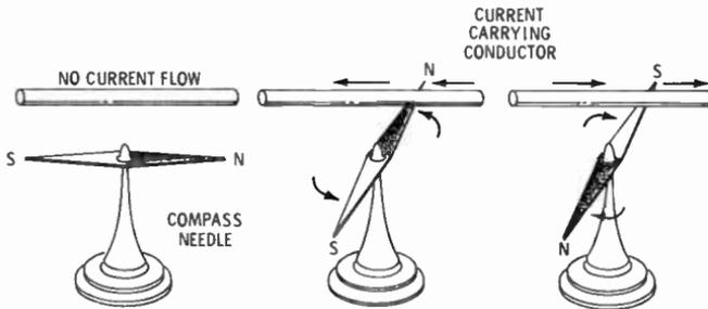
Fig. 31. Deflection of a compass needle when held near a current-carrying conductor.
