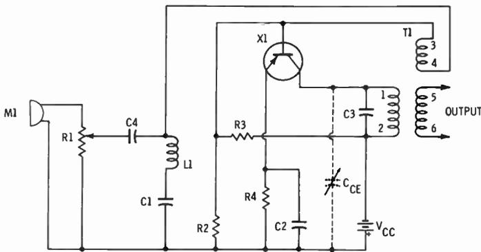
Fig. 8. An amplitude-modulated oscillator with base injection.
