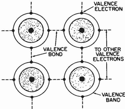
Fig. 4. Composition of the crystal structure from atoms.
