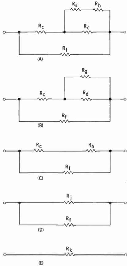
Fig. 30. A method by which a series-parallel combination of resistances may be reduced to an equivalent resistance.
