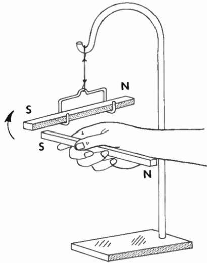
The foregoing facts also point to the conclusion that in any unmagnetized piece of iron, the atoms which comprise it are not lined up in any particular order; that is, the electrons circling the nuclei of the iron atoms produce magnetic effects, but these effects cancel
