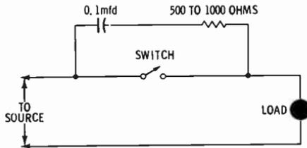
Fig. 7. Switch-filter connection.
