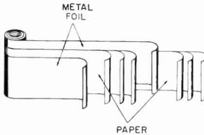
Fig. 6. Basic construction of a paper capacitor.
