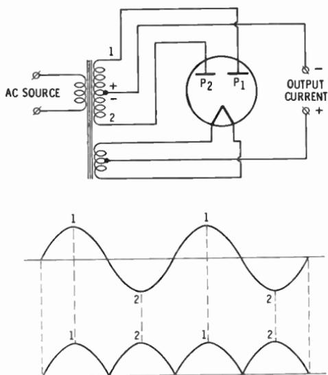
Fig. 9. A full-wave rectifier circuit.
