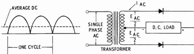
Fig. 4. Rectifier connections in a center-tapped, single-phase circuit.
