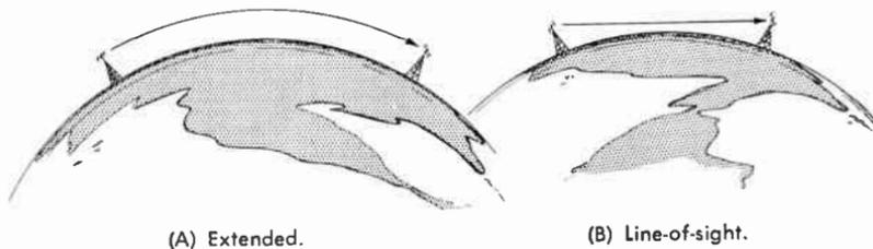
**Fig. 7. Two types of ground-wave propagation.**
