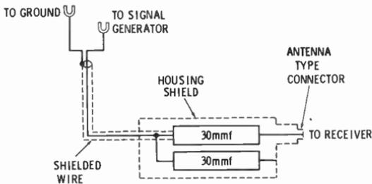
Fig. 5. Dummy antenna for use in alignment of auto radios.
