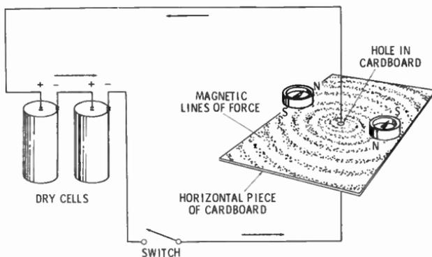
**Fig. 32.** Experiment showing direction of lines of force in the magnetic field of a conductor carrying an electrical current.
