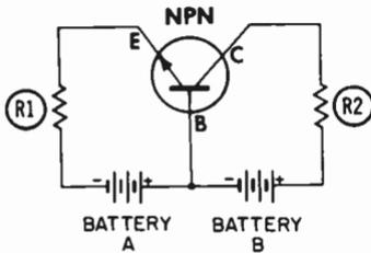
Fig. 16. Biasing common-base circuits.
