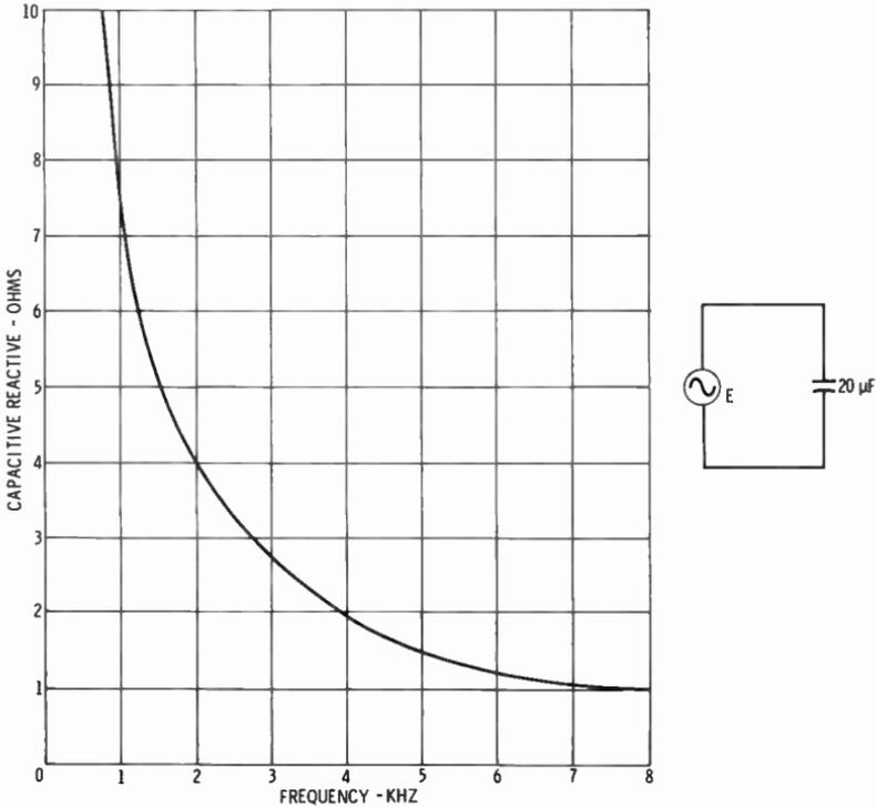
Fig. 5. Capacitive reactance versus frequency.
