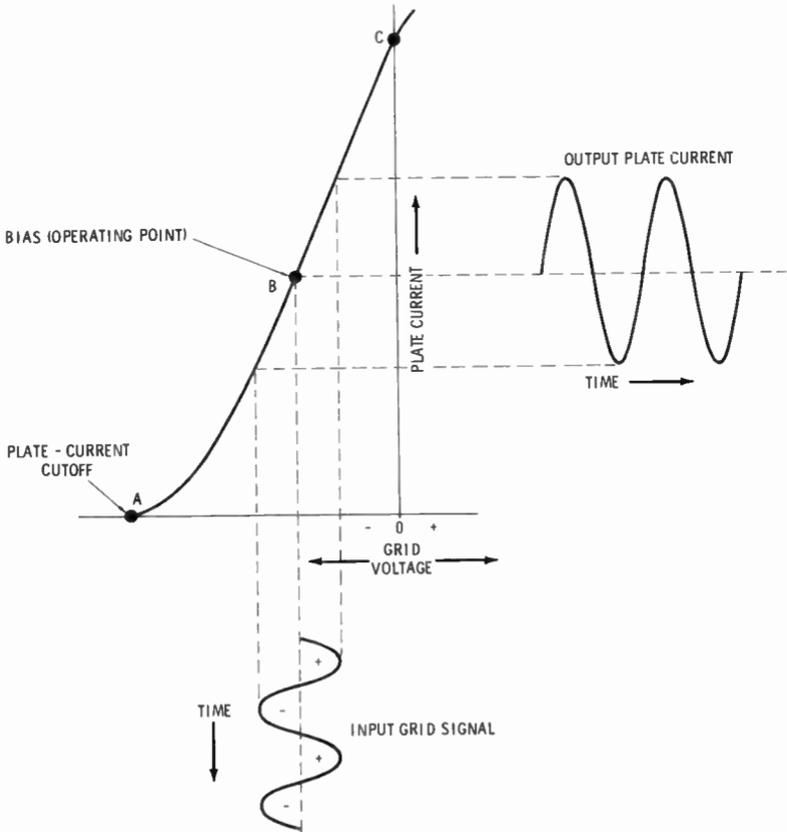
Fig. 7. Characteristic curve with class-A operation.
