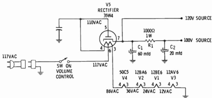
Fig. 18. A typical AC-DC power-supply circuit.
