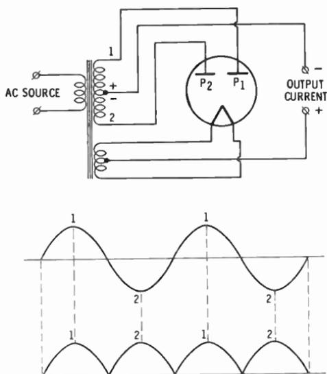
Fig. 9. A full-wave rectifier circuit.
