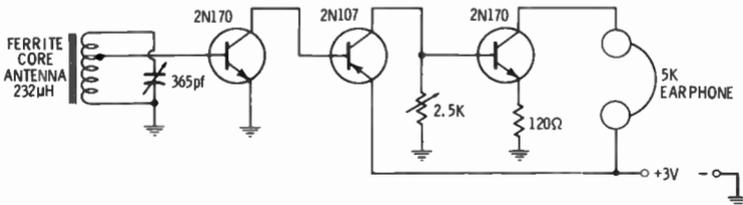
Fig. 25. A three-transistor receiver.
