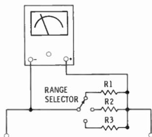
**Fig. 9. A multirange current meter.**
