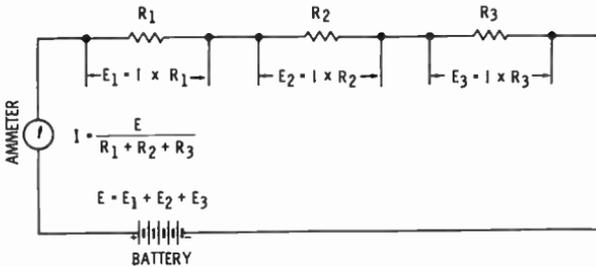
Fig. 19. Simple circuit with three resistances connected in series.
