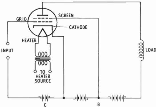
Fig. 14. Connection of electrodes in a tetrode.
