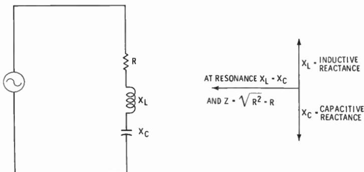
Fig. 10. A series-resonant circuit.
