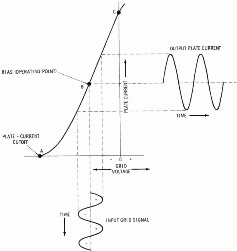
Fig. 7. Characteristic curve with class-A operation.
