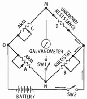
resistance D is equal to the ratio between resistance A and resistance B, then M and N will be at equal voltages. To determine if this condition is obtained, a sensitive galvanometer placed in a branch wire between M and N will show no deflection when M and N are at equal voltages or when the four resistances of the arms "balance" one another by being in proportion, thus:
