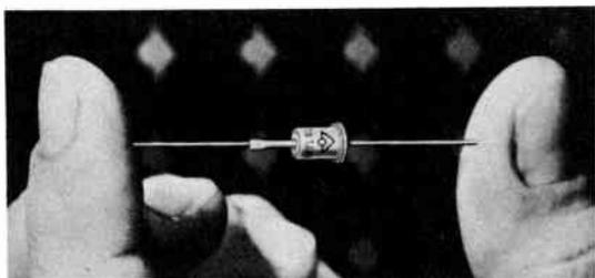
Fig. 4. A silicon diode with flexible wire leads.
