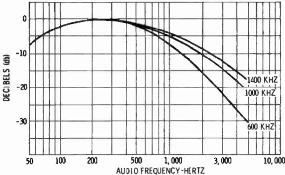
Fig. 6. Fidelity characteristics of a typical broadcast receiver.
