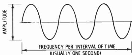
Fig. 6. Characteristics of a radio wave.
