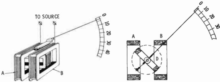
**Fig. 12. Construction of an electrodynamic instrument.**
