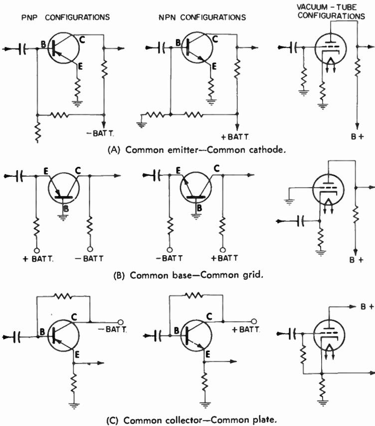
Fig. 21. Transistor circuits and their vacuum-tube counterparts.
