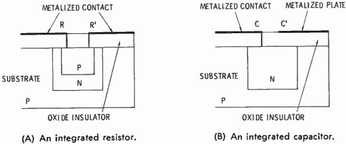
Fig. 28. How integrated resistors and capacitors are formed.
