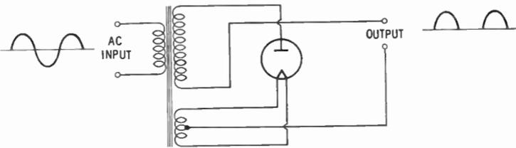
Fig. 2. Basic half-wave rectifier circuit.
