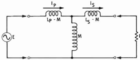
Fig. 11. Illustrating voltage decrease under load.
