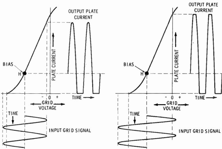
Fig. 13. Dynamic characteristic with class-AB operation.
