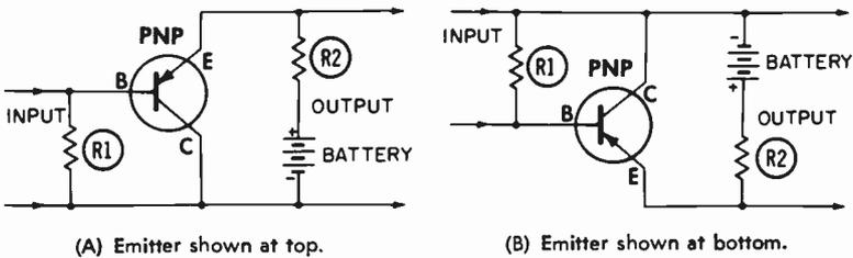
Fig. 15. Method of biasing common-collector circuits.
