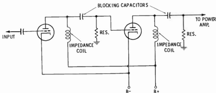
Fig. 33. An impedance-coupled AF amplifier.
