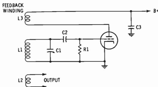
Fig. 17. "Tickler coil" oscillator circuit.
