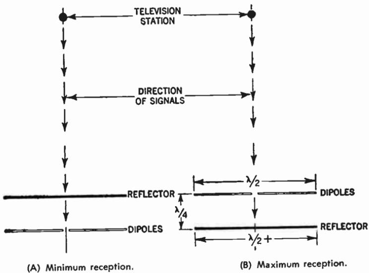
Fig. 9. Location of reflector element for maximum reception.
