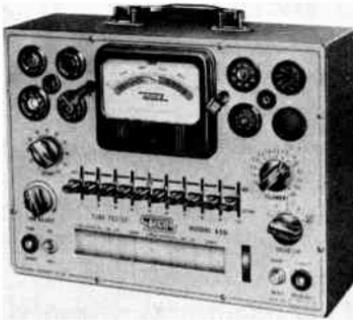
Fig. 22. An emission-type tube tester.
