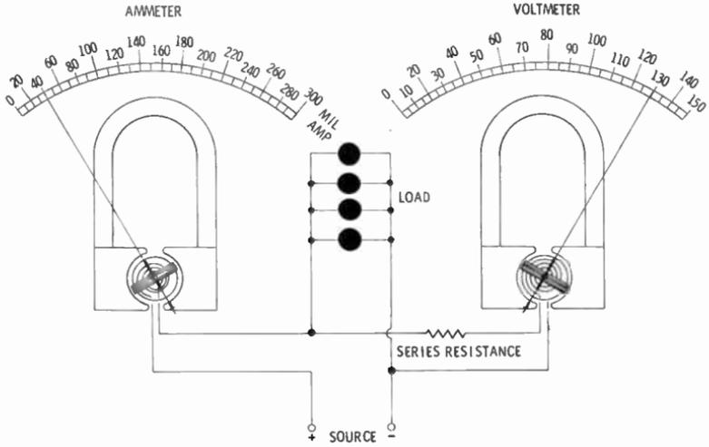
Fig. 5. Methods of connecting meters to indicate current and voltage.
