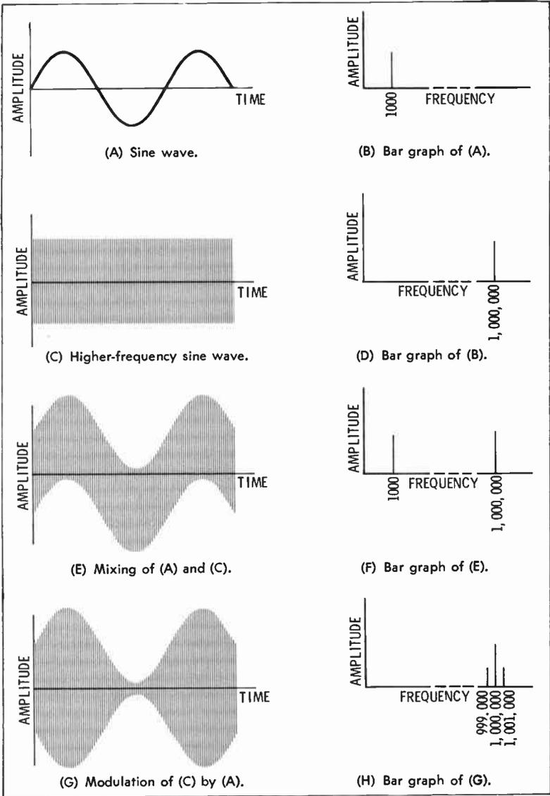
Fig. 3. Waveforms and their bar graphs.
