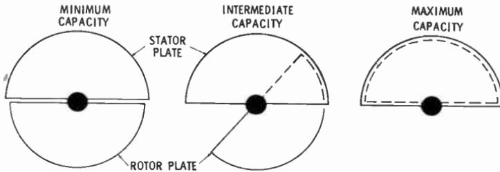
Fig. 10. Relationship between capacitor rotation and capacitor value.
