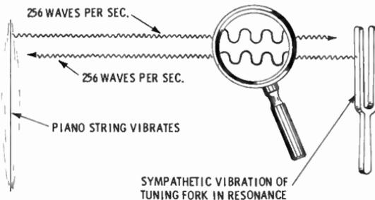
Fig. 12. Sympathetic vibration of tuning fork with vibrating piano string when tuned to the same pitch.
