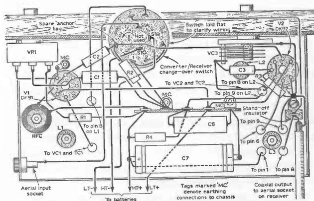
Fig. 40. Complete underchassis wiring diagram.
