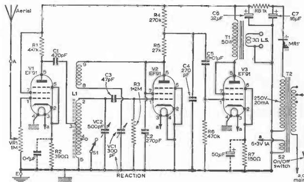
Fig. 16. The receiver circuit.
