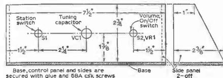
Fig. 47. Front and side views of the receiver case.
