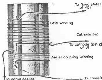
Fig. 2. Details of the aerial coil, L1.
