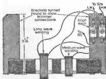
Fig. 55. Mounting and wiring details of ferrite rod aerial and trimmers.
