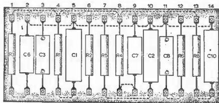
that practically all the small components can be mounted on to two groupboards which can be completely assembled and wired up before fitting to the chassis.
