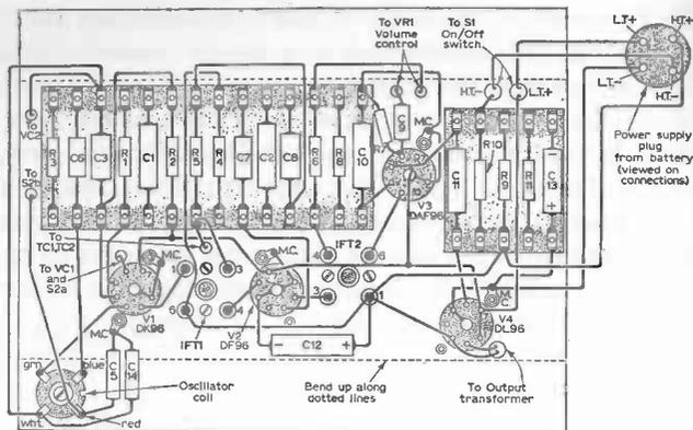
Fig. 54. Underchassis wiring extra to the group board wiring.
