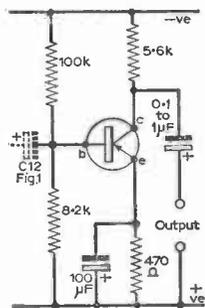
Fig. 30. An alternative circuit arrangement, operating Tr4 in the common-emitter mode.
