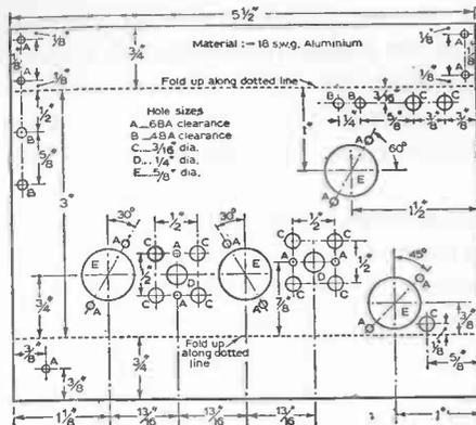
Fig. 51. Dimensions and drilling details of the chassis.
