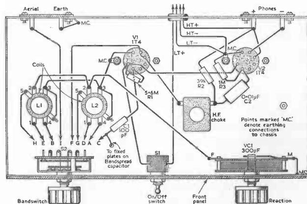
Fig. 21. Underchassis connections.
