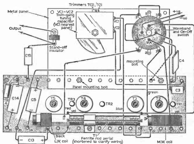
Fig. 34. Wiring on top of tag board and connections to aerial and front panel.
