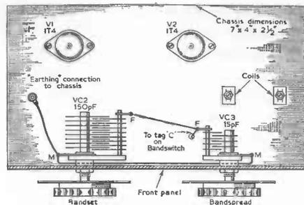
Fig. 20. The simple layout of components.
