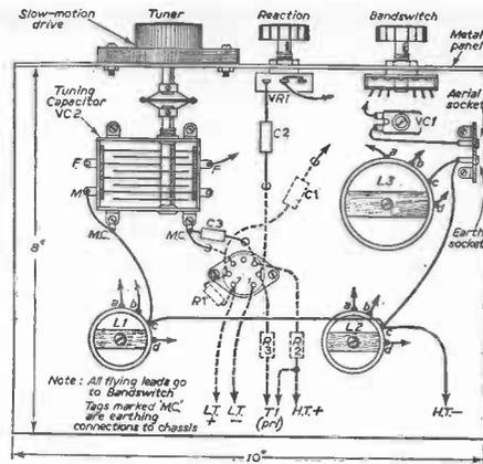
Fig. 24. Component-layout and wiring of the detector.
