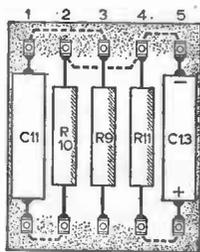
Fig. 50. Wiring of an auxiliary group board.
