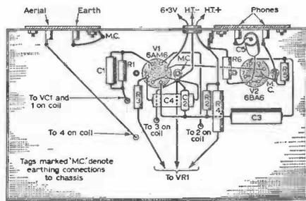
Fig. 4. The main wiring underchassis.
