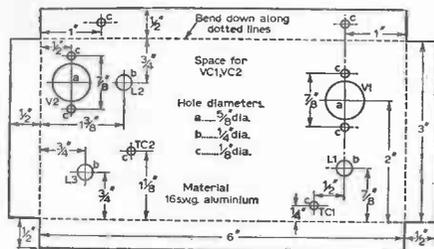
Fig. 37. Drilling dimensions of the aluminium chassis.
