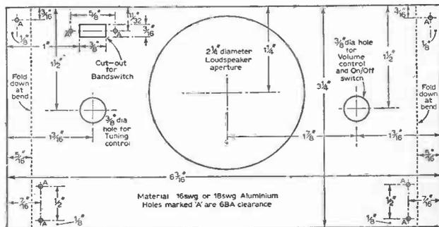
Fig. 52. Dimensions of the front panel.
