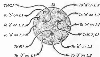
Fig. 25. S1 bandswitch connections.
