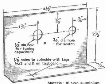
Fig. 32. Details of the panel which carries the tuning capacitor and wave-change switch, and which is bolted to the component tag board.
