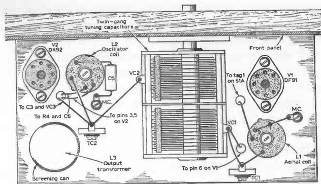
Fig. 39. Chassis component layout.
