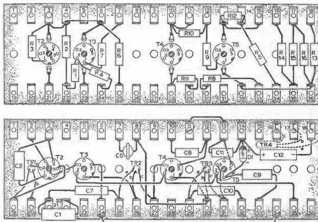
Fig. 33. Top—main positive- and negative-line wiring. Note connections of transformer cans to the positive-line. Bottom—remainder of tag board wiring.
