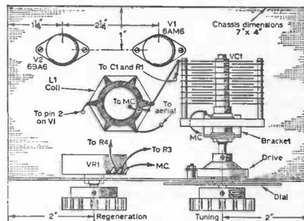
Fig. 3. Components and connections above chassis.
