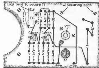
Fig. 10. Front-of-panel wiring details.
