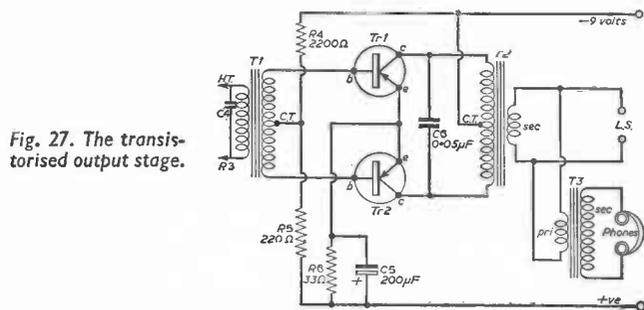
Fig. 27. The transistorised output stage.
