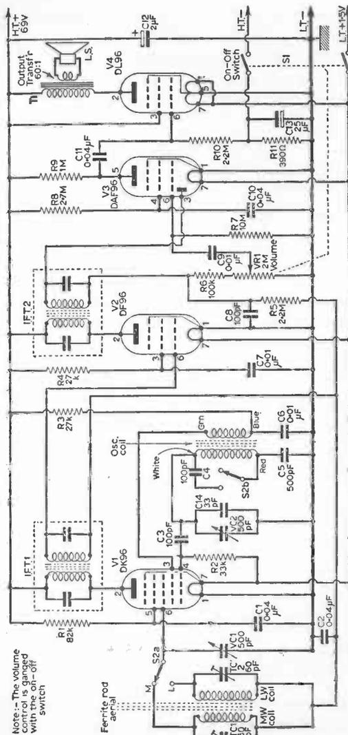
Fig. 48. The battery-operated circuit.
