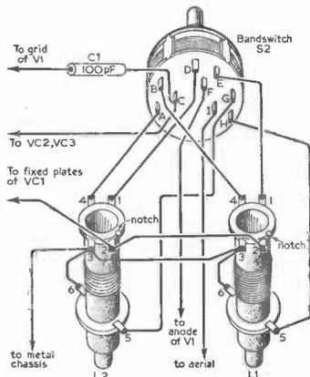
Fig. 22. Details of the switch and coil interconnections.
