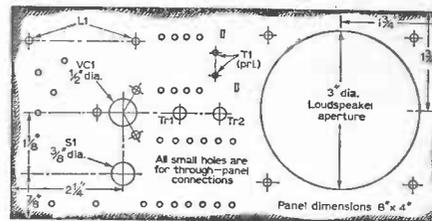
Fig. 8. Drilling details of the Paxolin panel.
