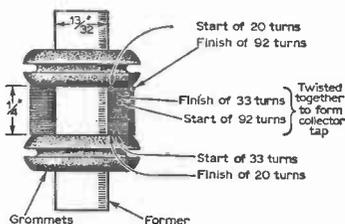
Fig. 43. Construction details of one of the r.f. transformers.
