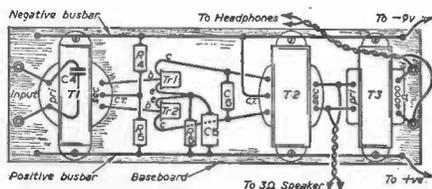
Fig. 28. Wiring of the output stage.
