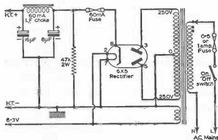
Fig. 6. Circuit of the power pack.
