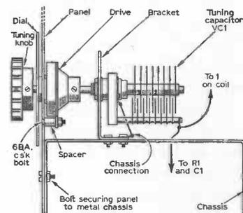
Fig. 5. Details of the tuning drive mechanism.
