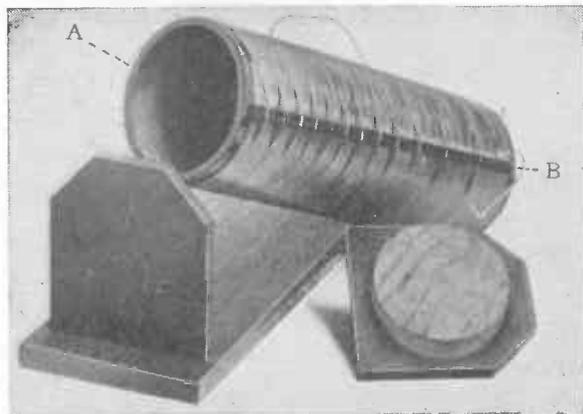
Fig. 93.—Photograph showing Method of Making Tappings from Cylindrical Coil
