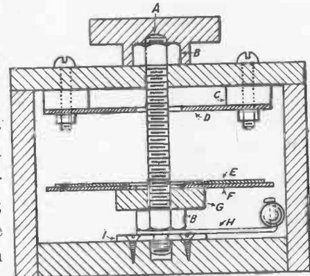
Fig. 156.—Section of Encased Condenser
