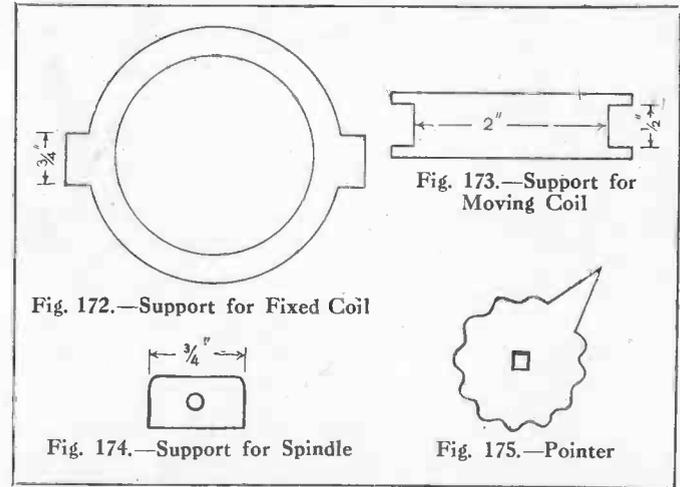
ring the same size as the coil, leaving a tab at each end as shown in Fig. 172. The coil is then placed on this, and tape is wound round both coil and wood to hold them together. Rubber tape will be found rather too thick and messy for this, and ordinary black tape fastened on with thin glue will make a much neater job. The inner coil should also be taped in the same way, but without a wooden support. To hold the inner coil a piece of wood should be cut as shown in Fig. 173.
