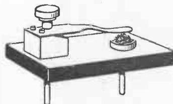
Fig. 26.—Carborundum-steel Detector
