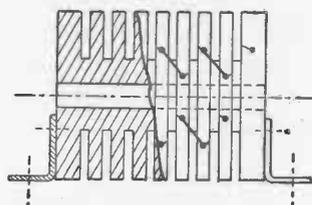
Fig. 201.—Former for Air-core Transformer
