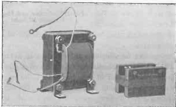
Fig. 196.—Two Patterns of Interval Transformer.
