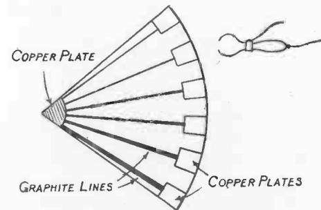
Fig. 151.—A Simple Variable Grid Leak
