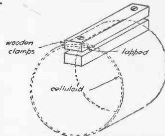
Fig. 171.—Method of Making Celluloid Cover
