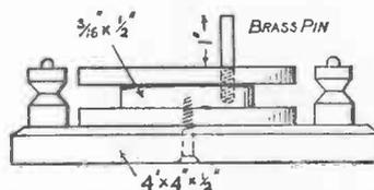
Fig. 121.—Hard-wood Former for Reaction Coil
