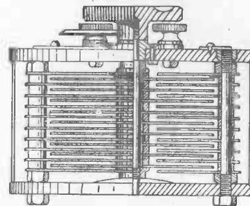
Fig. 163.—Half-section and Elevation of Variable Condenser
