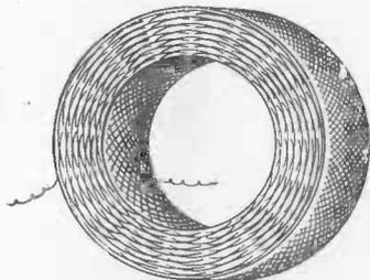
Fig. 109.—Finished Honeycomb Coil
