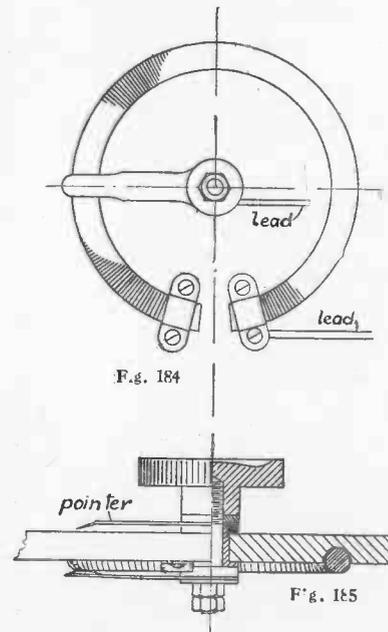
Figs. 184 and 185.—Underneath Plan and Part Section of Rotary Resistance
