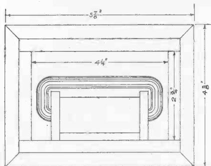
Fig. 200.—Diagram showing Position of Transformer in Case
