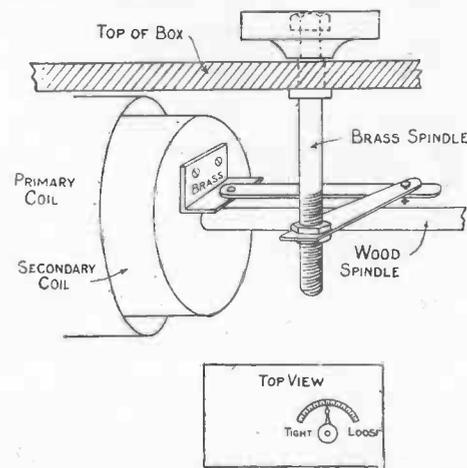
Fig. 100.—Device for Operating the Loose-coupler
