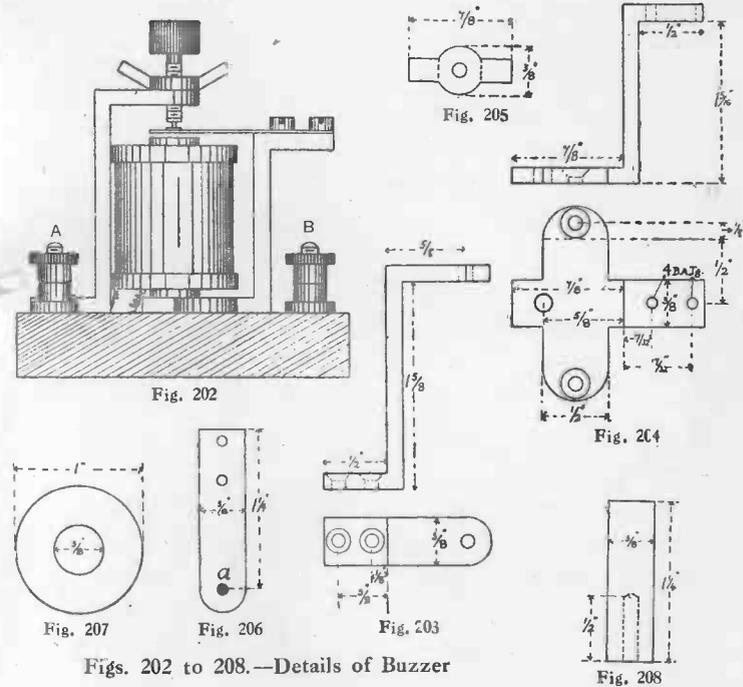
Figs. 202 to 208.—Details of Buzzer
