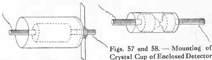
Figs. 57 and 58. — Mounting of Crystal Cup of Enclosed Detector
