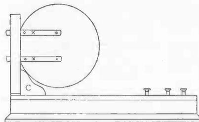
Fig. 136.—Side Elevation of Stand for Holding Coils
