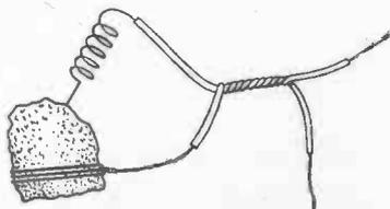
Fig. 69. Simple Improvised Detector
