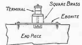
Fig. 71.—Method of Fixing Slider Rod to End Piece
