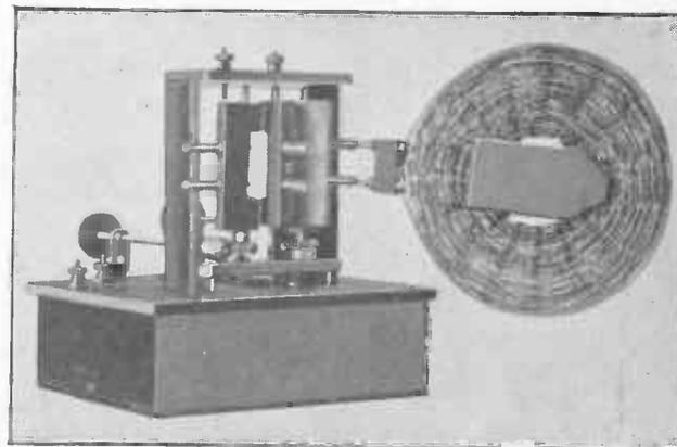
Fig. 115.—Photograph of Complete Basket-coil Tuner
