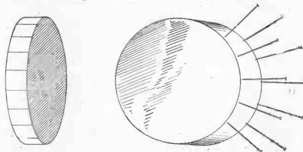
Fig. 105.—Wooden Disc for Winding Honeycomb Coils
