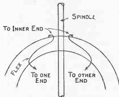
Fig 180.—Method of Making Connections
