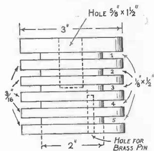
Fig. 120.—Hard-wood Former for Bank-wound Coil
