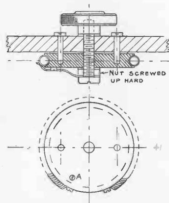
Fig. 195.—Section and Plan of Filament Rheostat
