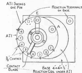
Fig. 123.—Plan of Complete Coil
