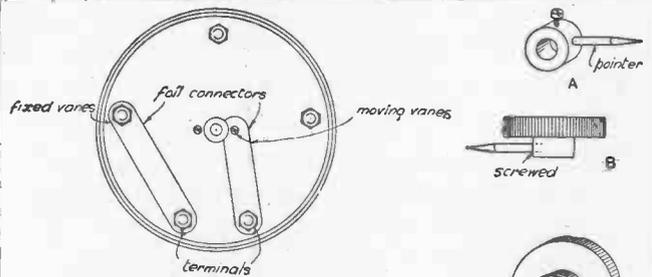
Fig. 167.—Bottom View of Top Plate showing Connections
