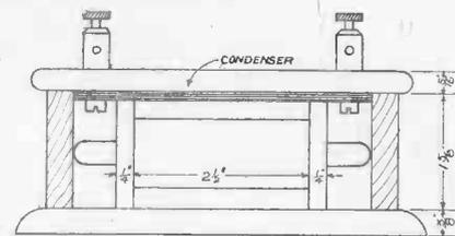
Fig. 199.—Sectional Elevation of Transformer
