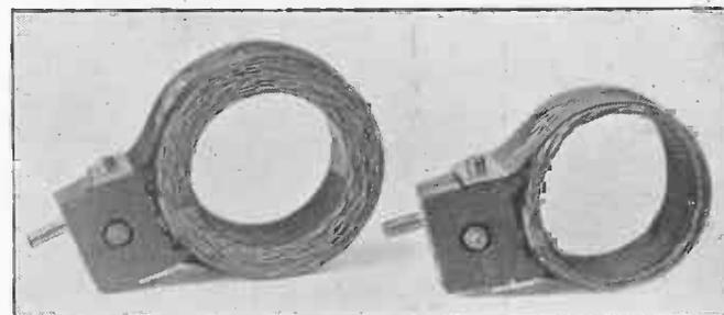
Fig. 110.—Mounted Honeycomb Coils
