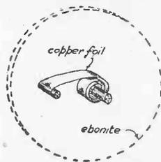
Fig. 168.—Positive Contact for Moving Vanes
