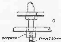
Fig. 169.—Methods of Taking End-thrust
