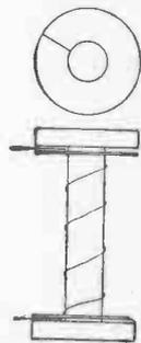
Fig. 197.—Method of Bringing Out Wire Between Paper Washers
