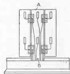
Fig. 137.—Back Elevation of Stand showing Wiring Connections
