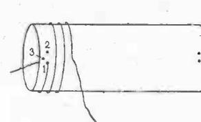
Fig. 70.—Method of Fixing Winding to Cardboard Tube
