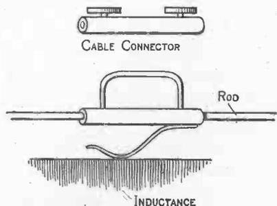
Fig. 83.—Inductance Slider made from Connector
