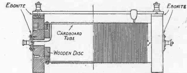
Fig. 72.—Half Section of Tuning Coil
