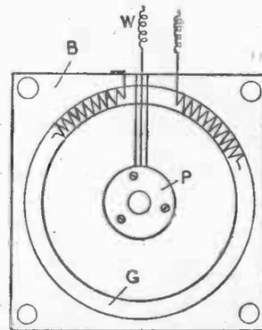
**Another Type of Rotary Filament Resistance.**—Figs. 192 to 194 give the constructional details of a rotary filament resistance.
