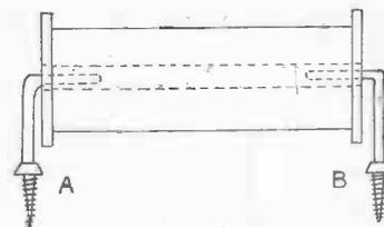
Fig. 84.—Spool for Supporting Wire during Winding
