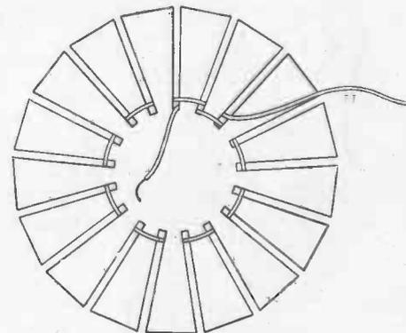
Fig. 112.—Method of Winding Basket Coil
