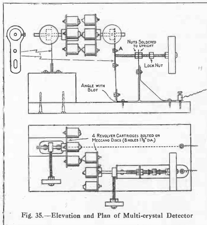
Fig. 35.—Elevation and Plan of Multi-crystal Detector
