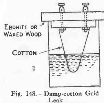
Fig. 148.—Damp-cotton Grid Leak
