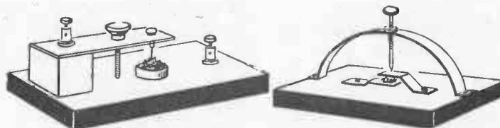
Fig. 28.—Simple One-crystal Detector Fig. 29.—Improved Detector
