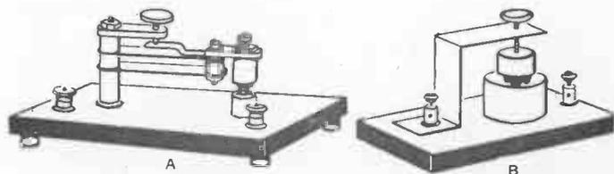
Fig. 25.—Two types of Detector, A, Spring-adjusted, B, Mercury-cup Detector
