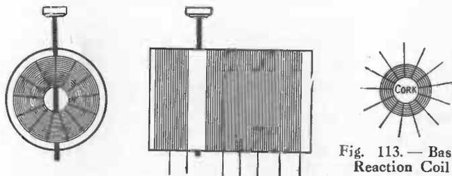
Fig. 114.—End and Side Views of Mounted Basket Reaction Coil Fitted in Inductance Coil
