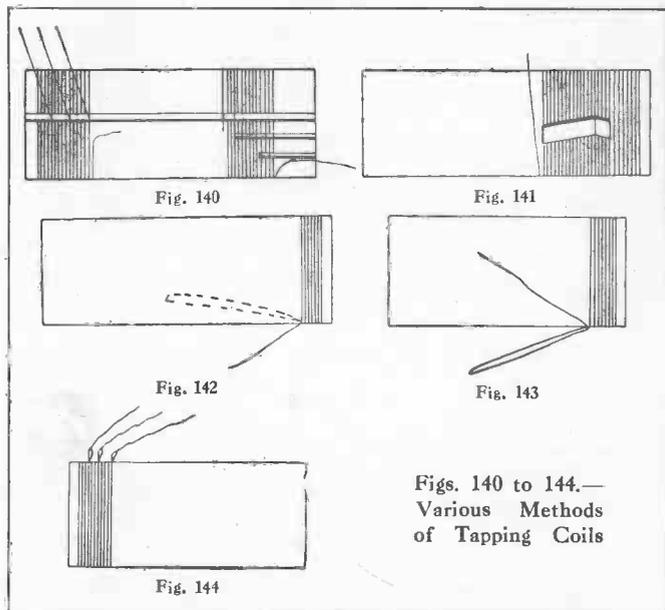
rod as indicated, and the wire at that point is subsequently bared and the tapping soldered to it. This method has the advantage that the soldering operation is not likely to affect the insulation of the adjacent coils. All the tappings, however, will be in a straight line, whereas it is desirable to make them lie along a spiral line. For very fine tapping, therefore, additional
