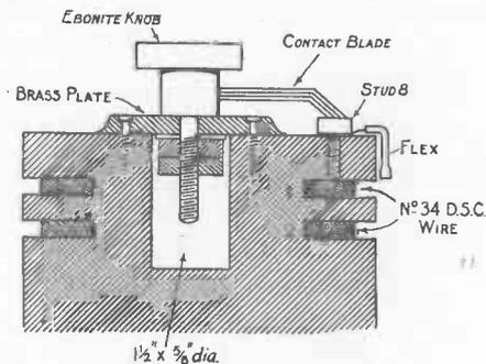
Fig. 122.—Part Section showing Method of Fixing Switch
