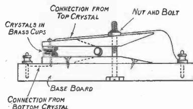
Fig. 36.—Detector made from Wooden Clip
