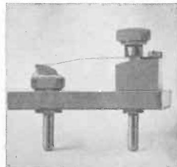
Fig. 50.—Vertical Detector
