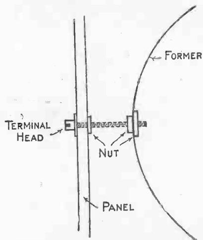
Fig. 176.—Method of Mounting Variometer.
