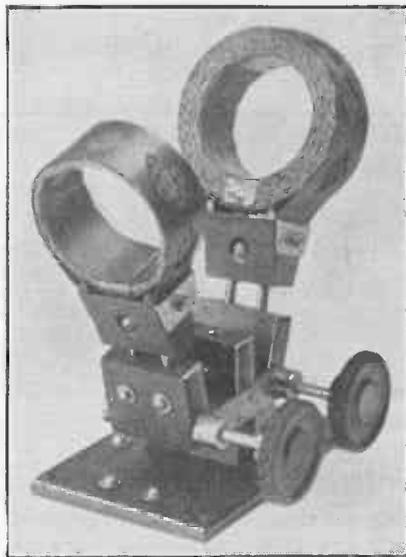
Fig. 111.—Honeycomb Coils in Use as Tuner
