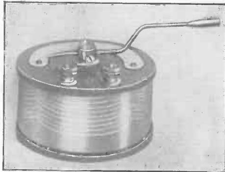
Fig. 161.—Standard Variable Condenser
