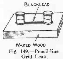
Fig. 149.—Pencil-line Grid Leak
