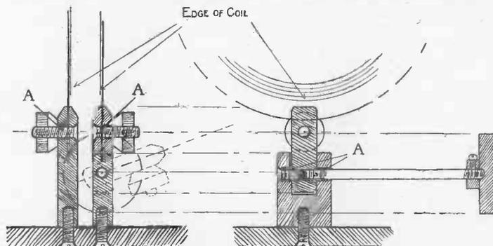
Fig. 129.—Sectional Views of Slab-inductance Stand
