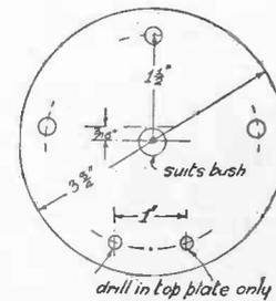
Fig. 165.—Ebonite Ends Marked Out
