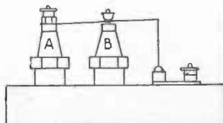
Fig. 37.—Crystal Detector made from Sparking Plugs
