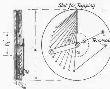
Fig. 119.—Former for Winding Slab Coils
