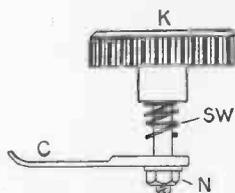
Fig. 194.—Details of Selector Switch
