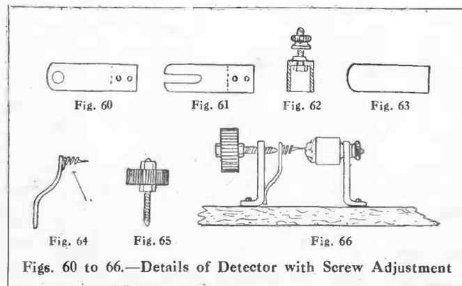
Figs. 60 to 66.—Details of Detector with Screw Adjustment
