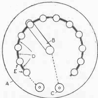
Fig. 152.—Variable Grid Leak
