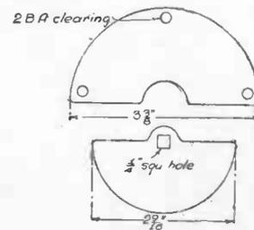
Fig. 164.—Plates of Variable Condenser
