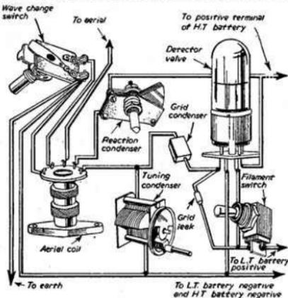
Fig. 63.—A typical detector stage in pictorial form.
