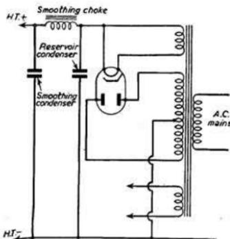
Fig. 97.—Practical and theoretical diagrams of a standard A.C. power pack
