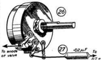
Fig. 26.—The variable resistor and condenser necessary for adding tone control.
