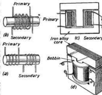
Fig. 72.—The essential parts of a simple transformer are shown at a and b; c and d illustrate the actual form of a transformer used in a wireless set.
