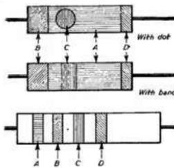
Fig. 29a.—The colour code diagram.
