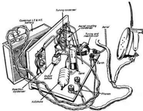
Fig. 10.—Fictorial wiring diagram of circuit shown by Fig. 1. Some of the wiring is underneath the baseboard, which is fixed to the panel about an inch from the bottom edge to clear the valve holder sockets.
