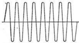
Fig. 51.—The waveform of an unmodulated carrier wave.
