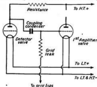
Fig. 67.—Theoretical circuit of an R.C. coupling.
