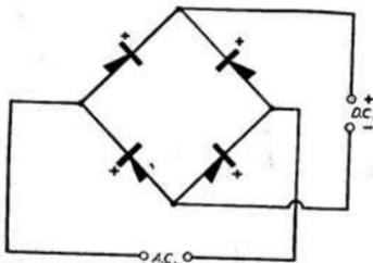
Fig. 100.—A bridge rectifier circuit.
