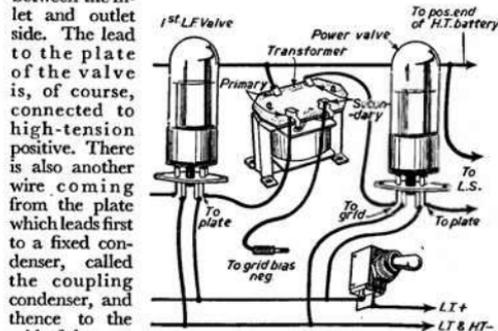
Fig. 71.—Pictorial representation of the arrangement shown in Fig. 70.
