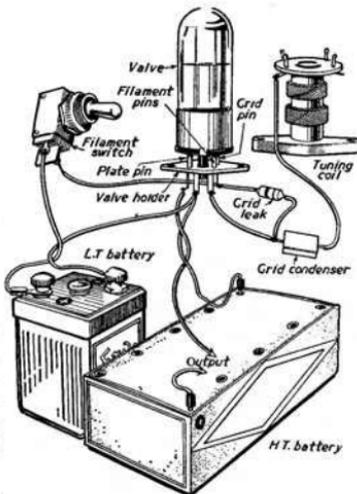
Fig. 65.—Battery connections.
