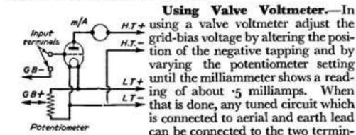
Fig. 84.—The circuit arrangement of a valve voltmeter which is suitable for comparing the efficiency of various coils.
