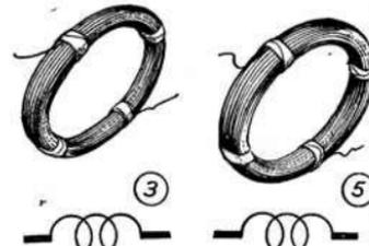
Fig. 3.—The aerial (40 turns) and reaction (60 turns) coils.
