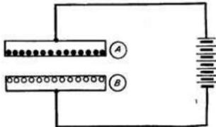
Fig. 39.—Dielectric strain in charged condenser.
