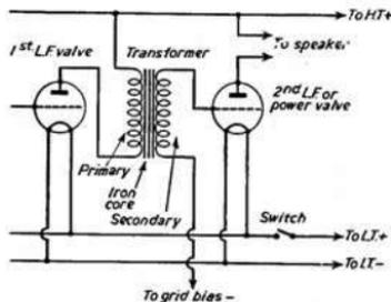
Fig. 70.—Theoretical circuit of transformer-coupled stage.
