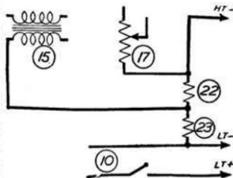
Fig. 23.—Modified circuit for providing automatic grid bias.
