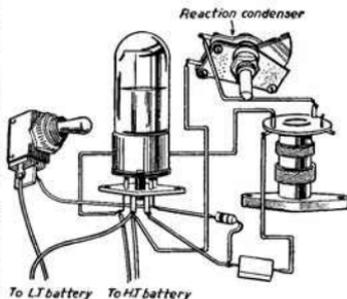
Fig. 66.—The reaction circuit.
