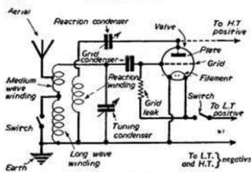
Fig. 64.—Circuit of a detector stage.
