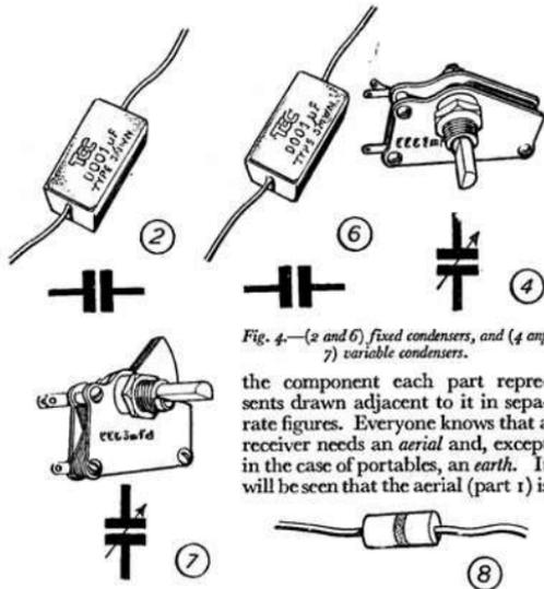
Fig. 4.—(2 and 6) fixed condensers, and (4 and 7) variable condensers.
