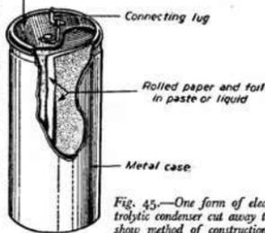
Fig. 45.—One form of electrolytic condenser cut away to show method of construction.
