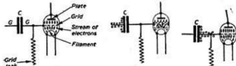
Figs. 60, 61 and 62.—(Left) The normal electron flow inside the valve. (Centre) The signal electrons on the grid and grid condenser. (Right) The accumulation on the grid side of the condenser.
