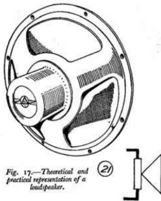
Fig. 17.—Theoretical and practical representation of a loudspeaker.
