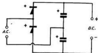
Fig. 99.—A metal rectifier voltage doubler circuit.
