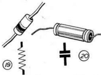
Fig. 16.—Two of the new components which form part of the R.C.C. coupling.
