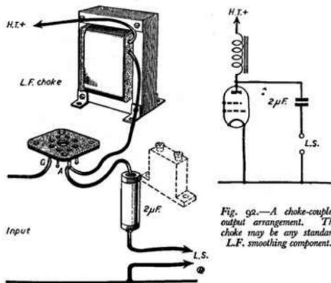
Fig. 92.—A choke-coupled output arrangement. The choke may be any standard L.F. smoothing component.
