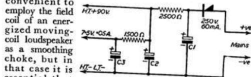
Fig. 101.—A half-wave rectifier with resistance smoothing.
