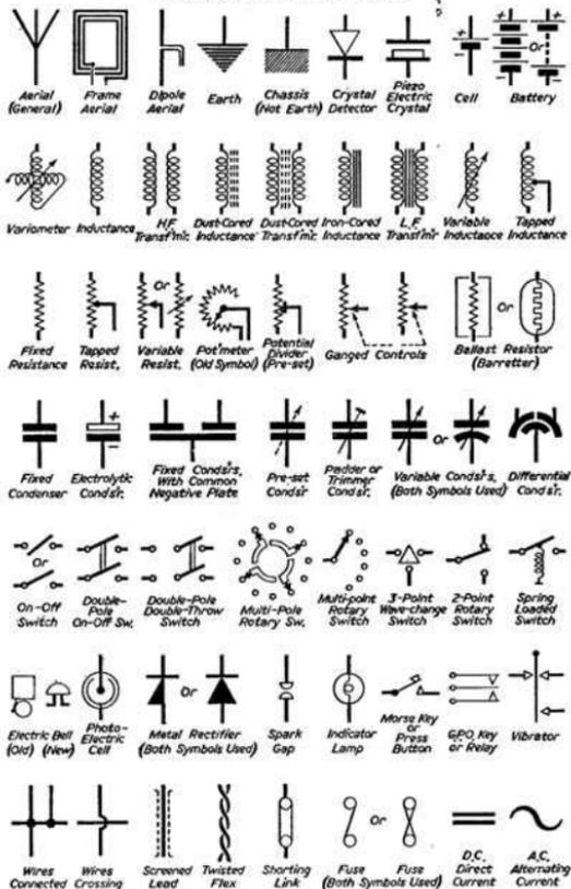
Conventional signs used in drawing a wireless circuit, which merely consists of a number of these signs joined together. Pictorial diagrams showing the actual components represented are given in the book in their correct alphabetical order.
