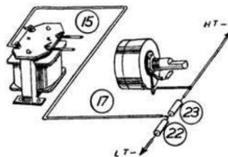
Fig. 24.—Pictorial diagram of the auto-bias wiring.
