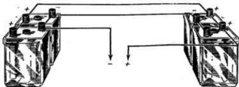
Fig. 103.—Accumulators in parallel.
