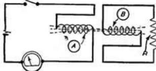
Fig. 41.—Circuit illustrating mutual induction.
