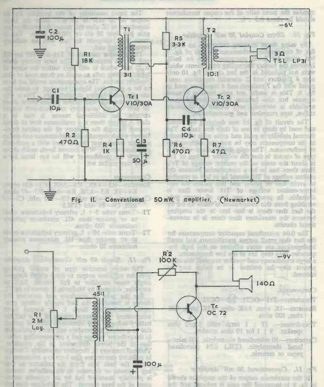
Fig. 12. Simple 60 mW. gramophone amplifier by Mullard.
