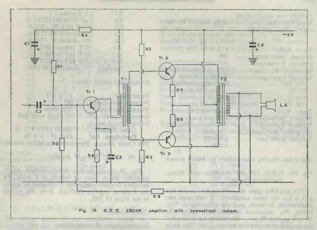
The only cure for this is to include resistors R5 and R6 in the emitters of the first two transistors. These can not be bypassed by electrolytic capacitors in the normal way because the reetifying action of the base-emitter junction would charge them up to the point where they would alter the bias conditions themselves. R5 and R6, therefore, cause a loss of gain.
