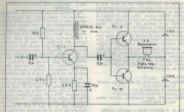
Fig. 7. Complementary symmetry Push-Pull amplifier.
