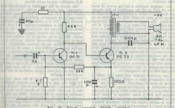
Direct Fig. 10. coupled 30 mW. amplifier.
