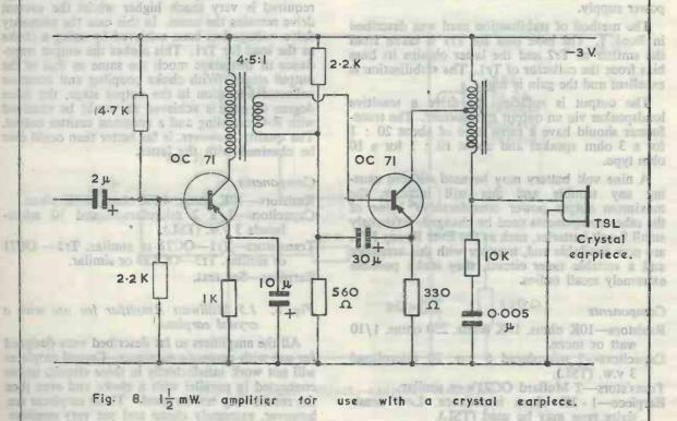
The reason for their failure to work in a conventional circuit is two fold. Firstly, the impedance of this type is normally around 150K ohms and secondly, they do not conduct electricity.
