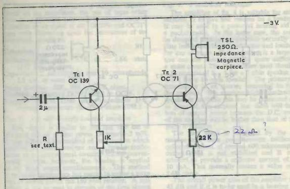
Fig. 5. Direct coupled amplifier with low battery drain.
