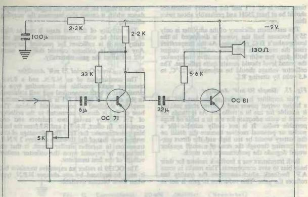
Fig. 13, Simple 90 mW. amplifier.
