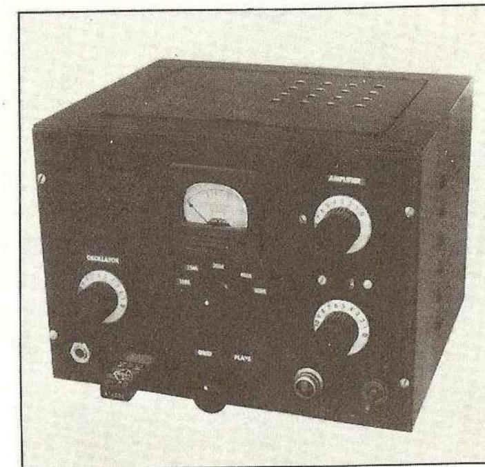
**Fig. 16** This all-band transmitter measures 7" x 8" x 10" in size, including power supply. Oscillator control is at left, with bandswitch and meter switch at center. Amplifier controls are at the right, with line switch and pilot.
