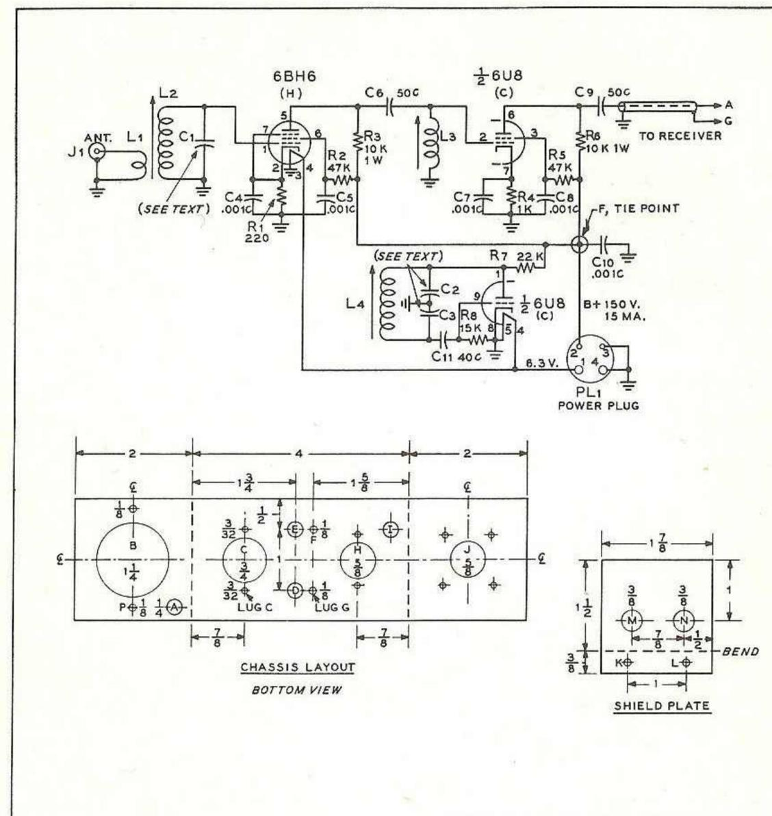
**Fig. 5** Schematic of two tube amateur band converter for 20, 15, 10 or 6 meters.
