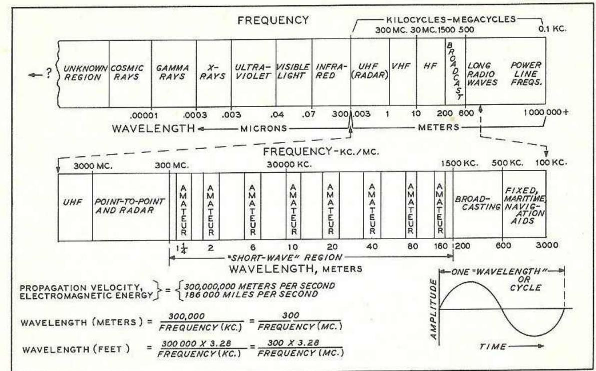
Fig. 1 The radio frequencies are but a small portion of the electromagnetic spectrum. As wavelength shortens, radio waves merge with infra-red waves.
