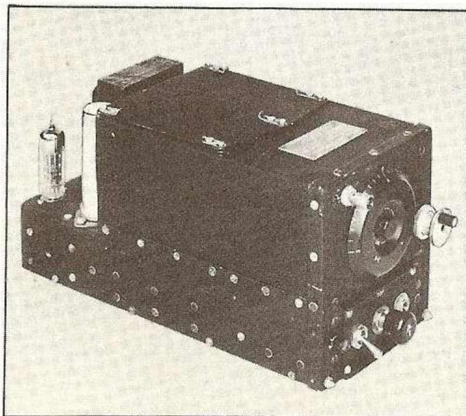
Fig. 8 When converted to a-c operation, the "Command" set makes an excellent receiver for the beginning amateur. Power supply is placed in dynamotor well of receiver, and control panel is added.
