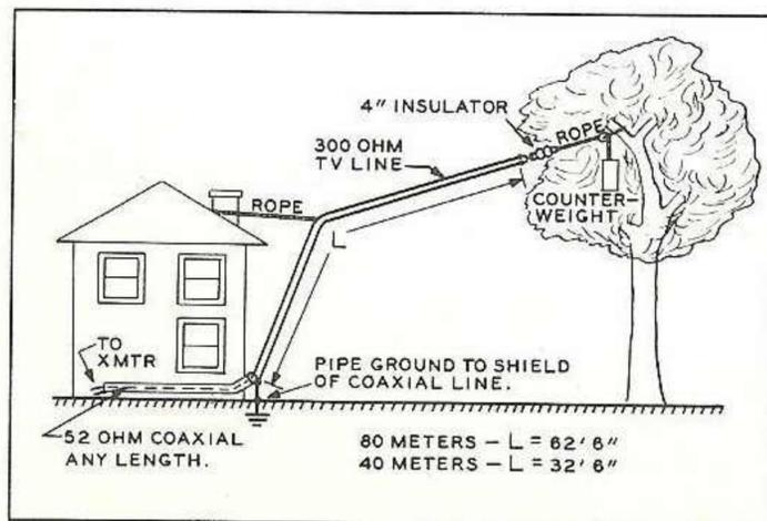
Fig. 5 Folded Marconi sky-wire is excellent antenna where amateur must contend with restricted space for his aerial. Water pipe ground may be used with antenna.
