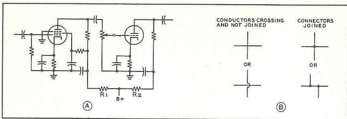
Fig. 3 The schematic diagram shows interconnections between various parts of electronic circuit, but does not show the actual placement of the parts. Different drawing techniques (B) create confusion for beginner, as it is hard to determine if crossed wires are junction (right) or merely cross-over (left).
