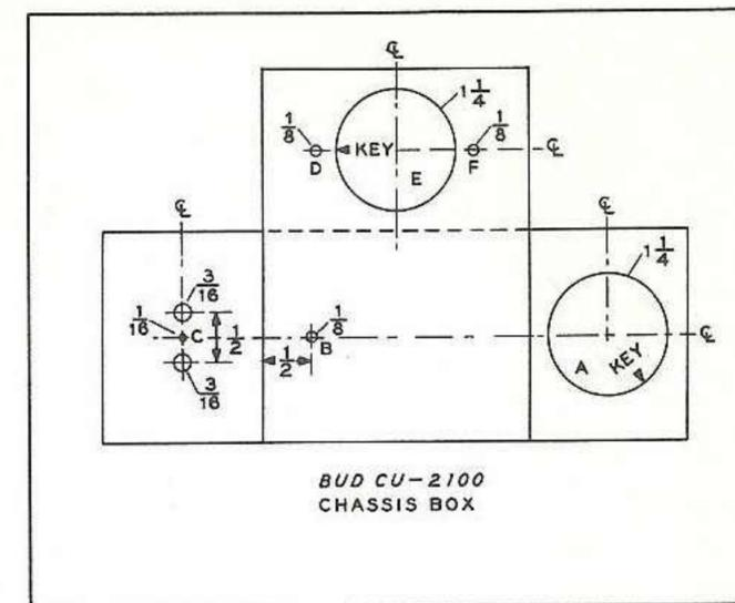
Fig. 15 Chassis layout for the adapter. One side of aluminum box is cut off and attached to the other half with sheet metal screws. Crystal receptacle is mounted on "top" of box, with octal power plug on "bottom."
