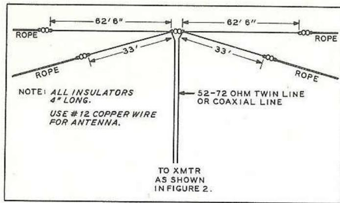
Fig. 3 Three bands may be worked with this multi-wire doublet antenna. As with any antenna of this type, care must be taken to make sure that harmonics of the transmitter are not radiated by the antenna.
