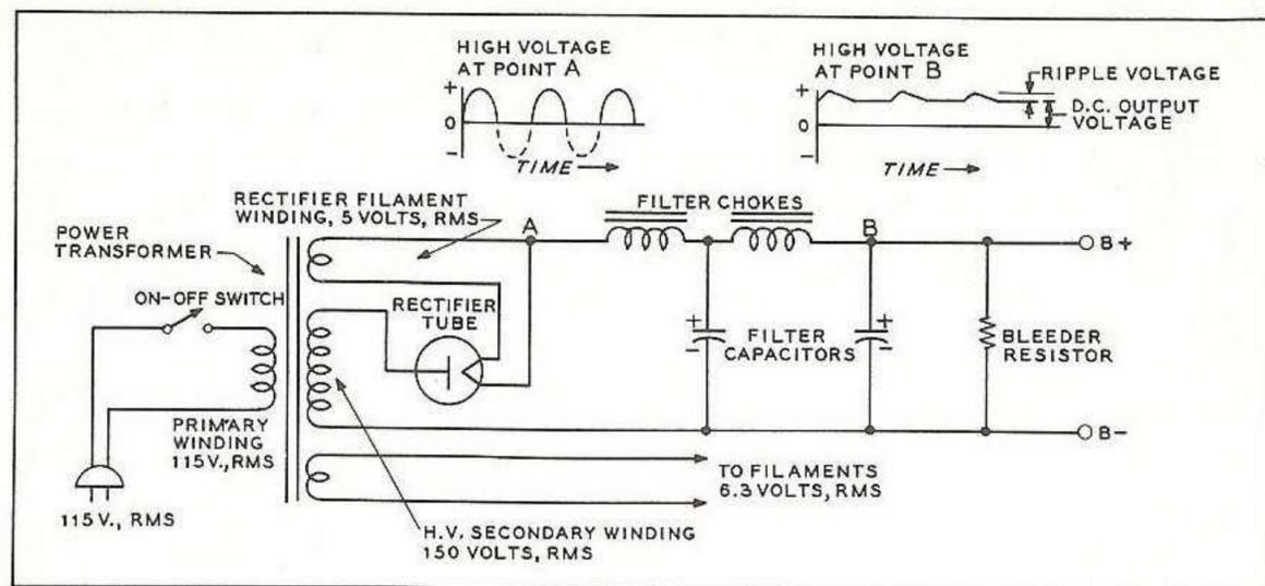
Fig. 2 Schematic diagram of a typical half-wave high voltage power supply.
