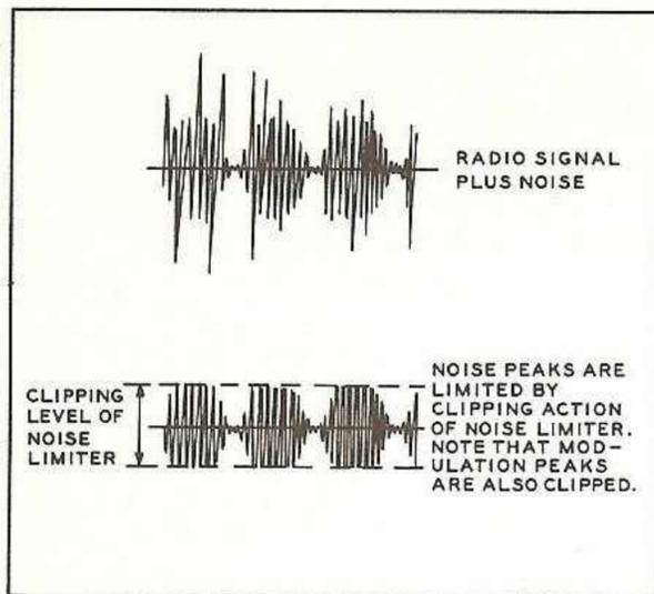
Fig. 5 Loud noise impulses tend to paralyze receiver between the pulses. A noise clipper can chop off the peaks of the noise and permit good copy of signal that is otherwise obliterated by high noise level.
