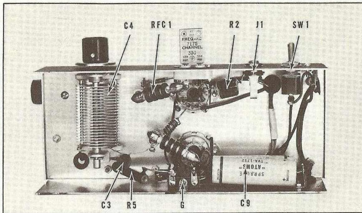
Fig. 8 Under-chassis view of SP-50 transmitter. Ceramic insulator holds one end of C3, RFC-2, and PC. Lead from C4 to coil L1 passes through grommet at lower left of tuning capacitor. Bypass capacitors C7 and C8 are mounted to insulated tie-point to the right of line switch SW1, at upper right.
