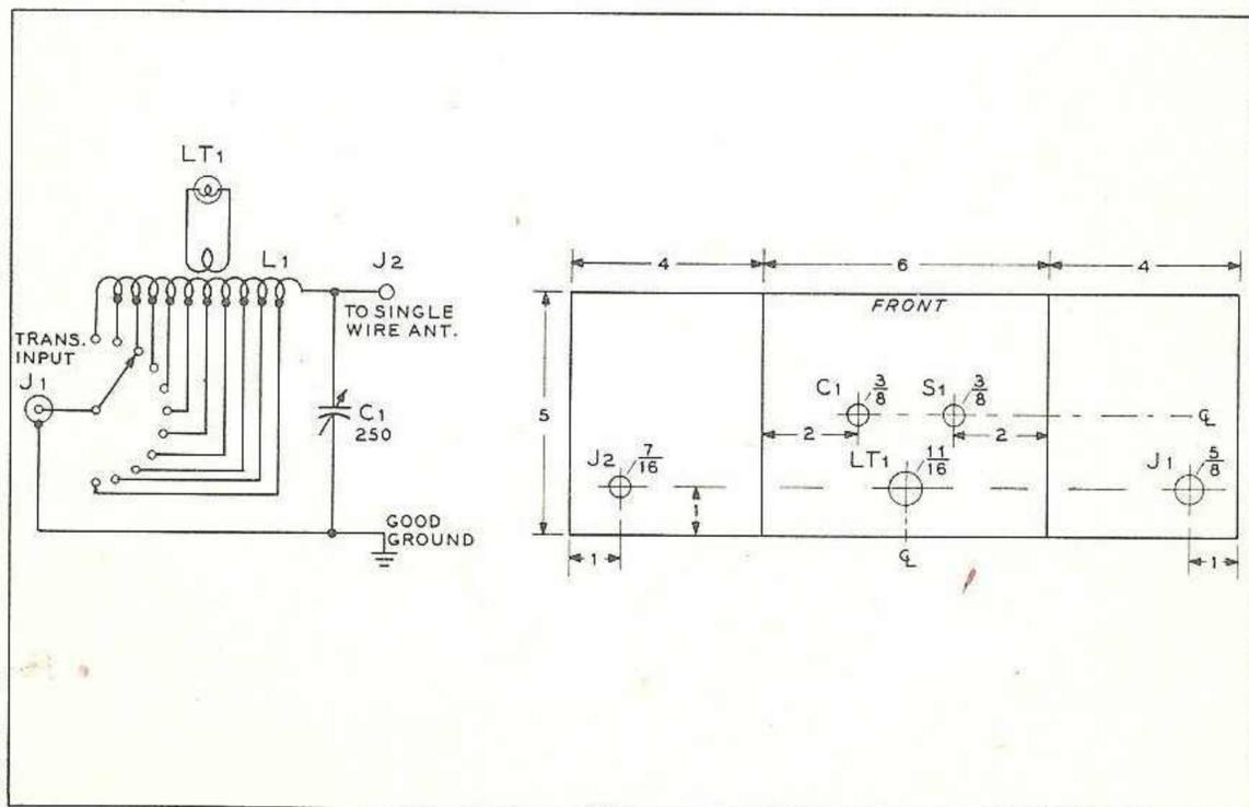
Fig. 7 Schematic of 75 watt antenna tuner suitable for 10-80 meter operation.
