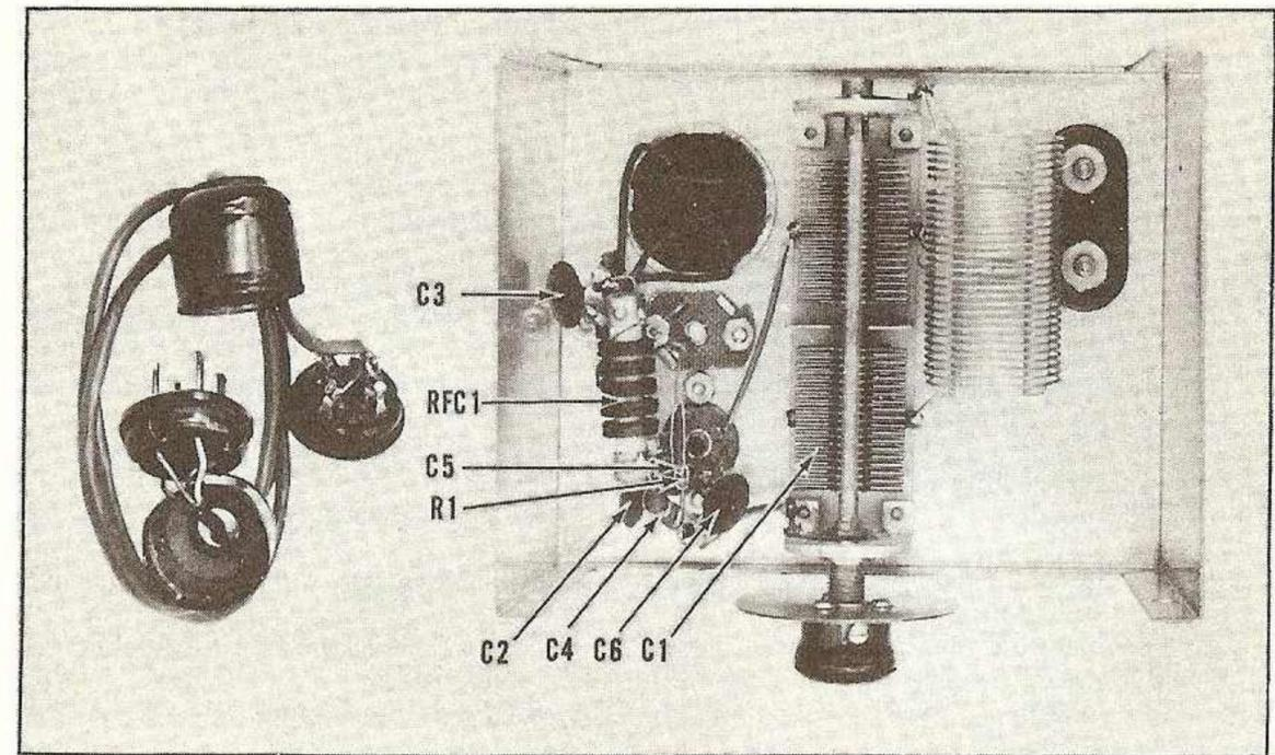
Fig. 3 The placement of the under-chassis components are shown here. Coil L1 is at the right of peaking capacitor C1, with the antenna terminals at the right of the chassis. Power cable is at left, showing wiring of plugs.
