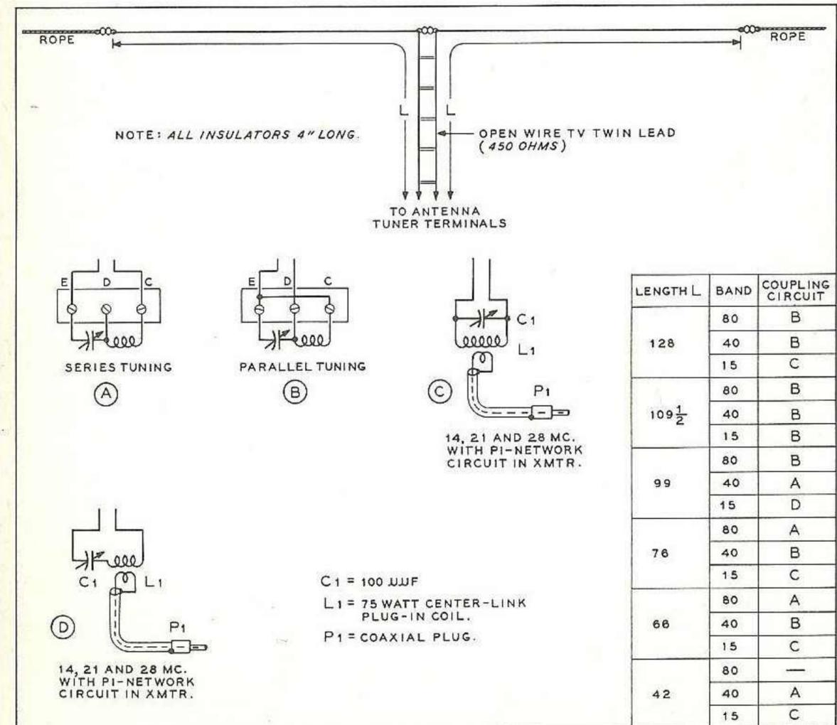
Fig. 6 Center-fed "Zepp" antenna is well suited for general amateur use.
