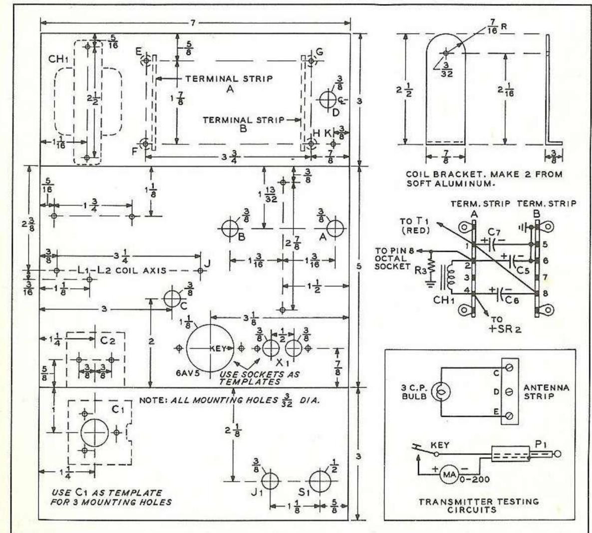
Fig. 3 Parts layout and chassis template for LJ-15 transmitter. Coil brackets for L1-L2 are shown at upper right. The test circuits are shown at the lower right.
