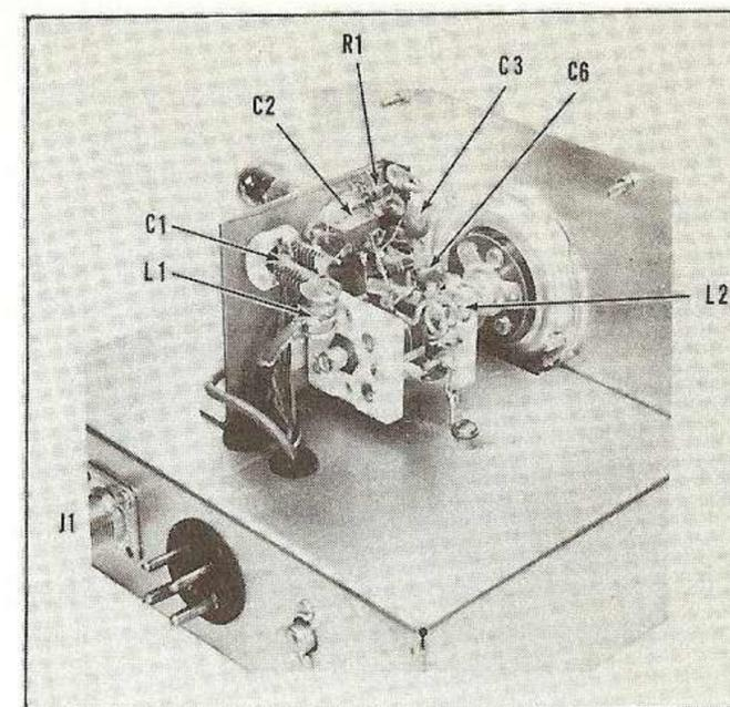
Fig. 14 Placement of the major components are seen in this rear view. Most parts are mounted upon the sub-assembly plate (B) shown in Figure 13. Power plug and output receptacle (J2) are to the right of antenna receptacle J1. Front of chassis has small cut-out to clear dial mechanism.
