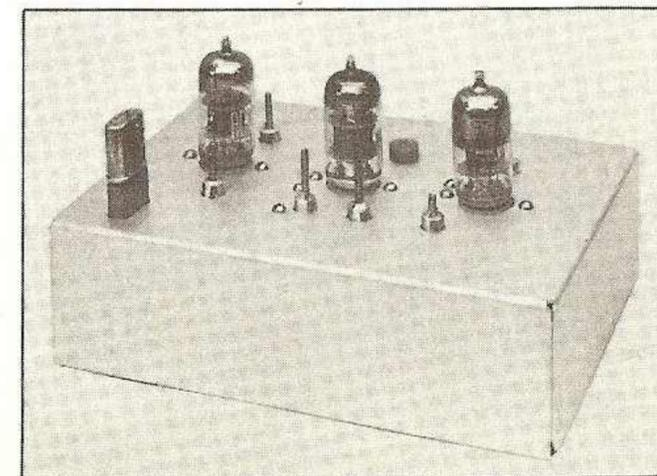
Fig. 15 Simple crystal converter will provide maximum performance on 2 and 6 meter bands. Crystal oscillator stage is at left, with 6BQ7A r-f amplifier at right.
