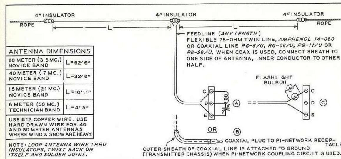
Fig. 2 The center-fed dipole (doublet) antenna is popular on all ham bands.
