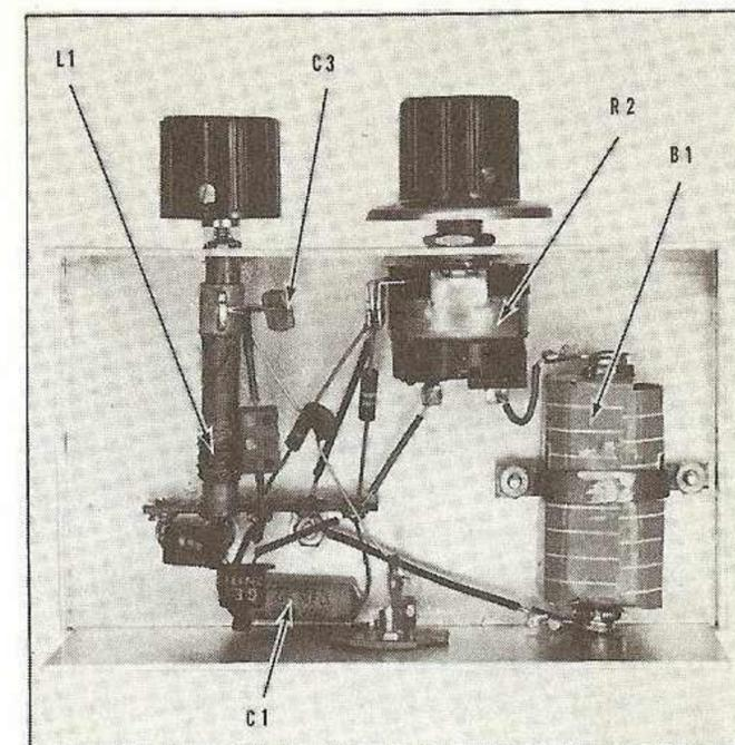
Fig. 25 Under-chassis view of T-QM. "Loopstick" coil (L1) is at left, with 2N170 transistor directly below it. 9-volt battery is mounted in clamp at right. Output receptacle (J1) is on the rear lip of chassis behind L1.
