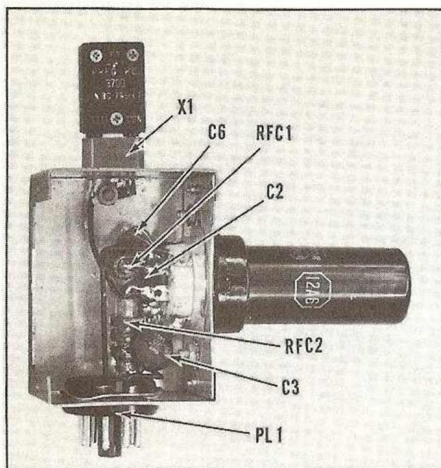
Fig. 13 Interior view of the crystal control adapter for a "Command" transmitter. The 12A6 oscillator tube mounts in a horizontal position over the unused sockets of the transmitter. Adapter plugs in 1626 oscillator socket of transmitter.
