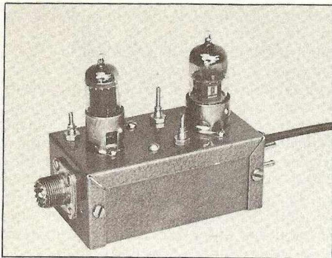
**Fig. 4** This two tube converter may be used up to the six meter amateur band with any good short wave receiver. The 6BH6 r-f amplifier is at the left, and the 6U8 mixer/oscillator tube is at the right. The tuning slugs of the three inductances project through the top of the chassis box for adjustment.
