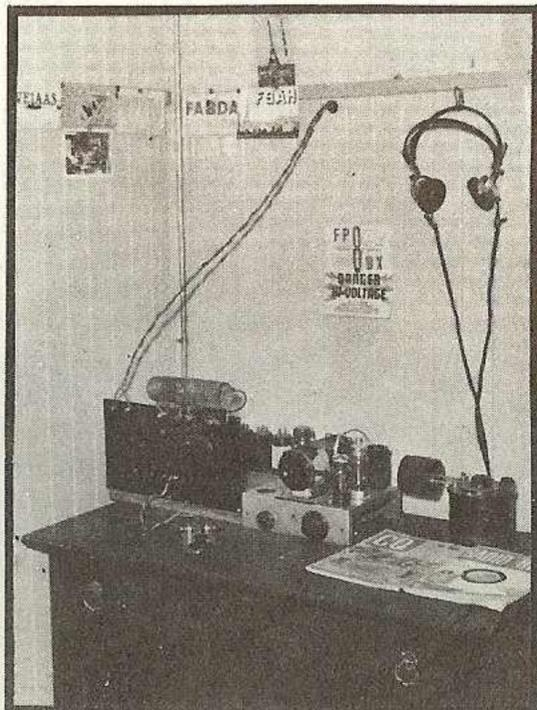
Many overseas amateurs do not enjoy radio parts, kits and equipment that is easily obtainable in W-land. Completely home built equipment is the rule, as shown in this photo of ex-FP8BX. Note the home-made coils on the transmitter at the left. Running but ten watts, FP8BX worked many DX stations in all parts of the world. What can you do with 75 watts? Try your hand at DX!
