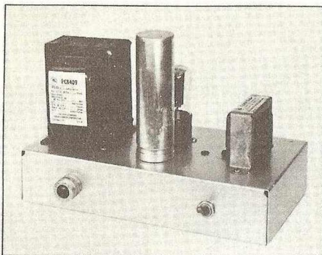
Fig. 7 350 volt power supply may be used for receivers or low power transmitters. The power transformer is at the left, with filter capacitor and rectifier tube in center. Filter choke is at right.
