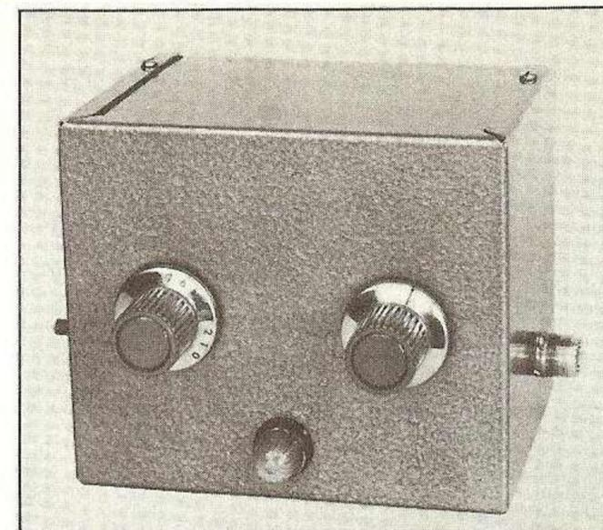
Fig. 8 Single-wire antenna tuner suitable for Novice work. The pilot lamp is inductively coupled to loading coil of unit, and indicates resonance of tuner. Inductance and capacitance should be added by adjusting tuner until maximum bulb brilliance occurs.
