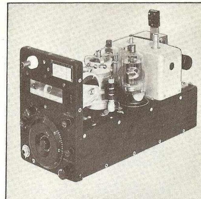
Fig. 9 Surplus "Command" transmitter makes ideal rig for the Novice. With the use of a simple adapter, the transmitter may be converted to crystal control operation. Removal of the adapter restores v-f-o operation. The complete conversion of the "Command" transmitter for a-c operation is given in the accompanying text.
