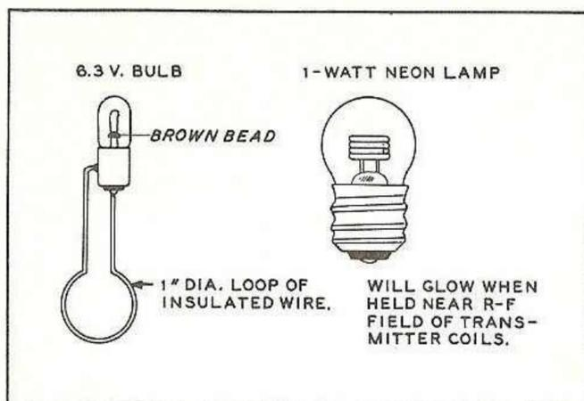
Fig. 5 Neon lamp, or flashlight bulb may be used as a simple r-f indicator. These basic instruments are helpful during preliminary tuning and adjustments.
