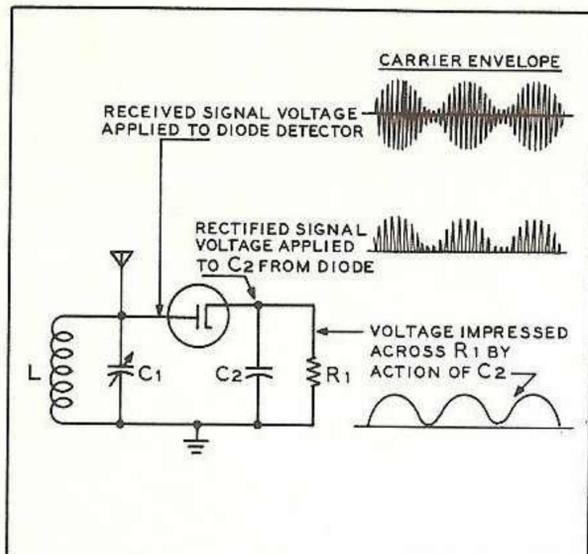
Fig. 2 The diode detector is a simple means of recovering the intelligence conveyed in the envelope of the carrier. The variations are rectified by the diode and charge capacitor C2. Indicating device across this capacitor will show variations in carrier envelope. This circuit is also called an "envelope detector."
