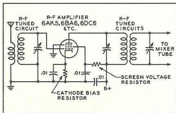
**Fig. 4** Simple radio frequency amplifier placed ahead of mixer tube reduces tendency of superhetrodyne circuit to receive two frequencies at once. R-f amplifier reduces response to unwanted signal by large amount.
