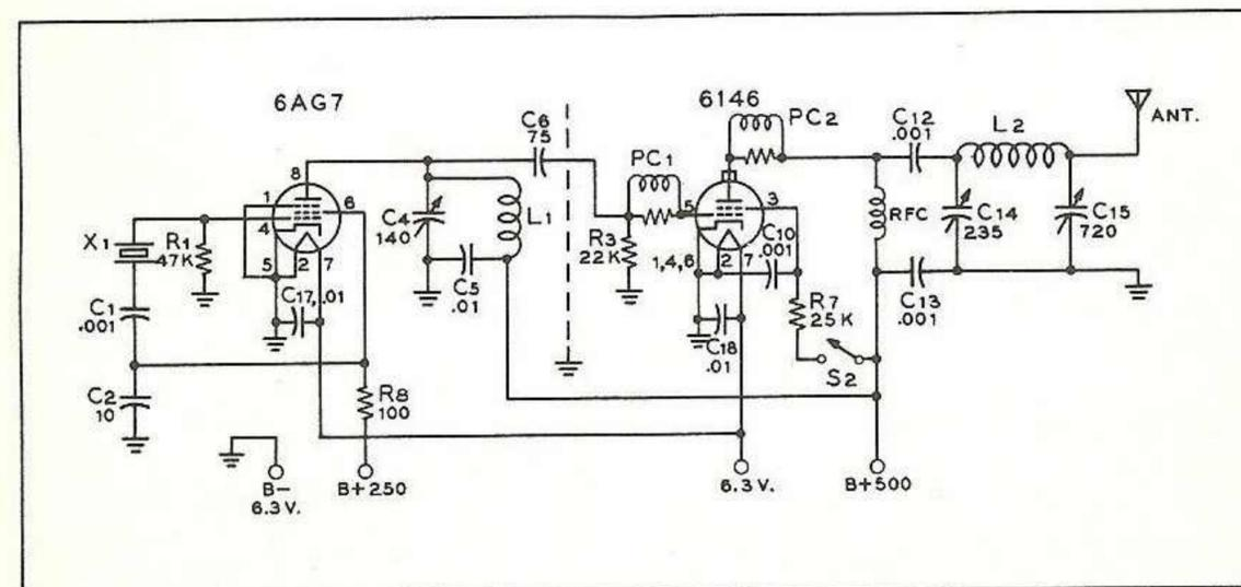
Fig. 2 A simplified diagram of the AB-60 transmitter shown in chapter 7. A 6AG7 harmonic crystal oscillator drives a 6146 amplifier-doubler stage. Good output may be obtained as high as eight times the crystal frequency. Operation of the complete circuit is covered in this chapter, as well as metering ideas.
