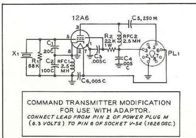
Fig. 14 Schematic of crystal control adapter. Regenerative circuit (C1, C2, RFC-1) lowers crystal current and provides better keying characteristic for crystal oscillator.
