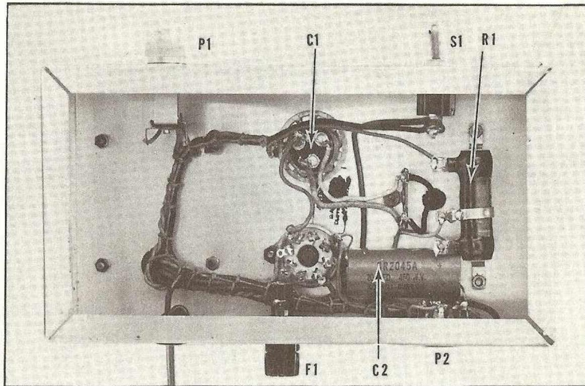
Fig. 9 Under-chassis view of medium voltage supply, showing major components.
