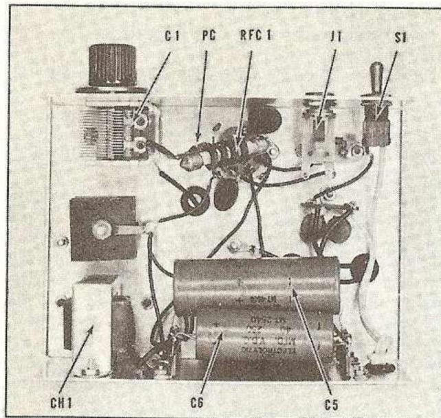
Fig. 4 Under chassis view of LJ-15 transmitter. Selenium rectifier is mounted to the chassis by long bolt. The line filter capacitors (C8, C9) are mounted to phenolic strip behind key jack, J1.
