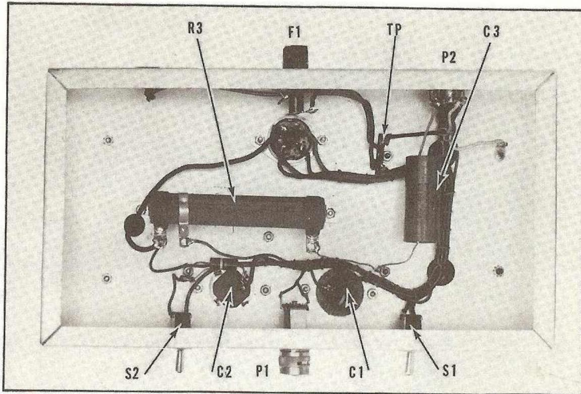
Fig. 12 Under-chassis view of 500 volt supply, showing placement of major components. For higher operating voltages, 5000 volt insulated "test lead" wire should be used for all high potential circuits. Filter capacitor should always be shorted out with piece of wire before any work is done on supply.
