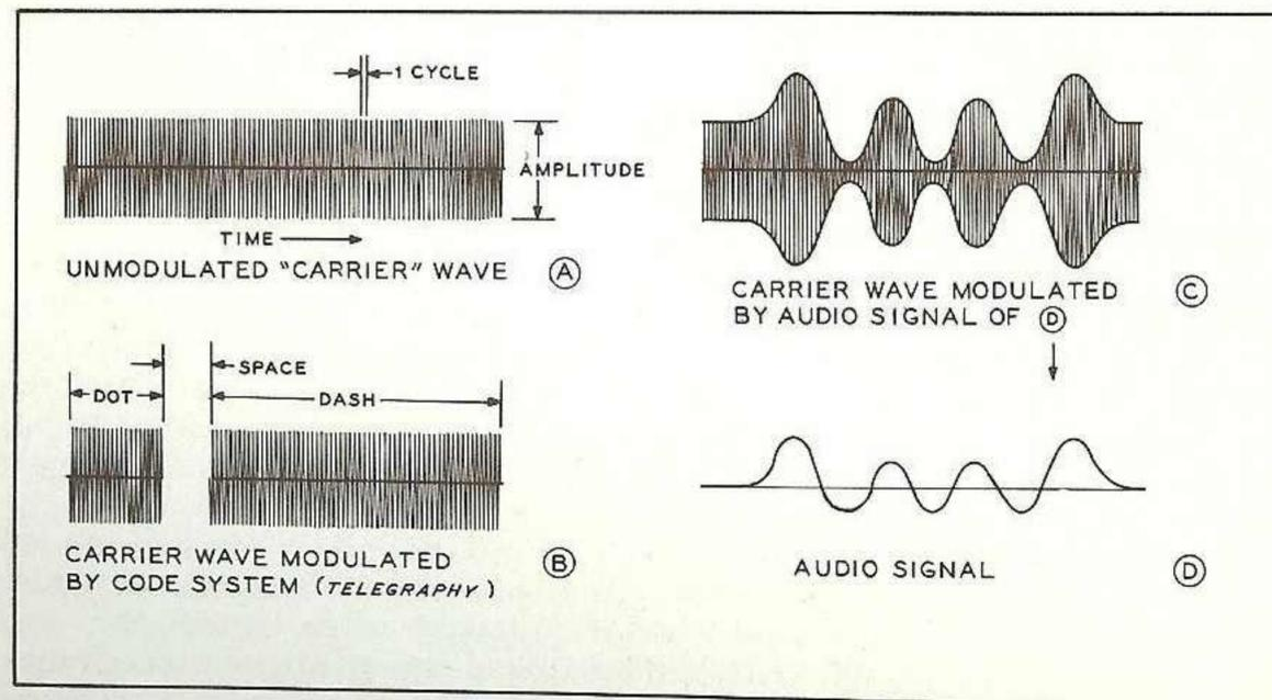
Fig. 2 Intelligence is transmitted on carrier wave by varying the amplitude. Code transmission breaks wave into "dot" and "dash" segments, while audio signal impresses its electrical equivalent upon envelope of carrier. Other forms of modulation such as frequency or pulse modulation may also be used.
