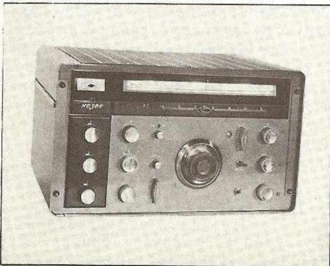
Fig. 6 Incorporating many of the special features required for serious amateur reception is the double conversion, 12 tube National NC-300 receiver. Converters are used to extend the tuning range of the set above 420 mc.
