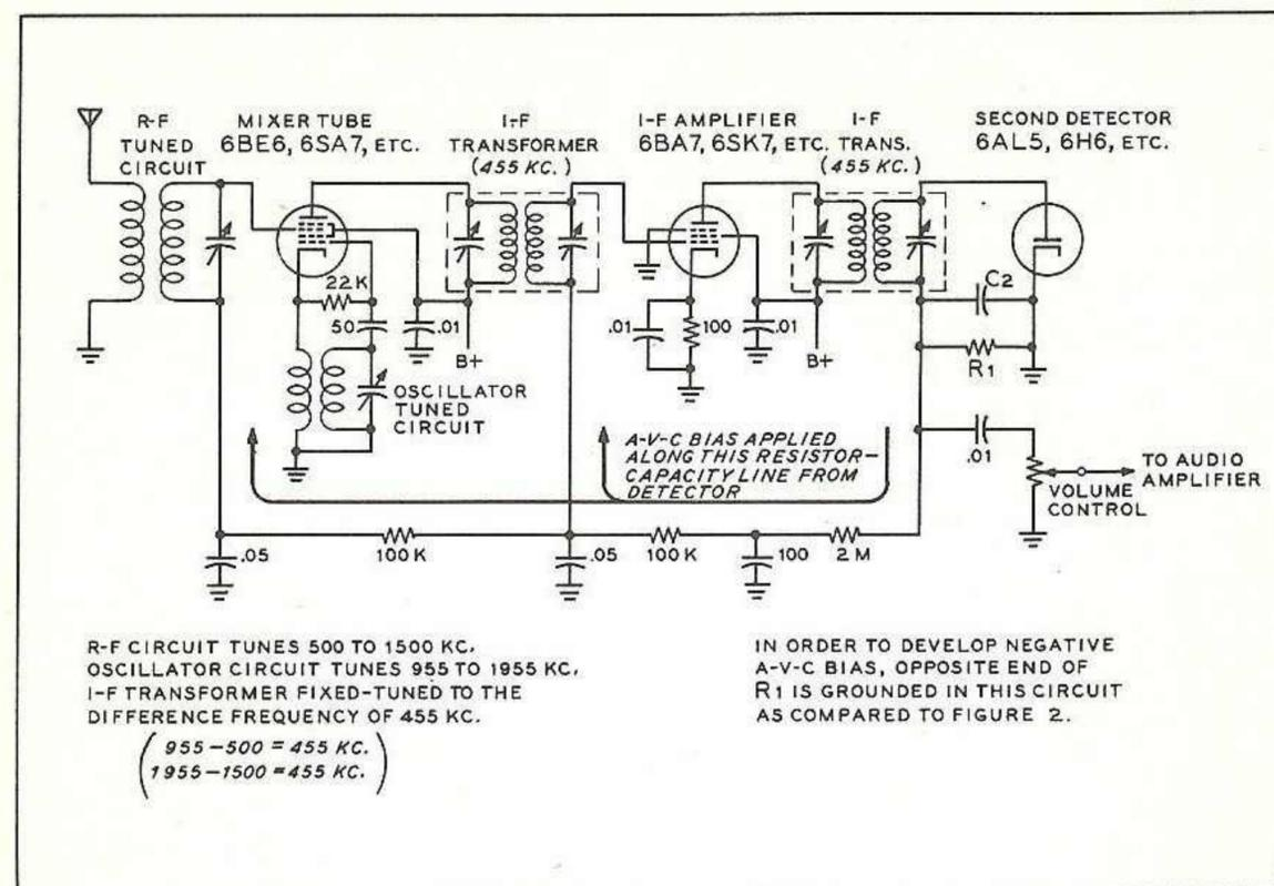
Fig. 3 The superheterodyne receiver translates all signals to a common low frequency and amplifies them at that frequency. Since tuned circuits may be made more selective at a lower frequency, high gain and good selectivity may be obtained that would be difficult and expensive to get at the signal frequency.
