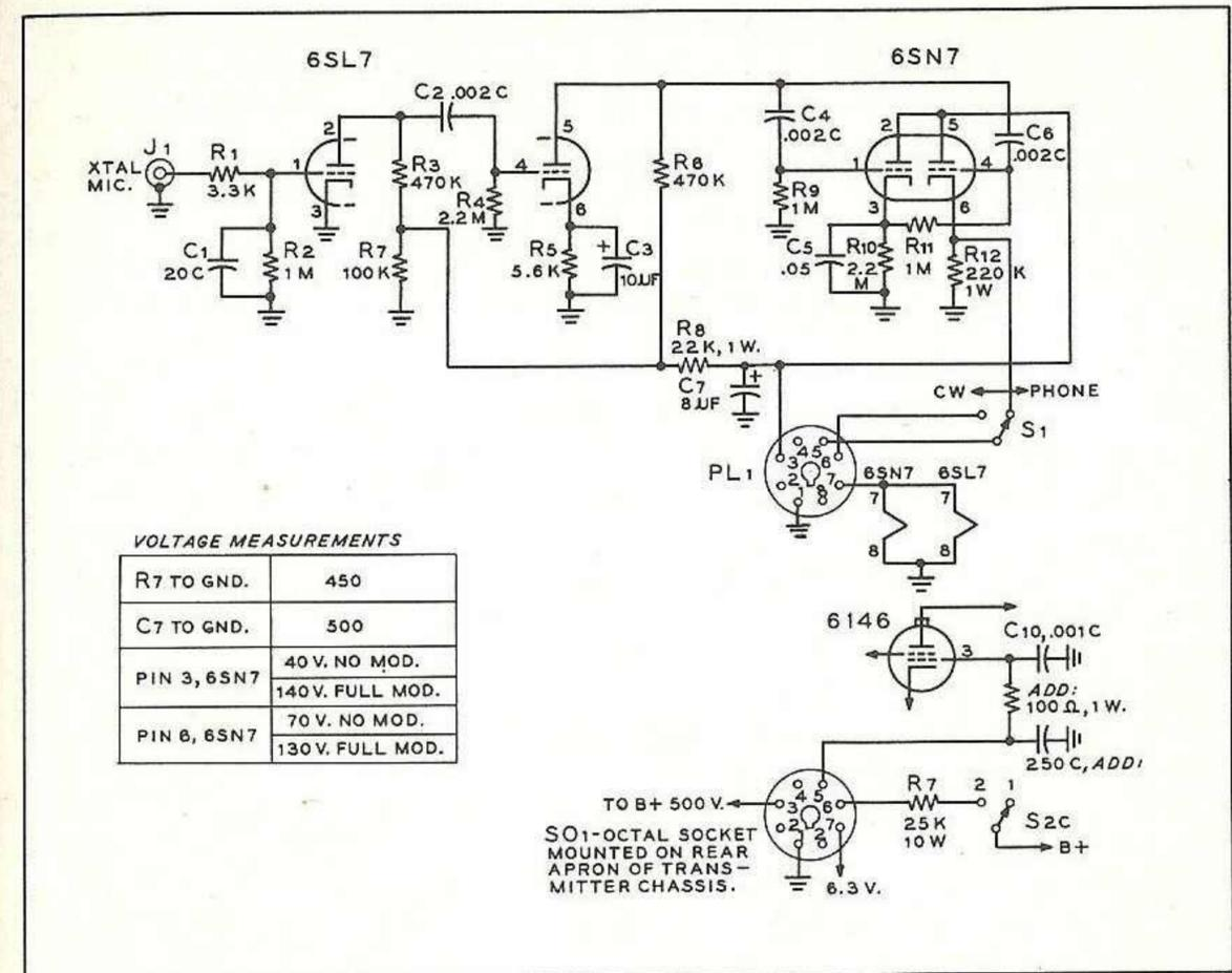
**Fig. 24** Schematic of screen modulator for AB-60 transmitter.
