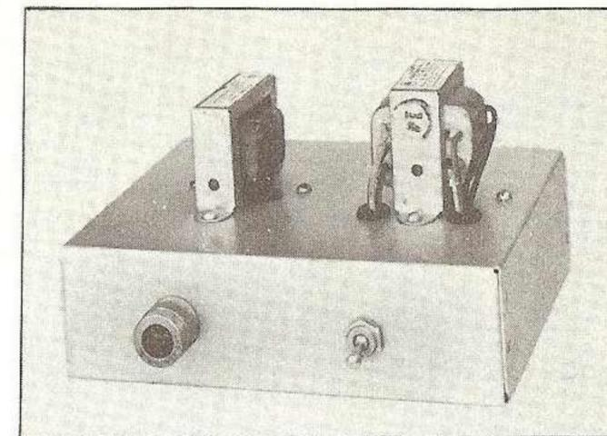
Fig. 4 This small power unit will provide 150 volts at a current drain of 25 milliamperes. Power transformer is at right, with filter choke to the left.
