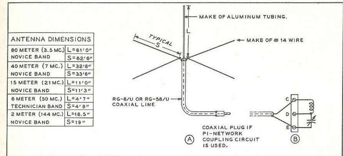
Fig. 4 The vertically polarized ground plane may be used on any band between 3.5 mc and 144 mc. For low frequency work, vertical whip may be made of wire.
