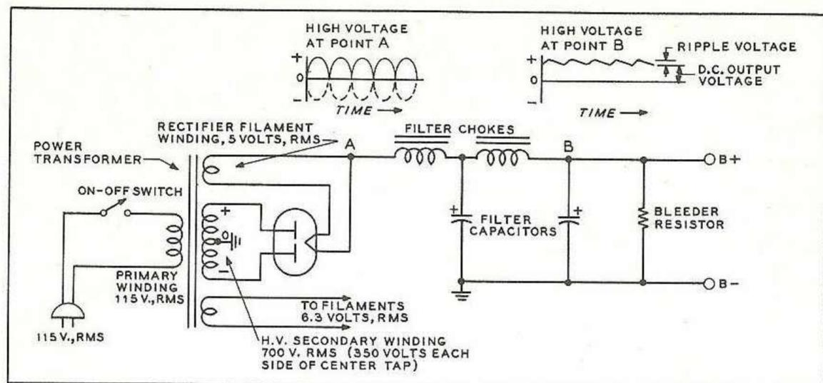
Fig. 3 Schematic diagram of a typical full-wave high voltage power supply.
