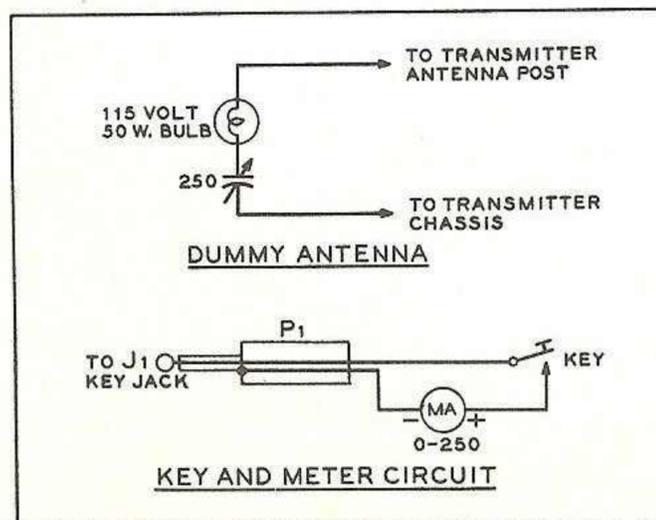
Fig. 12 A simple dummy antenna may be made from a 50-watt lamp bulb and a 250 mmf variable capacitor. This may be used with any of the "Command" transmitters. Keying circuit for the transmitters is also shown.
