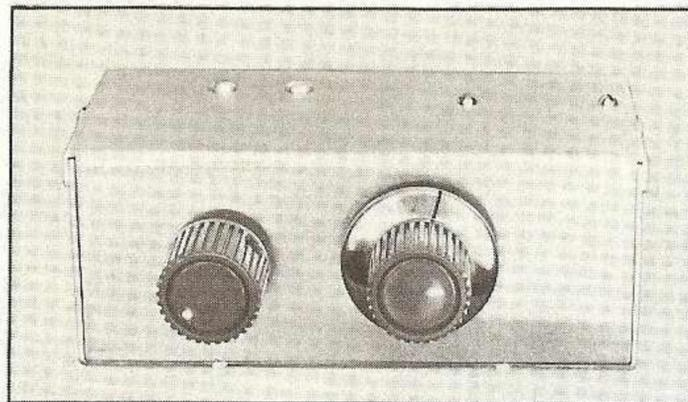
Fig. 23 The transistorized Q-multiplier works with any receiver having a 455 kc i-f amplifier. Life of the self-contained battery is extremely long, due to low current drain of transistor.
