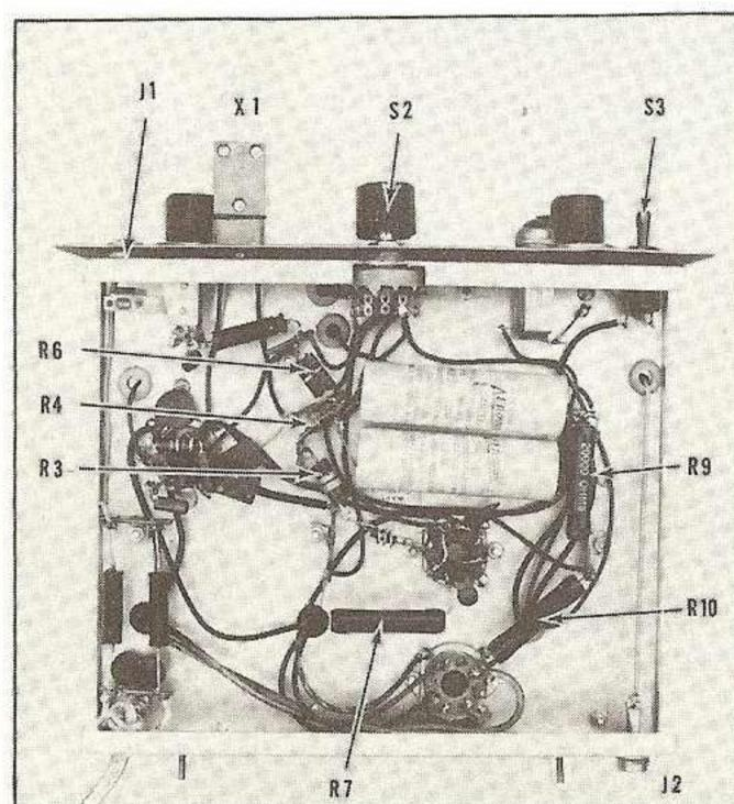
**Fig. 21** Under-chassis view of AB-60 transmitter. High voltage filter capacitors are near the center of chassis, supported at right end by two terminal tie-point strip. Oscillator components are at left.
