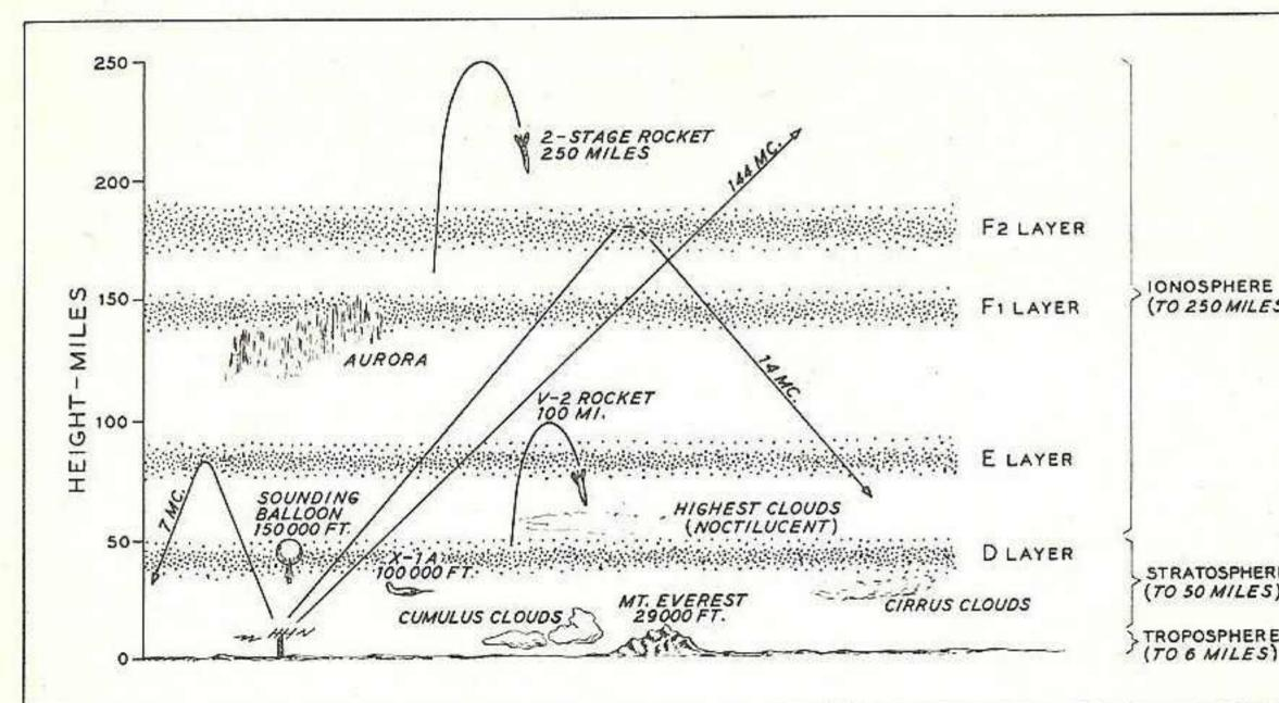
Fig. 4 The earth's atmosphere is composed of three layers, the lowest of which is the troposphere, or weather layer. The stratosphere (constant temperature zone) is next, extending to a height of about 40 miles. Above this is the ionosphere (ion layer) which is the region of reflection of radio signals. This layer is about 200 miles thick, extending to a height of approximately 250 miles.
