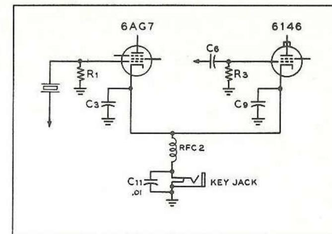
Fig. 4 Oscillator and amplifier may both be keyed in cathode circuit. Extra capacity is added across key (C11) to reduce key-click. R-f choke is added to keying circuit to reduce the harmonic radiation from the key leads.
