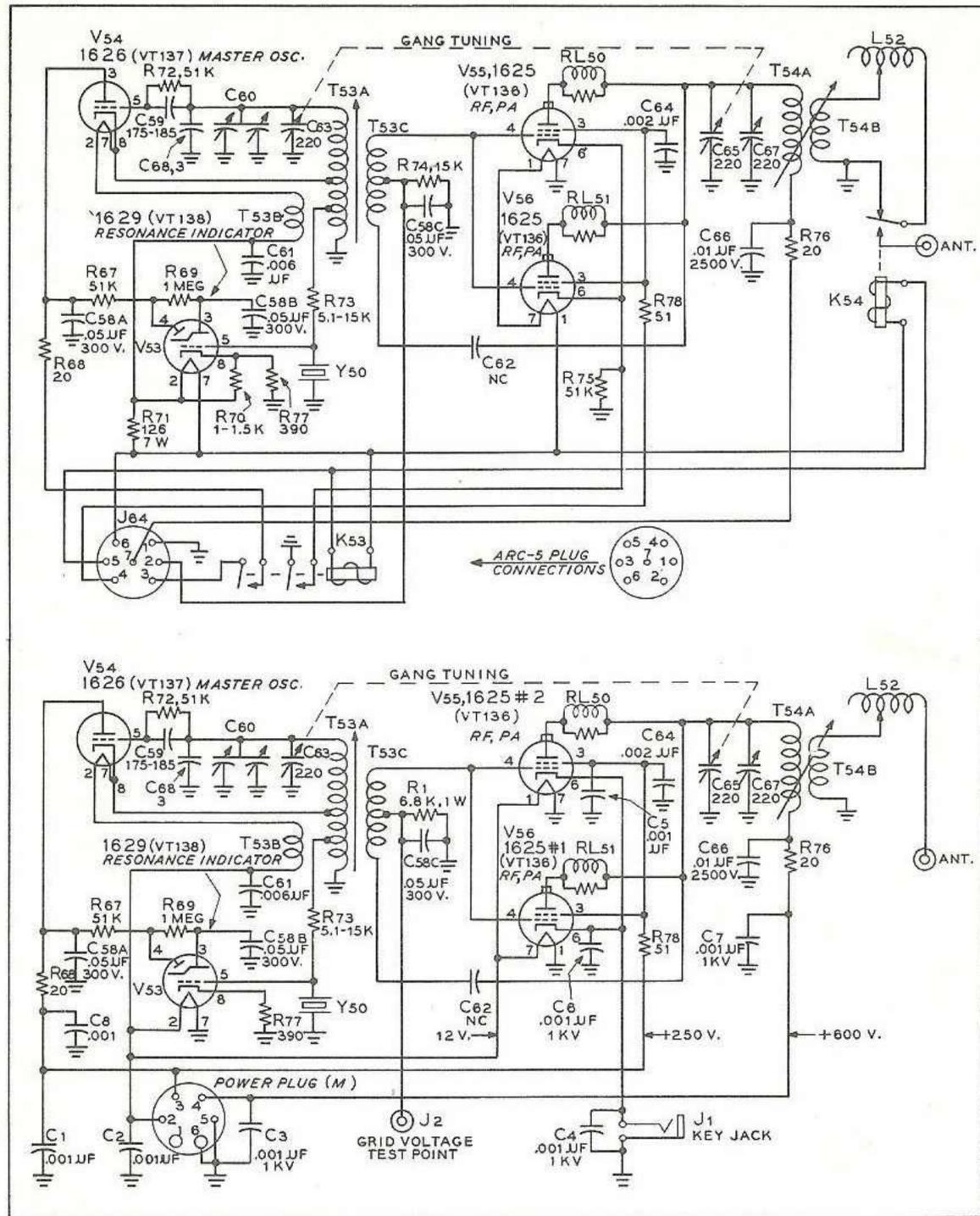
Fig. 10 Circuit of "Command" transmitter, before and after conversion.
