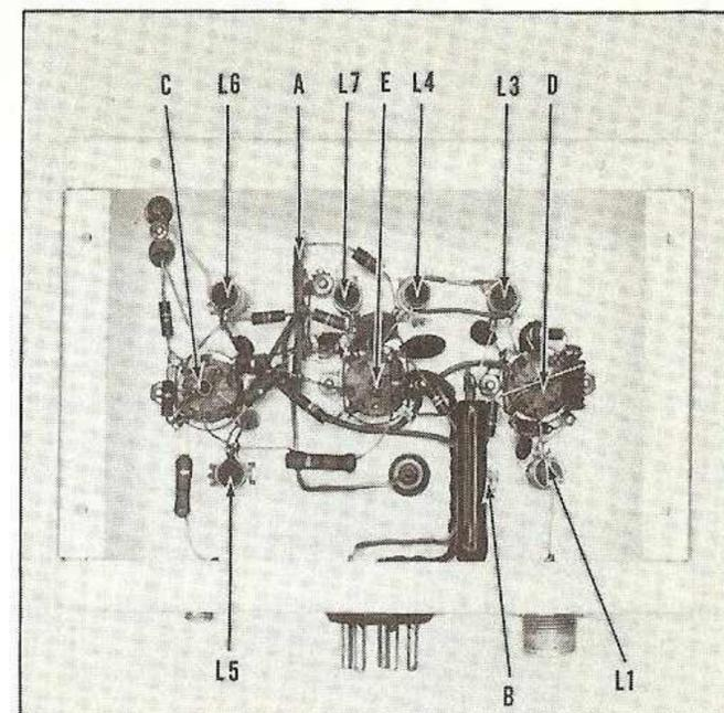
Fig. 18 Under-chassis view of 2N6 converter. Placement of major components is indicated. Crystal socket X1 is at upper left, and test point J1 is at center, below socket E. Note that all leads are short and direct. The 6BQ7A shield plate may be seen bisecting socket D.
