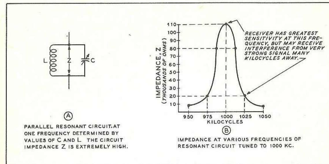
Fig. 1 The resonant tuned circuit has the ability to select radio signal of a given frequency, and to reject others at unwanted frequencies. Efficiency of rejection is determined by the "Q," or figur of merit of the circuit, and is largely determined by design and construction of the inductor (L).
