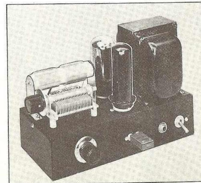
Fig. 5 The SP-50 transmitter runs 50 watts input on the 7 mc and 3.5 mc amateur bands. A 1614 pentode is used as a crystal oscillator, and a 5U4-GB serves as a high voltage rectifier. A built-in antenna tuner is a feature of the SP-50.
