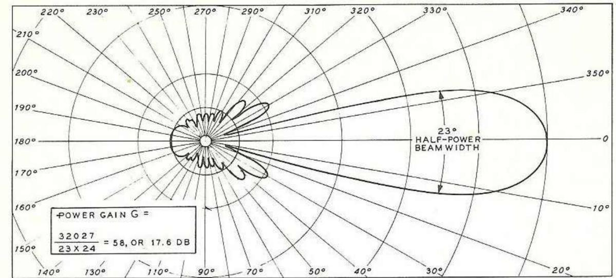
Fig. 3 A "beam antenna" concentrates the radio energy in one chosen direction, as shown in this horizontal pattern. Superimpose this plot upon a map and you will see how the radio signal may be "squirted" in the wanted direction.
