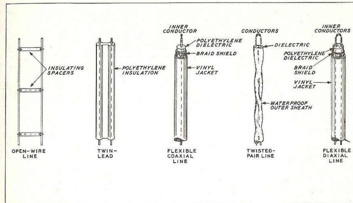
Fig. 1 Five types of transmission lines used by amateurs. The "TV-type twin lead" and shielded coaxial lines (RG-8/U and RG-59/U are the most popular.
