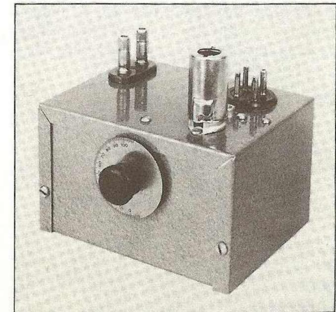
Fig. 1 The midget preselector is only 3" x 4" x 5" in size. A 6AK5 pentode tube in a unique all-band tank circuit provides maximum gain from 3.3 mc to 33 mc. Antenna terminals are at the left, and power plug and i-f output receptacles are behind the tube socket.
