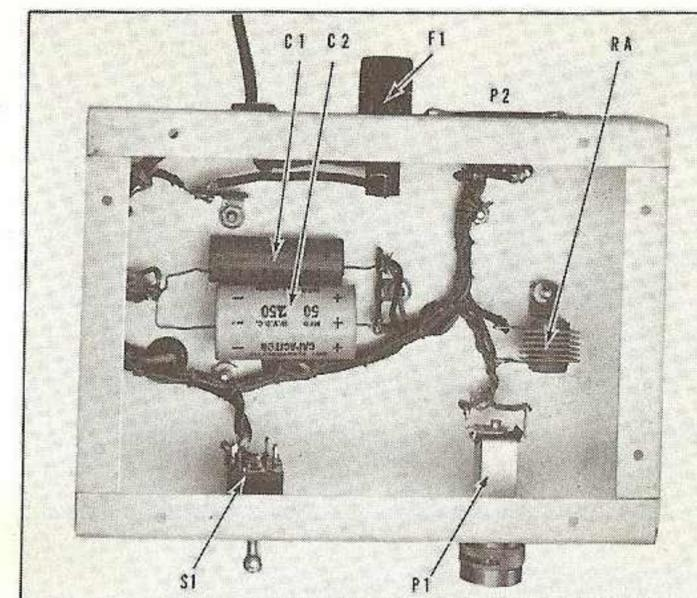
Fig. 6 Under-chassis view of low voltage supply, showing placement of major parts. The selenium rectifier is mounted to the chassis with a long 6-32 bolt.
