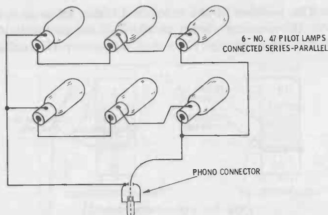
Fig. 5-6. Dummy-load bank for transmitter testing.
