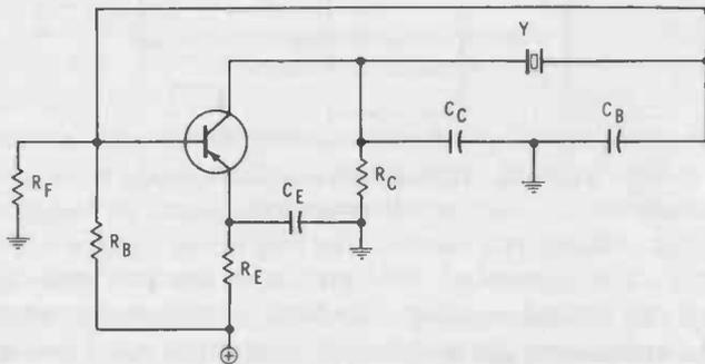
Fig. 2-23. Common-emitter Pierce oscillator.
