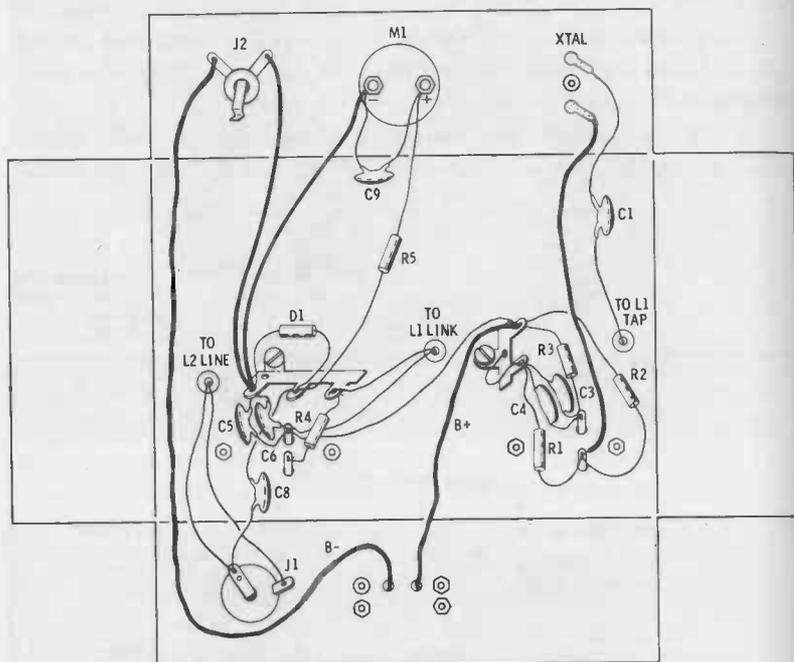
Fig. 5-4. Pictorial chassis-wiring diagram.
