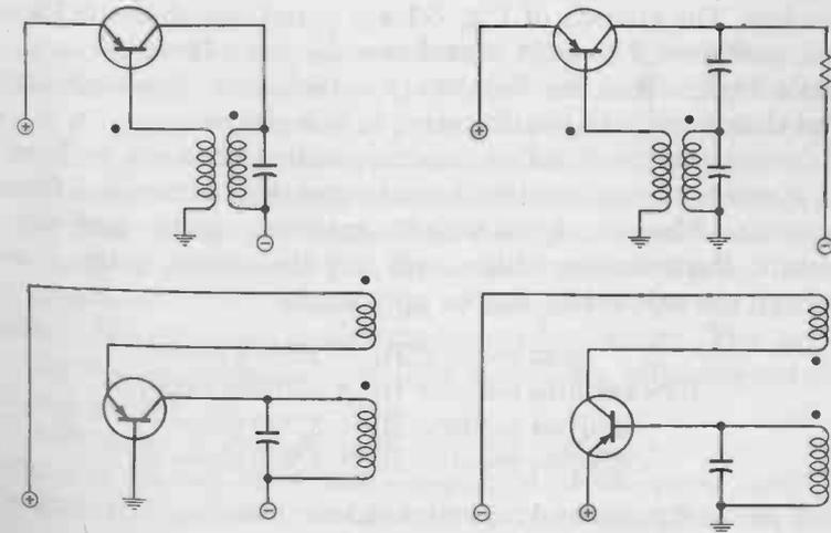
Fig. 2-1. Variations of tickler-coil oscillators.
