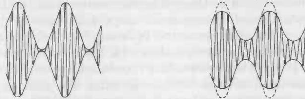
(A) Typical modulation envelope of a vacuum-tube final amplifier.
