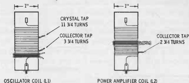
Fig. 5-5. Coil-winding detail.
