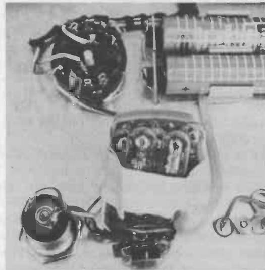
Fig. 1-16. Practical dummy-load system for transmitters.
