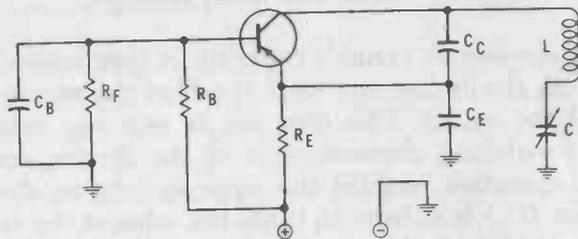
Fig. 2-15. Alternate Clapp oscillator circuit.
