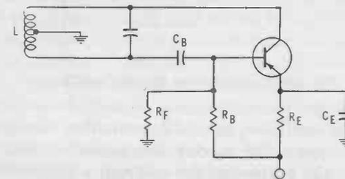
Fig. 2-8. Hartley-type oscillator.
