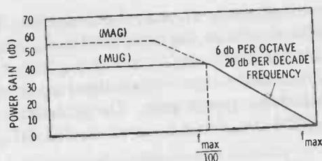
Fig. 1-8. High-frequency characteristics of typical transistor.
