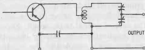
Fig. 4-6. Tapped coil for output impedance matching.
