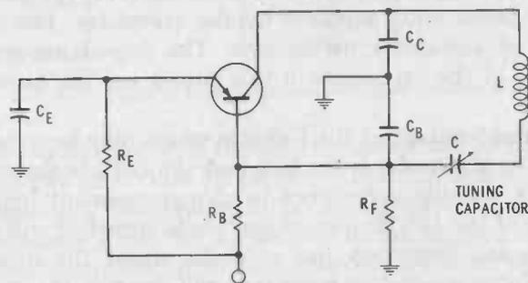
Fig. 2-14. Clapp oscillator configuration.
