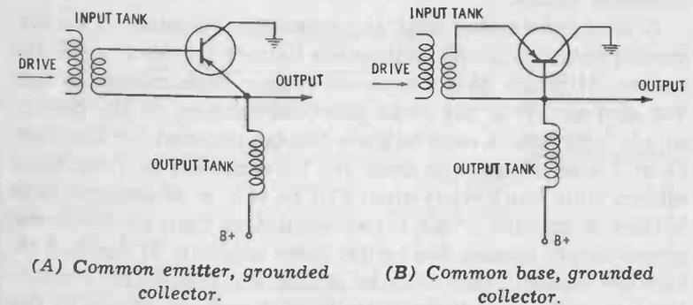
(A) Common emitter, grounded collector.
