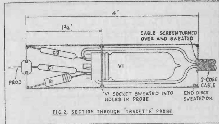
The back cover disc of the probe is drilled centrally to run over the screened cable, slipped up to the probe housing and the screening of the cable is unravelled for a  $\frac{1}{4}$ " or so and sweated down on to the interior face of the back disc, thus providing both a firm cable anchorage and the earth return between the probe and the main amplifier.
