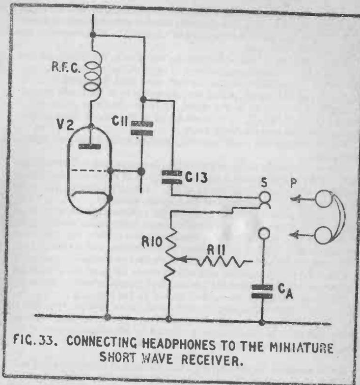
FIG. 33. CONNECTING HEADPHONES TO THE MINIATURE SHORT WAVE RECEIVER.
