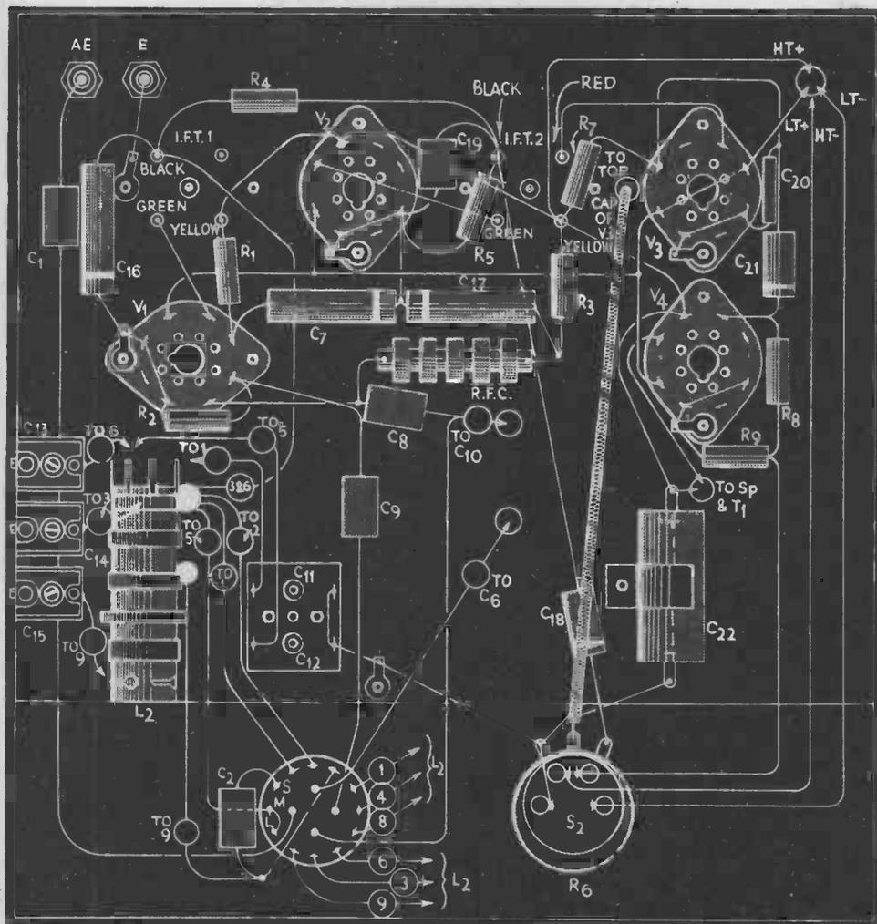
FIG. 19.—UNDER-CHASSIS VIEW OF THE BATTERY SUPERHET
