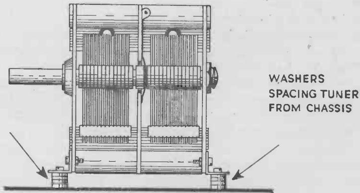
FIG. 9—MOUNTING THE TUNING CAPACITOR
