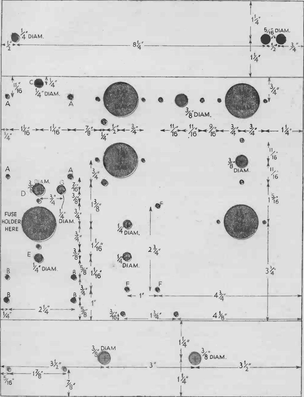
FIG. 21—THE A.C. MAINS SUPERHET, CHASSIS TOP VIEW
