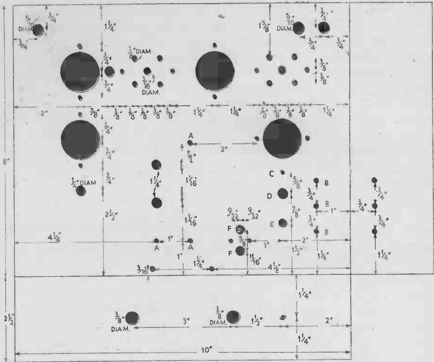
FIG. 18—THE BATTERY SUPERHET CHASSIS, TOP VIEW
