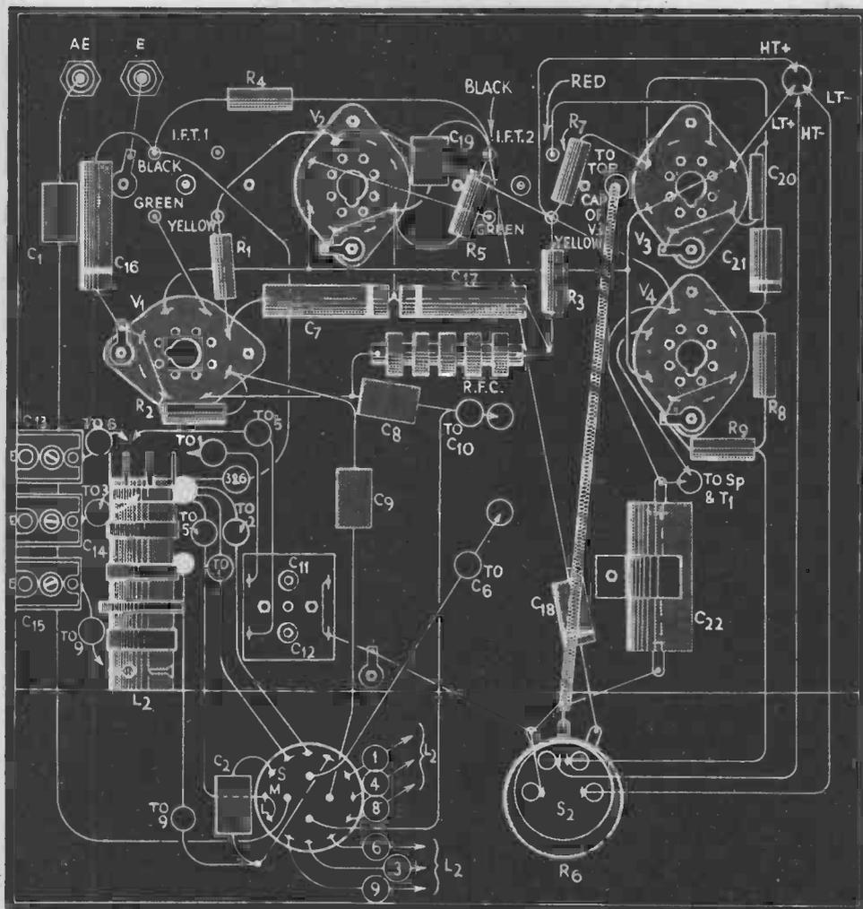
FIG. 19.—UNDER-CHASSIS VIEW OF THE BATTERY SUPERHET
