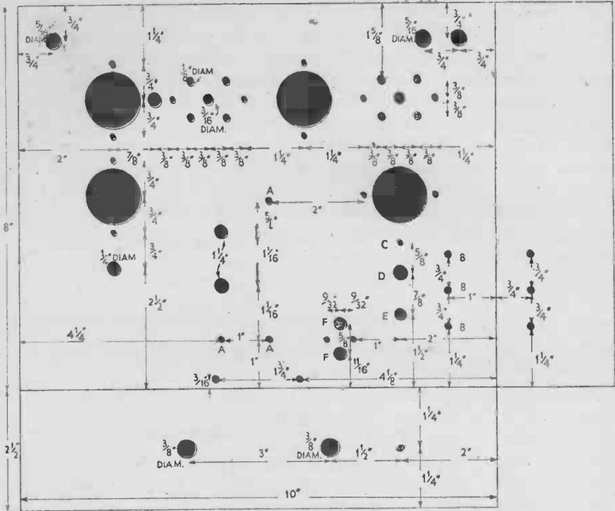
FIG. 18—THE BATTERY SUPERHET CHASSIS, TOP VIEW
