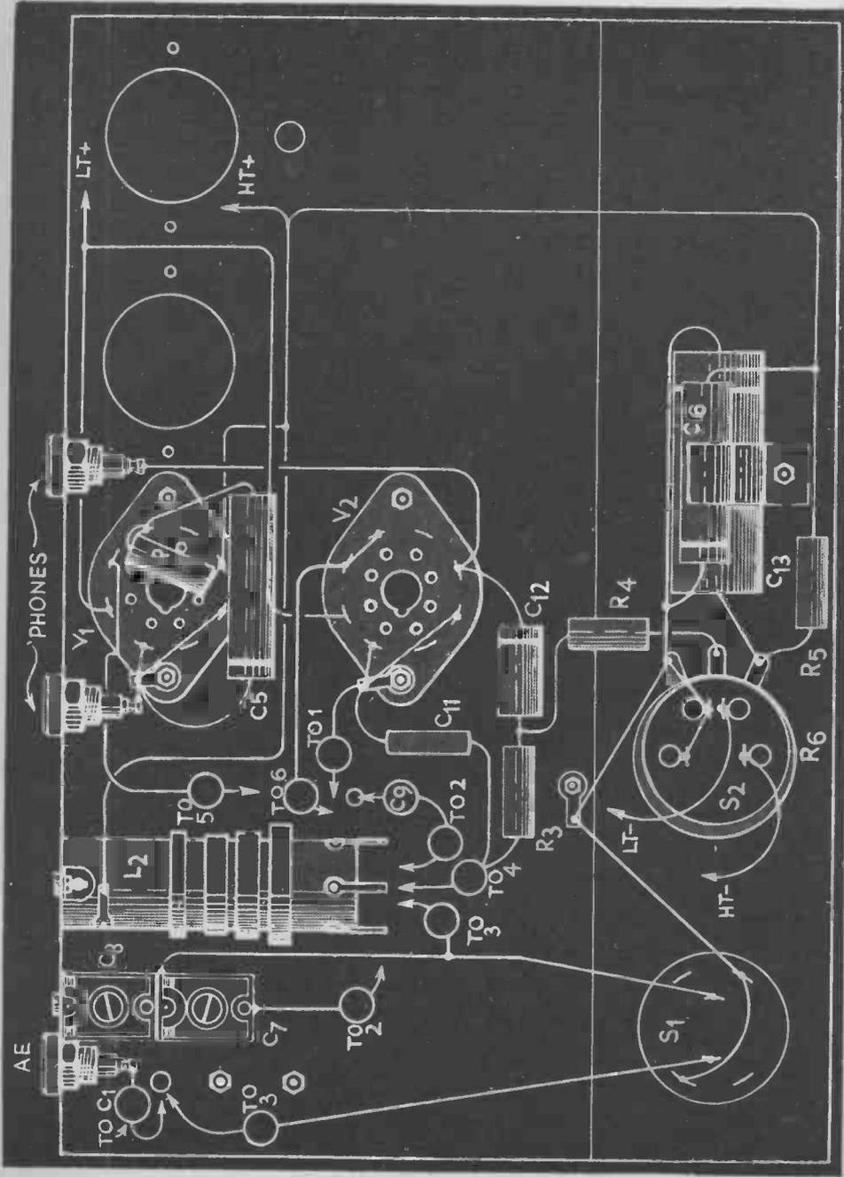
FIG. 11—UNDER-CHASSIS VIEW OF THE TWO-VALVE RECEIVER
