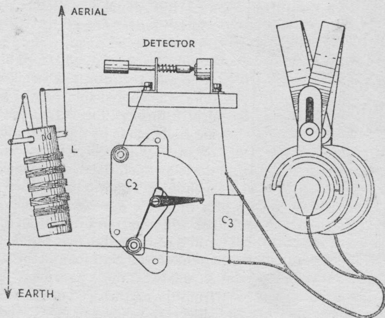
FIG. 2—THE CRYSTAL RECEIVER "HOOKED UP"
