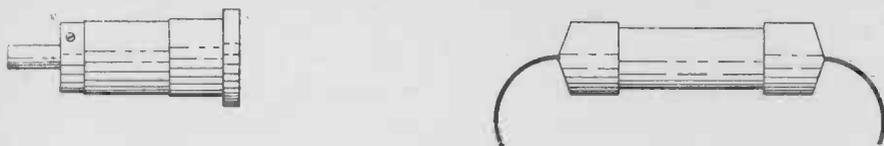
FIG. 4—RADAR CRYSTALS
