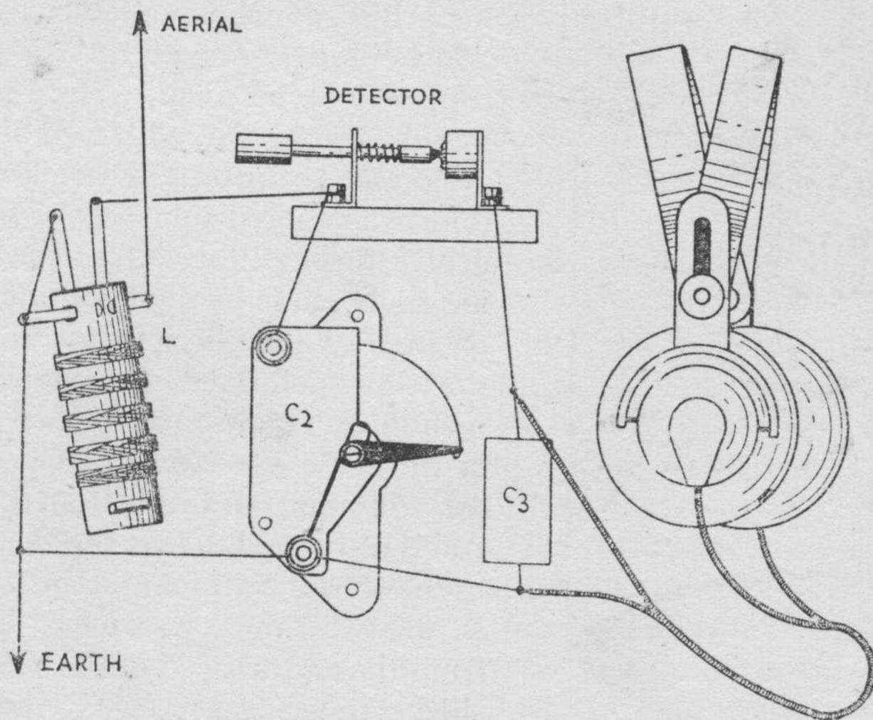
FIG. 2—THE CRYSTAL RECEIVER "HOOKED UP"
