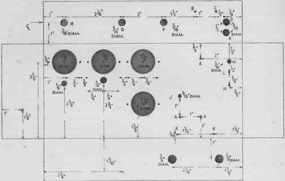
FIG. 7.—TOP VIEW OF THE CHASSIS, SHOWING HOW TO DRILL IT
