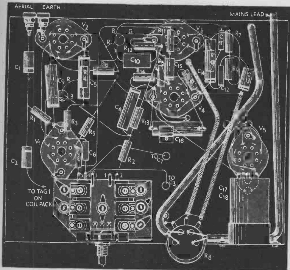
FIG. 22—THE A.C. MAINS SUPERHET, UNDER-CHASSIS VIEW, HEATER WIRING NOT SHOWN
