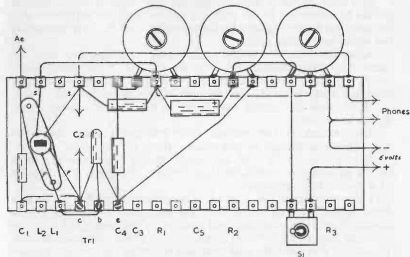
FIG. 11. EXPERIMENTAL LAYOUT
