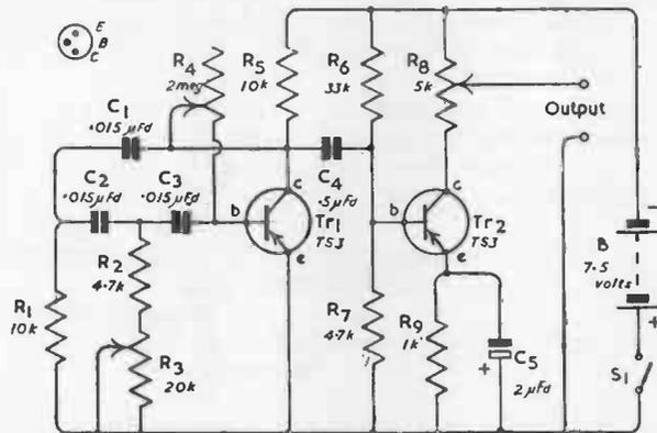
FIG. 12. A PHASE SHIFT OSCILLATOR
