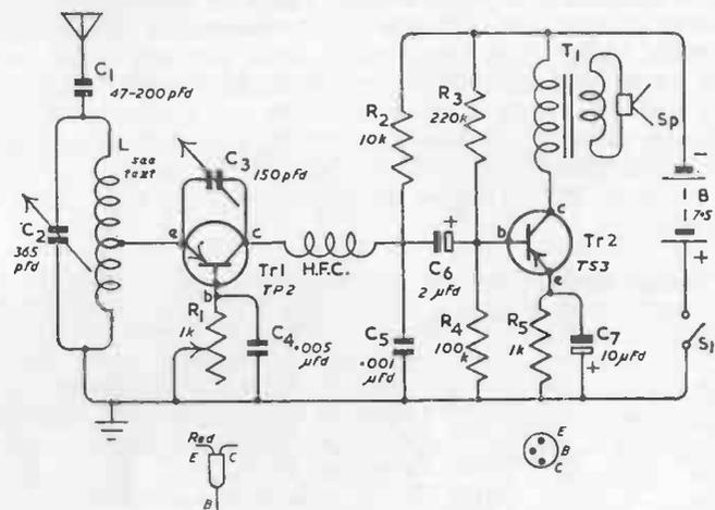
FIG. 4. A BEDSIDE RECEIVER USING A POINT-CONTACT DETECTOR
