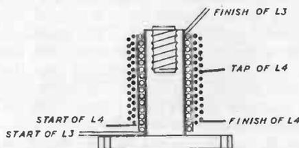
FIG. 7. AERIAL AND OSCILLATOR COIL DETAILS
