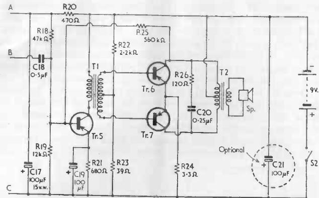
FIG. 6. THE 1-WATT OUTPUT STAGE
