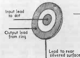
FIG. 1. A TRANSFILTER ELEMENT AND ITS TECHNICAL SYMBOL
