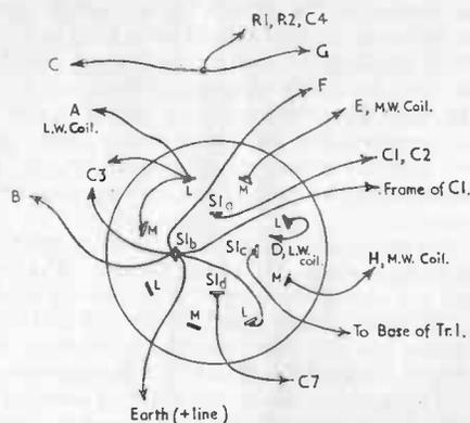
FIG. 12. SWITCH WIRING OF THE TRANSFILTER RECEIVER
