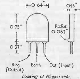
FIG. 2. TRANSFILTER DIMENSIONS AND CONNECTIONS
