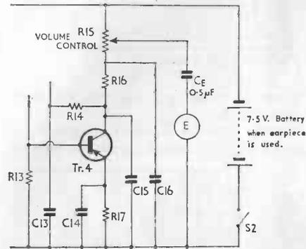
FIG. 9. PERSONAL EARPIECE OUTPUT FROM THE DETECTOR
