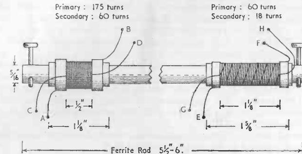
FIG. 11. DIMENSIONS OF THE FERRITE AERIAL (COILS SHOWN DIAGRAMMATICALLY)
