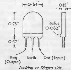
FIG. 2. TRANSFILTER DIMENSIONS AND CONNECTIONS
