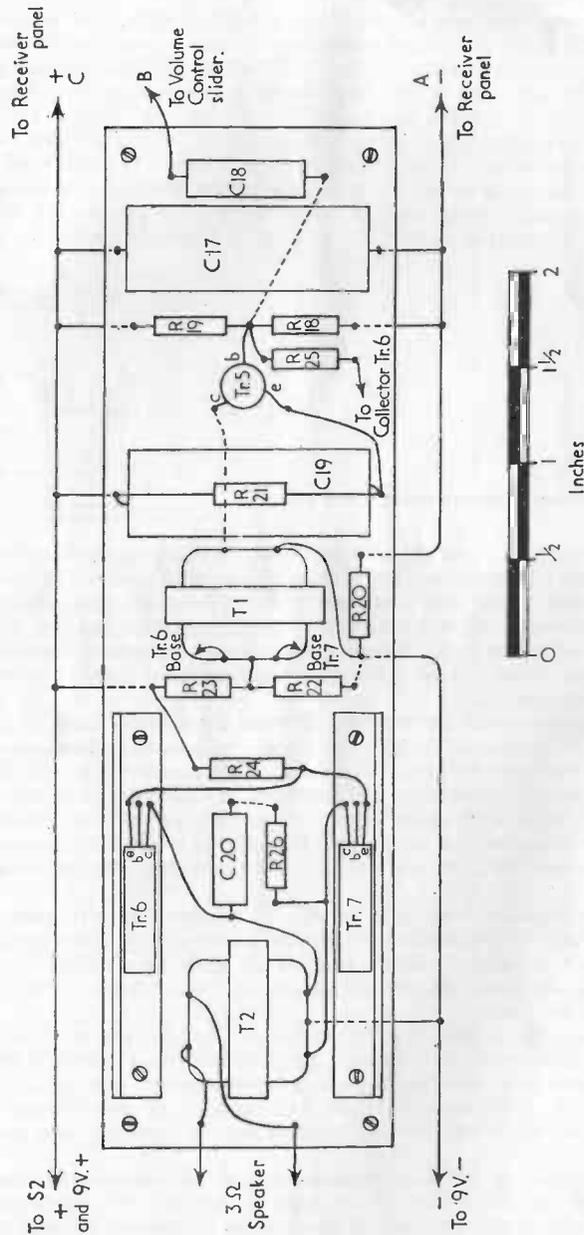
FIG. 7. THE 1-WATT OUTPUT STAGE PANEL
