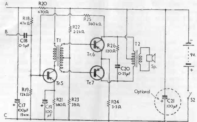
FIG. 6. THE 1-WATT OUTPUT STAGE
