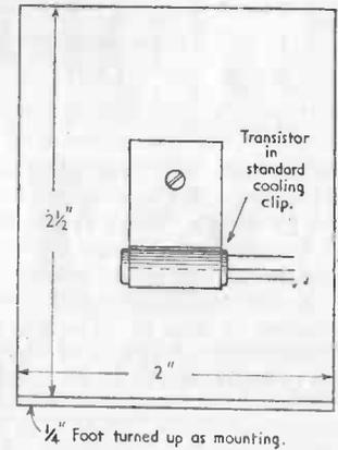
FIG. 8. THE HEAT-SINK AND TRANSISTOR MOUNTING
