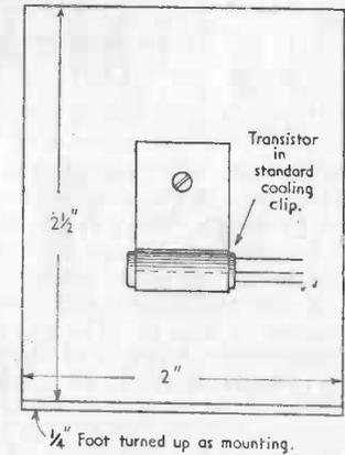
FIG. 8. THE HEAT-SINK AND TRANSISTOR MOUNTING
