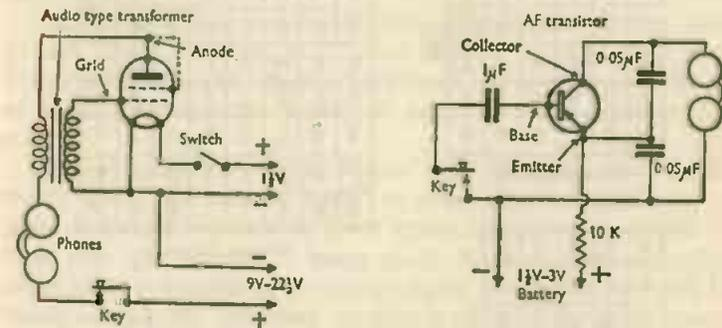
FIG. 3. Two oscillators suitable for Morse practice
