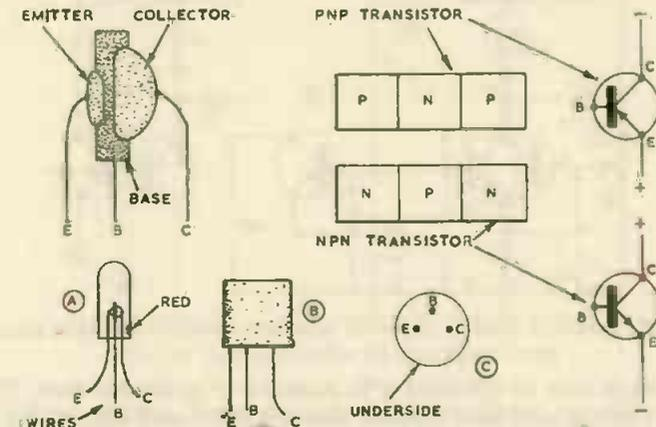
FIG. 91. Details of transistors
