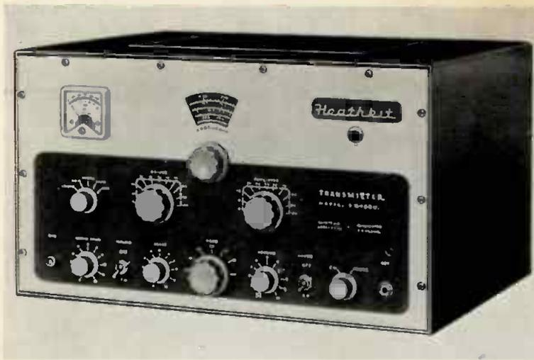
2. Above DX-100U table top transmitter, for speech and CW, 150 watts. 3. Below Morse practice outfit - transistor oscillator built to circuit in Chapter 1, and key.
