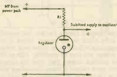
FIG. 69. Voltage regulation circuit to provide stabilized HT
