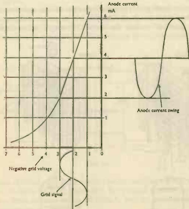
FIG. 18. Operation of class A amplifier
