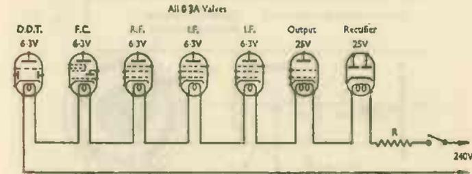
FIG. 7. Series heater circuit with mains dropper
