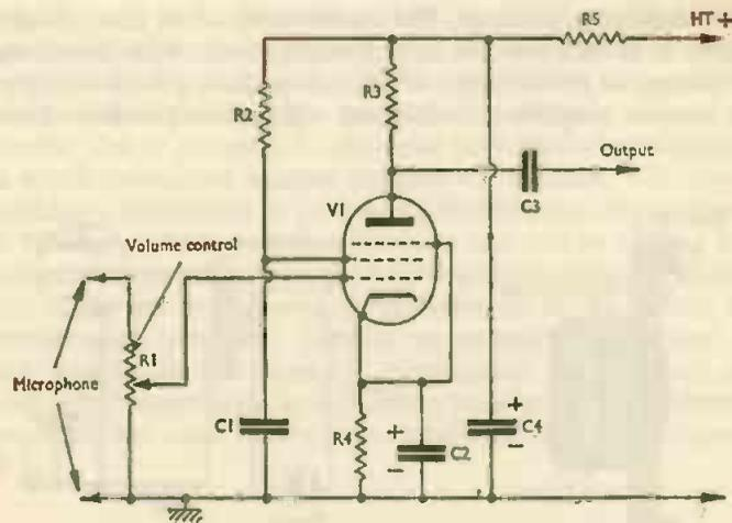
FIG. 59. Pre-amplifier or first audio stage
