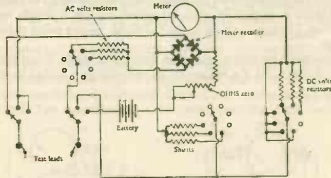
FIG. 81. Circuit of a multi-Range Test Meter.
