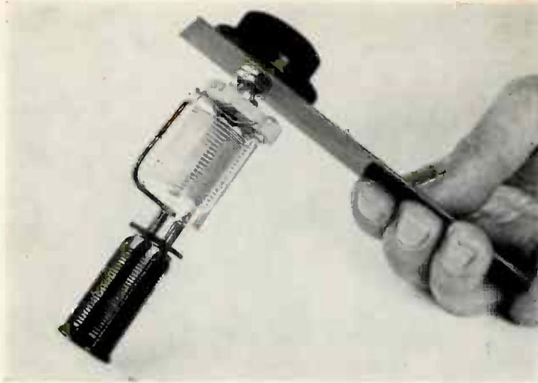
10. Above Absorption meter, as described in chapter on measurements.
