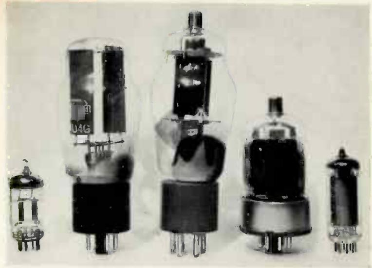
8. Above Receiver and transmitter valves: 1, 6B7G double triode; 2 5U4G full-wave rectifier; 3, 807 (top anode cap); 4, 6146 (top anode cap); 5, 6BW6 miniature output tetrode. 9. Below DX-40U 10 to 80 mc transmitter, 75 watts CW, 60 watts peak controlled carrier phone. (Heathkit Daystrom Ltd., Gloucester.)
