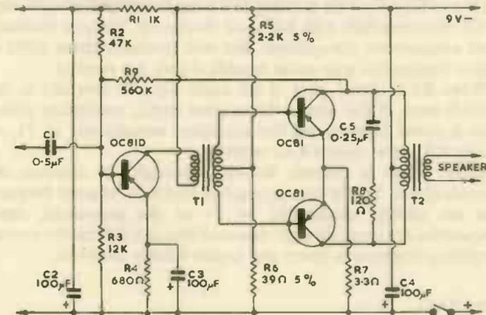
FIG. 98. Driver and push-pull output for  $\frac{1}{2}$  watt to 1 watt
