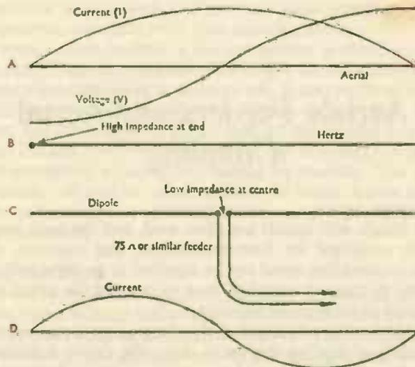
FIG. 70. Half-wave aerials A, B, and C. D is full-wave
