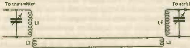
FIG. 46. Link coupling for use between valves or between transmitter and aerial tuner
