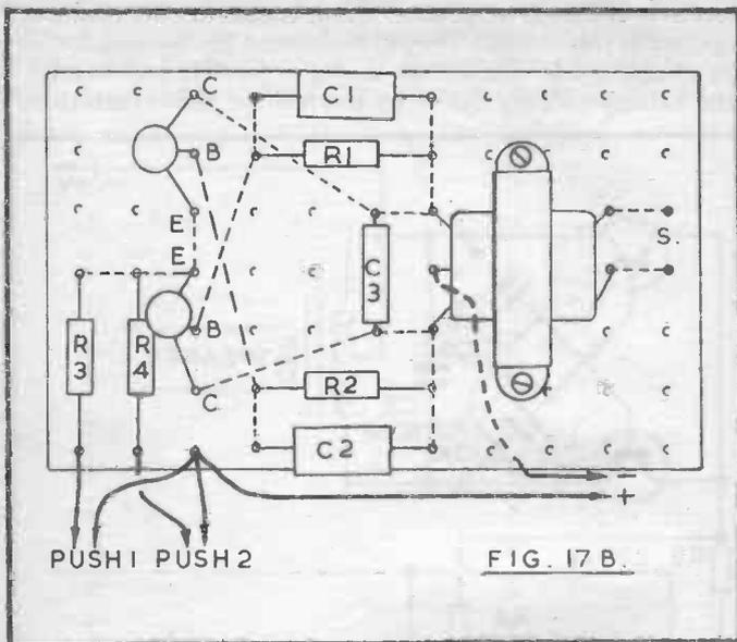
In some circumstances it may be convenient to run a single twin lead from Push 1 on to Push 2, including an extra resistor at Push 2 itself, to modify the tone. This may save taking leads from Push 2 all the way back to the oscillator board.
