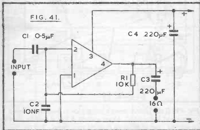
Audio input is to 2 of the IC, from the isolating capacitor C1. C2 is a by-pass capacitor to maintain stability. The IC has only four connections, 1 going to the negative line, and 3 to the positive supply. Audio output is from 4, and to the loudspeaker via C3. R1 provides negative feedback and bias to point 2.
