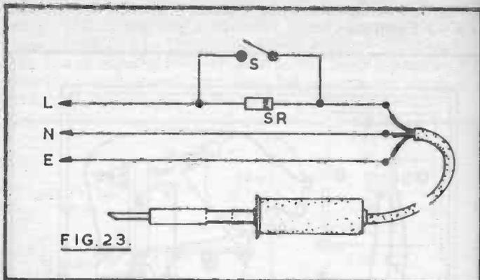
This device can be made by using an insulated junction box which will take a socket outlet and also the switch S. A 3-core cord with plug is run to the box, so that it can be used with any power point. The iron or other item can then be plugged into the outlet fitted to the junction box. Remember to make mains connections in the way described earlier, for safety. The switch S should be of fully insulated type.
