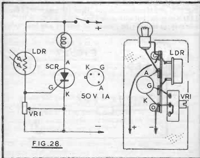
The LDR has a high resistance when in darkness or subdued light, so that the gate potential of the SCR is not sufficiently high to trigger this device. When light reaches the LDR, its resistance falls, and the SCR gate voltage rises. The SCR then moves into its conducting condition, so that current flows through the bulb. The sensitivity of the circuit, or level of illumination needed to trigger the SCR, is set by VR1.
