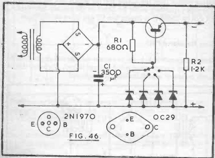
R1 supplies current for any diode, and 1 watt diodes should be used. With a 24v transformer and large transistor such as the 2N1970 or OC29, an output of up to 1 ampere can then be drawn. The bridge rectifier must of course be rated at 1A or higher.
