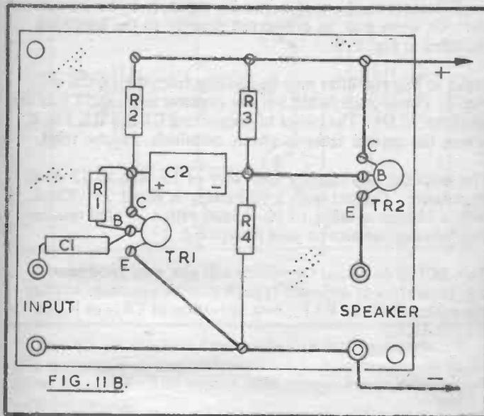
The board can be secured with bolts through its fixing holes, and through the bottom of the case. Extra nuts or other spacers must be placed between the case and board.
