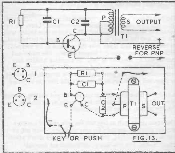
(1) shows leads from a typical NPN transistor, such as the BC108, 2N706, and similar types. (2) is the base of the PNP AC128 transistor.
