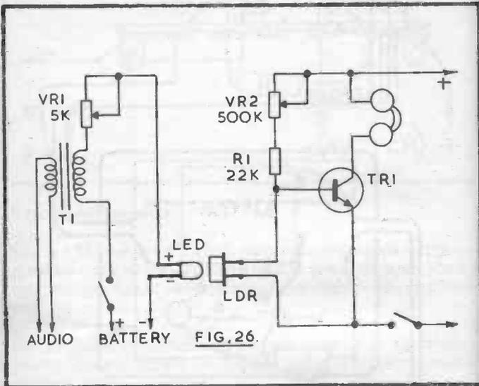
Electrically, the device is in two sections. The first has the light emitting diode LED, VR1, and transformer T1. When the battery is switched on, current flowing through the LED is adjusted by VR1, so that the LED glows dimly. A signal voltage in the secondary of T1 then modulates the LED light intensity.
