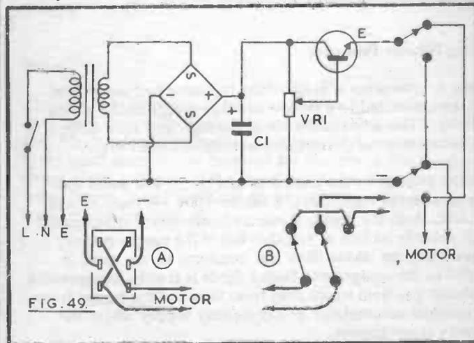
A transformer with a 12v secondary will be suitable for the usual model requiring up to 12v. The circuit is similar to that of the supply in Fig. 47. The potentiometer VR1 gives speed control. C1 can be around  $2,000\mu\text{F}$ .
