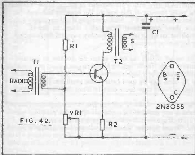
T1 is the coupling or driver transformer, which may receive audio signals from a radio receiver, smaller amplifier, or other equipment. A step down ratio of about 5:1 to 10:1 will generally prove to be suitable.
