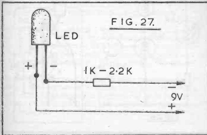
found by trial — the correct connections are those allowing the LED to light. The series resistor may be about 150 ohm to 1k or more, depending on the actual voltage, and brightness required. Current drawn varies with different LEDs, and with voltage and series resistance, but can be about 5mA or less, without reducing the brightness too far.
