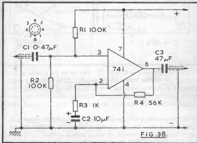
Modification to the values of R3 or R4 allow feedback and gain to be adjusted between quite wide limits, but for general purposes the values shown are satisfactory. A wide range of voltages (not exceeding 36v) may be used. The actual output is from a complementary pair, and is easily adequate for very good headphone volume, if required.
