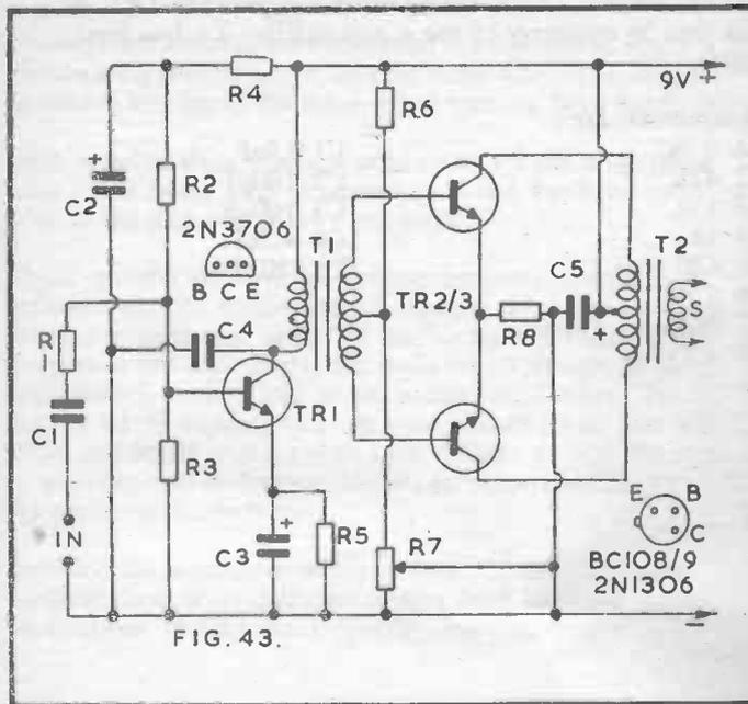
T1 is the driver transformer, with centre tapped secondary, so that TR2/3 may be operated in push-pull (see Fig. 12). T2 couples output to a 2/3 ohm speaker.
