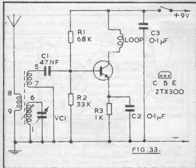
Fig. 33 is the circuit, and it uses a cored tuning coil with aerial coupling winding 8-9, tuned winding 6-1, and base coupling coil 5-7. These numbers are for the pins of the Denco (Clacton) "Blue" Range 2 component. It will be apparent that other coils, or surplus or home-wound inductors, can be substituted.
