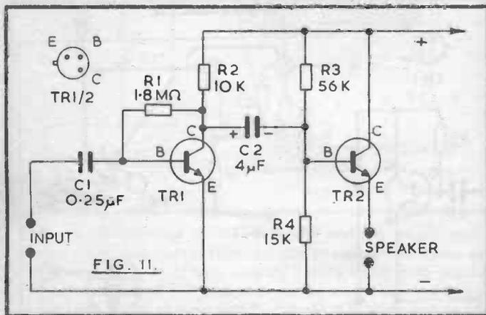
C1 couples the audio signal to the base of the first amplifier TR1, which receives base current through R1. An amplified signal is developed across the collector resistor R2, and is coupled to the base of the following amplifier TR2 by means of C2.
