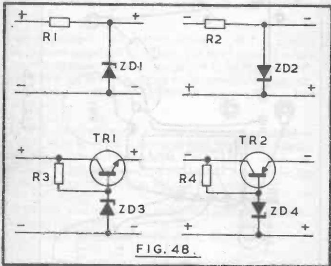
The second circuit is virtually the same, but polarity is reversed, so that the ground return is positive.
