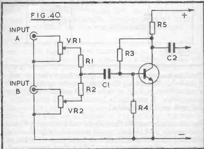
Input A has its individual volume control VR1, and Input B is similarly provided with VR2. Resistors R1 and R2 prevent short circuiting one input when the other potentiometer is set at zero. Coupling to the transistor base is by C1. R3 and R4 set base bias conditions, with R5 as the collector load and audio output from C2.
