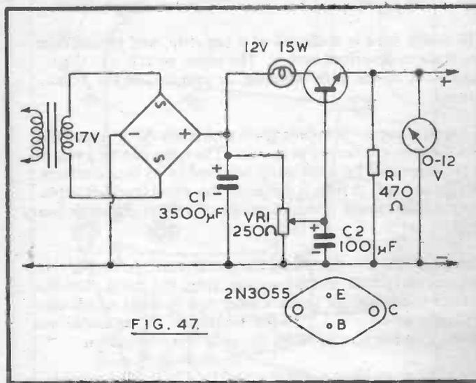
VR1 is panel mounted, and allows the base potential of the control transistor to be set at the required voltage. C2 provides "electronic smoothing" from the base circuit.
