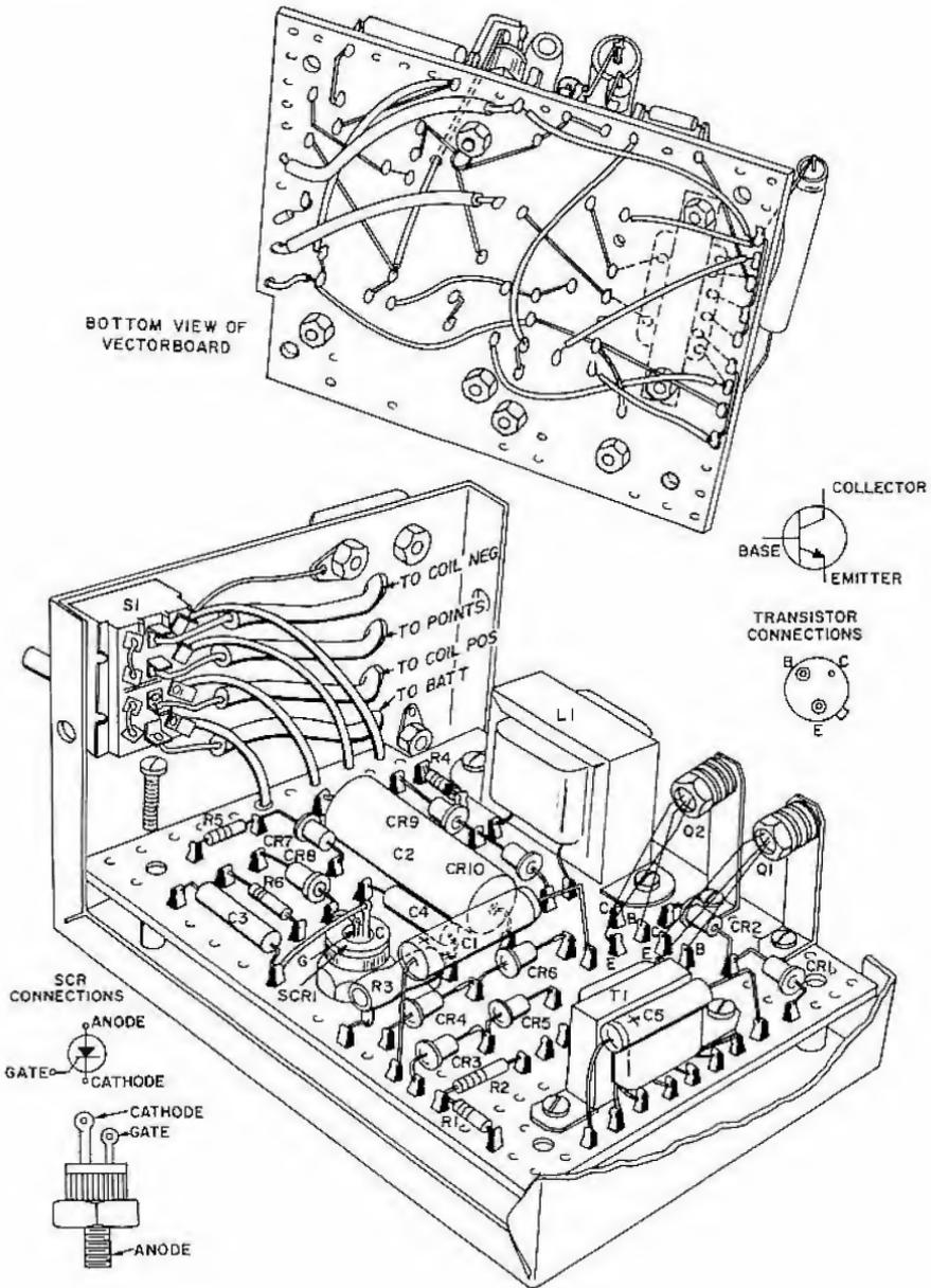
Figure A5.5 Capacitor discharge SCR ignition system pictorial diagram
