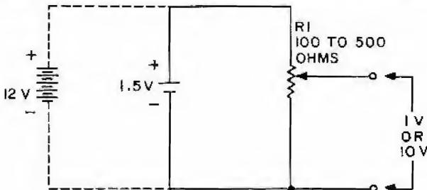
Figure W6.3 Voltage calibration source for adapter
