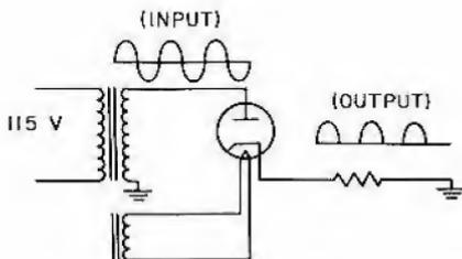
Figure 3. Diode connected for half-wave rectification
