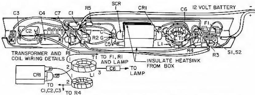
Figure H6.2 Battery-operated fluorescent light pictorial diagram
