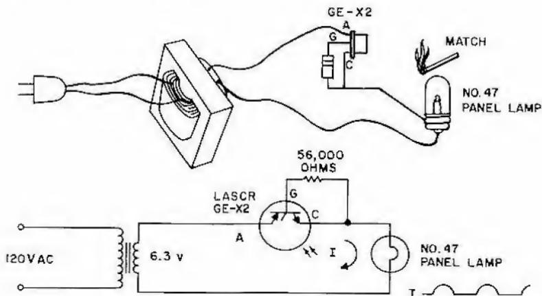
Figure 35. Electric candle circuit
