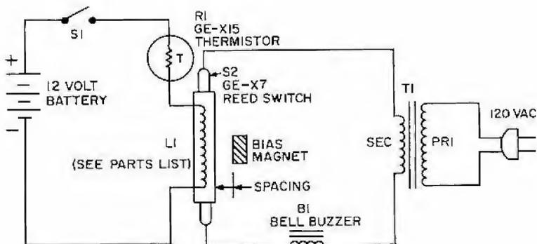
NOTE: BATTERY CIRCUIT CURRENT APPROXIMATELY 10 MILLIAMPERES. SELECT SUITABLE BATTERY
