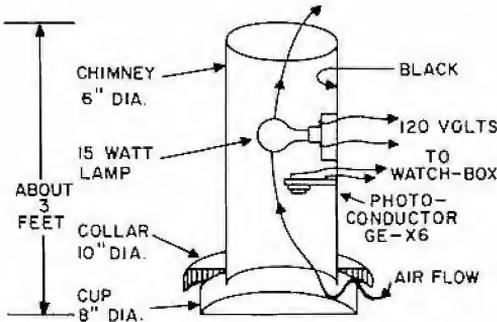
Figure H3.6 Cross-section view of smoke detector
