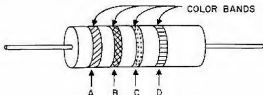
$$\text{Resistance} = (10A + B) \times 10^C \text{ ohms} \pm D$$
