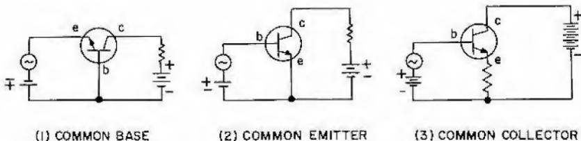
Figure 24. Transistor hook-ups
