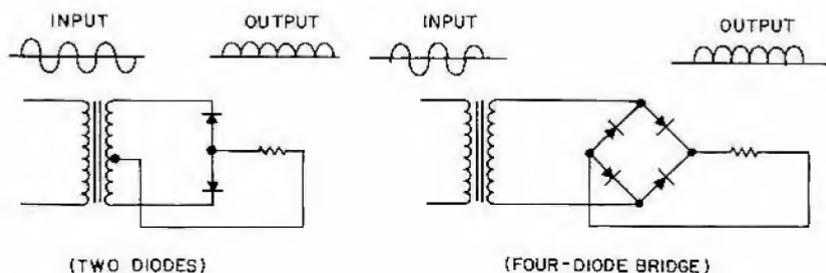
Figure 11. Solid-state full-wave rectifier circuits
