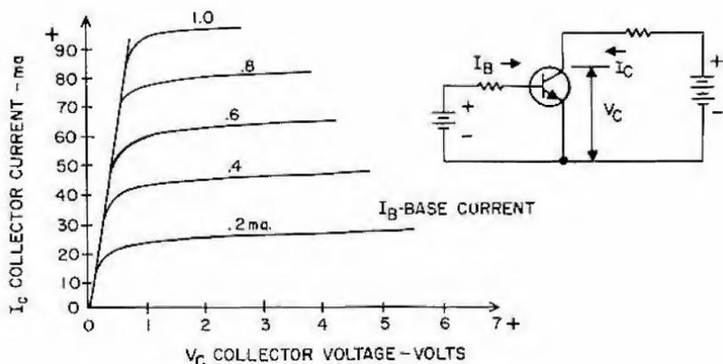
Figure 25. Transistor characteristic curves
