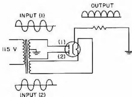
Figure 4. Diode connected for full-wave rectification
