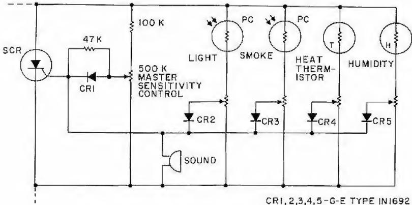
Figure H3.8 Multiple detector input circuit
