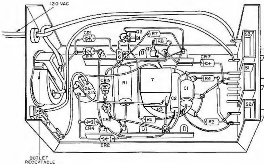
Figure H5.2 Time-dependent light dimmer pictorial diagram
