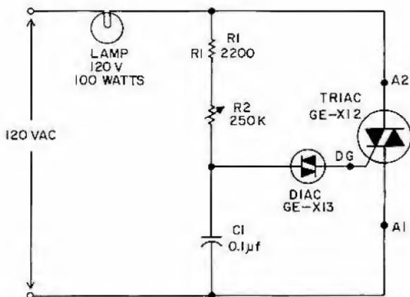
Figure 41. Basic Triac/Diac control circuit
