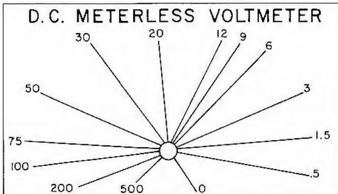
Figure W8.2 Scale used with calibrating potentiometers
