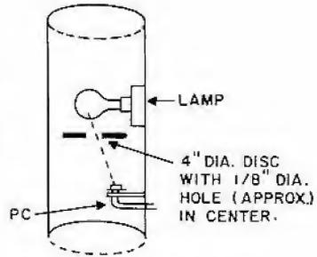
Figure H3.7 Alternate arrangement for smoke detector
