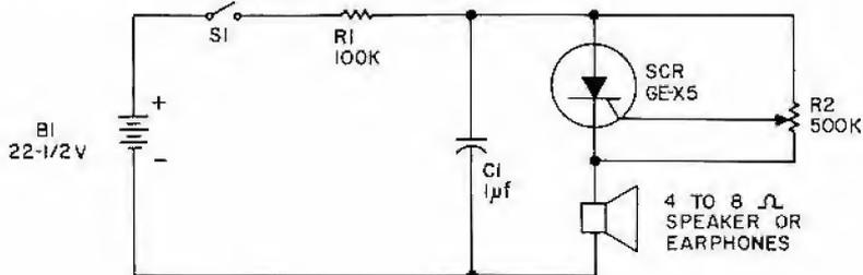
Figure H3.1 Basic relaxation oscillator schematic diagram
