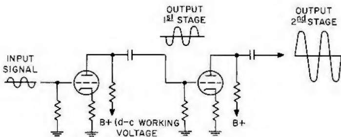
Figure 6. Two-stage triode amplifier
