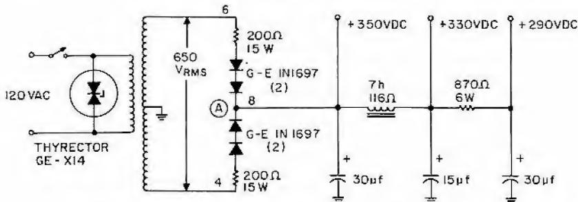
Figure W11.3 Alternate silicon rectifier replacement circuit—
