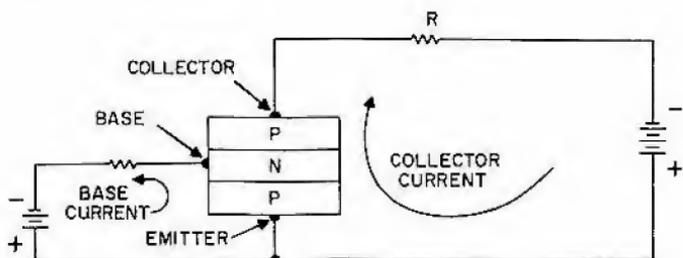
Figure 20. PNP transistor
