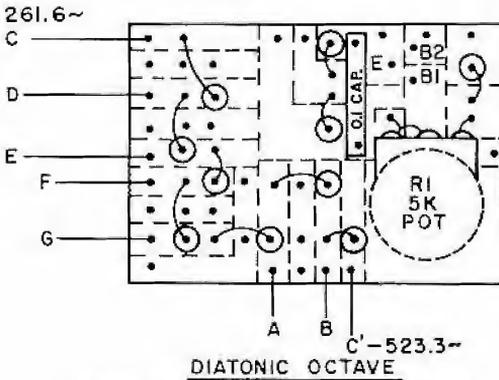
NOTE: USE POTENTIOMETER SHAFT NUT AS MOUNTING DEVICE.
