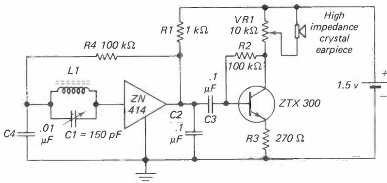
Figure 11. Adding a Transistor Amplifier to circuits in Figures 9 & 10.
