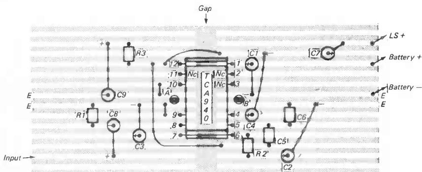
Figure 17. Veroboard layout of TCA 940 amplifier.
