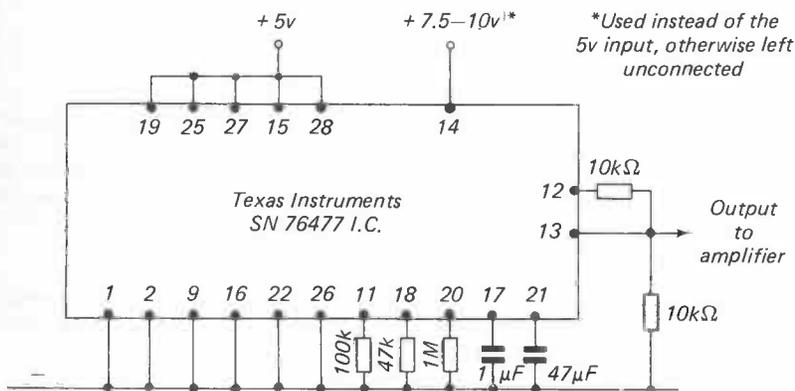
Figure 32. Texas design for "bleep-bleep" noise producer.
