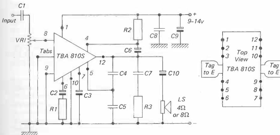
Figure 14. Audio Amplifier using TBA 810 S.
