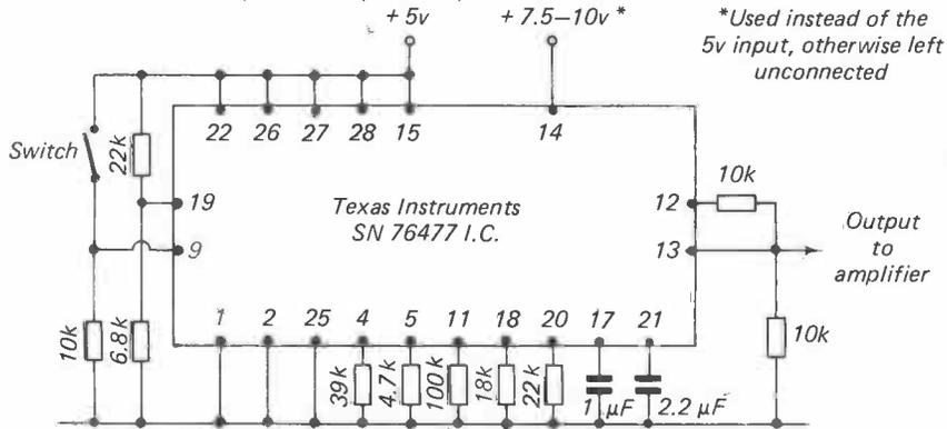
Figure 33. Texas design for "machine gun" noise producer.
