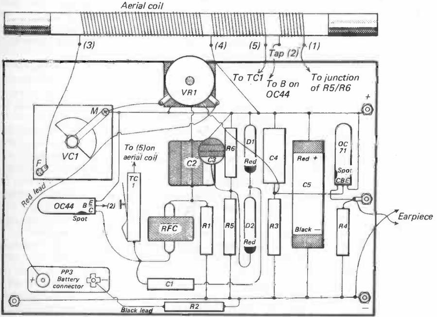
Figure 6B. Wiring diagram of the two-transistor pocket receiver.
