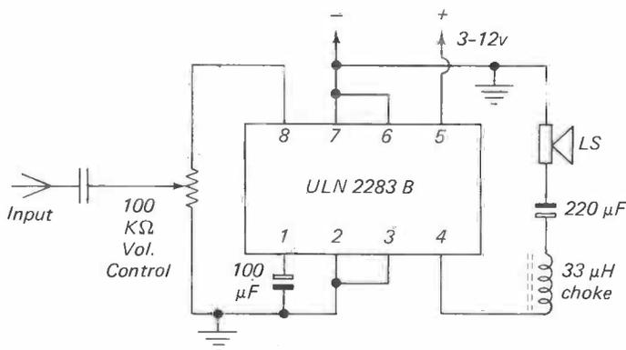
Figure 20. Schematic diagram of amplifier using ULN 2283 B.
