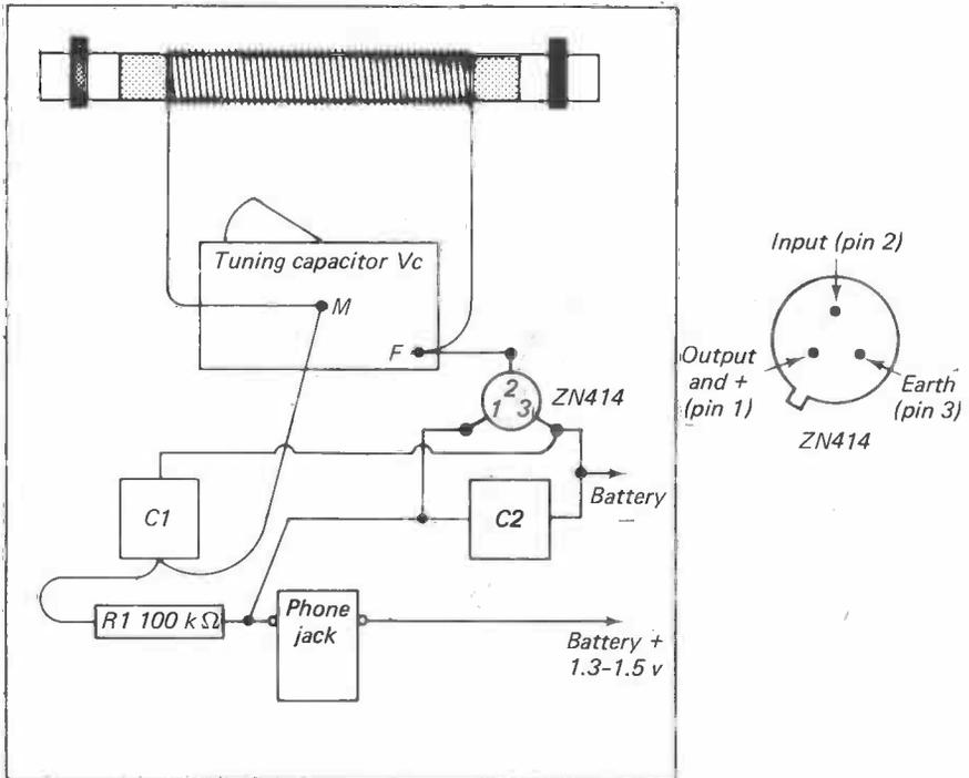
Figure 9. Wiring diagram of one-chip receiver.
