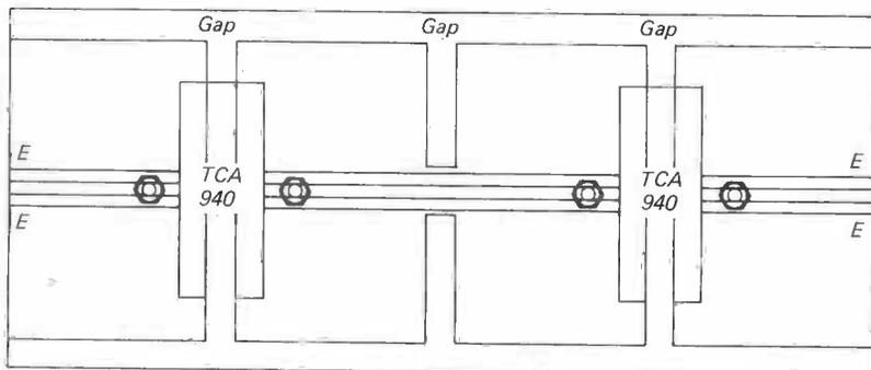
Figure 19. Layout for stereo amplifier.
