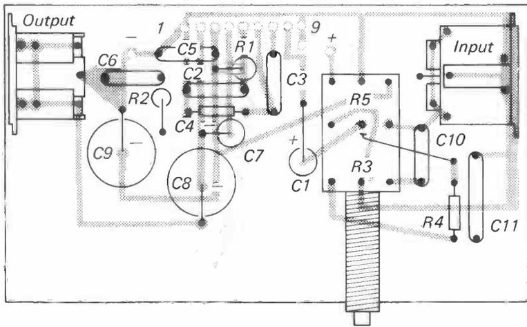
Figure 23. Track side (above) and component side (below) of layout of amplifier shown in Fig. 22. (Reproduced by courtesy of Mullard Ltd.)
