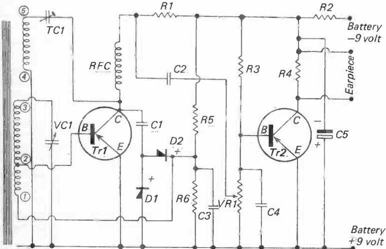
Figure 6A. Theoretical circuit and wiring diagram of the two-transistor pocket receiver.
