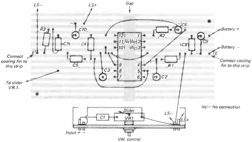
Figure 15. Veroboard mounting for Amplifier shown in Fig. 14.
