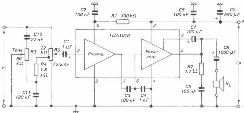
Figure 22. Complete mono audio amplifier using Mullard TDA 1010.
