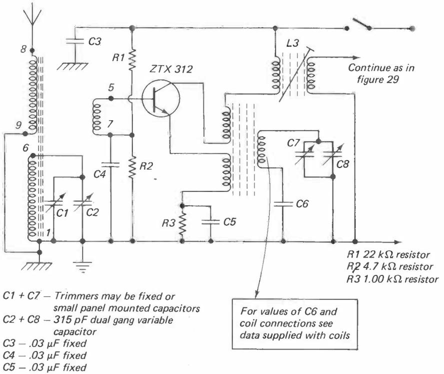
Figure 30. Denco short-wave coils for super-het "front end".
