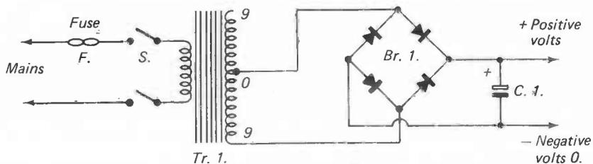
Figure 28. A mains unit for power supply.
