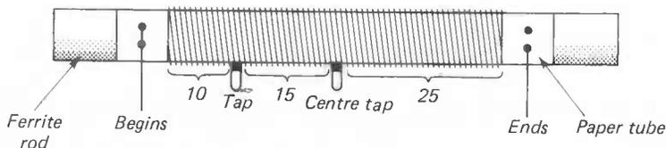
Figure 4. Ferrite Rod aerial coil.
