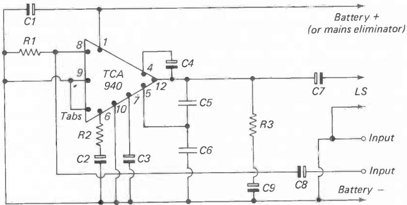
Figure 16. Schematic Diagram of TCA 940 amplifier.
