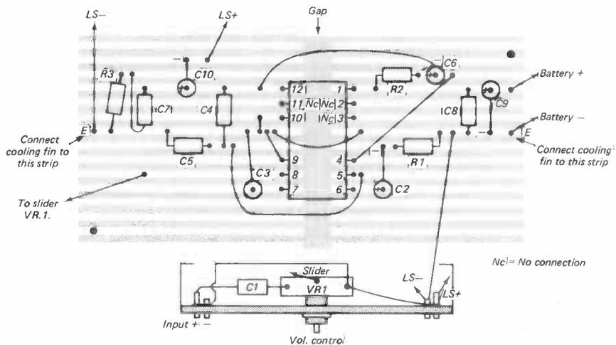
Figure 15. Veroboard mounting for Amplifier shown in Fig. 14.
