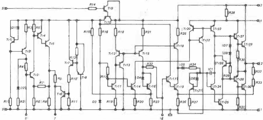
Figure 21. Internal connections of Mullard TDA 1010 chip.
