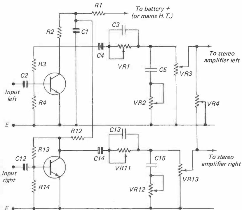
Figure 24. Pre-amplifier for stereo amplifier.
