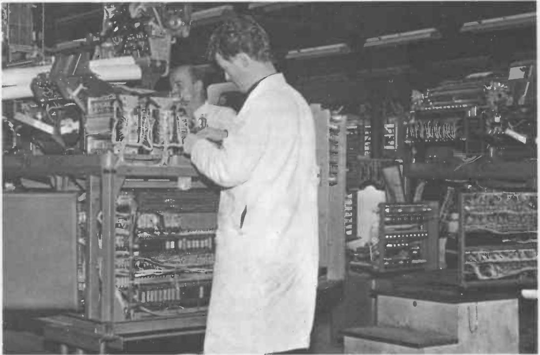
Fig. 26 Miles of complicated wiring go into a high-speed IBM accounting machine, here shown being assembled at their Greenock factory
