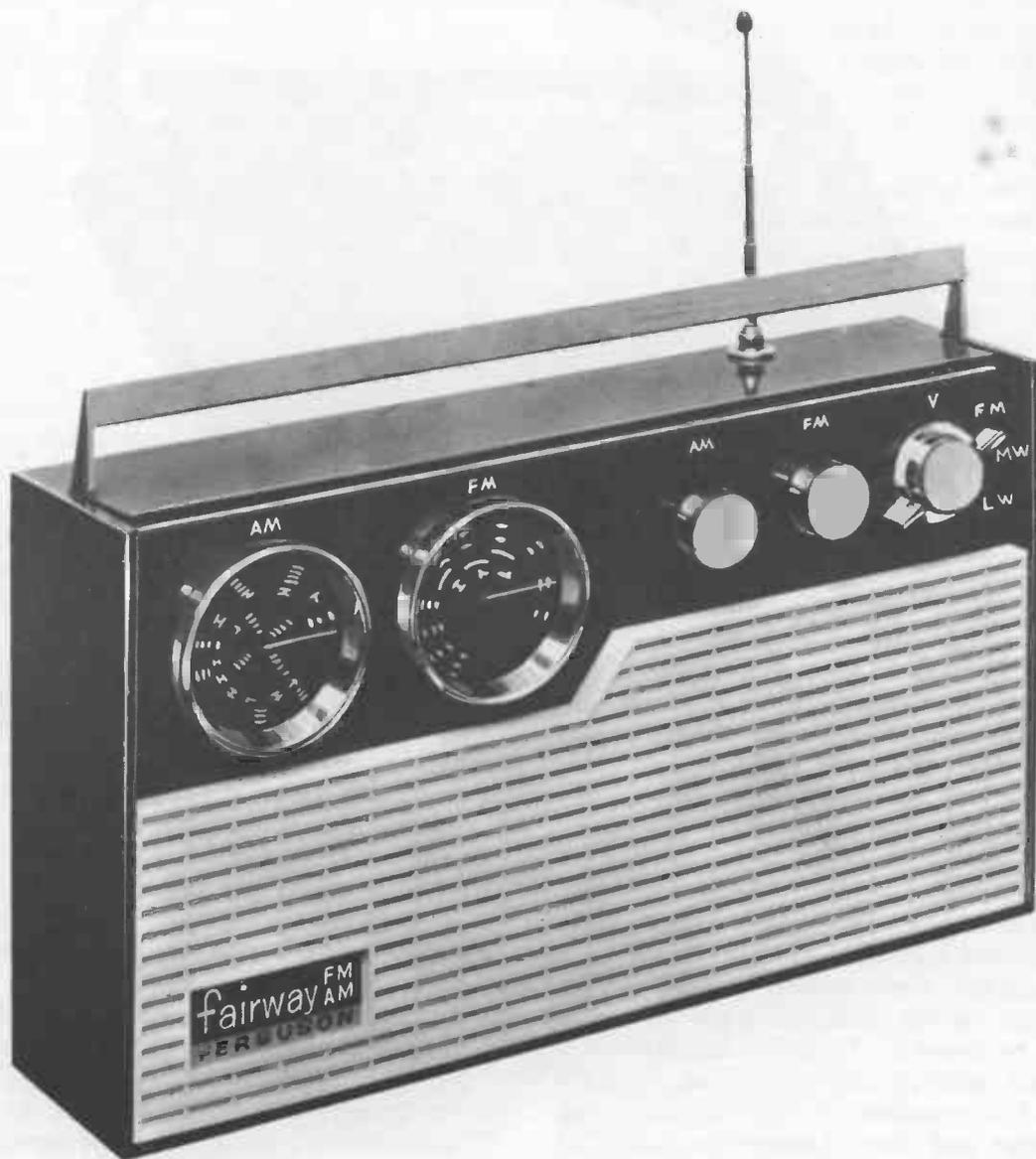
Fig. 20 The *Ferguson 3112* model—nine transistors, two germanium diodes and an impressive power output of 800 mW class B push-pull
