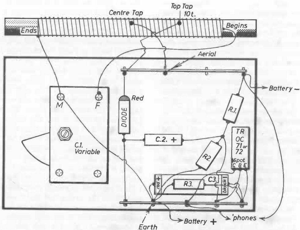
Fig. 5 Wiring diagram of the diode/transistor receiver
