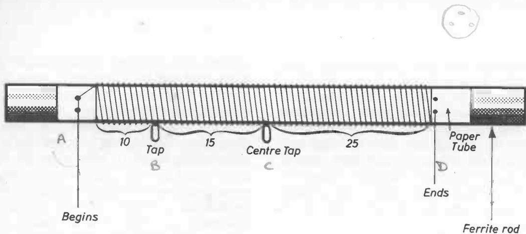
Fig. 4 The special coil for the receivers described in Chapters 3 and 4
