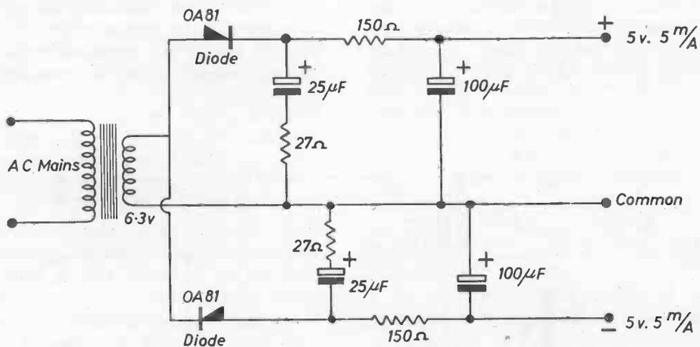
Fig. 24 An experimental mains supply unit
