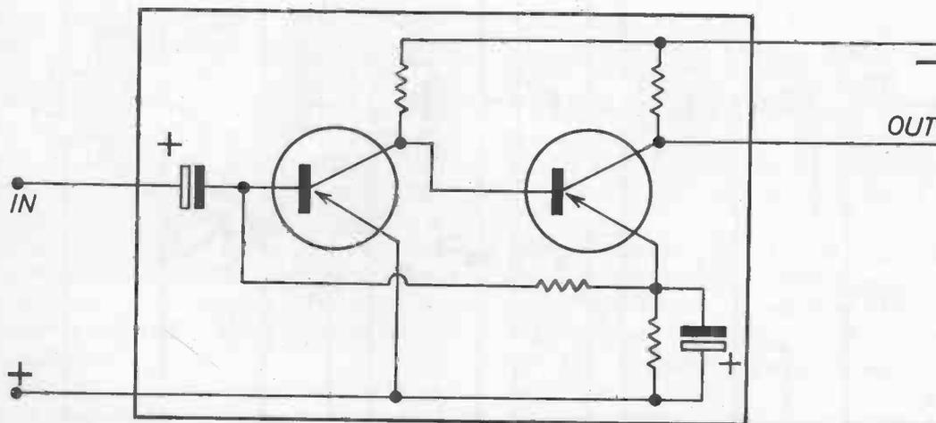
Fig. 13 Theoretical circuit of the *Sinclair Radionics* midget amplifier
