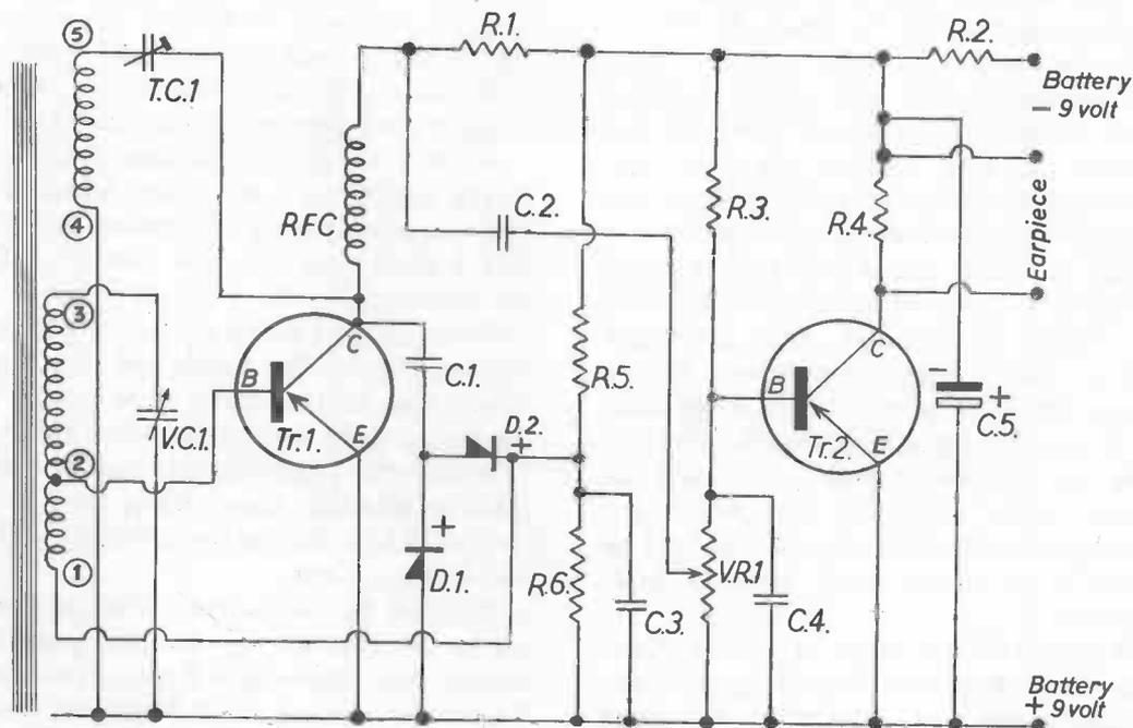
Fig. 6 Theoretical circuit of the two-transistor pocket receiver
