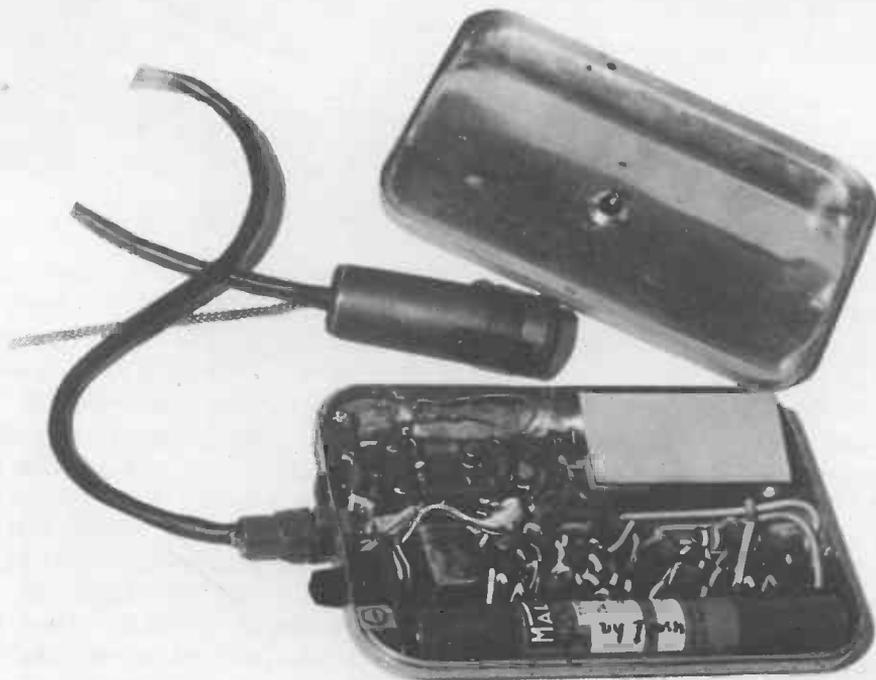
Fig. 27 BBC radio microphone using semi-conductors
