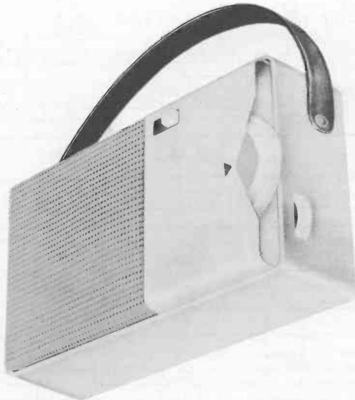
Fig. 12 The *Osmor* pocket transistor superhet receiver built into a neat plastic cabinet
