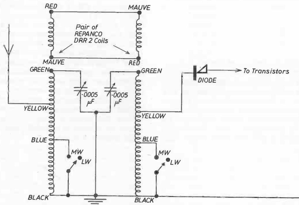
Fig. 8 Bandpass tuning arrangements of *Three-Dee* transistor receiver designed by Repanco
