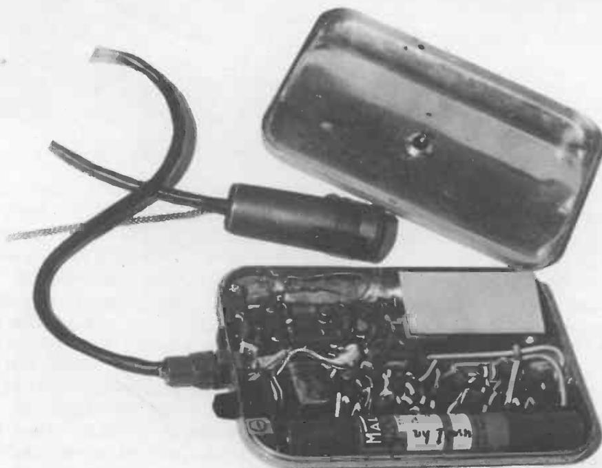
Fig. 27 BBC radio microphone using semi-conductors
