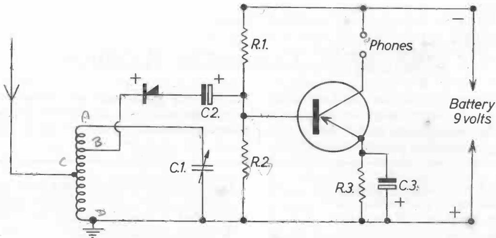
Fig. 3 Theoretical circuit of the diode/transistor receiver
