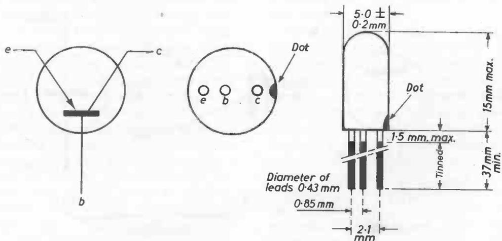
emitter goes to the positive side of the battery with the collector negative.
