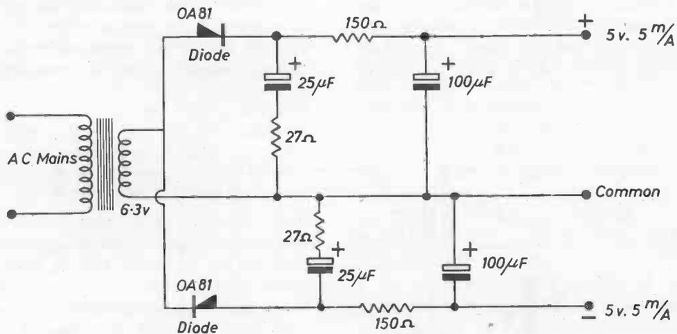
Fig. 24 An experimental mains supply unit
