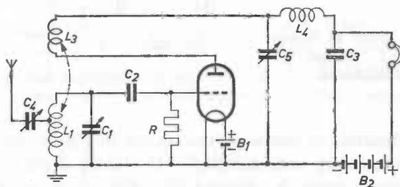
Fig. 11. The triode as detector with feedback by means of an extra coil. Adjustable with variable capacitor.  $L_4$  and  $C_3$  prevent r.f. voltages from reaching the headphones.
