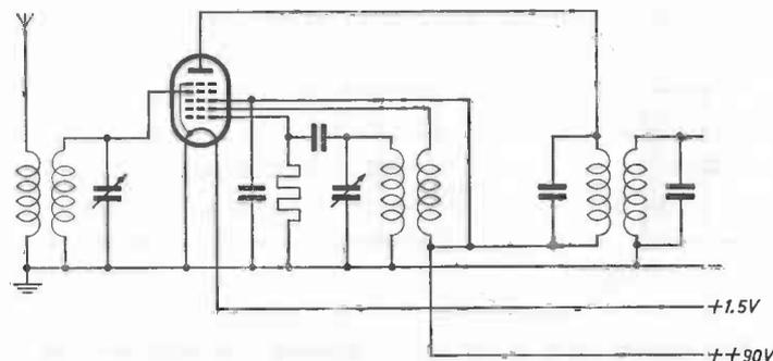
Fig. 23. In battery receivers, the mixer valve is usually a heptode in order to reduce the current consumption.
