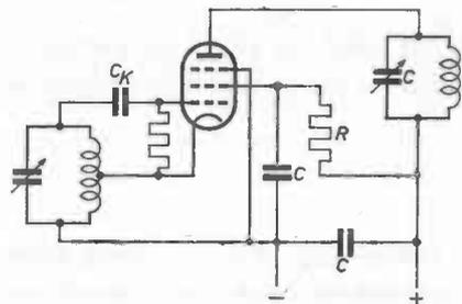
Fig. 42. Electron-coupled oscillator (ECO) with Hartley oscillator circuit.
