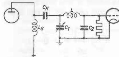
Fig. 58. Two transmitter stages coupled by means of a  $\pi$ -network.
