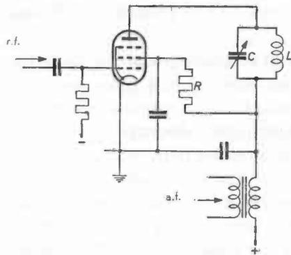
Fig. 76. Combined anode and screen-grid modulation. The correct screen-grid voltage is obtained by means of resistor  $R$ .
