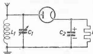
Fig. 5. Circuit diagram of a simple receiver.  $L_1$  and  $C_1$  form the tuning circuit. The detected voltages are produced across  $C_2$  and  $R$ .
