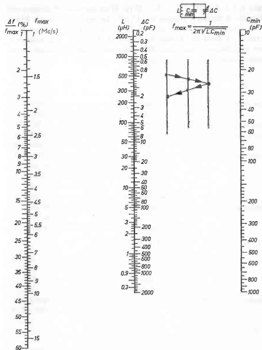
Fig. 125. Nomogram for bandsread calculations.
