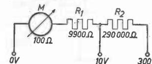
Fig. 107. Use of several resistors in series for various measuring ranges of the voltmeter.
