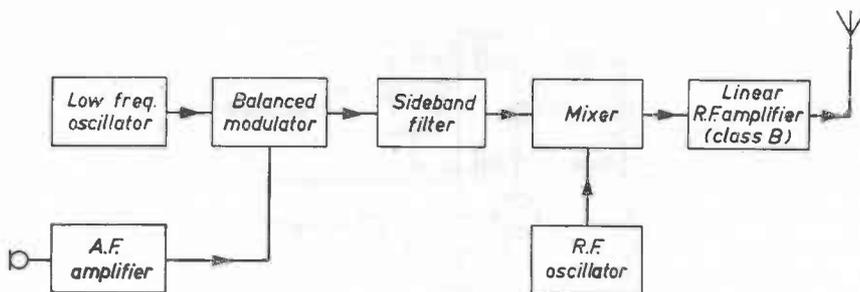
Fig. 87. Single-sideband modulation according to the "filter" system. The audio signal, together with an a.f. oscillator signal is fed into a balanced modulator, the carrier wave being suppressed. The sideband filter filters out one sideband. This is then transformed to the correct frequency.
