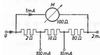
Fig. 110. Principle of the universal shunt.
