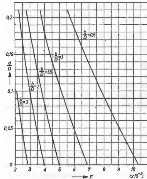
Fig. 127. Graph for determining the form factor  $F$  from  $\frac{d}{D}$  and  $\frac{b}{D}$
