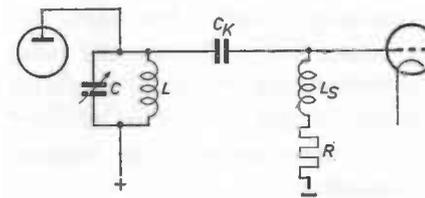
Fig. 55. Capacitive coupling between two transmitter stages.
