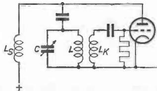
Fig. 39. Tuned anode circuit, parallel-fed via choke  $L_s$ .
