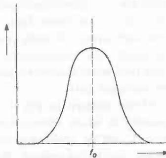
across the circuit (see Fig. 3). The voltages energised in the aerial are channelled off to earth more readily because of the lower impedance. For frequencies far removed from the tuning frequency the circuit behaves practically as a short-circuit. The more efficiently the voltages of the adjacent frequencies are attenuated, the better the "quality" of the circuit.
