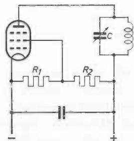
Fig. 65. Feeding the screen-grid by means of a potentiometer ("bleeder").
