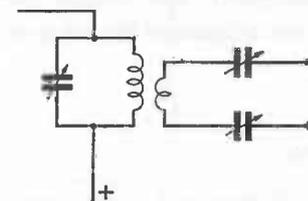
Fig. 99. Matching the feeders by means of series capacitors.
