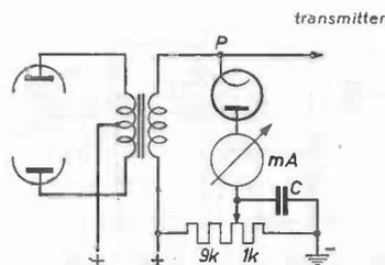
Fig. 81. Indication at modulation amplitudes of less than 100 %, in this figure 90 %. This is determined by the ratio of the bleeder resistors.
