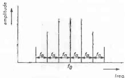
Fig. 71. Carrier wave  $f_0$  modulated with frequency  $f_m$ . Overmodulation occurred because the modulation amplitude is greater than 100 %.
