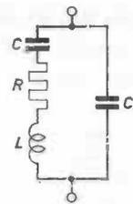
Fig. 46. Equivalent diagram of a quartz crystal.  $CRL$  represents the crystal,  $C_e$  the capacitance of the electrodes.
