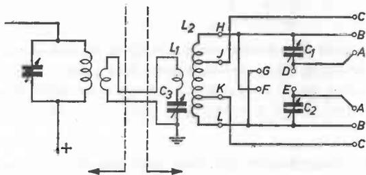
Fig. 100. Aerial coupling unit for matching to high and low-impedance.
