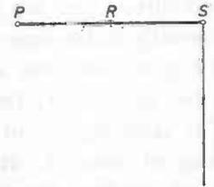
Fig. 93. Half-wave radiator, fed at one end (Zeppelin aerial).
