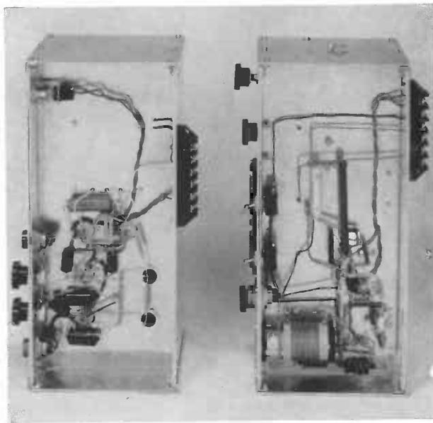
Photo 12. *Underneath view of the transmitter and modulator.* On the right the transmitter with the very robust oscillator coil visible at the bottom. To the right of this the trimmer of the permanently tuned 80-metre circuit. The wiring of the modulator (left) needs no further explanation.
