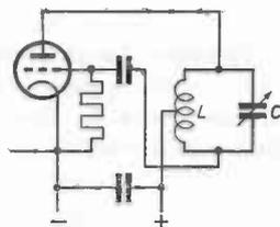
Fig. 40. Hartley oscillator, series-fed. Tapping on coil  $L$ .
