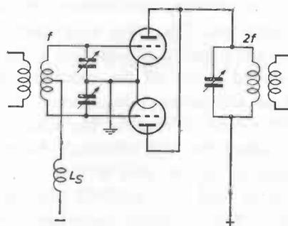
Fig. 54. "Push-push" amplifier specially suitable as "doubler".
