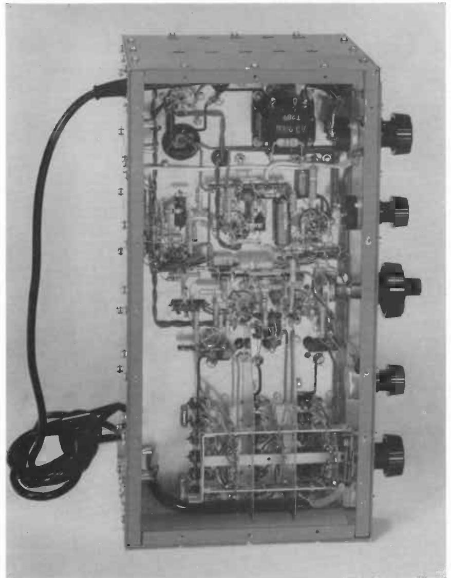
Photo 7. *Underneath view of short-wave superheterodyne receiver*. At the bottom the wave range switch with the two screens to separate the aerial circuit, the second tuned circuit and the oscillator circuit from each other. In the centre slightly to the left the screening over the valve holder of the i.f. valve. The loudspeaker transformer is at the top.
