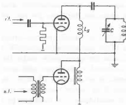
Fig. 72. Principle of Heising modulation, i.e. a form of anode modulation employing a choke.
