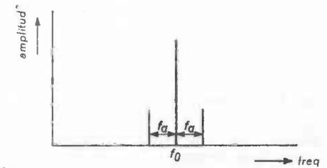
Fig. 70. Carrier wave  $f_0$  modulated with a frequency  $f_a$ . Modulation amplitude and approx. 30 %.
