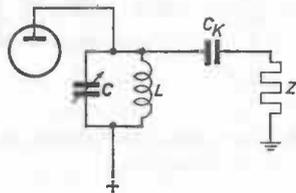
Fig. 61. High impedance matching between aerial and output stage.
