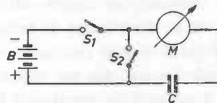
Fig. 2. If  $S_1$  is closed,  $M$  deflects momentarily and then returns to zero. If  $S_1$  is subsequently opened and  $S_2$  closed,  $M$  deflects in the other direction.
