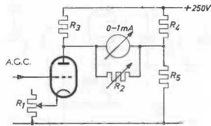
Fig. 32. Signal-strength meter with compensation circuit.
