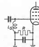
Fig. 66. Negative bias obtained from a separate supply source.
