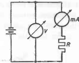
Fig. 114. Resistance measurement by means of ammeter and voltmeter. The voltmeter also indicates the voltage drop across the milliammeter.
