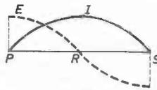
Fig. 92. Half-wave radiator ( $\lambda/2$ ) in contrast with the radiator in Fig. 91 which is equal to a complete wavelength ( $\lambda$ ).
