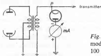
Fig. 80. Overmodulation indication for amplitude modulation systems with transformer. Indication at 100 % modulation.
