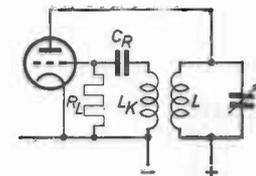
Fig. 37. Negative bias obtained by means of grid capacitor  $C_R$  and grid-leak resistor  $R_L$ . Tuned series-fed anode circuit.
