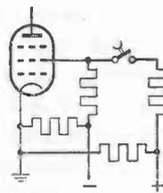
Fig. 67. Keying the screen-grid circuit with negative bias.
