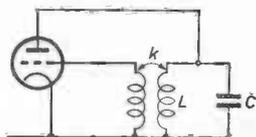
Fig. 36. Principle of oscillator circuit.
