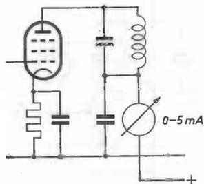
Fig. 31. Simple signal-strength meter.
