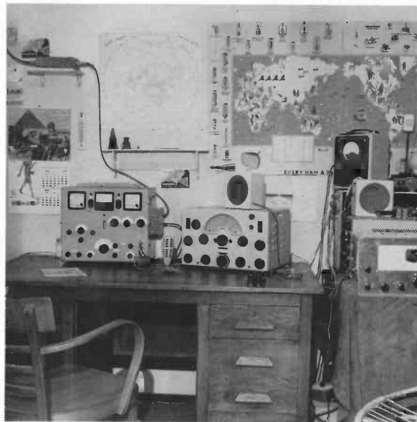
Photo 1. Shack belonging to PA0IB. The transmitter (left) and the receiver (right) are placed in convenient positions, plenty of space having been left for the morse key, microphone, log and other necessary attributes. On the right-hand side there is room for measuring instruments and for equipment which is being built. The aerial filter is seen in the left-hand top corner.
