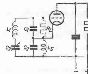
Fig. 43. Clapp oscillator.
