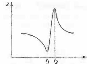
Fig. 47. Impedance curve of a quartz crystal. Series resonance at frequency  $f_1$ ; parallel resonance at frequency  $f_2$ .
