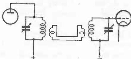
Fig. 57. Low-impedance coupling (link-coupling).
