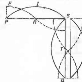
Fig. 95. Zeppelin aerial with distribution of current (*I*) and voltage (*E*) along radiator and feeders.
