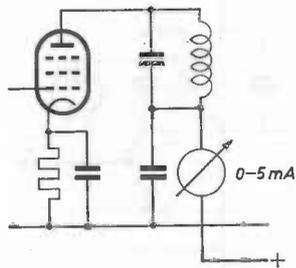
Fig. 31. Simple signal-strength meter.
