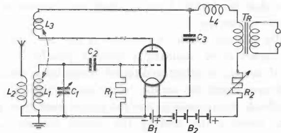
Fig. 12. Variable feedback by means of a variable series resistor. Headphones matched by means of a transformer.
