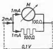
Fig. 109. Use of a parallel resistor (shunt) to extend the measuring range as ammeter.
