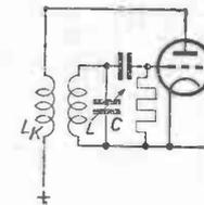
Fig. 38. Tuned grid circuit.
