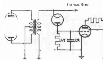
Fig. 82. Indication by means of a "magic eye".
