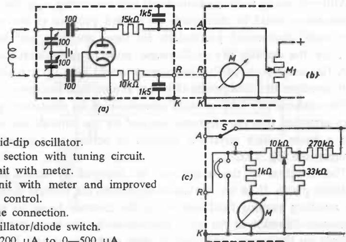
Fig. 120. Grid-dip oscillator.
