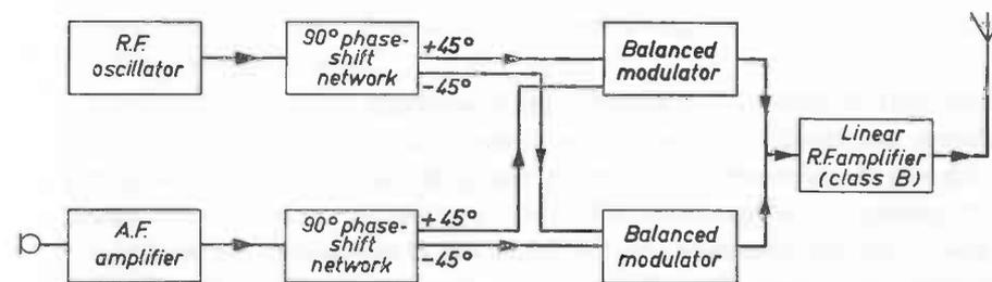
Fig. 88. Single-sideband modulation according to the phase-displacement system. By means of 90° phase-shift networks, the phases of both the carrier wave and the modulation are changed 90°. In the balanced modulators in which the carrier is suppressed again, the signals are combined in such a way that one sideband is suppressed.
