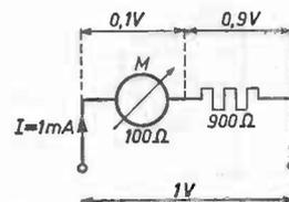
Fig. 106. Use of a series resistor to extend the measuring range of a voltmeter.
