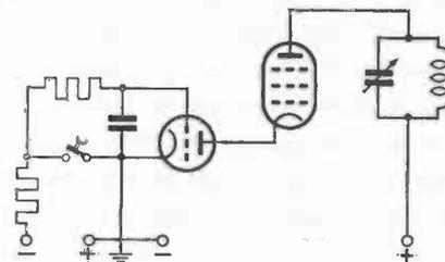
Fig. 68. Extra "keying" valve operates as electronic relay and cuts off the transmitter valve when the key is up.
