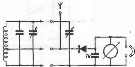
Fig. 119. Absorption meter, also field strength meter and modulation monitor. Coils have their own parallel capacitances for bandspread.
