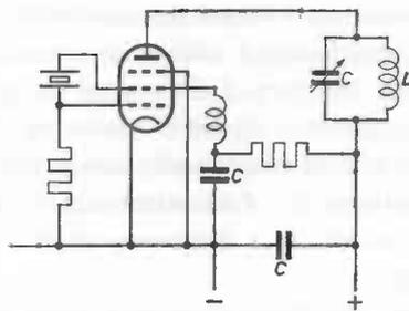
Fig. 51. Improved Pierce oscillator, consisting in fact of an ECO with a crystal oscillator and combining the advantages of both these circuits.
