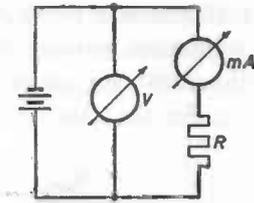
Fig. 114. Resistance measurement by means of ammeter and voltmeter. The voltmeter also indicates the voltage drop across the milliammeter.
