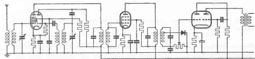
Fig. 21. Circuit diagram of a simple superheterodyne receiver employing three valves: a triode-heptode as mixer, a pentode as i.f. amplifier and a double-triode as two-stage audio amplifier. A germanium diode is used as detector.
