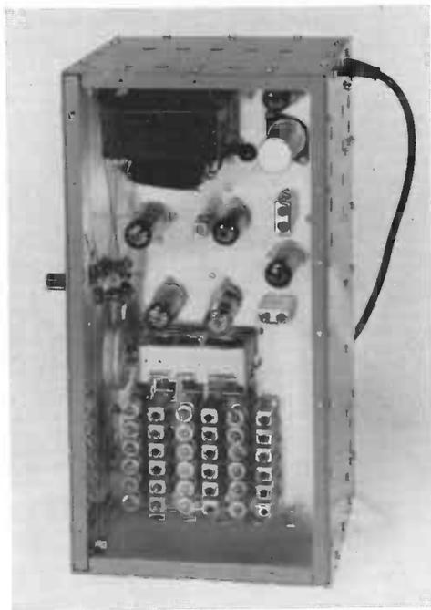
Photo 6. *Top view of short-wave superheterodyne receiver*. The set of coils is seen at the bottom. For each of the 6 ranges the aerial coil, second tuned circuit coil and oscillator coil (from left to right), each accompanied by a trimmer, are seen clearly. Above them are the triple variable capacitor with special oscillator section (right), the two i.f. transformers and the beat coil. The mains transformer is at the top.
