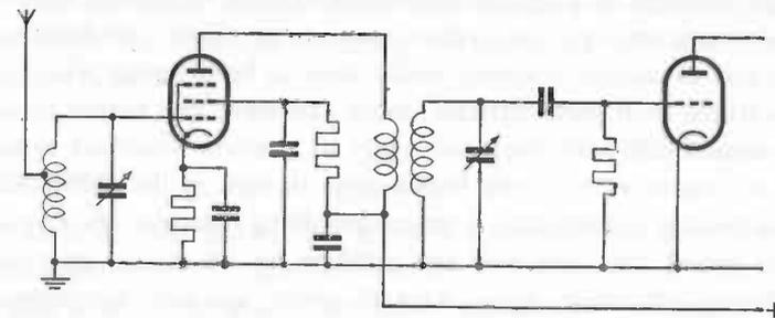
Fig. 18. The detector tuning circuit is earthed. The signal is received from the r.f. stage via a coupling coil.
