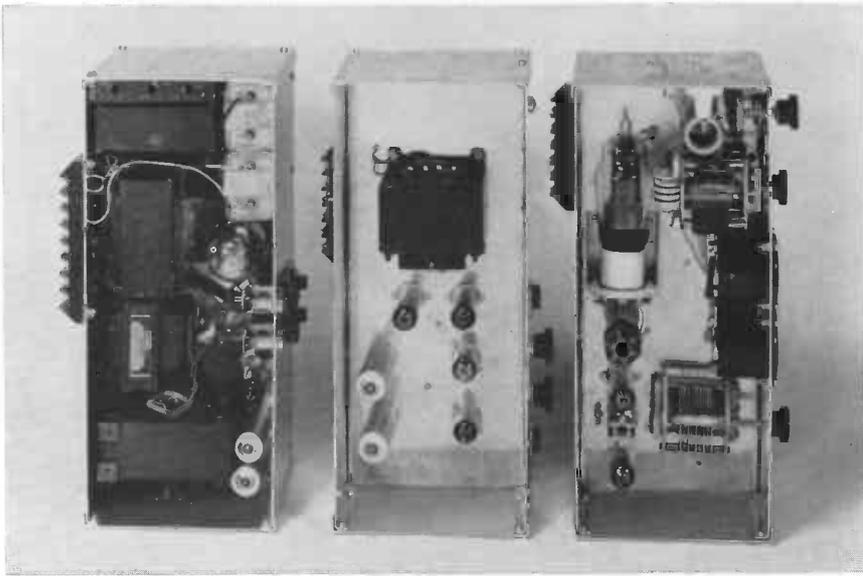
Photo 11. *Top view of the three sections.* On the left the supply unit with transformers, chokes, capacitors and rectifiers. In the centre the modulator with modulation transformer. On the right the transmitter with the variable capacitor of the oscillator at the bottom, the buffer stages beyond this and, right at the top, the output stage.
