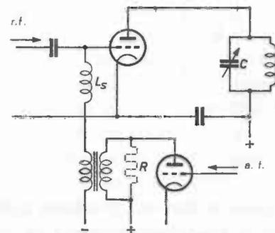
Fig. 74. Control-grid modulation. Transformer coupling.
