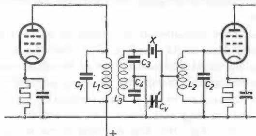
Fig. 27. I.F. band-pass filter with crystal filter for improved selectivity.
