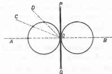
Fig. 101. Radiation pattern of half-wave aerial ( $l = \lambda/2$ ).
