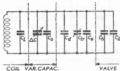
Fig. 34. Capacitances occurring in a tuning circuit.
