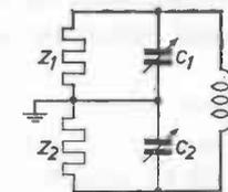
Fig. 59. Equivalent circuit diagram of the  $\pi$ -network;
