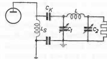
Fig. 62.  $\pi$ -network as coupling element between output stage and aerial.
