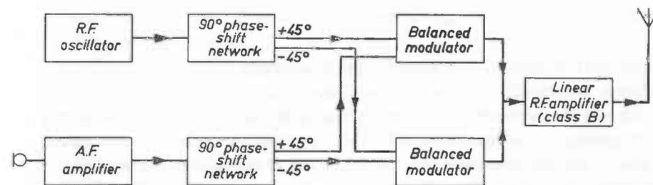
Fig. 88. Single-sideband modulation according to the phase-displacement system. By means of  $90^\circ$  phase-shift networks, the phases of both the carrier wave and the modulation are changed  $90^\circ$ . In the balanced modulators in which the carrier is suppressed again, the signals are combined in such a way that one sideband is suppressed.
