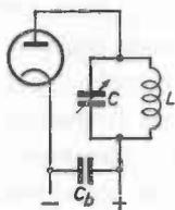
Fig. 64. Series-fed anode voltage of transmitter valve.
