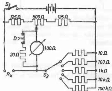
Fig. 116. Practical example of a Wheatstone bridge for resistance measurement. Switch  $S_2$  selects the measuring range. The sensitive meter position is obtained by means of push button  $D$ .
