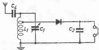
Fig. 9. Valve diode replaced by germanium diode. The diode is matched by means of a tapping on the coil. For practical data, see text.
