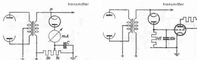
Fig. 81. Indication at modulation amplitudes of less than 100 %, in this figure 90 %. This is determined by the ratio of the bleeder resistors.
