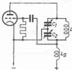
Fig. 41. Colpitts oscillator, series-fed. Tapping on junction between the two capacitors  $C_1$  and  $C_2$ .
