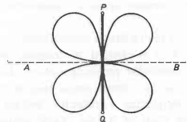
Fig. 102. Radiation pattern of full-wave aerial ( $l = \lambda$ ).
