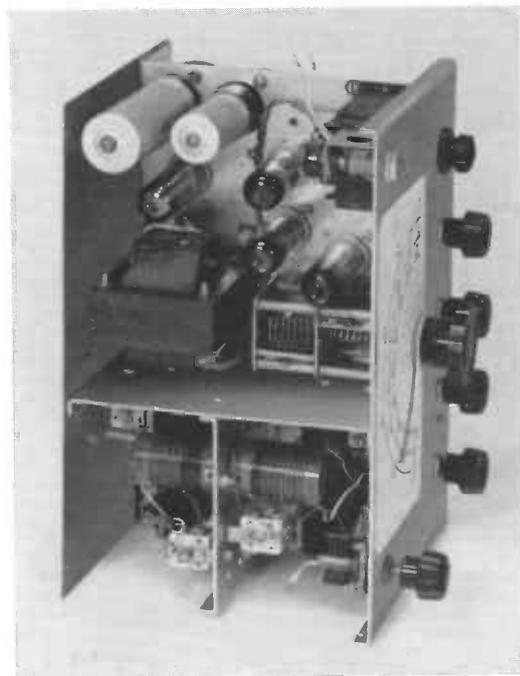
Photo 3. *Top view of straight receiver.* The two coil compartments are seen at the bottom of the photograph (detector on the left, aerial on the right). Each compartment contains three coils, one for each band, which are mounted perpendicularly to each other. Behind the twin capacitor is the mains transformer; the loudspeaker transformer is seen on the top r.h. side.
