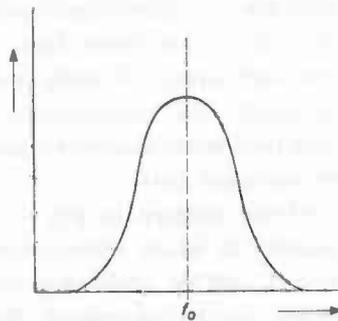
Fig. 3. The voltages across the tuning circuit are smaller according as the difference between the frequency and the tuning frequency  $f_0$  is greater.
