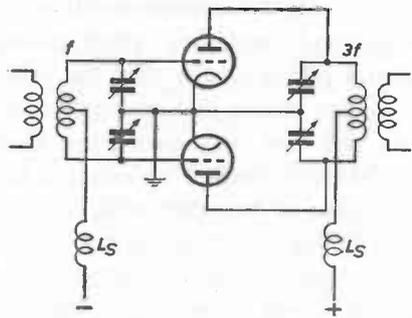
Fig. 53. "Push-pull" amplifier suitable as "trebler".
