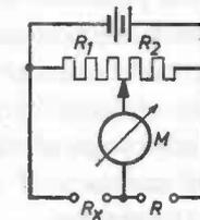
Fig. 115. Resistance measurement by means of the Wheatstone bridge. The resistor  $R_x$  to be measured is compared with a known resistance  $R$ .
