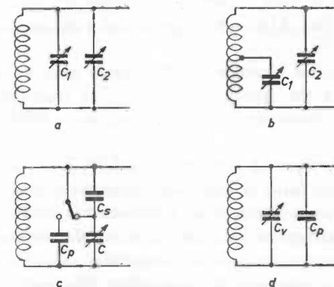
Fig. 35. Methods of bandsread.
