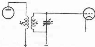
Fig. 56. Inductive coupling between two transmitter stages.
