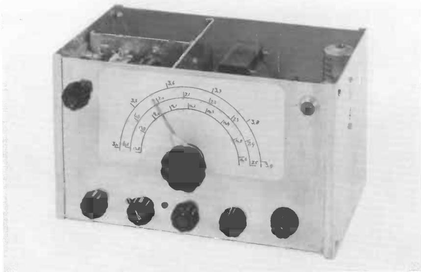
Photo 2. *The straight receiver* (described in Chapter 10). In the centre the large dial with the three ranges. The 5 knobs at the bottom are (from left to right): r.f. gain control, wave switch, feedback control, a.f. gain control + mains switch, fuse holder. The aerial capacitor is on the top l.h. side and the signal lamp on the top r.h. side.
