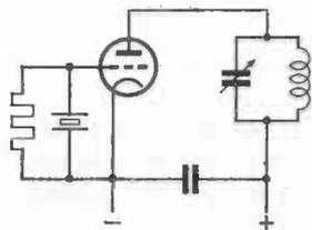
Fig. 48. Simple quartz crystal oscillator.
