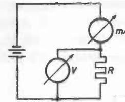
Fig. 113. Resistance measurement by means of ammeter and voltmeter. The milliammeter also indicates the current through the voltmeter.
