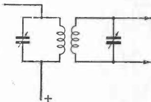
Fig. 97. Matching to feeders with high input impedance.
