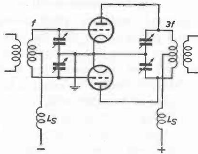
Fig. 53. "Push-pull" amplifier suitable as "trebler".
