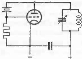
Fig. 50. Pierce oscillator with tuning circuit to increase the delivered r.f. voltage.
