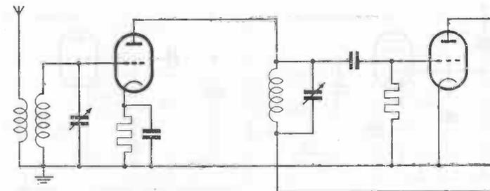
Fig. 16. Triode as r.f. amplifier with by-passed cathode resistor for correct adjustment of the negative bias. The heaters of the indirectly heated valves have been omitted in this and the next figures for the sake of simplicity.
