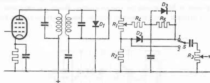
Fig. 33. Circuit diagram of interference limiter. Diode  $D_2$  is the limiter and diode  $D_3$  gives improved action. The limiter is disconnected in position 2 of switch  $S$ .
