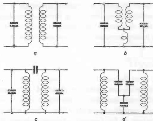
Fig. 4. Coupling methods with band-pass filters
