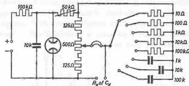
Fig. 117. Wheatstone bridge with a.c. voltage source, suitable for resistance and capacitance measurement. Headphones as indicator.
