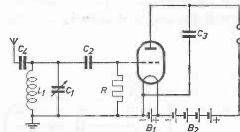
Fig. 10. The triode as detector.  $C_3$  prevents r.f. voltages from reaching the headphones.
