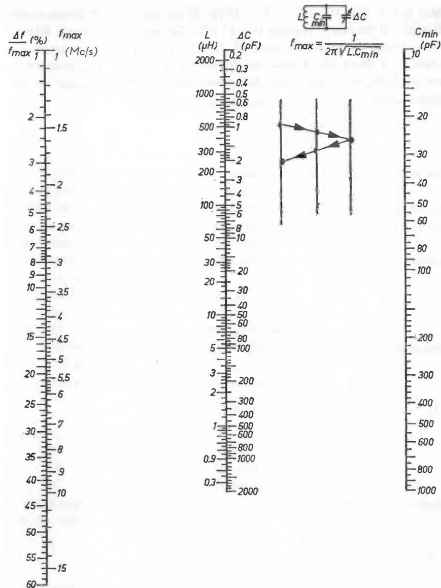
Fig. 125. Nomogram for bandsread calculations.
