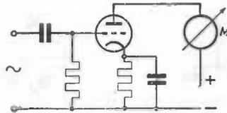
Fig. 112. Valve detector for the measurement of alternating voltages (valve voltmeter).
