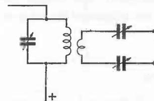
Fig. 99. Matching the feeders by means of series capacitors.
