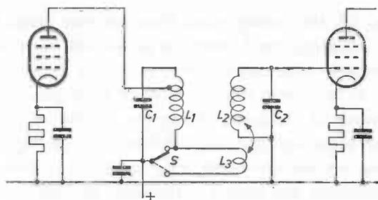
Fig. 26. Variable bandwidth with the aid of an extra coupling coil. (e.g. graphs I and II, Fig. 25).
