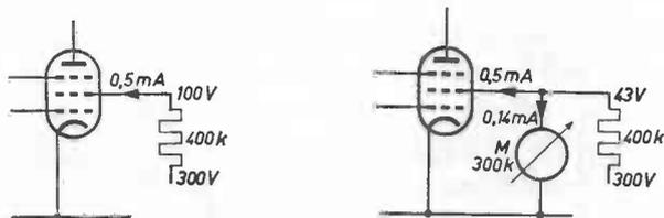
Fig. 108. Effect of a voltmeter on the actual voltage on the screen-grid of a valve during measurement.
