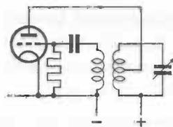
Fig. 45. Anode connected to tapping on tuning circuit to reduce the effect of valve capacitance.
