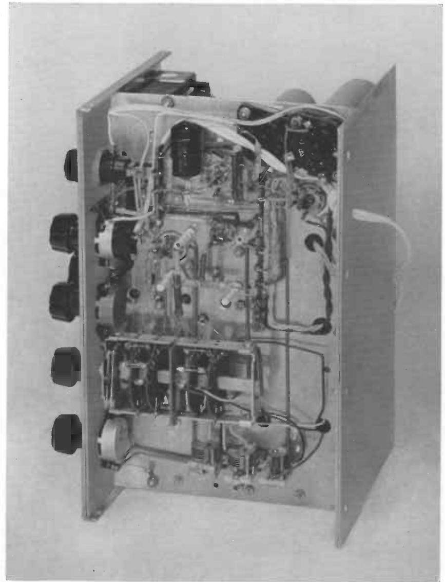
Photo 4. *Underneath view of straight receiver.* The wave-switch has four sections with a screen in the centre. This is in line with the screening on the top of the chassis between the aerial and detector circuits. The three trimmers for adjusting the feedback are seen at the bottom.
