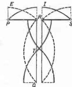
Fig. 96. Dipole with distribution of current and voltage along radiator and feeders.
