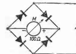
Fig. 111. Graetz-circuit for rectifying the alternating voltage to be measured by means of a d.c. meter.
