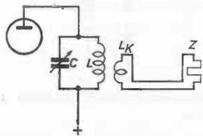
Fig. 60. High impedance matching between aerial and output stage.
