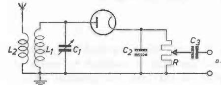
Fig. 7. Receiver with inductive aerial coupling. A potentiometer is chosen for  $R$  and  $C_3$  acts as separating capacitor.
