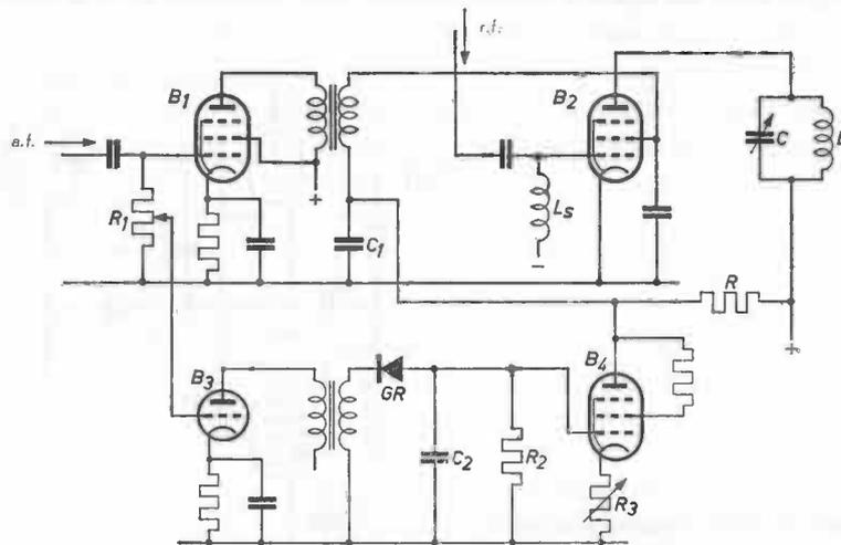
One method of indicating overmodulation in amplitude-modulation circuits is shown in Fig. 80. Across the secondary winding of the modulation transformer a rectifier valve in series with a milliammeter is connected to earth. If overmodulation occurs the audio frequency voltage in the
