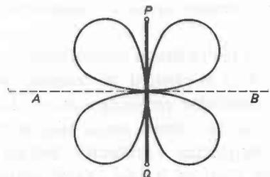
Fig. 102. Radiation pattern of full-wave aerial ( $l = \lambda$ ).
