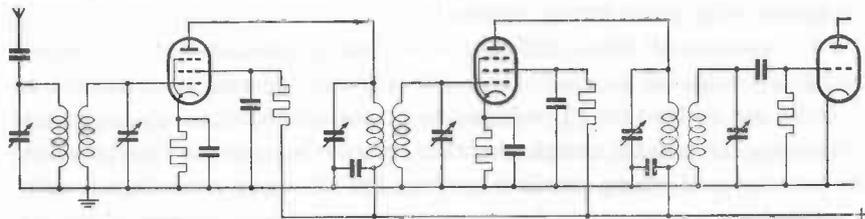
Fig. 19. Example of two stages of r.f. amplification, employing band-pass filters
