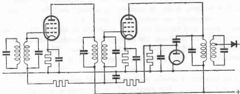
Fig. 29. I.F. amplifier with automatic gain control (a.g.c.).
