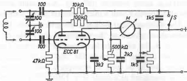
Fig. 121. Grid-dip oscillator with amplifier.
