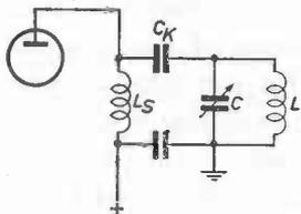
Fig. 63. Parallel-fed anode voltage of transmitter valve.
