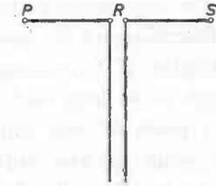
Fig. 94. Half-wave radiator, fed in the centre (dipole or Herz aerial).
