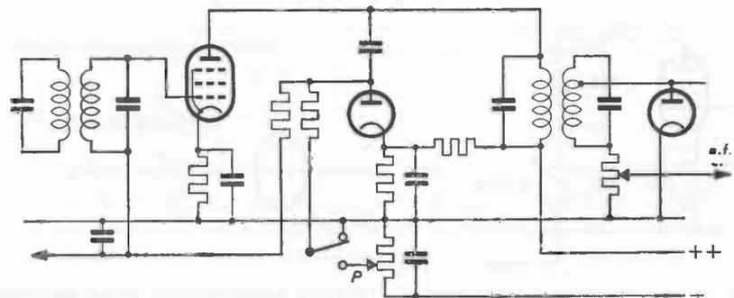
Fig. 30. Combined a.g.c. and manual control.
