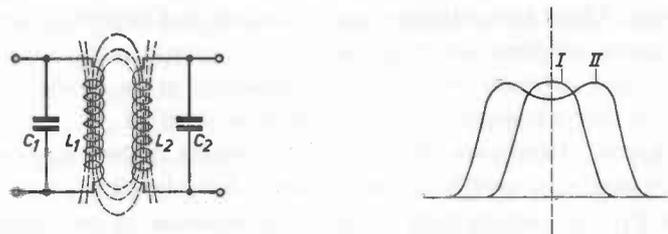
Fig. 25. Two circuits tuned to the same frequency. Coupling greater than "critical".
