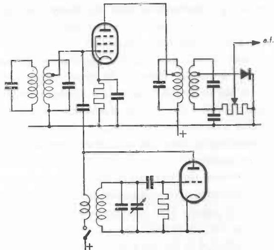
Fig. 28. I.F. amplifier with "beat-oscillator" for telegraphy reception.
