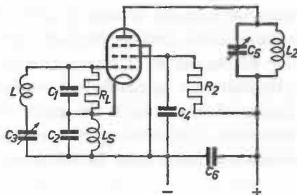
Fig. 44. Electron-coupled oscillator with Clapp oscillator circuit.
