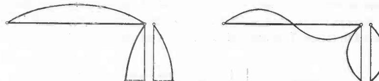
Fig. 98. Zeppelin aerial (Zepp) with radiator ( $\lambda/2$ ) on 80 metres and feeders ( $\lambda/4$ ).
