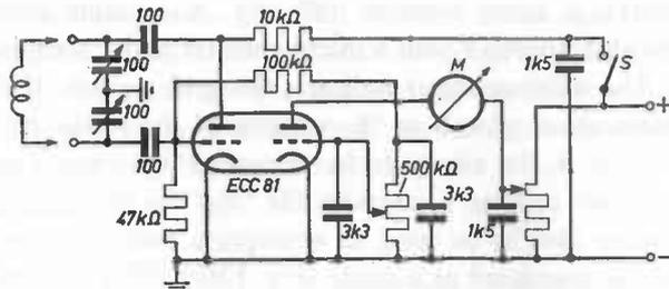
Fig. 121. Grid-dip oscillator with amplifier.
