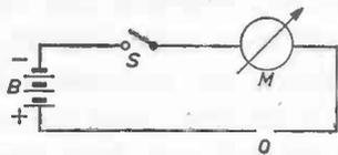
Fig. 1. If  $S$  is closed, no current flows, because the circuit is interrupted at  $O$ .
