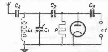
Fig. 8. Receiver with capacitance aerial coupling. Diode with earthed cathode. (Parallel detection).
