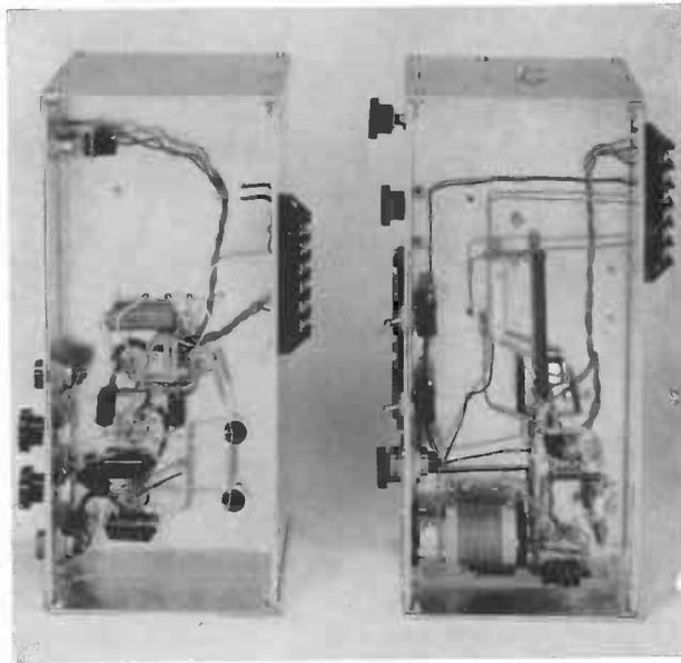
Photo 12. *Underneath view of the transmitter and modulator.* On the right the transmitter with the very robust oscillator coil visible at the bottom. To the right of this the trimmer of the permanently tuned 80-metre circuit. The wiring of the modulator (left) needs no further explanation.
