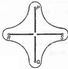
Fig. 103. Turnstile aerial is "omnidirectional".
