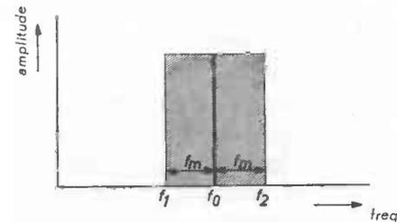
Fig. 69. Graphical representation of a carrier wave  $f_0$  with side frequencies  $f_1$  and  $f_2$ .
