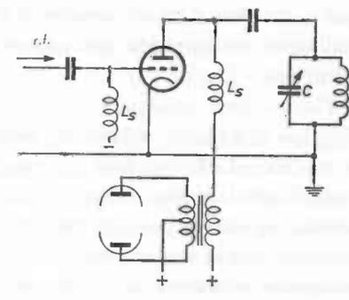
Fig. 73. Anode modulation with transformer coupling between transmitter and modulator.
