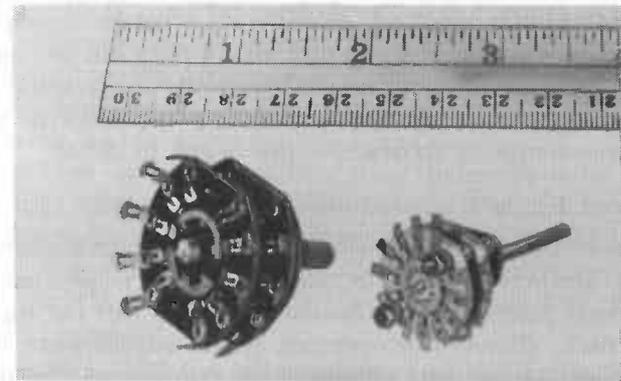
Fig. 206. Standard and miniature multiposition rotary switches. Rule scale indicates size.
