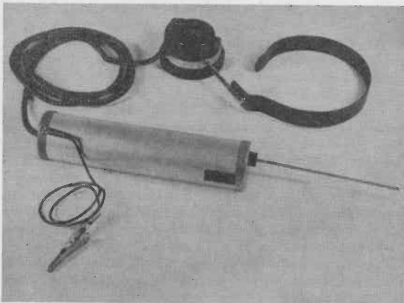
Fig. 9-28.—Author's model of the Signal Tracer. Courtesy Radio & Television News
