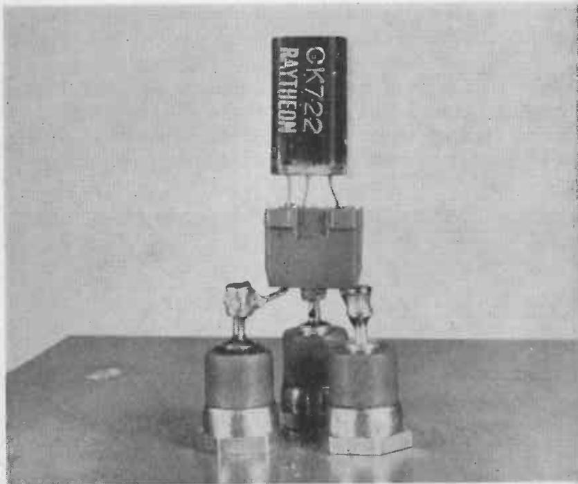
Fig. 2-5.—Detail of transistor socket mounting.
