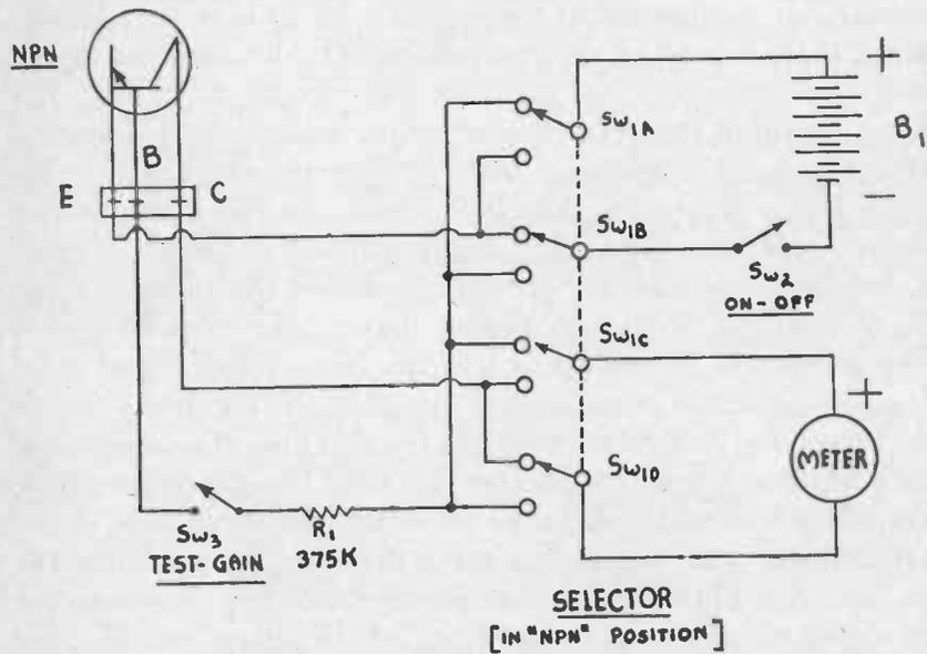
Fig. 9-18.—Circuit for a simple Transistor Checker. Courtesy Lafayette Radio
