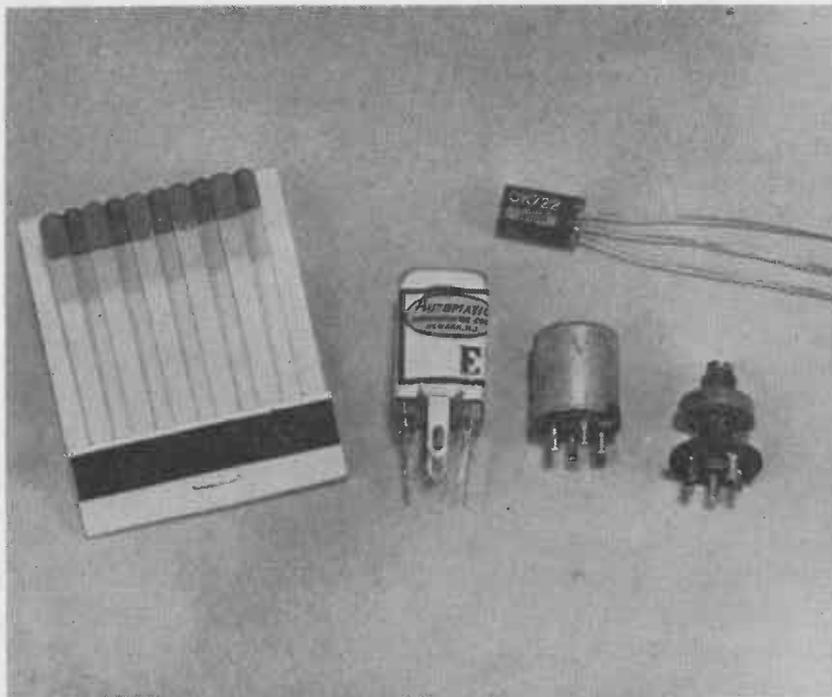
Fig. 3-3.—Subminiature R.F. coils and I.F. transformers.
