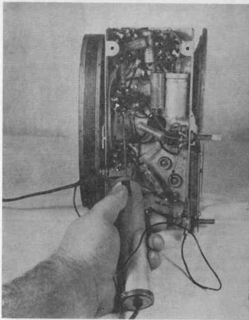
Fig. 9-29.—Using the Signal Tracer to service a broadcast receiver.
