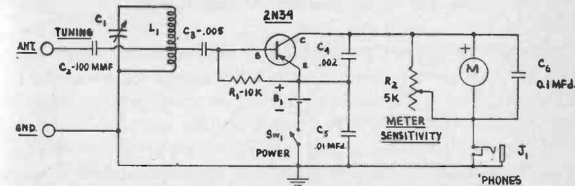
Fig. 8-22.—Circuit for a transistorized R.F. Frequency Meter.
