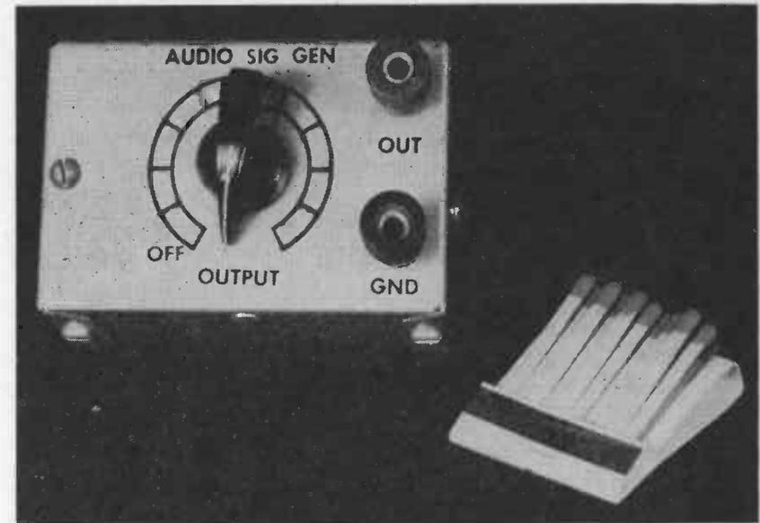
Fig. 9-2.—Exterior view of the Audio Sine Wave Generator—book matches show size.
