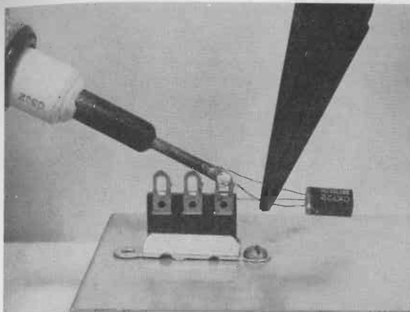
Fig. 2-9.—Proper use of a heat sink in soldering a transistor lead.
