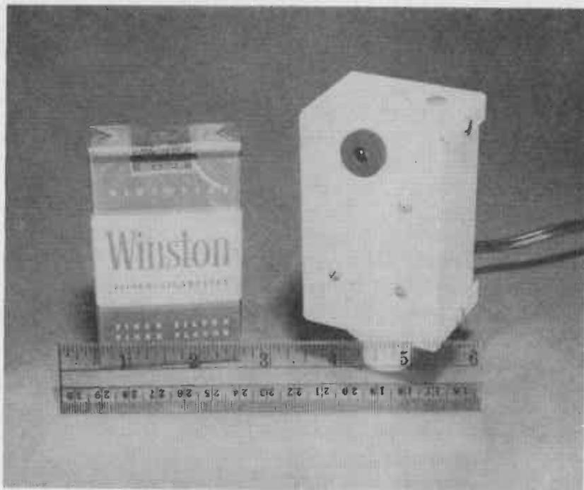
Fig. 10-22.—Author's model of the CdS Photocell Relay.
