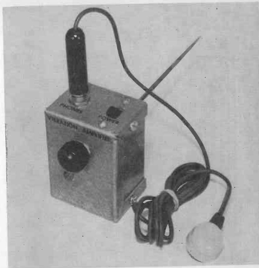
Fig. 7-6.—Exterior view of the electronic "Stethoscope".
