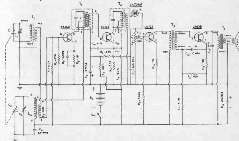
Fig. 8-11.—Schematic diagram of a four-transistor Superheterodyne Receiver.
