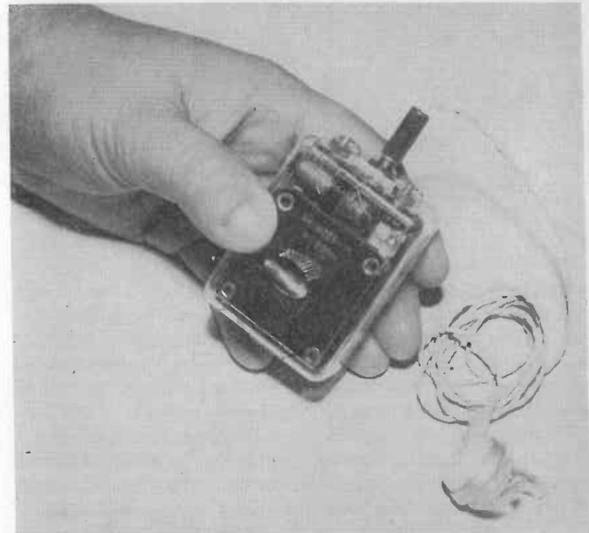
Fig. 8-6.—Exterior view of the Pocket Receiver . . . assembled in a small plastic box!
