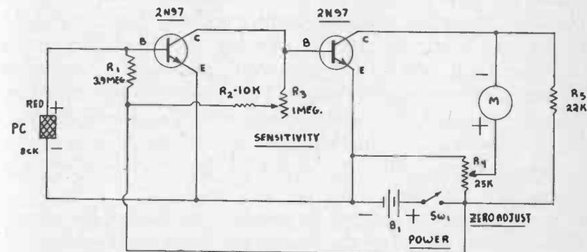
Fig. 9-25.—A very Sensitive *Light Meter* circuit featuring a cascaded complementary amplifier.
