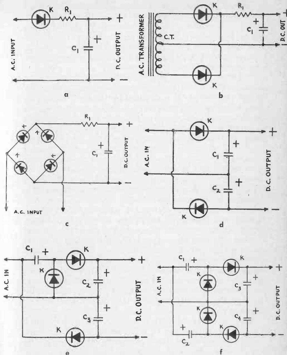
Fig. 10-20.—Basic semiconductor diode Rectifier circuits: (a) Half-Wave; (b) Full-Wave; (c) Full-Wave Bridge; (d) Voltage-Doubler; (e) Voltage-Tripler; (f) Voltage-Quadriplier.
