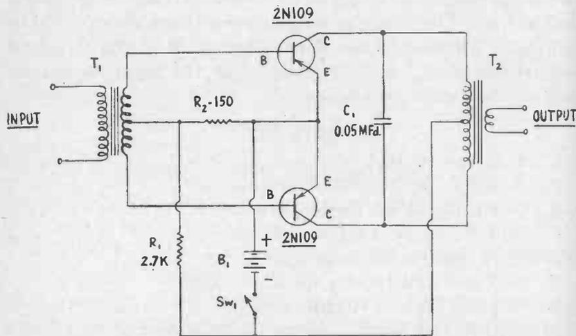
Fig. 7-2.—Basic Push-Pull Power Amplifier.
