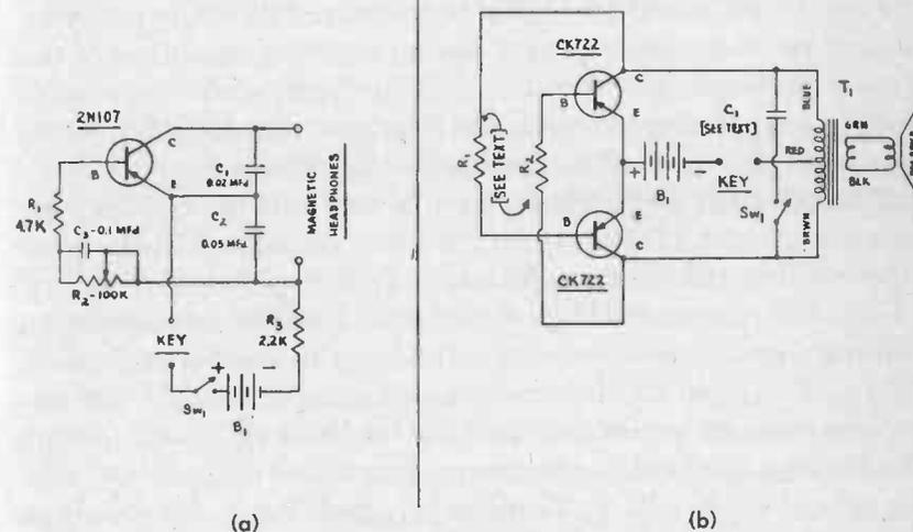
Fig. 10-12.—Diagrams for two easily built Code Practice Oscillators—(a) Headphone type; (b) Loudspeaker type.
