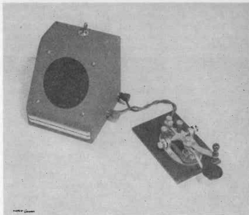
Fig. 10-14.—Loudspeaker type Code Practice Oscillator.
