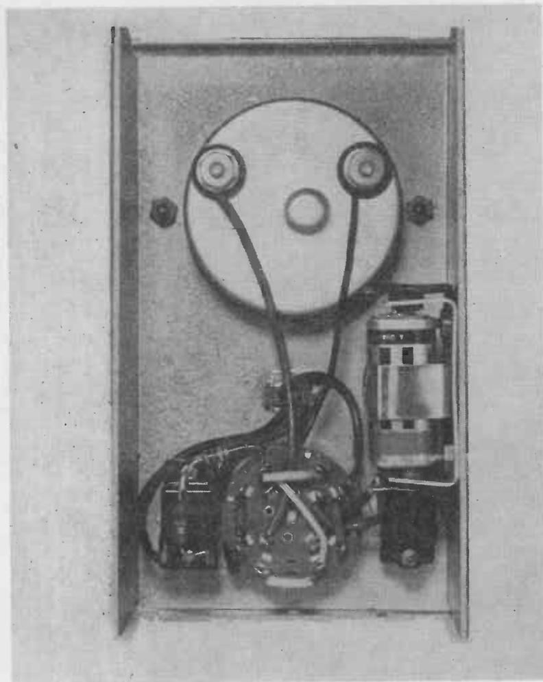
Fig. 9-20.—Interior view of the Transistor Checker.
