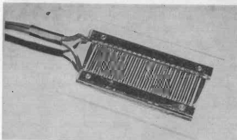
Fig. 10-5.—Sensor Plate used with the Rain Alarm.
