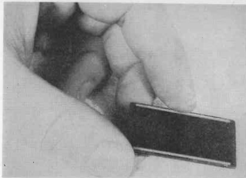
Fig. 10-28.—A single selenium Photocell.
