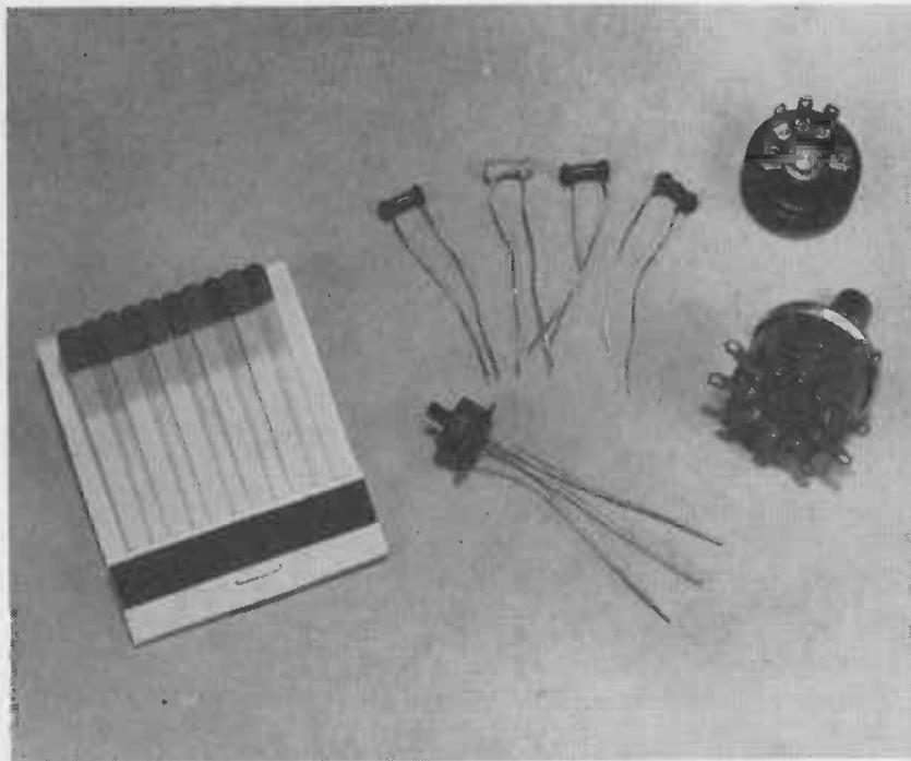
Fig. 3-1.—Subminiature resistors, volume control, and selector switch. Transistor and bookmatches included for size comparison.
