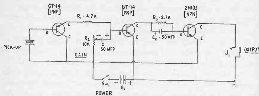
Fig. 7-5.—A transistorized electronic "Stethoscope".
