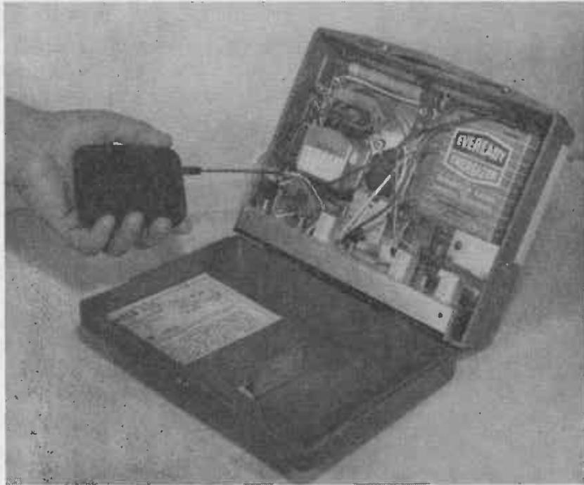
Fig. 9-9.—Using The Signal Squirrel to service a transistorized receiver.
