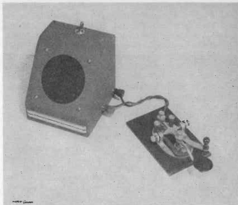
Fig. 10-14.—Loudspeaker type Code Practice Oscillator.
