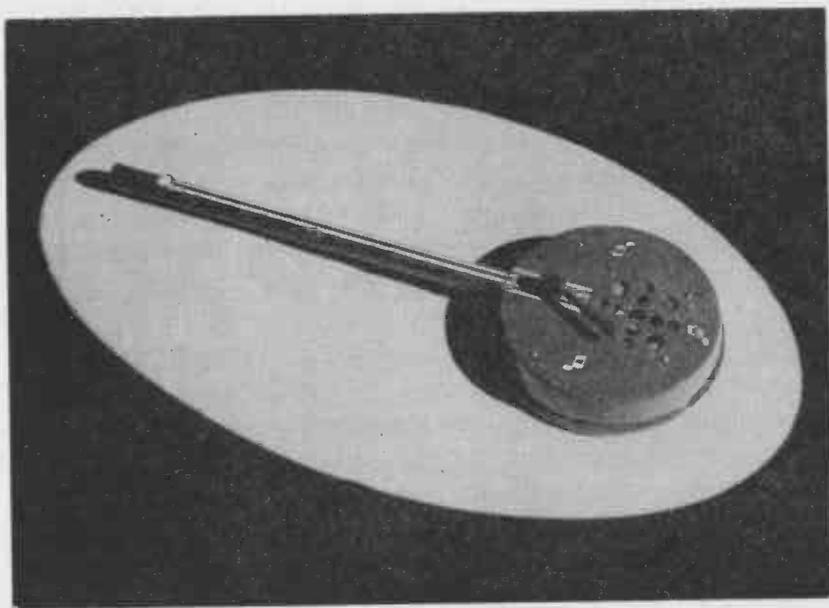
Fig. 10-19.—Author's model of a transistorized electronic "Banjo".
