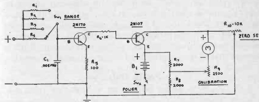
Fig. 9-22.—Schematic of a high impedance transistorized D.C. Voltmeter.
