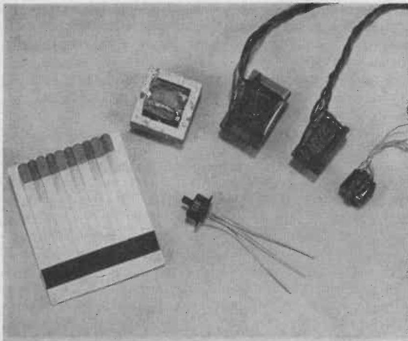
Fig. 3-4.—Subminiature iron-core audio transformers and choke.
