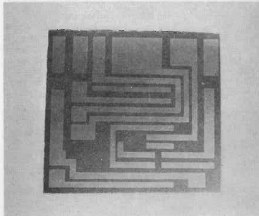
Fig. 13-5.—A typical etched circuit board.
