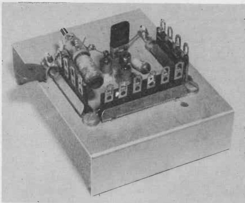
Fig. 8-25.—Breadboarded Frequency Doubler.
