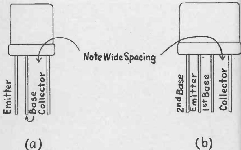
Fig. 2-7.—Pin connections for standard triode (a) and tetraode junction (b) transistors.
