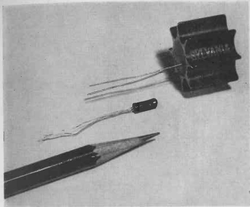
Fig. 1-2.—A TRANSISTRON hearing aid type transistor compared to a SYLVANIA power transistor to show relative sizes. Pencil gives an idea of true size.
