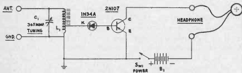
Fig. 8-1.—Simple transistorized Receiver using a diode detector.
