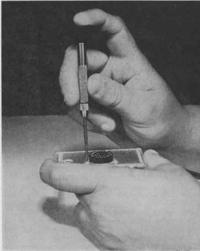
Fig. 2-2.—Proper technique for using a jeweler's screwdriver.
