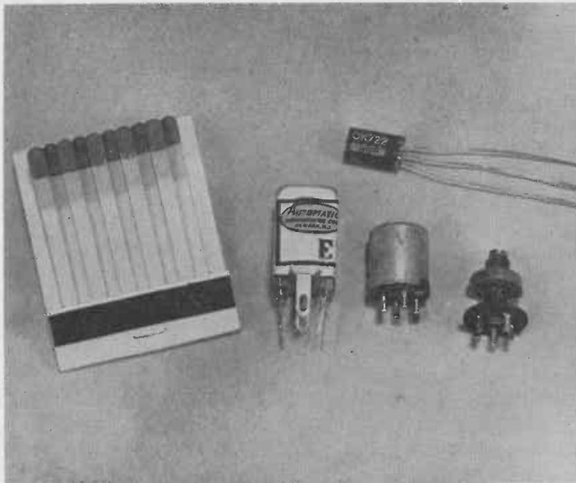
Fig. 3-3.—Subminiature R.F. coils and I.F. transformers.
