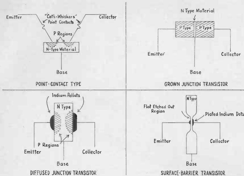
Fig. 1-3.—The four types of transistor construction are shown schematically in this sketch.
