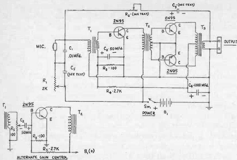
Fig. 7-19.—A transistorized P.A. System.
