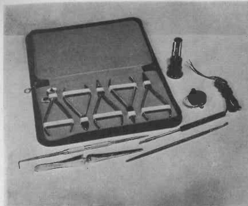
Fig. 2-1.—Hand tools useful when working with transistor circuits.
