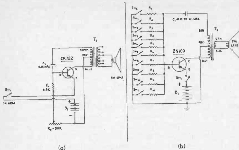
Fig. 10-18.—Two transistorized Musical Toys—(a) an electronic "Banjo"; (b) an electronic "Organ".
