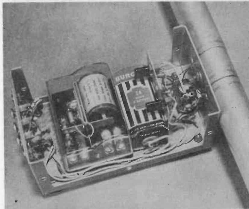
Fig. 10-9.—Interior view of the "ON-OFF" Light Controlled Relay.
