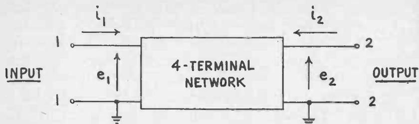
Fig. 12-1.—Basic four-terminal network representation shown as a "black box." Input and output terminals and input and output voltages and currents are identified. Arrows show conventional flow.
