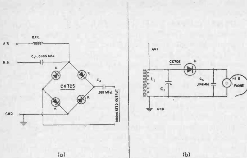
Fig. 10-26.—R.F. Semiconductor Diode applications: (a) Bridge Modulator; (b) Simple Crystal Receiver.
