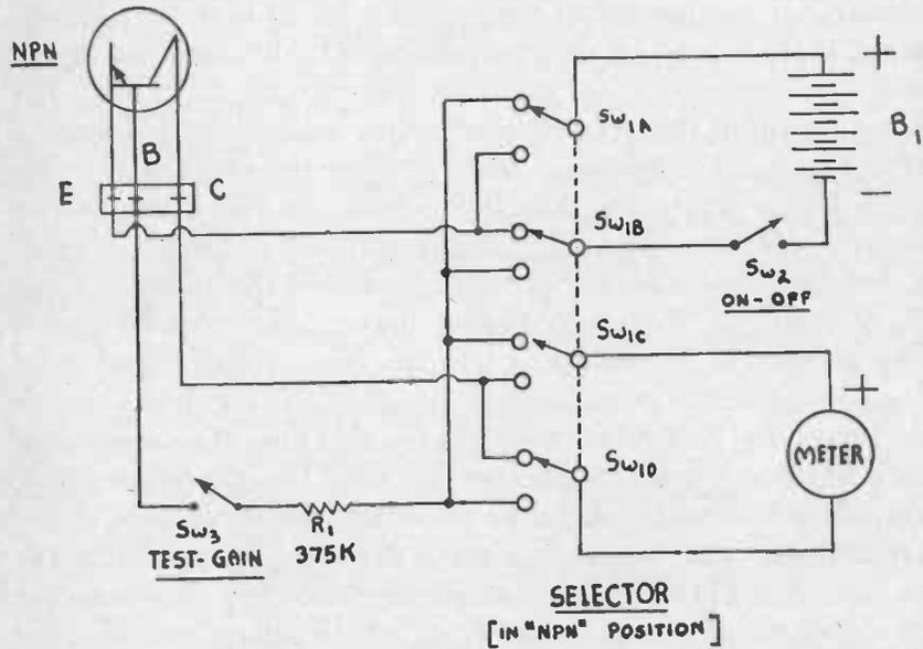
Fig. 9-18.—Circuit for a simple Transistor Checker.
