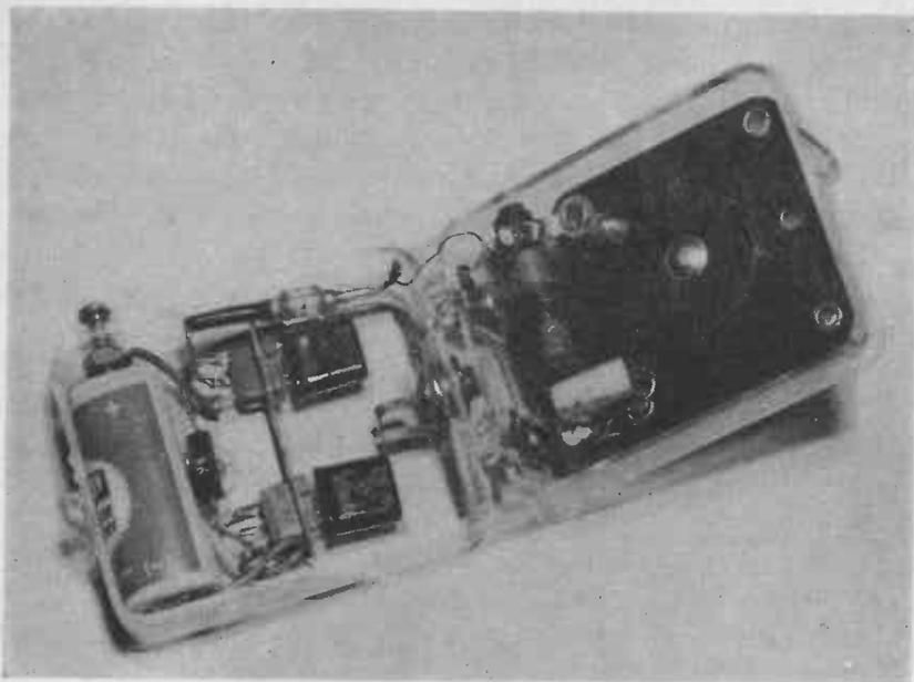
Fig. 8-7.—Interior view of the Pocket Receiver.
