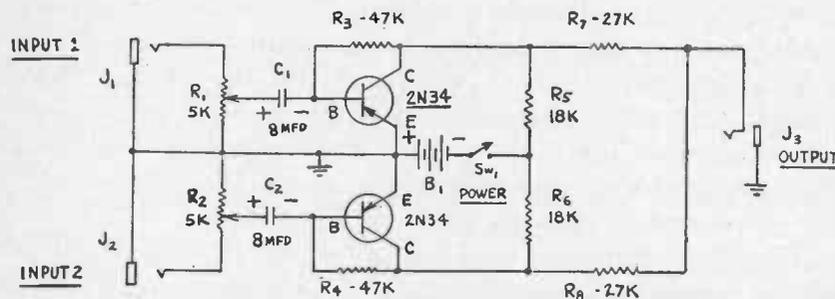
Fig. 7-17.—A transistorized 2-Channel Audio Mixer.
