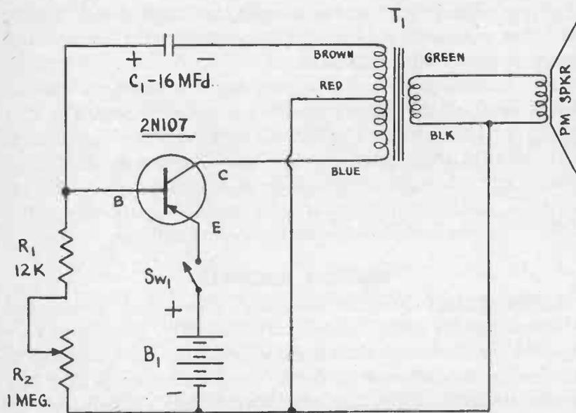
Fig. 10-16.—Schematic diagram of a transistorized *Metronome*.
