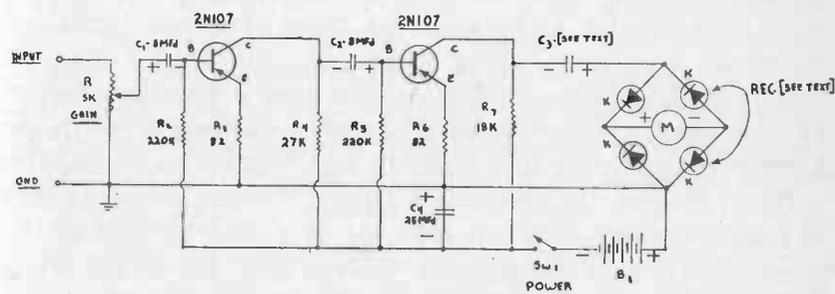
Fig. 9-26.—Schematic of an easily built *Audio Level Meter*.
