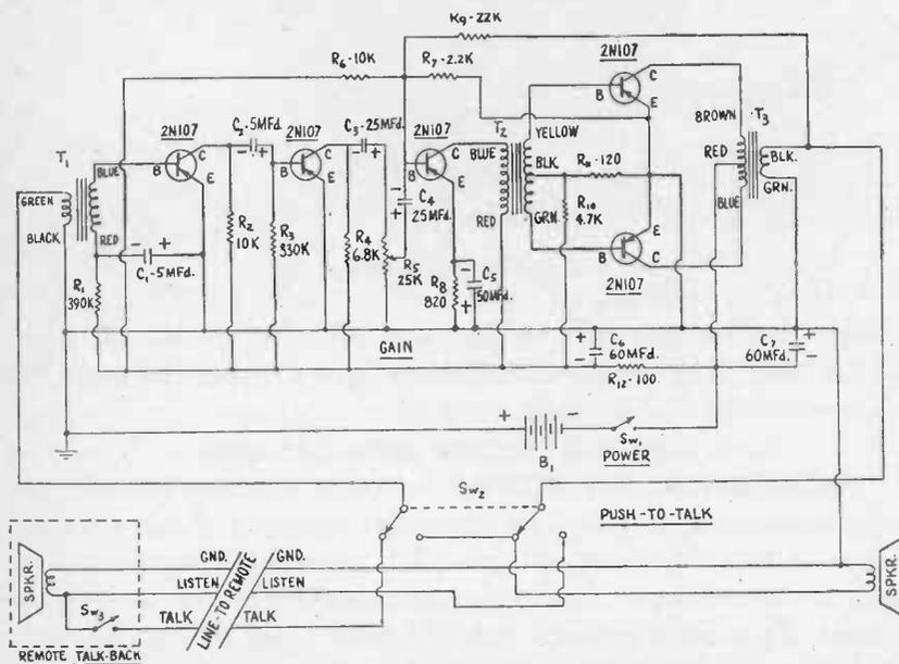
Fig. 7-13.—A transistorized two-station *Intercom*.
