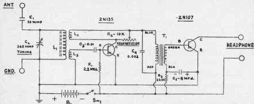
Fig. 8-3.—Transistorized Regenerative Receiver with audio stage added.
