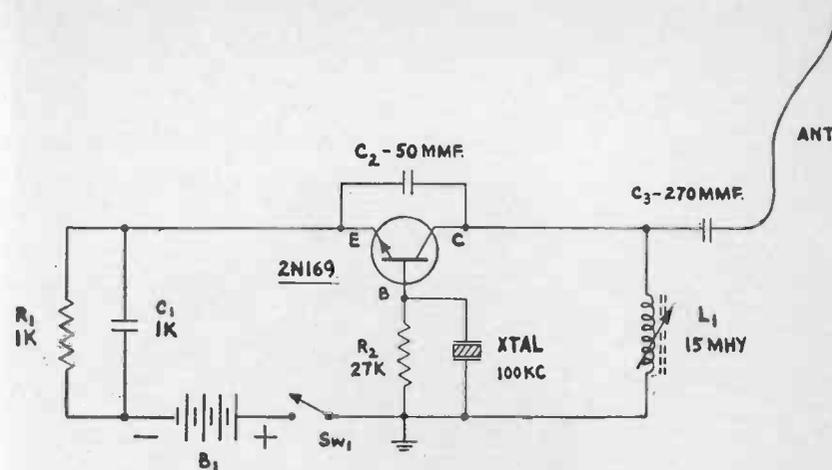
Fig. 8-18.—Diagram of a 100 KC crystal-controlled Calibrator.
