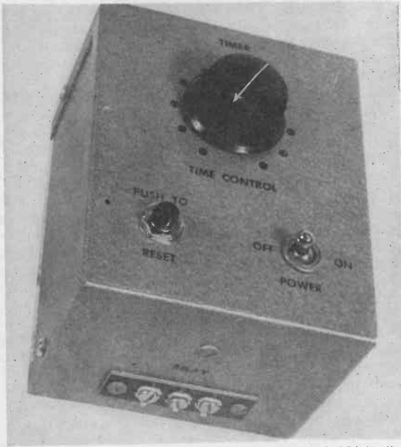
Fig. 10-3.—Author's model of a transistorized Timer. Courtesy Radio & Television News
