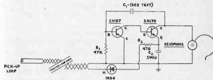
Fig. 8-21.—Schematic of an easily built Ham Station Monitor.
