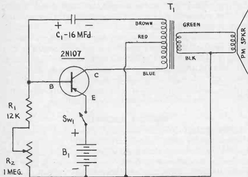
Fig. 10-16.—Schematic diagram of a transistorized *Metronome*.
