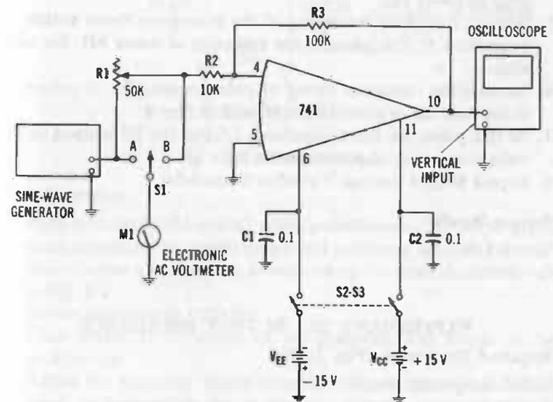
Fig. 2-26. Input impedance.
