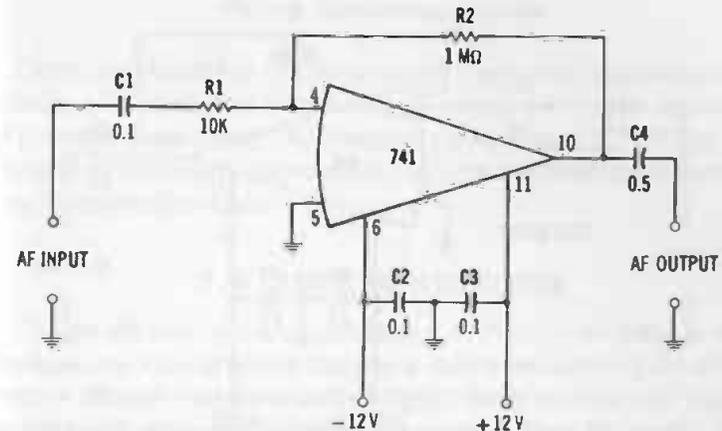
Fig. 3-3. Gain-of-100 audio amplifier.
