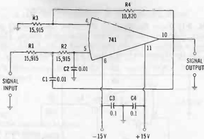
Fig. 3-13. Low-pass filter.
