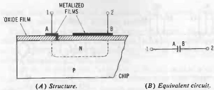
Fig. 1-4. Integrated capacitor.
