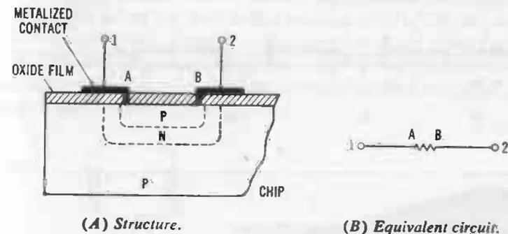
Fig. 1-3. Integrated resistor.
