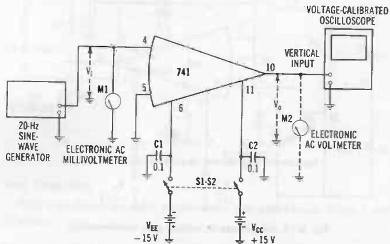
Fig. 2-13. Open-loop ac voltage gain.
