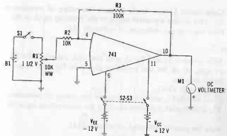
Fig. 2-4. Output polarity (step 1).
