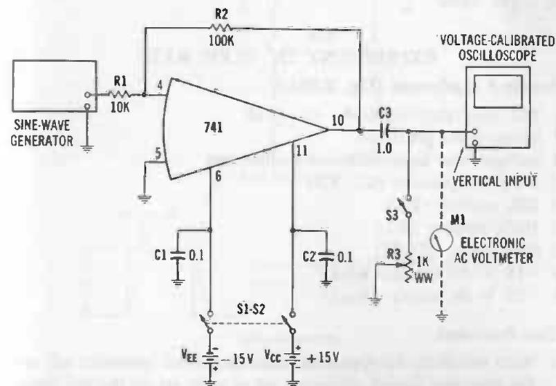
Fig. 2-27. Output impedance
