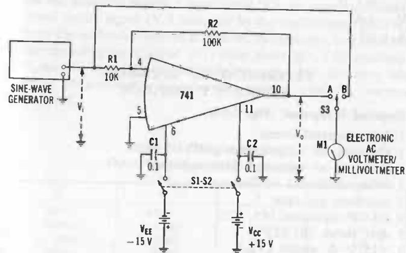
Fig. 2-14. Closed-loop ac voltage gain.
