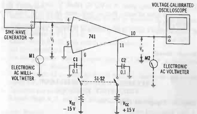
Fig. 2-15. Open-loop frequency response.
