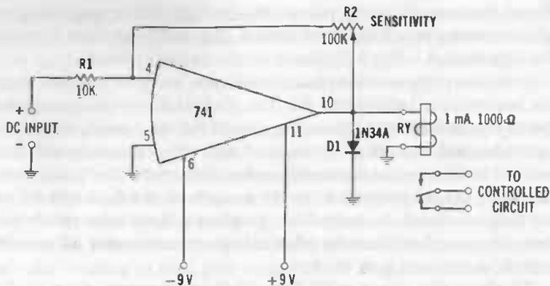
Fig. 3-32. Sensitive dc relay.
