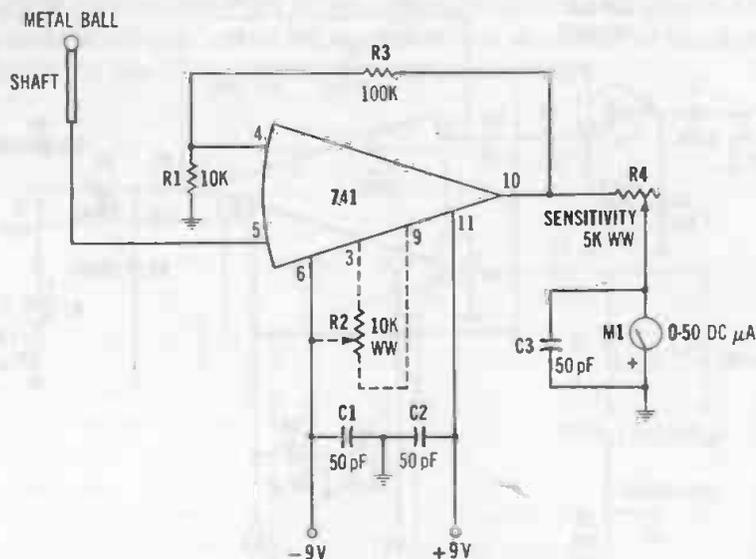
Fig. 3-31. Electrostatic voltmeter.
