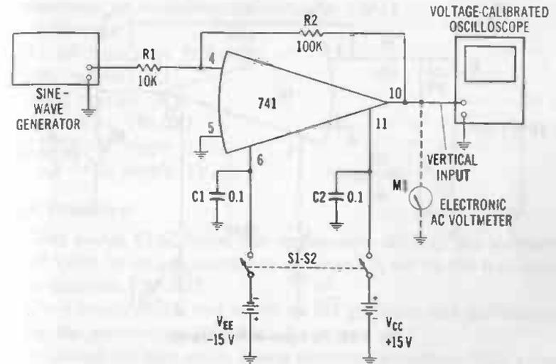
**Fig. 2-19. Maximum ac output-voltage swing.**
