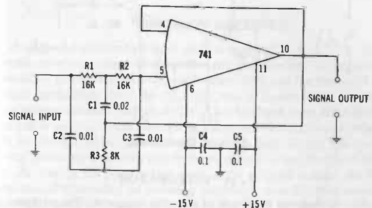
Fig. 3-17. High-Q notch filter.
