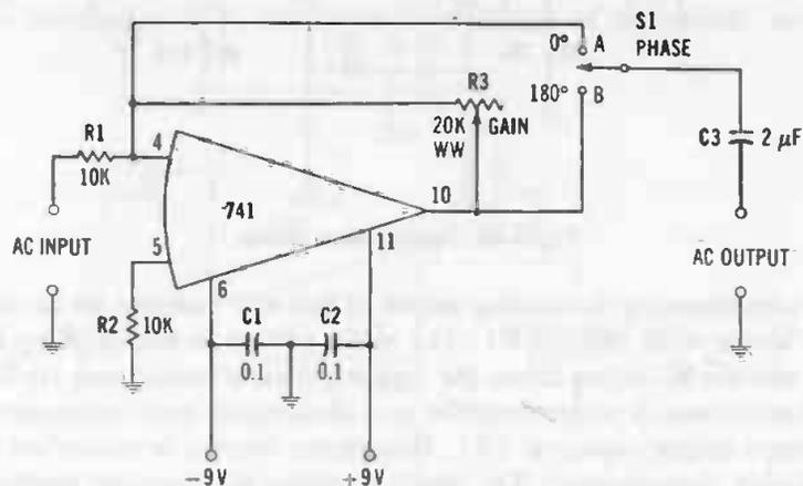
Fig. 3-41. Phase reverser.
