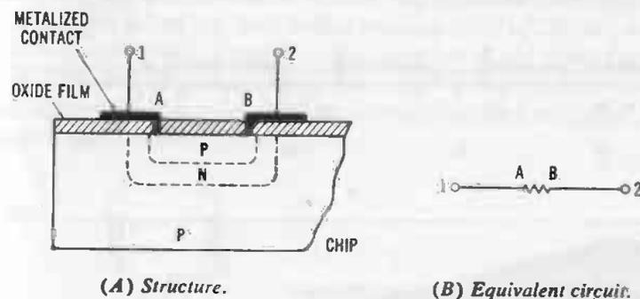
Fig. 1-3. Integrated resistor.
