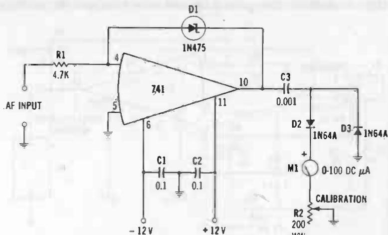
Fig. 3-29. Analog-type audio frequency meter.
