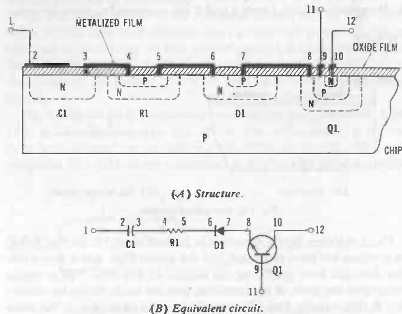
Fig. 1-5. Example of complete integrated circuit.
