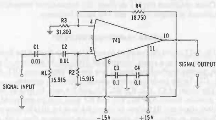
Fig. 3-14. High-pass filter.
