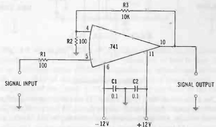
Fig. 3-5. Noninverting amplifier.
