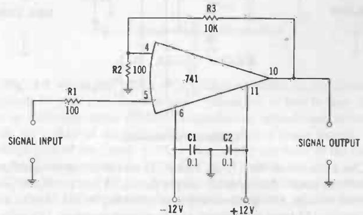
Fig. 3-5. Noninverting amplifier.
