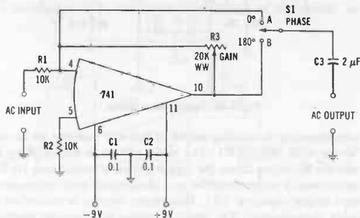
Fig. 3-41. Phase reverser.
