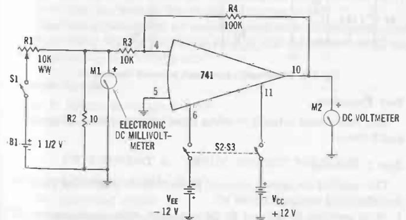
Fig. 2-7. Offset-null adjustment, external (method 1).
