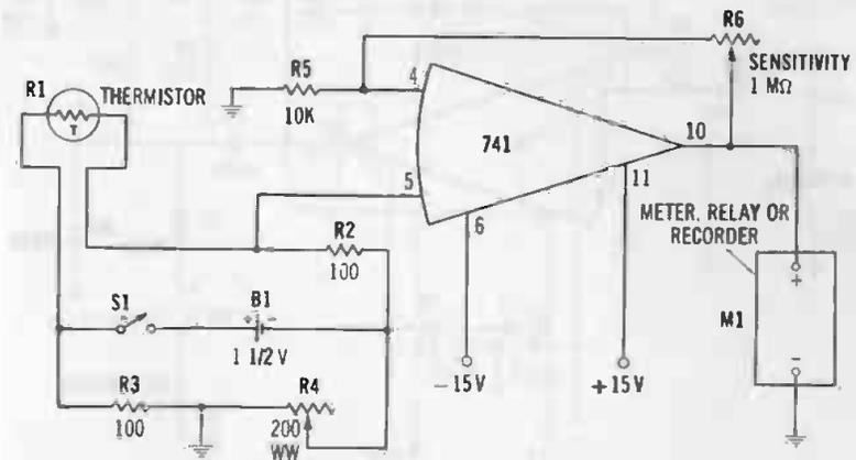
Fig. 3-28. Electronic thermometer.
