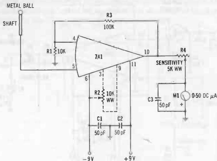
Fig. 3-31. Electrostatic voltmeter.
