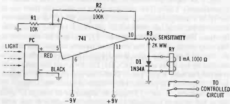
Fig. 3-35. Photorelay.
