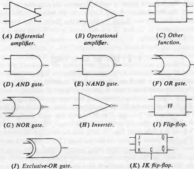
Fig. 1-7. Integrated-circuit symbols.
