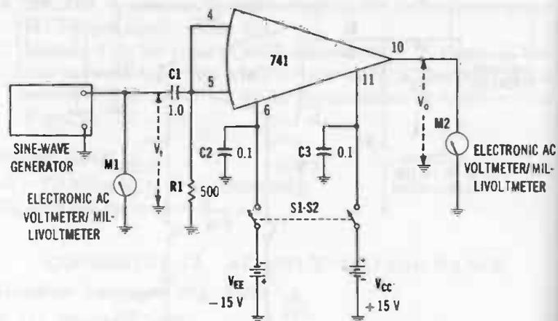
Fig. 2-22 Common-mode rejection.
