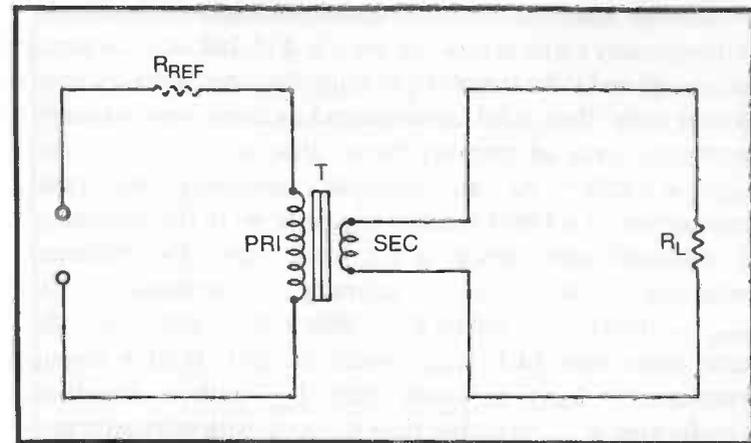
Fig. 2-12. Reflected impedance in the primary of a transformer with resistance  $R_L$  loading the secondary.
