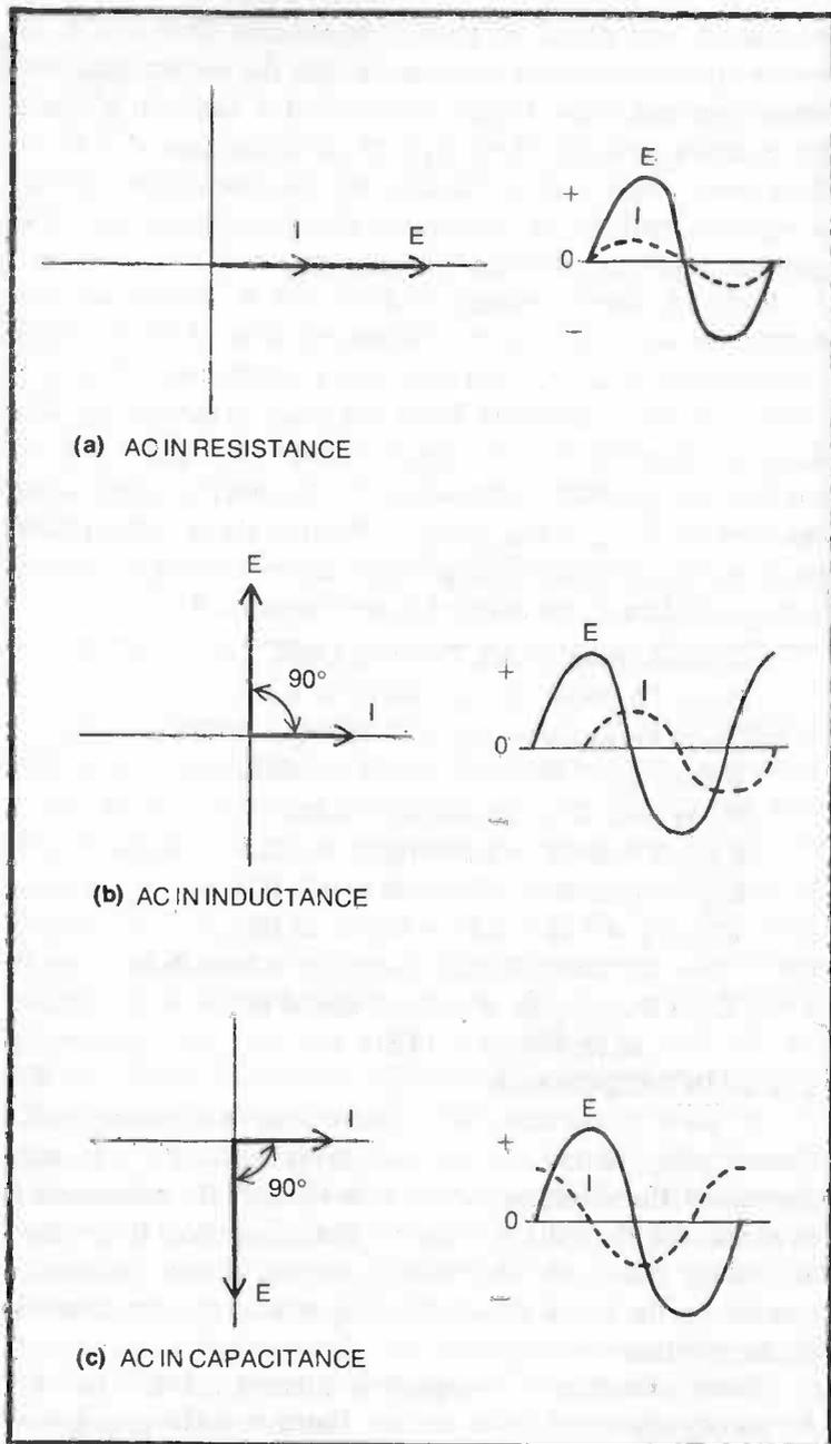
Fig. 1-8. Current/voltage/phase relationships with voltage applied to (a) a pure resistance, (b) a pure inductance, (c) a pure capacitance.
