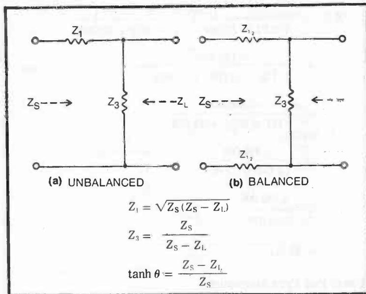
Fig. 2-20. L-type pad attenuators: (a) unbalanced and (b) balanced. Equations given are for finding impedance values.
