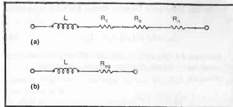
Fig. 4-5. Equivalent circuits of core-type inductors with: (a) losses shown as series-resistance components, and (b) losses simplified to the equivalent resistance.
