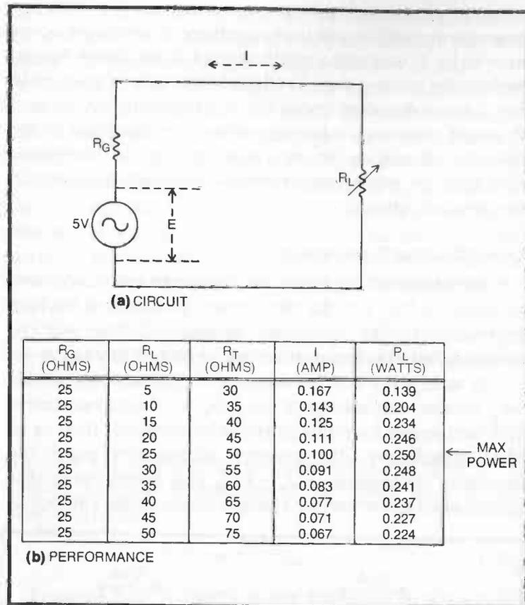
Fig. 2-13. Illustration of impedance matching. The circuit (a) has a variable load resistance connected to a generator. The chart (b) shows the performance of the circuit as the resistance ( $R_L$ ) is varied.
