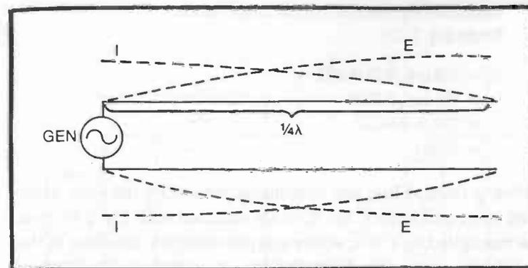
Fig. 2-7. Current and voltage distribution on an unterminated quarter-wave line.
