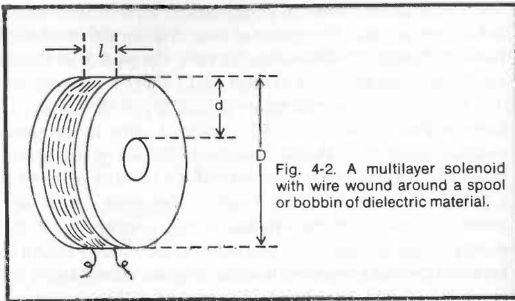
Fig. 4-2. A multilayer solenoid with wire wound around a spool or bobbin of dielectric material.
