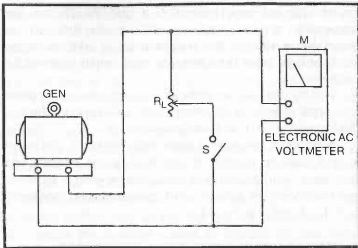
Fig. 3-13. Test setup used to measure the impedance of a mechanical generator.
