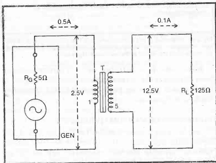
Fig. 2-14. Impedance-matching transformer.
