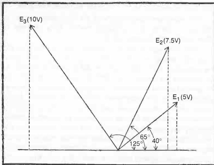
Fig. 1-7. Vector diagram of out-of-phase components.
