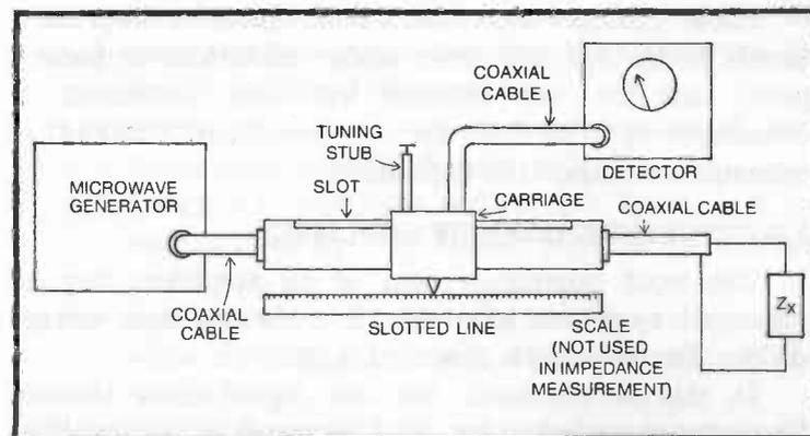
Fig. 3-8. Test setup using the slotted line to measure impedance at microwave frequencies.
