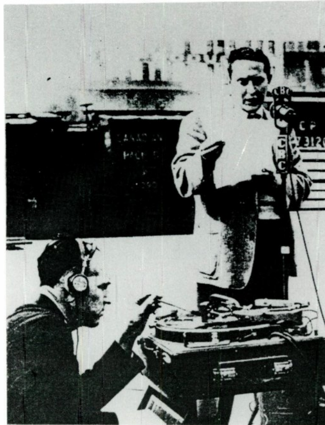
Announcer Bill Herbert recording a program “in the field” with technician Clayton Wilson in the 1940’s. Herbert’s commentary is being recorded on a Model Y disk recorder; Wilson is ensuring that the strands of cut acetate do not foul the cutting stylus.
