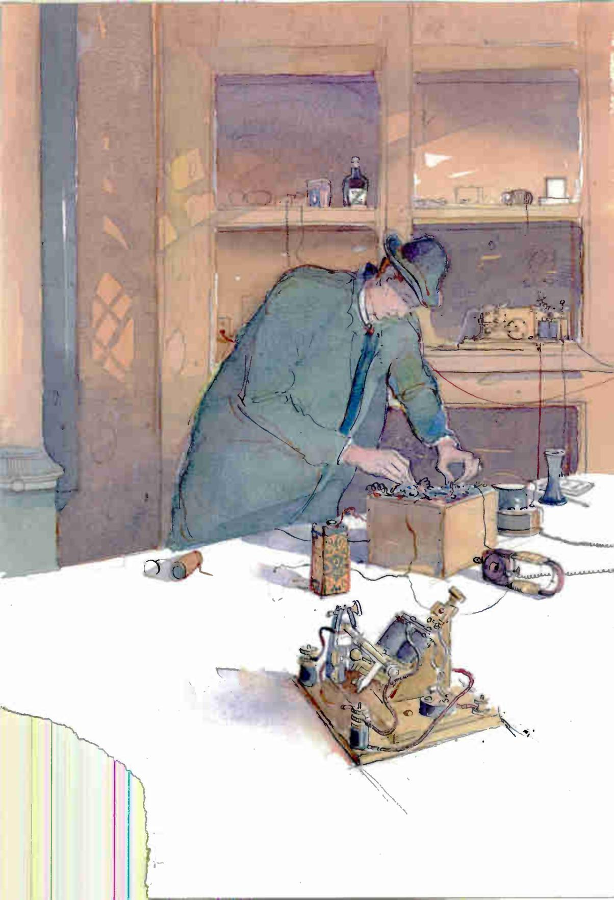
The coherer was linked to the aerial. When an electrical vibration touched the aerial, a burst of electricity ran down the wire to the filings in the tube. These would stick together and let the electricity pass across them—they formed a *switch*, switching electricity “on.” At once the tapper would knock the filings loose and the electricity would switch “off” again.
