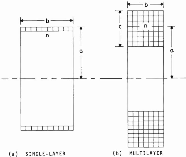
10.1 Fig. 1 — The two common forms of air-core inductor.
