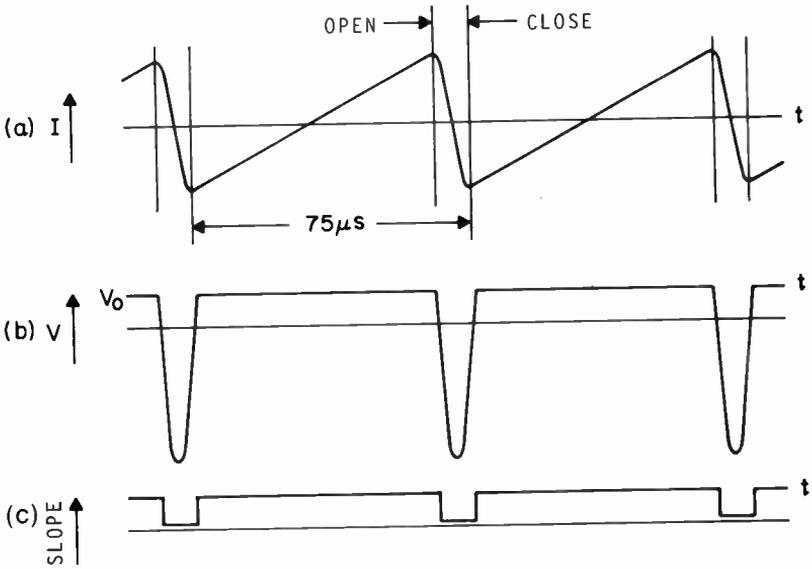
7.5 Fig. 1 — Sawtooth-current horizontal scanning.
