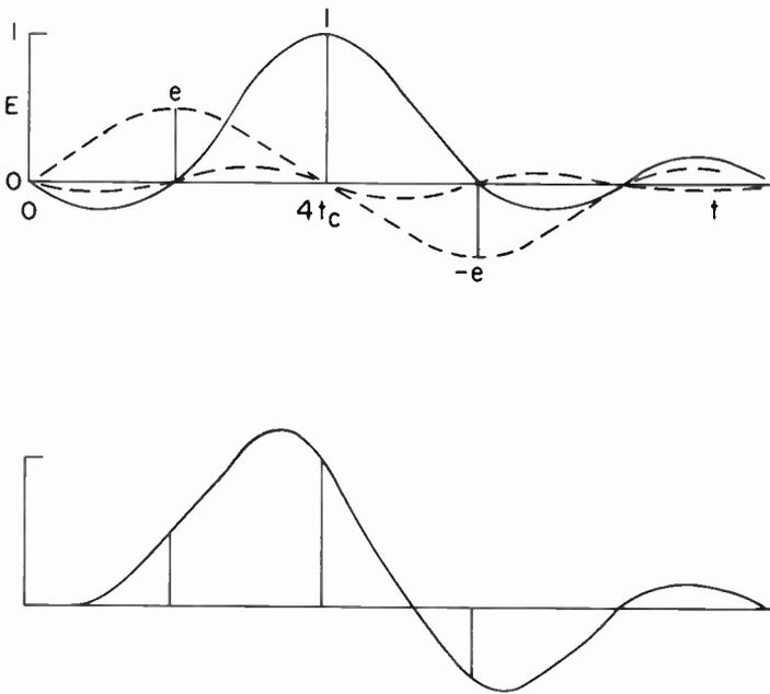
7.3 Fig. 3 — The application of paired echoes to evaluate the effects of the phase distortion.
