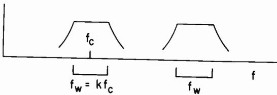
7.4 Fig. 8 — Preselector with channel switching and equal bandwidths
