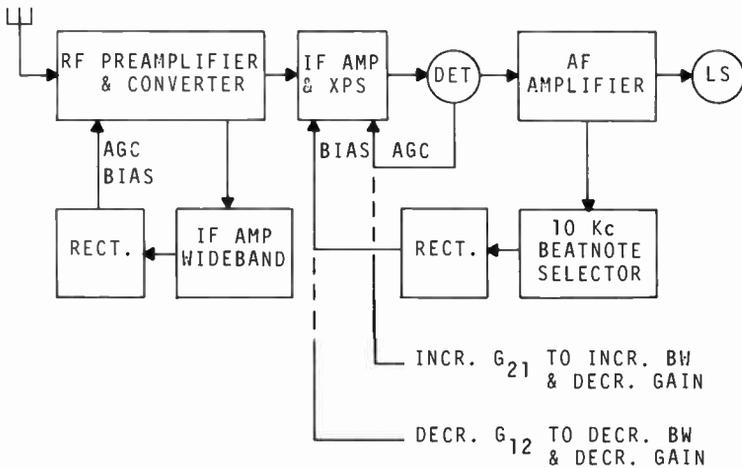
6.6 Fig. 3 — Superheterodyne receiver with AXPS.
