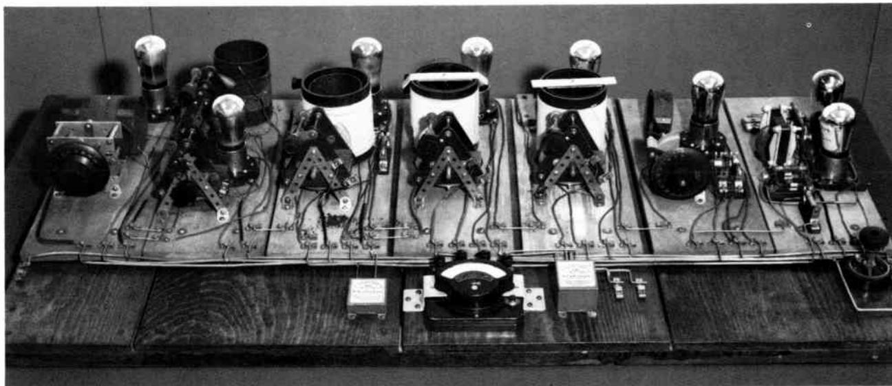
Photo 9 — Washington receiver with diode AVC 1926.
