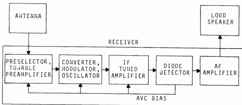
6.1 Fig. 1 — Superheterodyne receiver around 1931.
