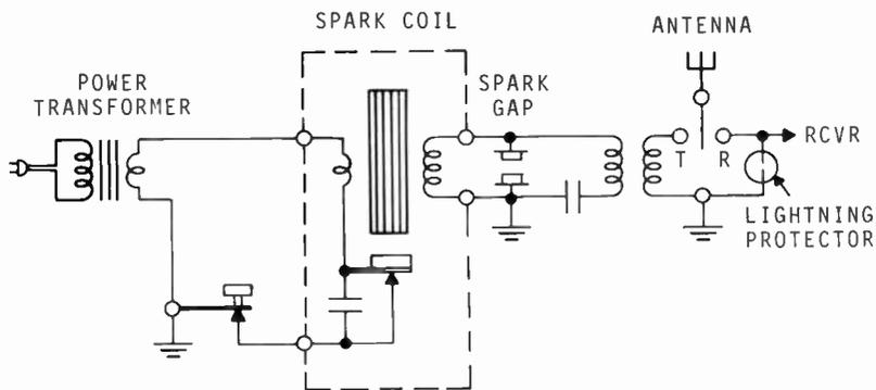
1.4 Fig. 1 — Transmitter circuit of Station 3QK.
