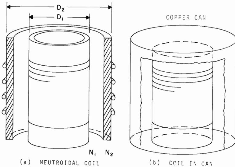
10.2 Fig. 1 — Comparable coils with small external field.
