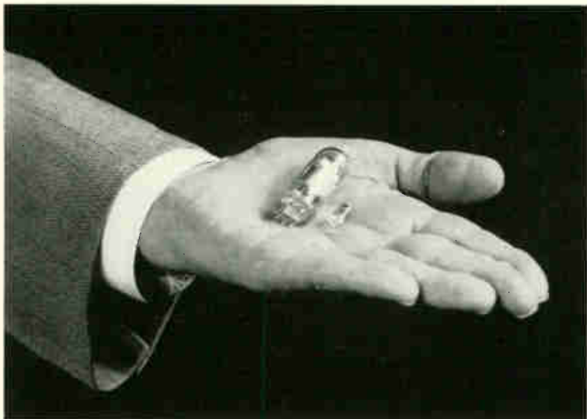
BELOW: The tiny transistor is compared with a miniature vacuum tube which it is rapidly replacing in radio sets and other electronic apparatus.
