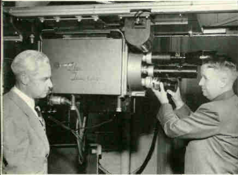
The first compatible color TV system for medical use was designed by RCA. The TV camera is fitted horizontally and "sees" the subject via a mirror which picks up reflections through an opening in a surgical lamp.
