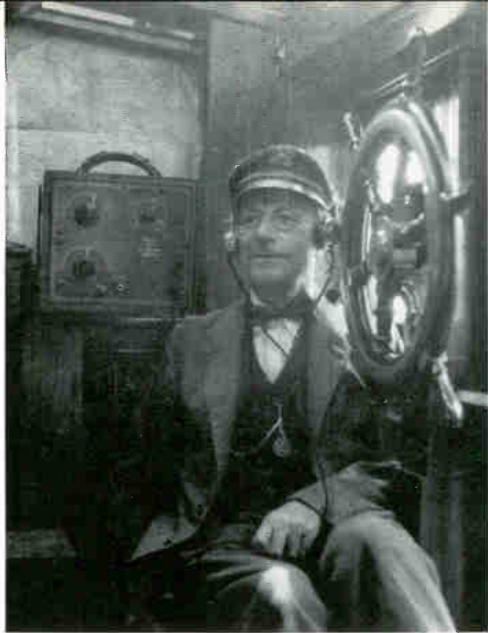
Radio entertainment became available to ships at sea with the introduction of the RCA Radiola II—one of the earliest battery portable receivers.
