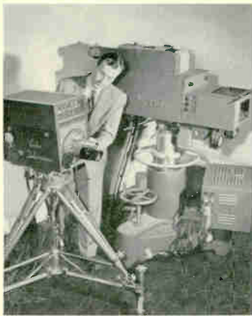
Brainchild of RCA engineers is this color TV camera, which uses only one pickup tube.
