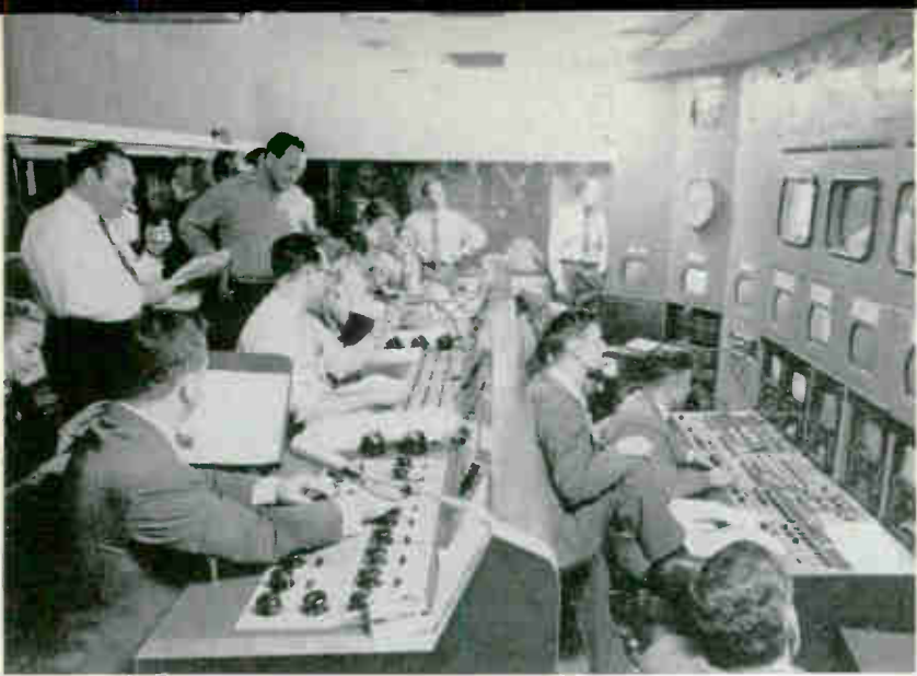
In NBC's TV Studio 5H at Radio City, New York, a single coordinator can view material picked up by various cameras and can switch from one to another in order to keep pace with developments of general interest.
