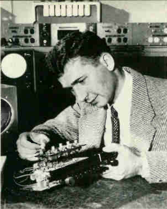
A boon to motorists is this automobile radio, operating from transistors instead of tubes. The transistors operate directly from a 6-volt car storage battery.
