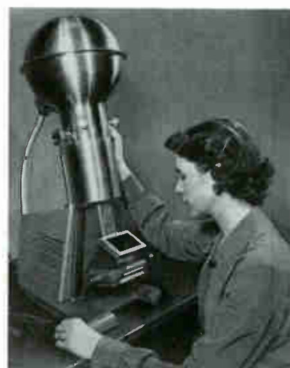
A compact table model electron microscope was developed by RCA for use in colleges, hospitals, and industrial laboratories.
