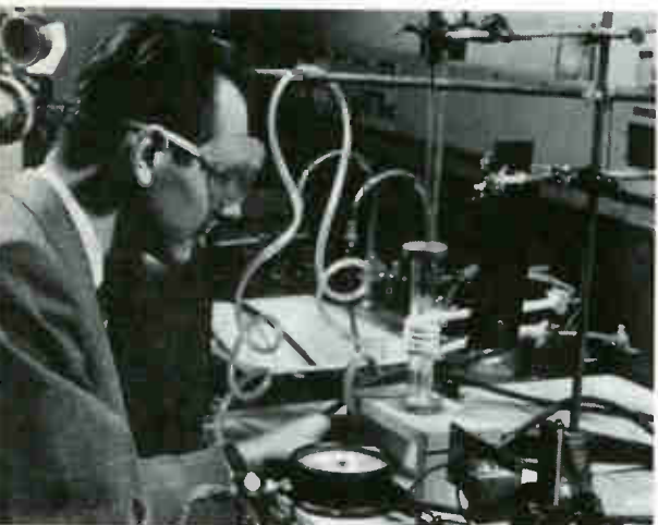
A germanium crystal is grown with the aid of heat generated by a small radio-frequency furnace.
