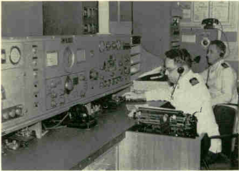
Equipment in the radio room of the "U.S.S. America" includes a direction finder and an automatic S.O.S. detector.
