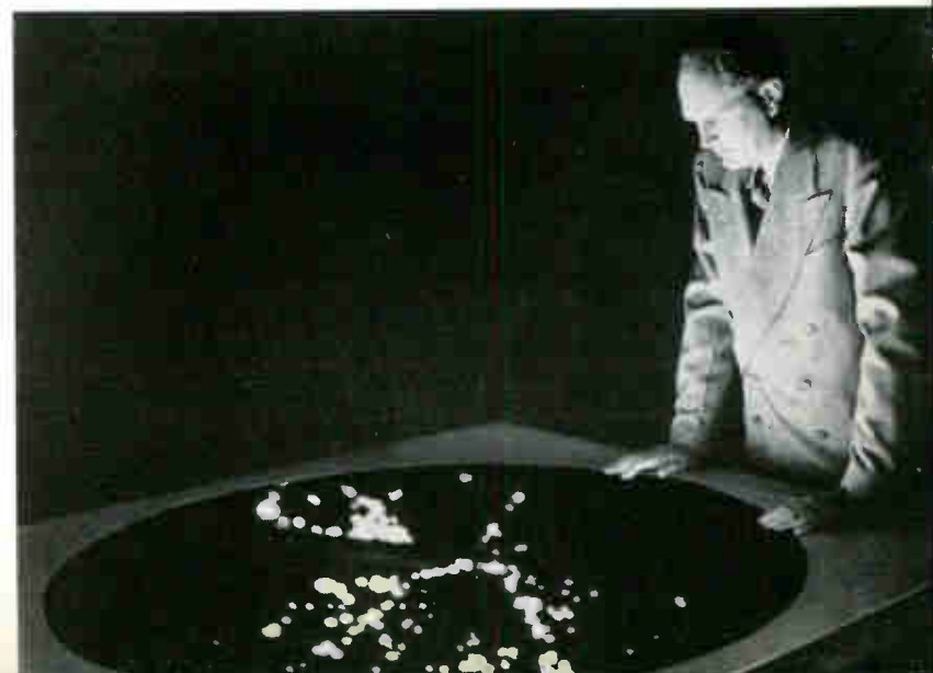
Large-screen radar, which can be viewed in normal lighting conditions, has been developed for air traffic control and similar uses.
