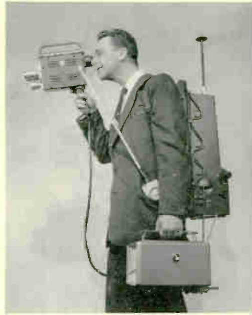
Well-known news commentator Chet Huntley carries a portable TV camera and back-pack transmitter, two-way "transceiver" for radio communication (in pocket) and a light portable TV set.
