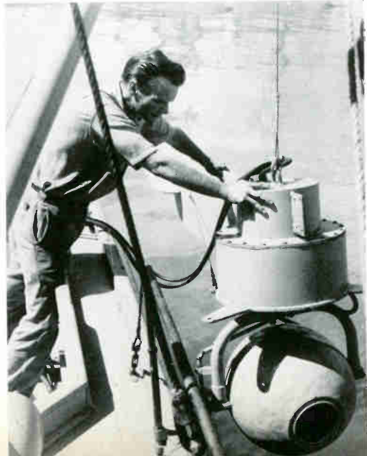
The use of underwater closed-circuit television enables the U.S. Fish and Wildlife Service to observe experimental equipment and methods under actual oceanic conditions.
