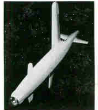
One of the U.S. Navy's flying weapons which employs television "eyes" to guide it to its target.
