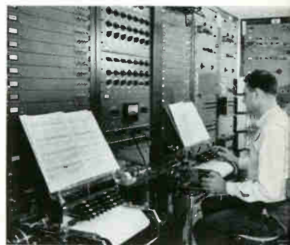
This electronic synthesizer will create any musical tone; it translates coded information into musical sounds for disk recording.
