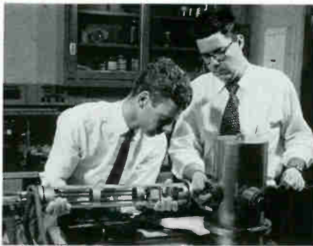
Demountable vacuum systems are used in studying the interaction of electron beams with microwaves.
