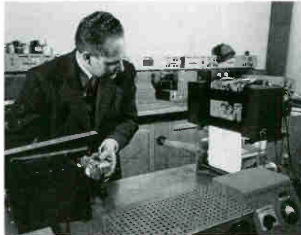
Adjusting a laboratory model of a continuous microfilm enlarger making prints on Electrofax paper.
