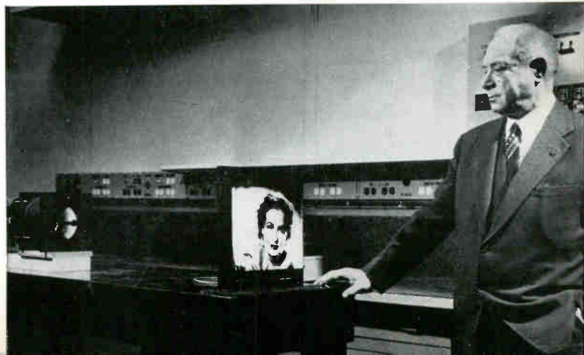
David Sarnoff watches a demonstration of the RCA light amplifier, which presages important developments in television, radar, and associated fields. For example, the light amplifier will make it possible to see a TV show on a screen that can be framed and hung like a picture.
