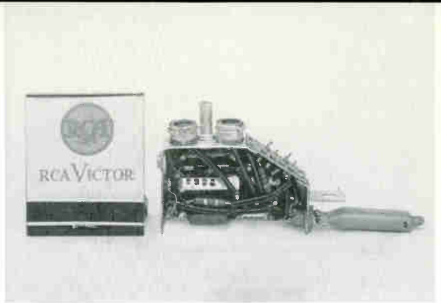
The complete receiver output section of a modern half-size walkie-talkie compared to a match folder. This assembly is a typical result of sub-miniaturization techniques.
