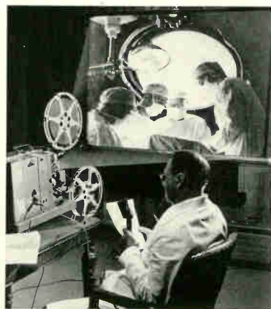
An ancillary aid to medicine is a 16 mm recorder-projector which enables sound to be recorded magnetically on the edge of 16 mm film. The recording can be played back immediately and any necessary erasures or alterations made.
