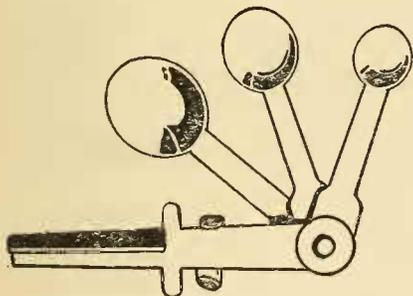
A New Measuring Spoon Which Saves Much Time and Many Poor Mixtures. It Always Levels Off the Spoon Even and Is Graduated as Indicated.
