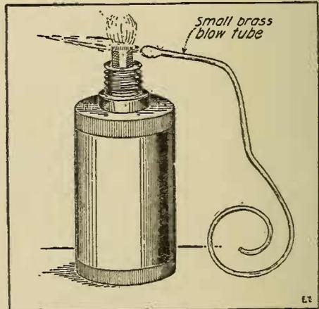
Simply Fill a Fan Grease Cup with Wood Alcohol, Insert a Wick in the Hole, and You Have a Serviceable Little Spirit Lamp for Light Soldering.
