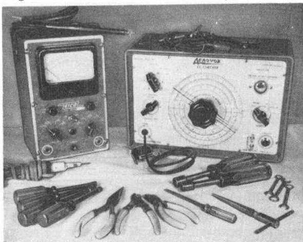
Fig. 2503. *Basic equipment needed to begin a radio repair business.*
