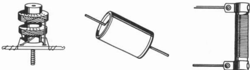
Fig. 604. Chief actors—inductor, capacitor, resistor.
