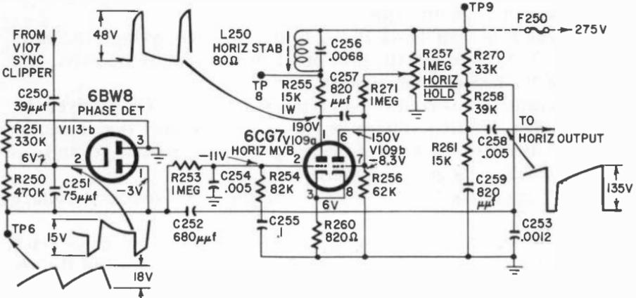
Fig. 1107. The error voltage from the phase detector controls the frequency of the cathode-coupled multivibrator. Appropriate waveforms are indicated.
