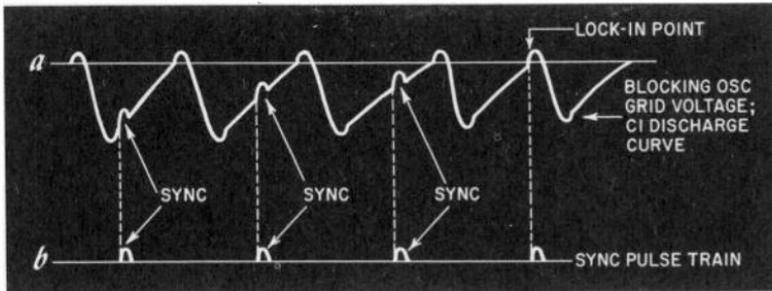
Fig. 1109. Capacitor discharge curve (a) shows how sync pulses (b) ride in on grid-voltage waveform to lock in the oscillator.
