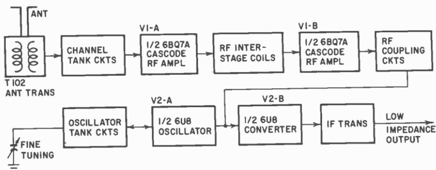
Fig. 508. Block diagram of incremental type cascode tuner.
