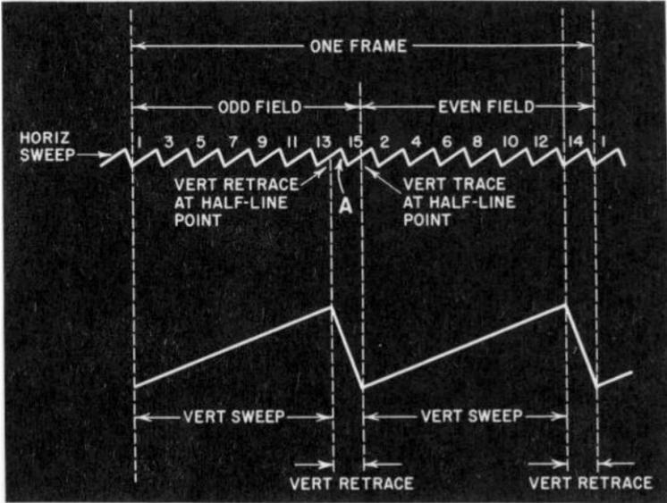
Fig. 303. Sawtooth waves across top show rise and fall of horizontal sweep energy which pulls spot across screen. Sharp, downward slope is retrace. Large sawteeth (below) show how spot is pulled down while being swept across screen. (Waveform amplitudes are not drawn to same scale.)
