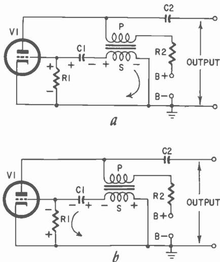
Fig. 1108. Circuit diagram of a blocking oscillator. (a) First part of cycle shows capacitor  $C_1$  charge path. Current flow through tube reaches saturation. (b)  $C_1$ 's discharge path. At saturation, plate current no longer rises and  $C_1$  discharges through  $R_1$ , repeating the cycle in (a).
