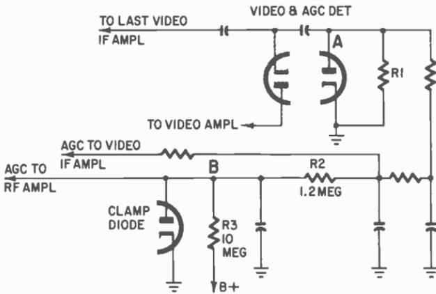
Fig. 710. This simplified schematic of a delayed agc system has delay for the rf amplifier only.
