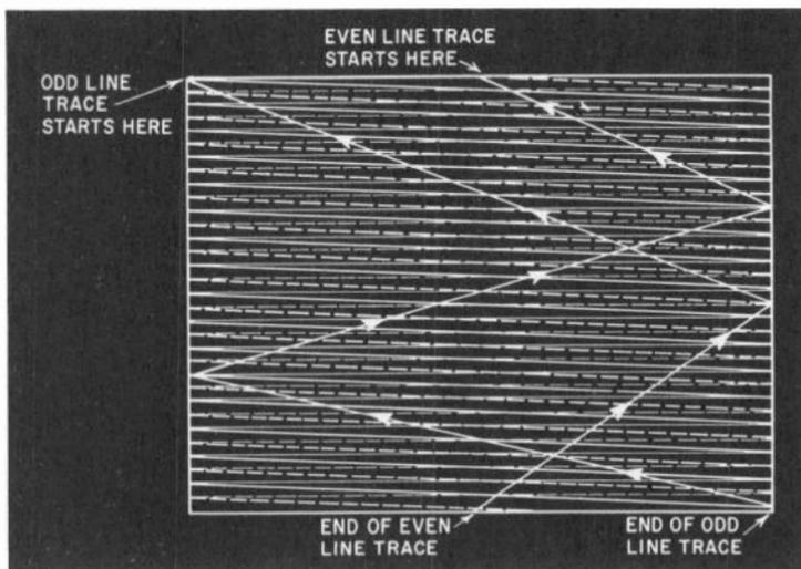
Fig. 106. For simplicity only a small number of the 525 lines are shown in this basic interlaced scan. The vertical sweep causes the downward tilt of the horizontal lines.
