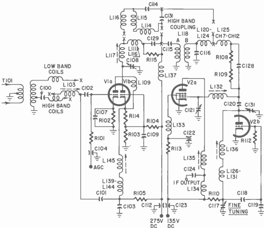
Fig. 509. Cascode-tuner circuit. Direct coupling is used by the rf amplifier.
