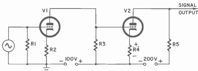
Fig. 507. Schematic diagram of basic direct-coupled amplifier circuit.
