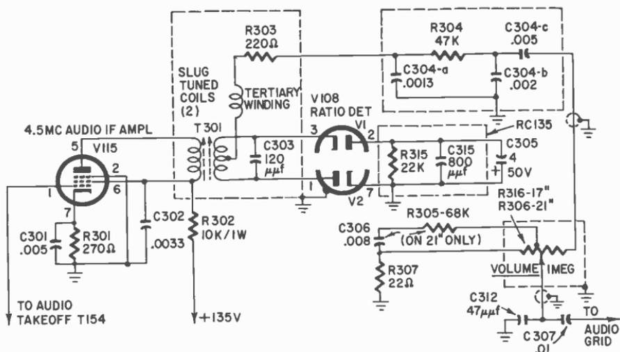
Fig. 1309. Typical ratio-detector circuit.
