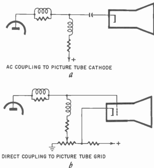
Fig. 811. Simplified schematic showing: (a) ac coupling to picture tube cathode; (b) dc coupling to picture tube grid.
