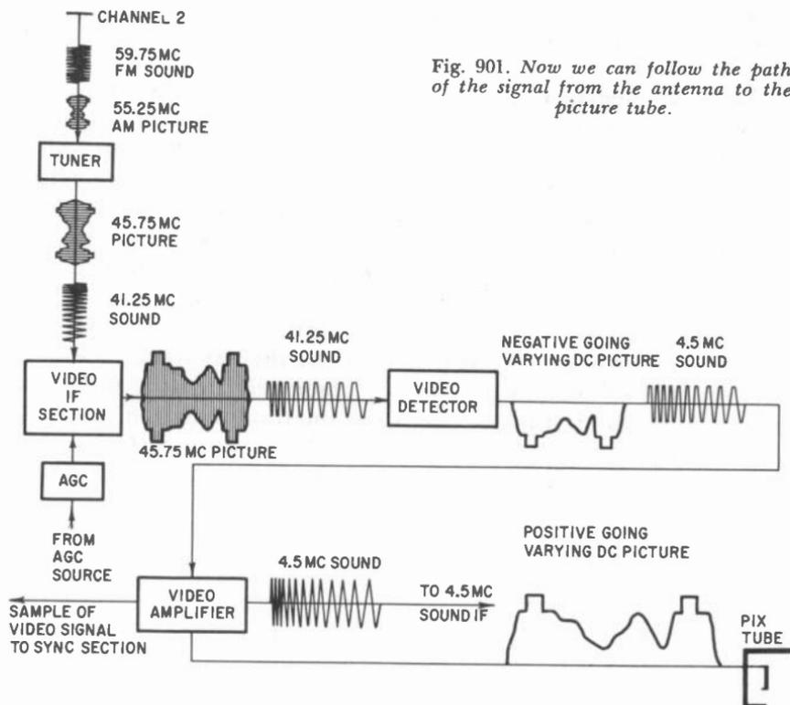
Fig. 901. Now we can follow the path of the signal from the antenna to the picture tube.
