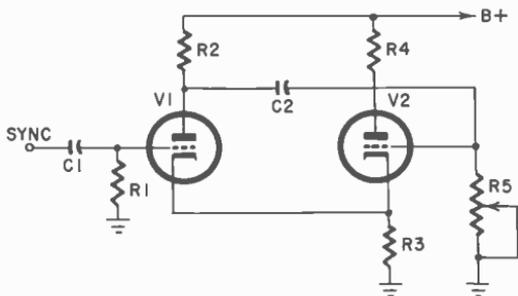
Fig. 1106. Cathode-coupled multivibrator circuit.
