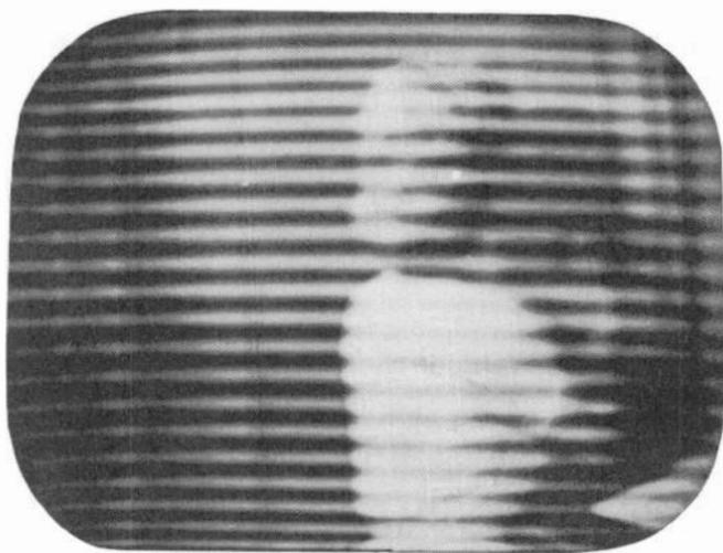
*Fig. 812. Sound bars are most commonly caused by an improperly adjusted local oscillator in the tuner. Sound bars are more pronounced when picture signals are not being transmitted or during scenes of low contrast.*
