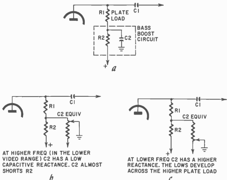
Fig. 804. (a) Bass-boost circuit ( $R_2$  and  $C_2$ ) for low-frequency compensation. (b) Equivalent circuit using variable resistor in place of  $C_2$ .  $C_2$  acts like a short circuit at higher end of low-frequency portion of spectrum. (c) At lower frequencies,  $C_2$  has a higher reactance.
