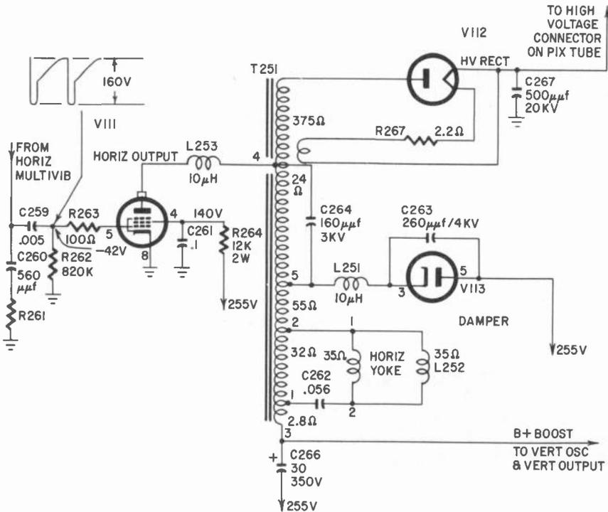
Fig. 1203. Horizontal sweep output and high-voltage rectifier stages.
