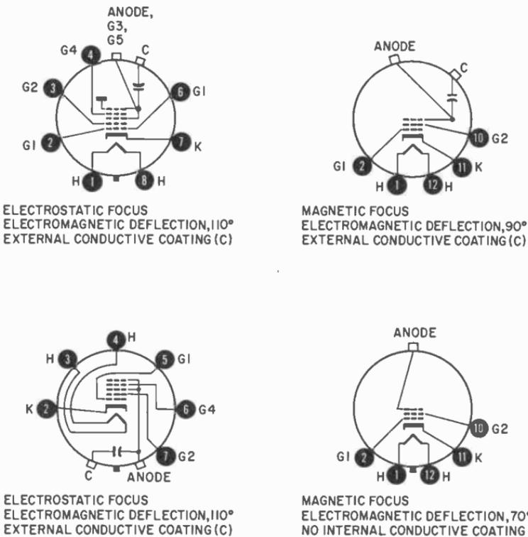
Fig. 215. CRT base connection diagrams show a more complex internal structure when designed for electrostatic focusing.
