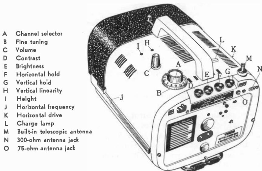
Fig. 1503. Even the rear of the case would require more than a quick glance to distinguish between tube and transistor TV receiver. (Sony Corp.)
