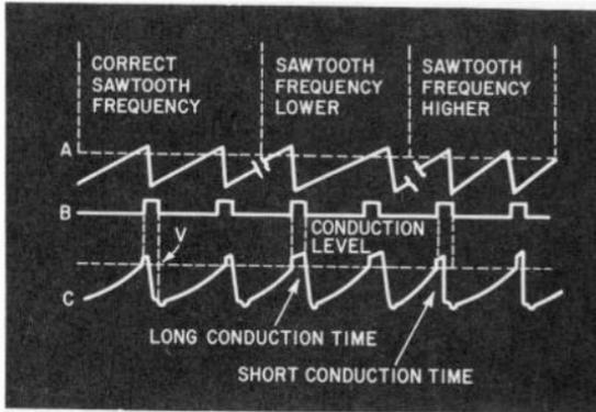
Fig. 1016. Illustration shows how varying the frequency at V1-a's grid (Fig. 1015) makes the sync pulses either narrower or wider, thus increasing or decreasing the current at V1-b's grid and keeping the oscillator at one frequency.
