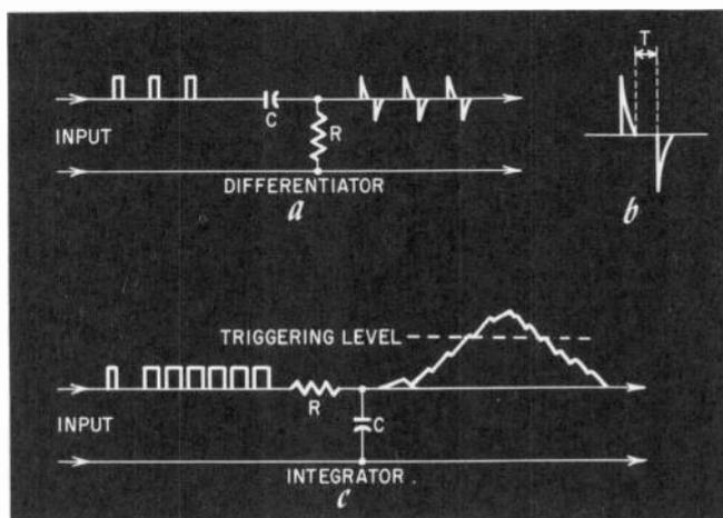
Fig. 1008. (a) Output pulses of differentiator are sharp spikes. (b) Spikes enlarged to show rapid rise and fall time. (c) Integrator circuit has a long time constant, charges and discharges very slowly. Triggering level is point at which the vertical oscillator frequency is locked.
