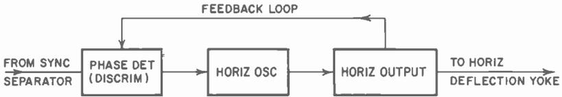
Fig. 1009. Block diagram of basic horizontal afc system.
