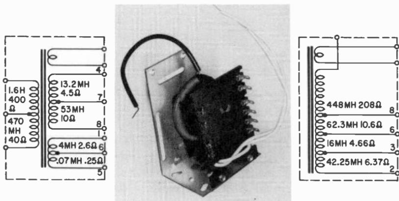
Fig. 1206. Isolation and autotransformer types of horizontal output transformer.
