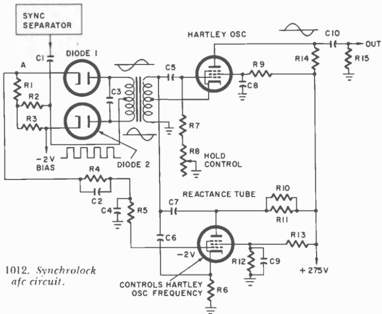
Fig. 1012. Synchrolock afc circuit.
