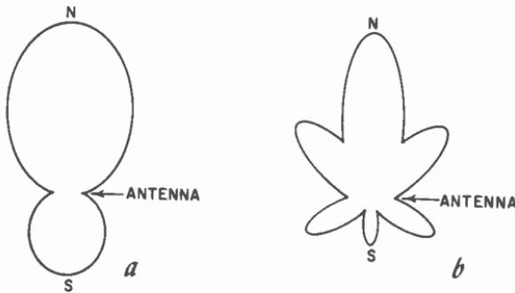
Fig. 502. Lobe pattern (a) is typical for a wide-band antenna operating at a low-channel frequency. Used for reception on one of the high-band vhf channels, the pickup pattern often develops many minor lobes (b) that make orientation difficult.
