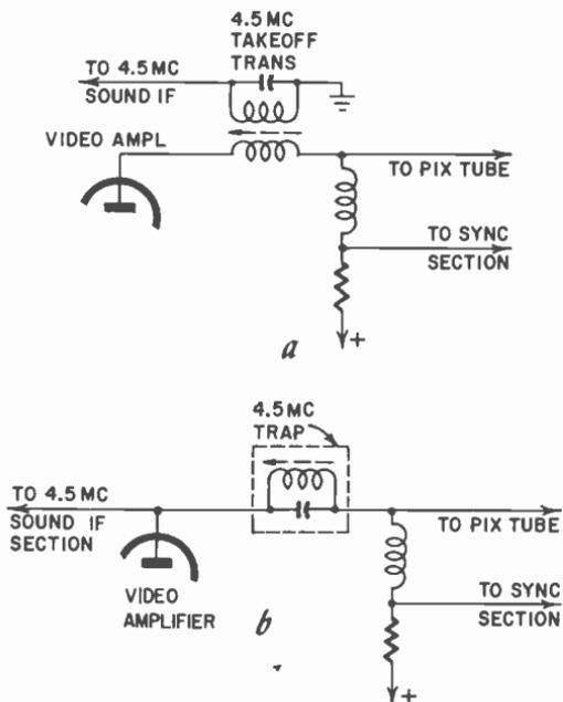
Fig. 810. Two methods for removing the 4.5-mc sound signal from the video amplifier plate circuit. (a) 4.5-mc sound takeoff transformer absorbs signal. (b) 4.5-mc trap prevents sound signal from getting into picture tube.
