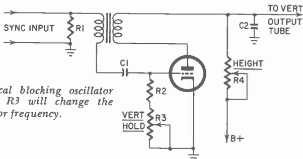
Fig. 1110. Typical blocking oscillator circuit. Varying  $R3$  will change the oscillator frequency.
