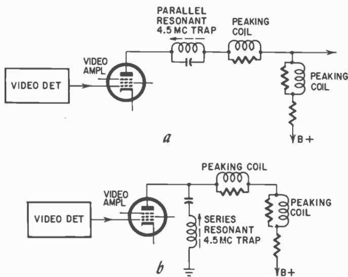
Fig. 808. (a) Parallel resonant 4.5-mc trap. (b) Series resonant 4.5-mc trap. Any 4.5-mc signal that may have leaked through from the video detector stage is trapped out with either type.
