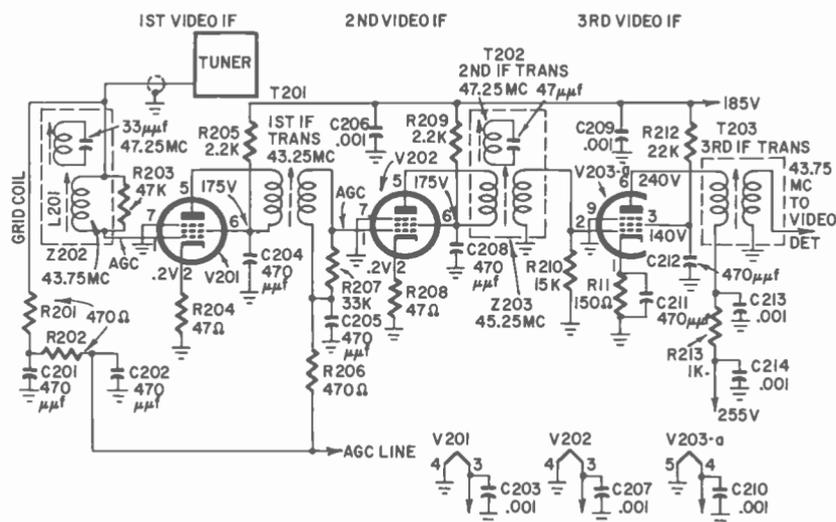
Fig. 603. Stagger tuned if circuit.
