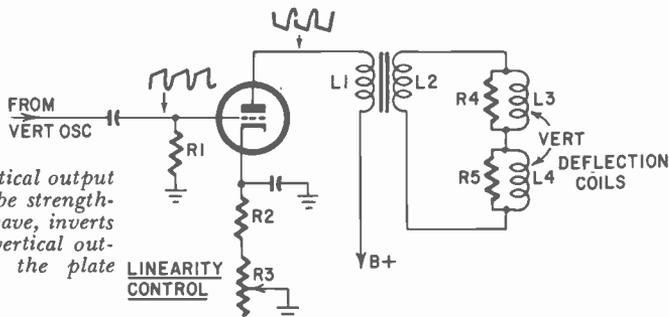
Fig. 1114. Typical vertical output tube circuit. The tube strengthens the trapezoidal wave, inverts it and feeds it to a vertical output transformer in the plate circuit.
