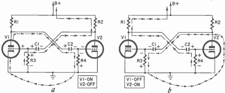
Fig. 1102. Circuit diagram of a basic plate-coupled multivibrator. (a) Operation of multivibrator with V1 conducting and V2 cut off. (b) Operation with V2 conducting and V1 cut off.
