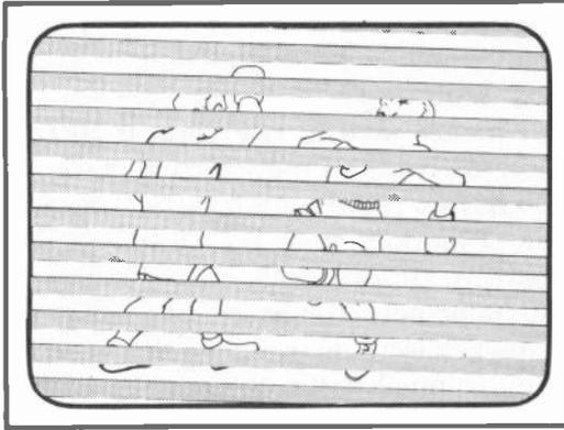
Fig. 104. This is the picture traced by the spot during the *even-line field*.
