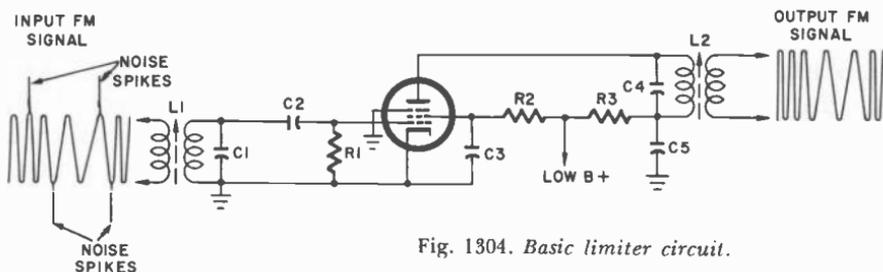
Fig. 1304. Basic limiter circuit.
