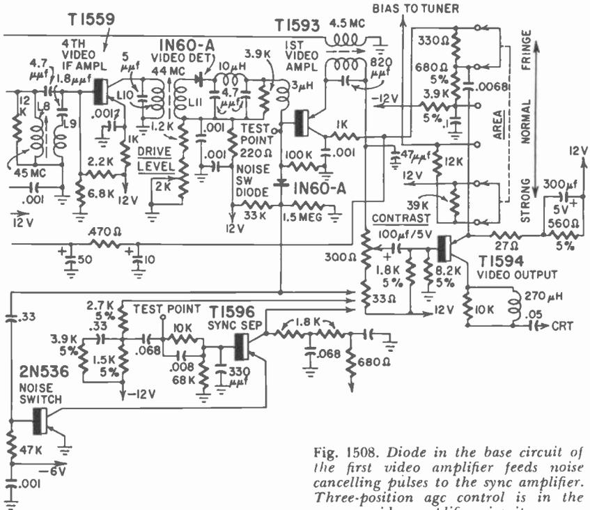
Fig. 1508. Diode in the base circuit of the first video amplifier feeds noise cancelling pulses to the sync amplifier. Three-position agc control is in the video amplifier circuit.
