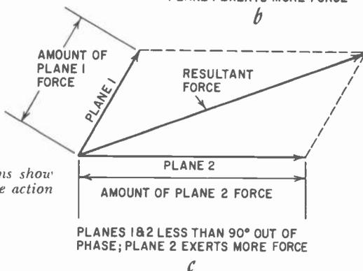
Fig. 1306. Vector diagrams show the resulting forces of the action in Fig. 1305.
