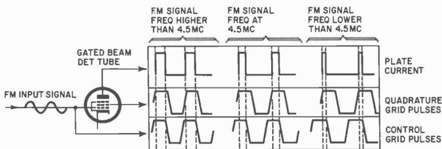
Fig. 1313. How the overlapping pulses on control and quadrature grids gate current through the gated-beam detector tube. Dashed lines show overlap (coincident) periods when the FM signal is higher, at, and below 4.5 mc.
