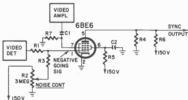
Fig. 1007. Pentagrid sync separator designed to squelch noise pulses that trigger the sweep oscillators.
