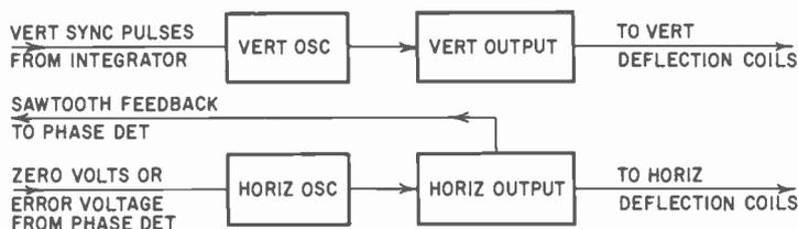
Fig. 1101. Block diagram of the horizontal and vertical sweep sections of a TV receiver.
