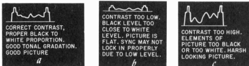
Fig. 806. (a) *Correctly proportioned video signal—pleasing picture.* (b) *Incorrectly proportioned signal—picture has too little contrast.* (c) *Incorrectly proportioned signal—contrast too strong.*
