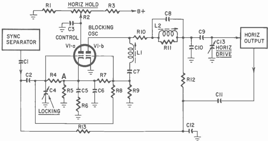
Fig. 1015. Circuit diagram of Synchroguide afc system. V1-a is the control tube; V1-b the blocking oscillator.
