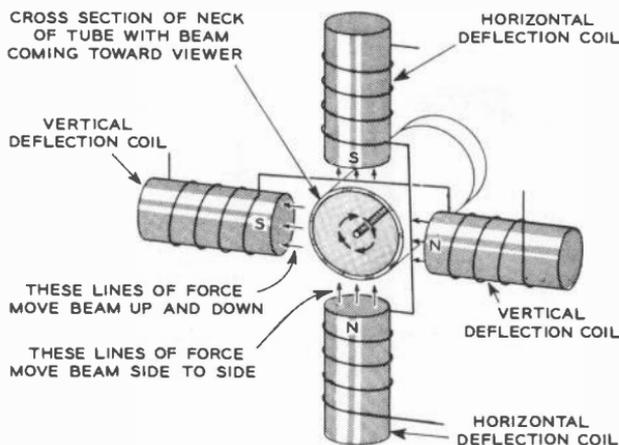
Fig. 205. Descriptive view of the horizontal and vertical deflection coils and the forces they generate.
