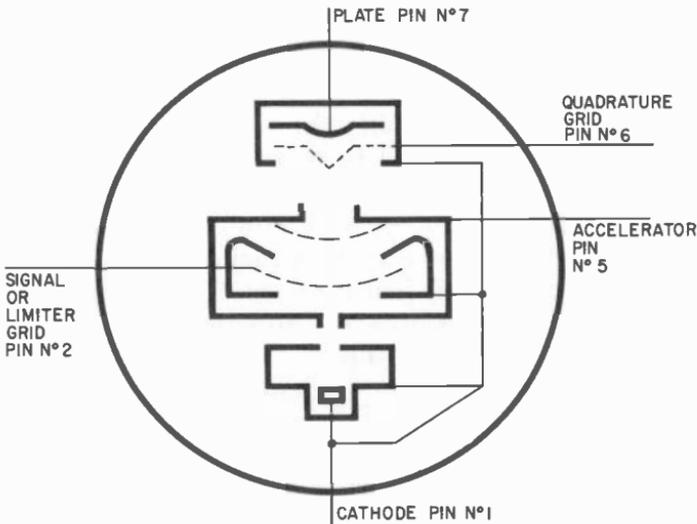
Fig. 1311. Internal placement of elements in a gated-beam detector tube.
