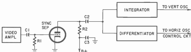
Fig. 1006. This circuit diagram shows how the sync separator feeds the sync component of the composite video signal to the integrator and differentiator circuits.
