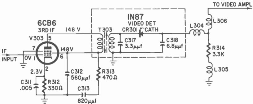
Fig. 703. Schematic of typical video detector showing coupling circuitry between third video if and video amplifier. Parts inside the box are contained in a shield can.
