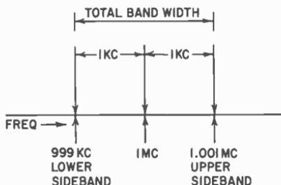
Fig. 309. 1-mc carrier amplitude-modulated by a 1,000-cycle tone. Illustration shows points where upper and lower sidebands appear.
