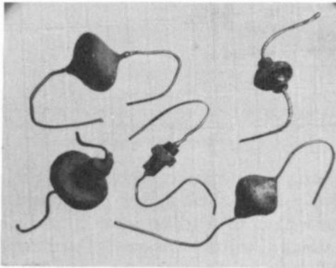
Fig. 702. Peaking coils have many forms. Some are encapsulated or dipped in moisture-excluding compounds.
