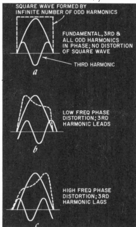
Fig. 805. (a) Square wave formed by odd harmonics of sine wave. (b) Resultant distorted wave when harmonics are phase-shifted. (c) Broken line shows high-frequency phase distortion.
