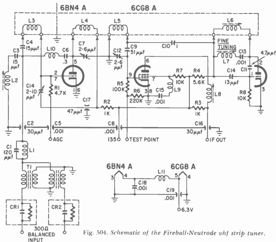
Fig. 504. Schematic of the Fireball-Neutrode vhf strip tuner.
