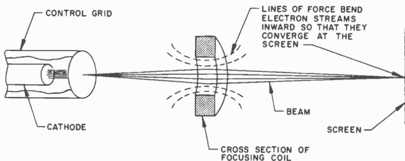
Fig. 208. *Focusing by magnetic lines of force.*
