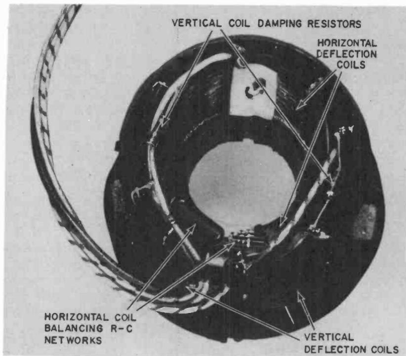
Fig. 206. *Internal construction of a typical deflection yoke.*
