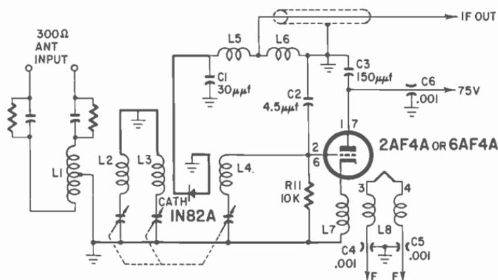
Fig. 510. Schematic of "Piggyback" uhf tuner. The entire unit is a high-frequency oscillator and a crystal mixer.
