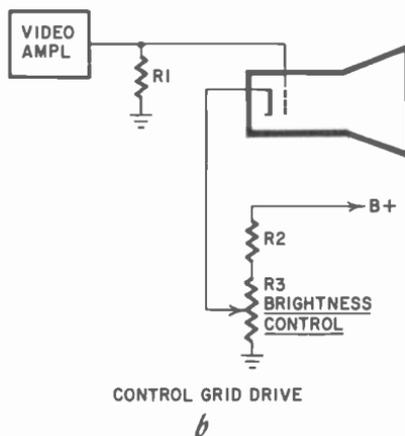
Fig. 807. Two methods of coupling video amplifier to picture tube. In both cases, brightness control arrangement remains the same.
