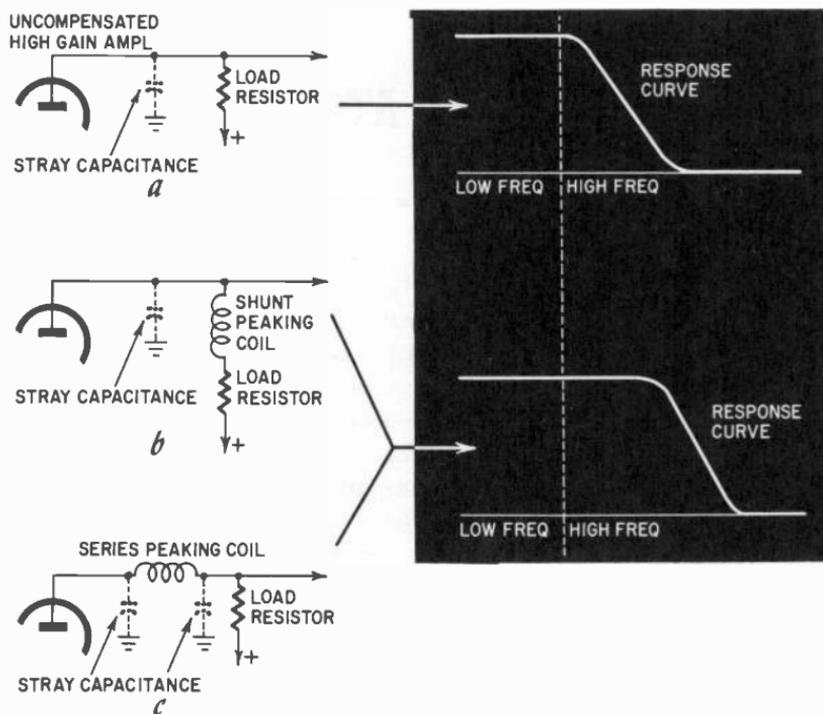
Fig. 801. Some methods used to broaden the response of a video amplifier. (a) Stray capacitance (dashed lines) of an uncompensated high-gain amplifier destroys high-frequency response. (b) Shunt peaking-coil hookup. (c) Series peaking-coil hookup.
