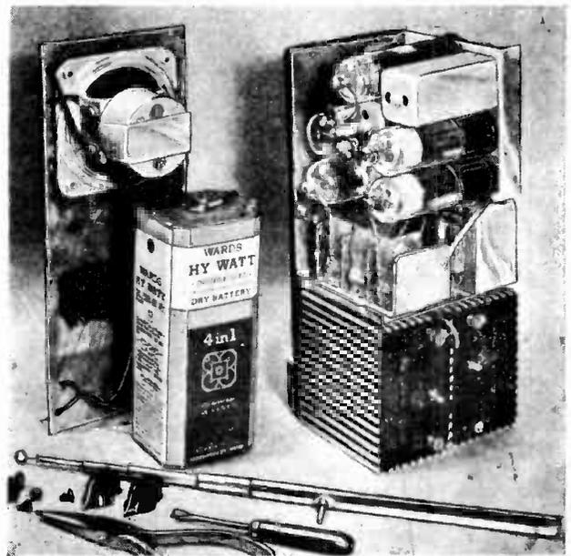
Fig. A. The "innards" of the Lunchbox Portable. One No. 6 dry-cell will run the set for months. Note the P.-M. dynamic speaker above the cell; and note the telescoping fishpole-type antenna which plugs into the front panel and extends to 45 ins.
