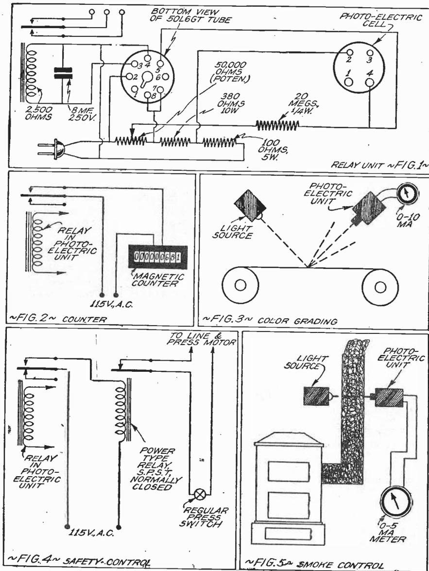
using the meter as for grading will register the relative density of the smoke passing through the chimney breach.
