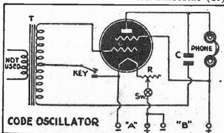
may be any available of about 30 ohms resistance and is used to drop the "A" battery voltage to the required tube filament voltage. The "on and off" switch (Sw) may be on the rheostat or it may be separately mounted. In most cases the phones may be substituted by a P.M. speaker with a suitable speaker transformer. The key is placed as it is in the circuit to eliminate "key-clicks."
