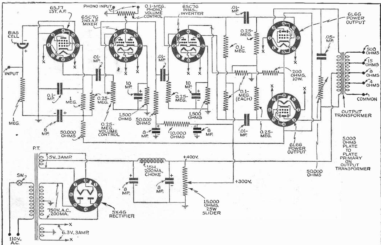
Considering the number of condensers used in isolating circuits from each other, the underchassis wiring is clear and uncomplicated. Resistance-capacity networks are inserted not only in the pre-amplifier plate circuit, but also in the high-voltage lead to the inverter stage. These working in conjunction with the "balanced" inverter circuit, produce an amplifier with remarkable stability.
