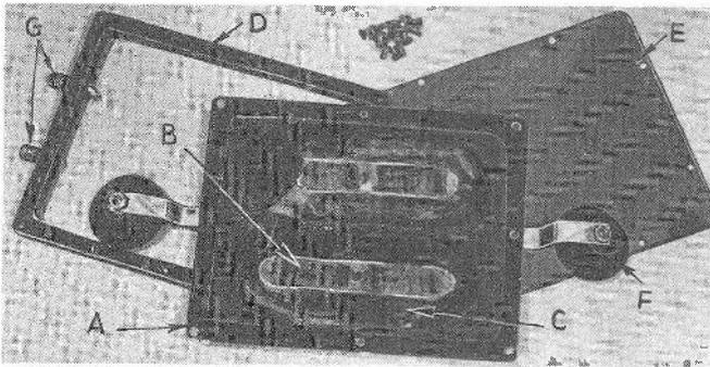
Fig. A. Exploded view of the pickup; A, brass plate; B, saw blade core; C, winding; D, frame; E, fibre back; F, action cup mounts; G, terminal posts. Note the insulating compound.
