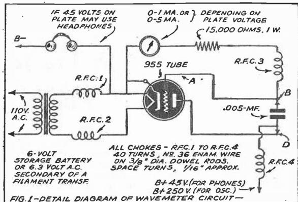
FIG. 1 - DETAIL DIAGRAM OF WAVEMETER CIRCUIT -
