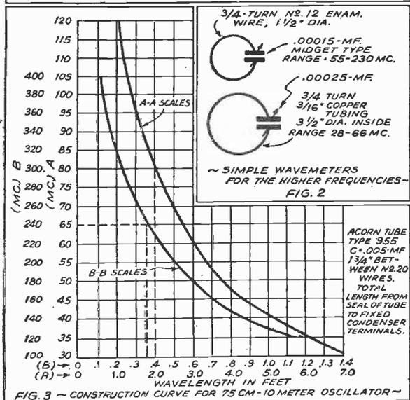
FIG. 3 - CONSTRUCTION CURVE FOR 75 CM.-10 METER OSCILLATOR -
