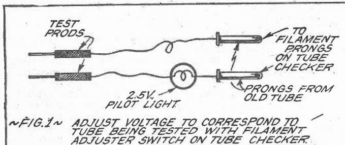
~FIG. 1~ ADJUST VOLTAGE TO CORRESPOND TO TUBE BEING TESTED WITH FILAMENT ADJUSTER SWITCH ON TUBE CHECKER.
