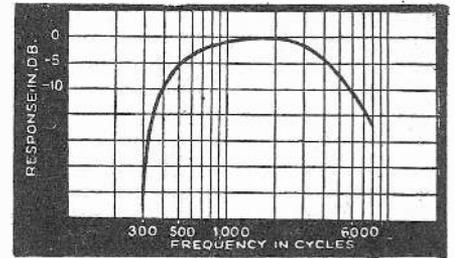
Fig. 2. Frequency characteristic of equipment used in the Robeson Technique. Only "significant" frequencies are fed back to the performer. The selected frequency band constitutes a highly directional beam, at an optimum intensity level, which only the performer can hear.
