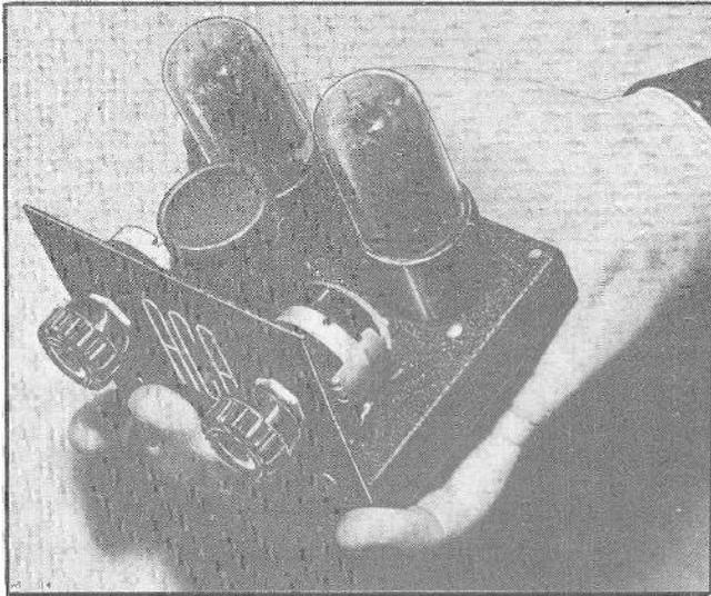
Here is a 2-Tube, Low-Power, Multi-Use Amplifier admirably adapted for low-level, high-fidelity phonograph reproduction, and for radio (receiver output) amplification.
