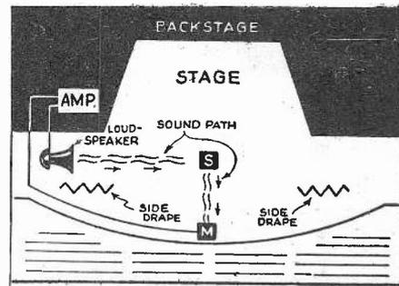
Fig. 1. Diagram showing instrument placement on concert stage for Robeson Technique. The letter S indicates the position of the singer; M represents the microphone (located in the footlights trench).
