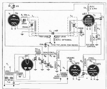
cycles. The link circuit is broken on one side and brought out to pin tip jacks. The tuned circuit is connected to a 6B7 pentode section. The output of the pentode section is rectified in the diode section and the negative potential developed is applied to
