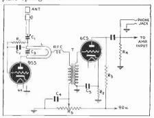
Fig. 2-Receiving unit of the relay system.
