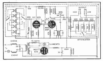
For audio oscillator I used a small interstage 1-3 transformer parallel-fed to triode section of 6K8. Checking with an oscilloscope, almost perfect wave form was found at 400 cycles with depth of 30%. The attenuator was governed by values on hand and works quite well.
