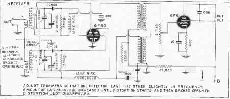
Fig. 3—Complete diagram of the 2-tube FM receiver, with 1-stage audio for headpnones.
