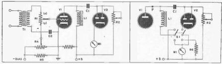
Figs. I and 2—Basic circuit of the simple transconductance tester described in this article.
