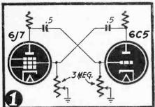
Fig. I-Fundamental circuit of the device.
