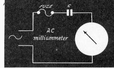
Fig. 4—A.C. milliammeter as capacity meter.
