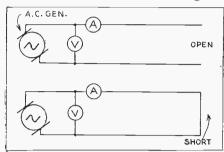
Fig. 2—How the characteristic impedance of an alternating-current transmission line is arrived at.
