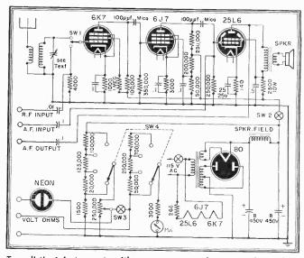
Two distinct instruments with one power supply are combined here.
