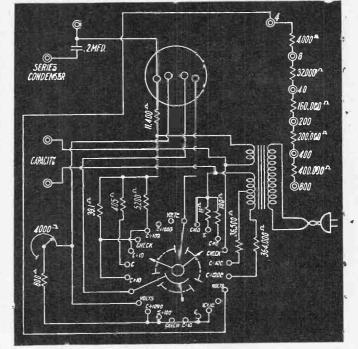
Fig. 7-The Weston 664, a wide-range commercial capacitance meter.
