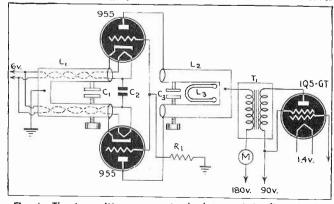
Fig. I—The transmitter uses a standard transmission-line circuit
