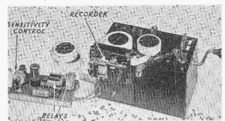
The code recorder together with its amplifier and two rolls of tape.
