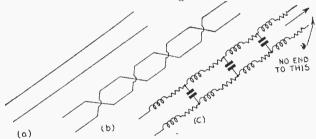
Fig. I—At (a) we have a standard radio transmission line, and at (b) the same line as it often appears in practice with transpositions (c) shows how such an "infinite" line looks to the radio-frequency currents flowing through it.
