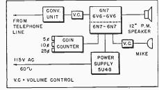
Fig. 7-Block diagram of the remote receiver.
