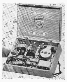
Layout of the three-tube broadcast receiver.
