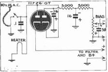
3-One 117Z6-G used to supply high and bias voltages for receiver or amplifier.
