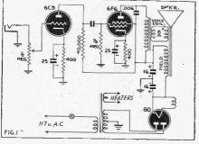
Fig. I-The common power amplifier circuit.
