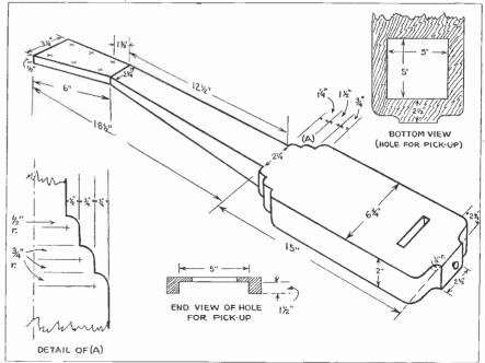
Construction of the guitar body. This should be a simple matter for any handy workman, but it is worth noting that the impression made by the instrument will depend almost as much on its appearance as sound.
