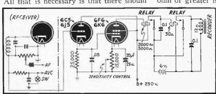
Fig. 1, above—The amplifier circuit, to the right of dashed line. Right--Clearer detail on the recording unit and pen-holding device.
