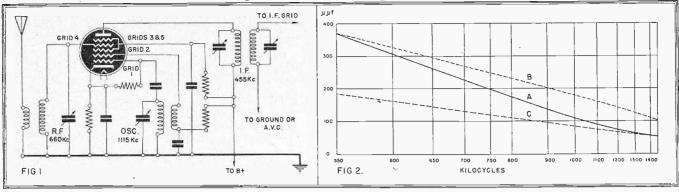
Fig. I-Mixer stage of simple superheterodyne
