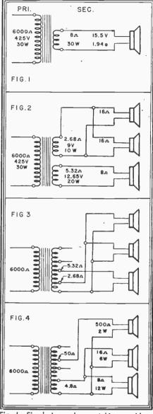
Fig. I—Simplest speaker matching problem. Fig. 2—How three speakers could be matched. Fig. 3—All three on one output transformer. Fig. 4—Matching widely different speakers.
