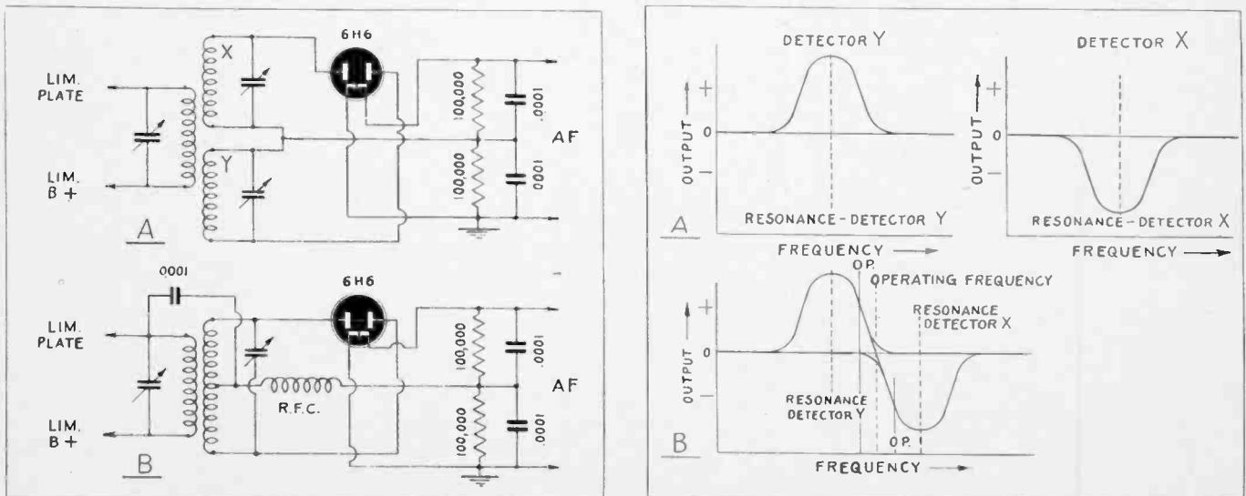
Fig. 1, left—Two fundamental FM discriminator circuits. The system at B is the one now most commonly used in commercial FM receivers. Fig. 2, right—How the two separate AM detectors of Fig. 1-A can be made to operate as a discriminator for detection of FM signals.
