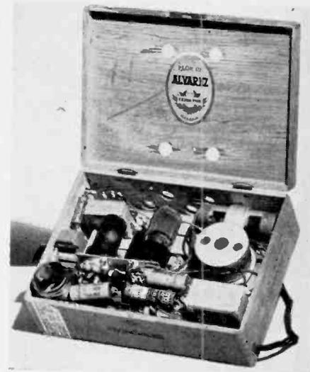
Layout of the three-tube broadcast receiver.
