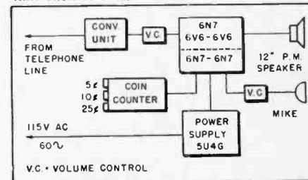
Fig. 7—Block diagram of the remote receiver.
