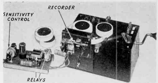
The code recorder together with its amplifier and two rolls of tape.
