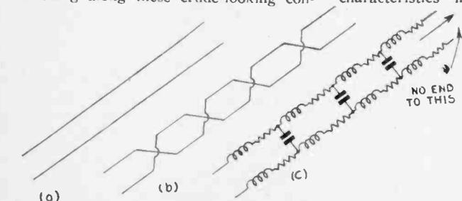
Fig. 1.—(a) At (a) we have a standard radio transmission line, and at (b) the same line as it often appears in practice with transpositions; (c) shows how such an "infinite" line looks to the radio-frequency currents flowing through it.
