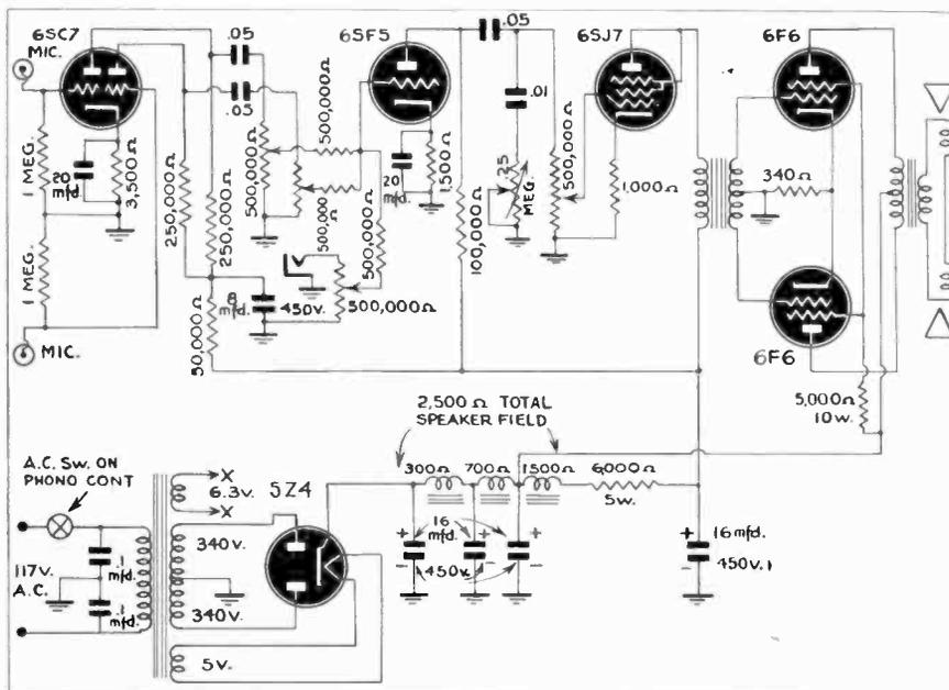
The guitar amplifier. Microphone as well as instrument pick-up is provided, and the inputs can be mixed. The filter system is unusually thorough, obviating both hum and feedback. Note the two loudspeakers.
