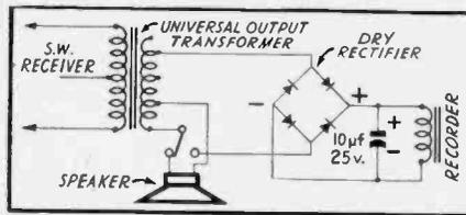
Fig. 2—Hookup for recording from receiver
