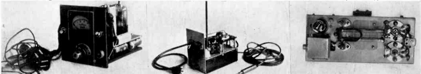
Complete radio P. A. system. Left—Speech amplifier; center—receiver; right—transmitter.
