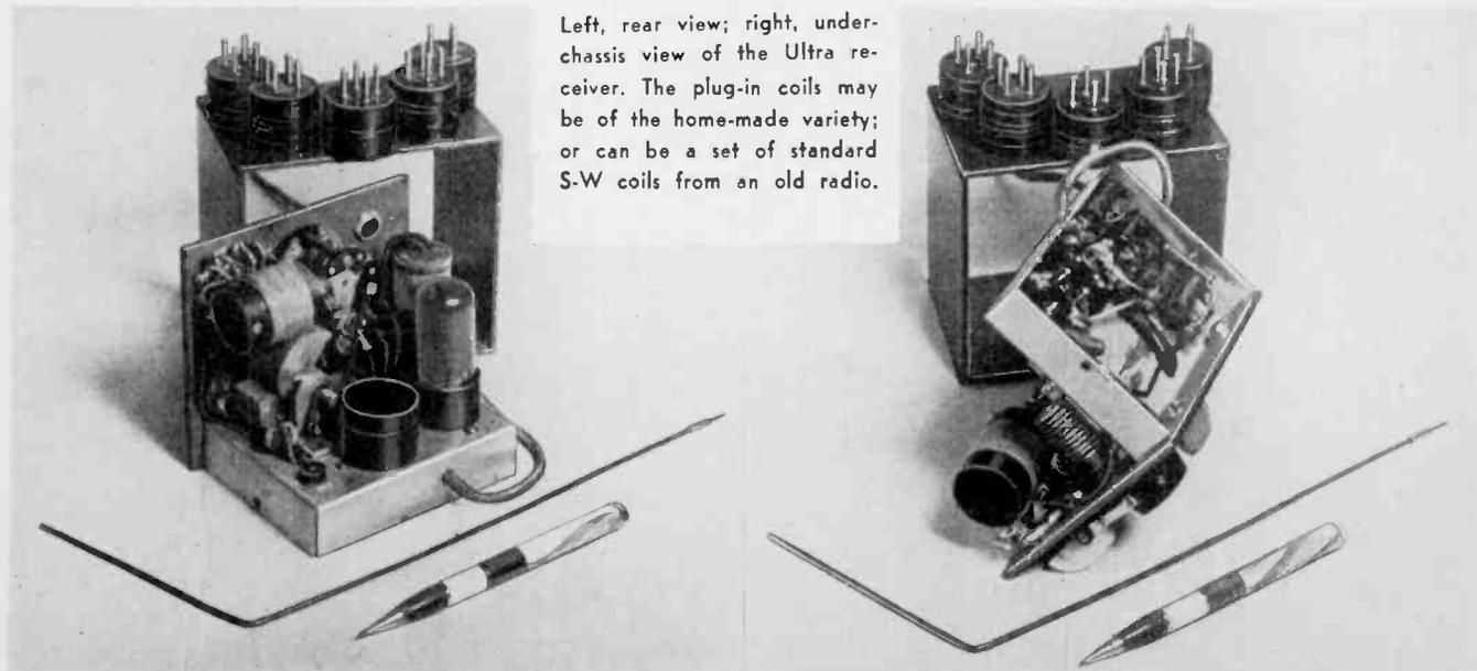
Left, rear view; right, under-chassis view of the Ultra receiver. The plug-in coils may be of the home-made variety; or can be a set of standard S-W coils from an old radio.
