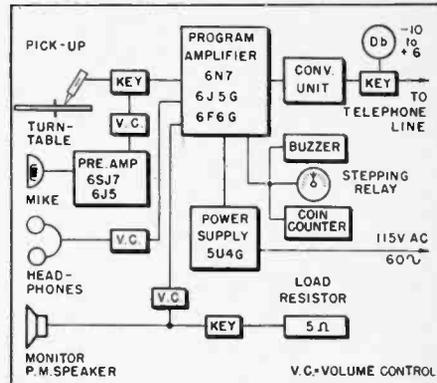
Fig. 6—Rough diagram of the Central Station.
