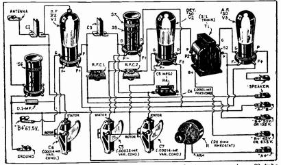
Pictorial Diagram Showing Placement of Parts. R. F. stage uses a type 32 tube.
