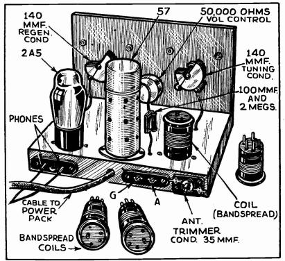
Rear View of the Bandspread "Doerle" Receiver.
