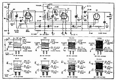
Schematic Diagram and Coil-Winding Data.
