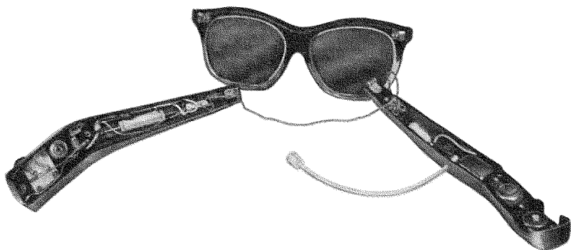
Fig. 312. Complete radio in eyeglass frame utilizes many hearing-aid principles.
