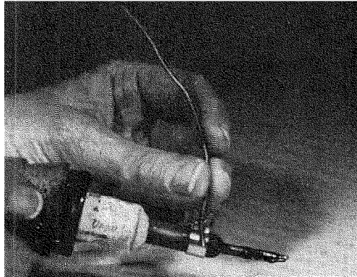
Fig. 718. Adapter type heat-stripper can be mounted permanently on the soldering iron.
