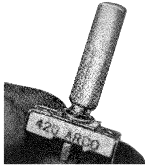
Fig. 217. Shafts can be added to many types of miniature adjustable components. Avoid heat whenever possible. Various cements can be used to do the job solder might be selected for. Use them sparingly and carefully.
