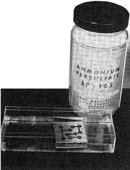
Fig. 405. Etching solution is made from powder dissolved in warm (105°F to 140°F) water. When etching, solution should be between 65°F and 70°F. Solution is good for about a week, so don't make any more than you expect to use in that time. Use non-metallic containers.
