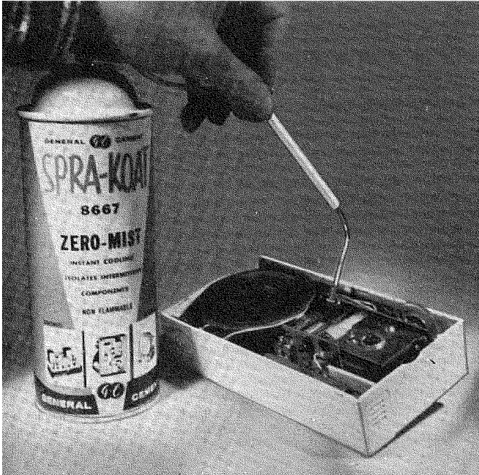
Fig. 716. Freon aerosol dispenser helps pinpoint temperature-sensitive components.
