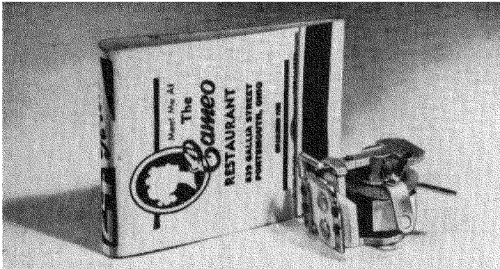
Fig. 224. The small coil of this relay draws only about one milliamper. The wire-like contacts can handle about 200 ma.
