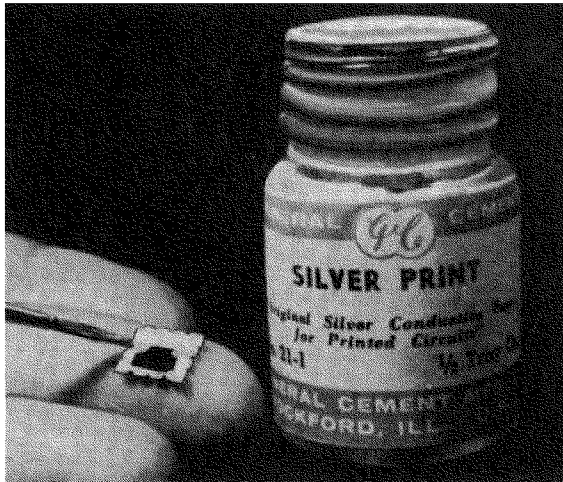
Fig. 203. Conducting paints are used to connect resistive coatings to the wafer terminals.
