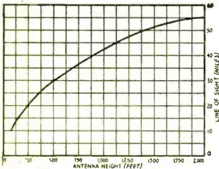
Fig. 1—Antenna height for given radio range.
