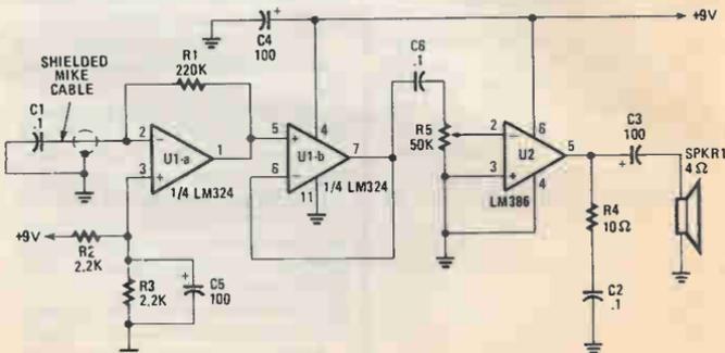
Fig. 1. Our drum simulator uses a capacitor to detect the tapping of the stick. The detected signal is then amplified, conditioned, and used to drive a 4-ohm speaker.
