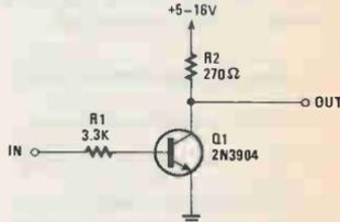
Fig. 9. This simple inverting amplifier, built around discrete components, can be driven from most CMOS or TTL IC's.
