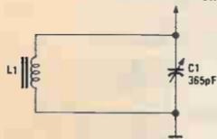
Fig. 4. The Signal Scrubber is a frequency-selective circuit for the wire stretcher. When a desired signal is receivable, but buried in noise, this circuit can pull it out of the mud, clean it up, and send it on to the receiver.
