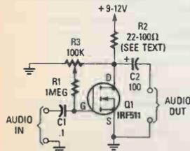
Fig. 1. In this circuit the IRF511 is configured as a class A amplifier. Ideally, for class-A operation, the voltage across Q1 and the load resistor should be equal.
