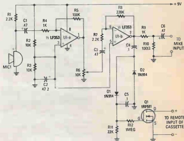
Fig. 7. The electret microphone MIC1 picks up the sound and feeds the signal to a two-stage amplifier circuit, consisting of U1-a and U1-b, the output of which is fed to a voltage-doubler circuit (made up of D1, D2, C4, and C5).
