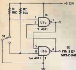
Fig. 6. This bounce-free switch circuit can be connected to the timer circuit. Pressing S1 clears and resets the timer circuit.
