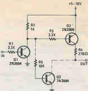
Fig. 10. The non-integrated buffer, like its integrated counterparts, can be used to increase the output drive current.
