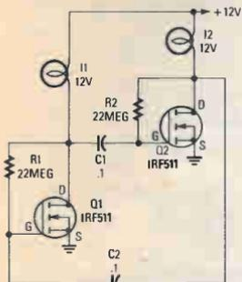
Fig. 4. In this circuit, two hexFET's are configured as a simple astable multivibrator to alternately switch the two lamps, I1 and I2, on and off.
