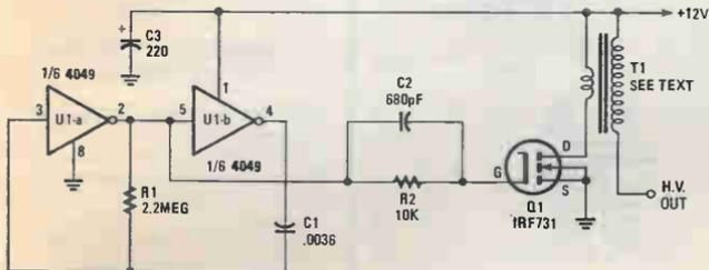
Fig. 8. In this circuit, an IRF731 hexFET and two gates of a 4049 hex inverting buffer are configured as a square-wave-generator circuit, with Q1 operating as a switch.
