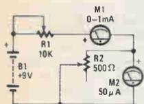
Fig. 3. If your most accurate measuring instrument is a current meter that can monitor 1-mA, use this circuit to determine R3's value.
