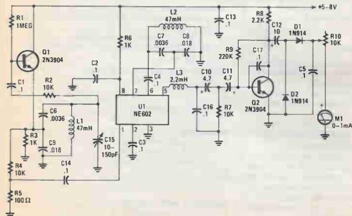
Fig. 3. The NE602 is the heart of the permanent magnet detector. By bringing a magnet close to either L1 or L2, the circuit will respond by producing a meter reading, indicating the relative field strength of the magnet.
