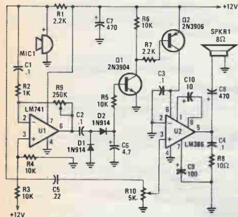
Fig. 1. The one-way intercom uses an omnidirectional electret microphone to pick up sound and convert it to an electrical signal. The resulting signal is used to activate the audio amplifier (U2) that drives the speaker (SPKR1), and is also the audio signal that is output by the speaker.
