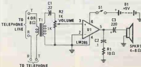
Fig. 3. This simple telephone amplifier circuit (which can be switched off for privacy) allows everyone in the room to listen in on your telephone conversations.
