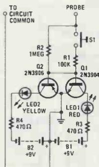
Fig. 3. The AC/DC Indicator can help you in your electronics lab by distinguishing between AC and DC signals, and more.
