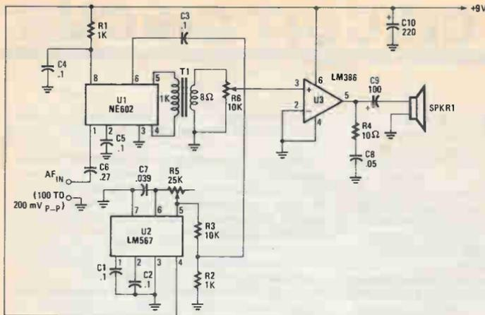
Fig. 2. In this single-mode inversion voice scrambler/decrambler circuit, the NE602 is configured as a balanced modulator/demodulator.
