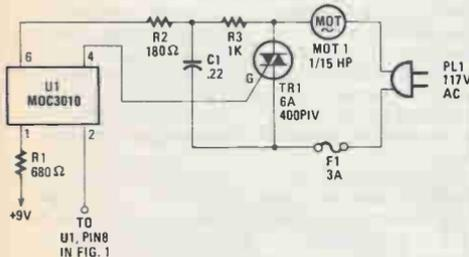
Fig. 2. The Triac Driver can be added to the proximity switch to control a small AC motor.
