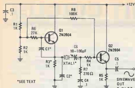
Fig. 2. Built around two general-purpose transistors, this oscillator produces a sine-wave output of from 2 to 6 volts peak-to-peak.
