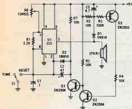
Fig. 1. This time-out circuit differs from conventional 555-timer applications in that this circuit has the 555 configured in the astable mode as opposed to the monostable, or one-shot mode.
