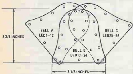
Fig. 2. The 36 LED's of the bell animation circuit are grouped by 12 and arranged to form three bell outlines. Here is the layout of the basic overlapping three-bell outline.
