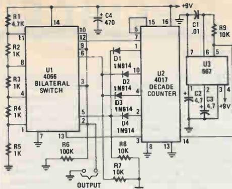
Fig. 4. In the Waveform Generator, the 4066 (U1) is used to perform sequential switching to produce a symmetrical stepped waveform.
