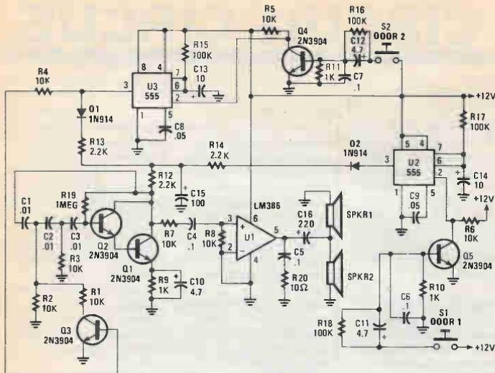
Fig. 2. This expandable two-door annunciator circuit (built around three IC's, five transistors, and a few support components) provides two distinctively different tones, so that you can tell which door to answer.
