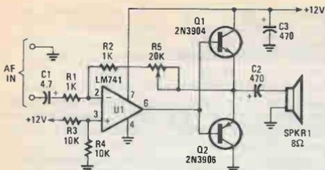
Fig. 3. This simple audio-power amplifier can be added to an existing project or incorporated in a future one.
