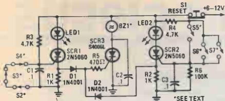
Fig. 5. The High-Power Alarm Driver uses the low-powered SCR's from the circuit in Fig. 4 to control a higher power SCR, which can then be used to turn on a hefty sounder.
