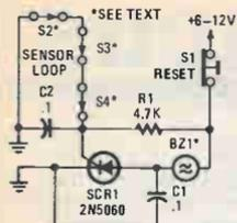
Fig. 2. The Closed-Loop Alarm uses a string of three series-connected normally closed switches (the closed-loop configuration) connected to the gate of an SCR.
