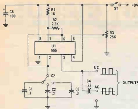
Fig. 2. Built around a 555 oscillator/timer, this audio-frequency, square-wave generator makes an inexpensive addition to your electronics workbench.
