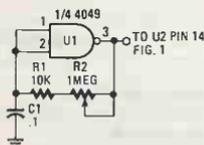
Fig. 2. The staircase generator can easily be converted into a self-generating circuit by reconfiguring U1 to conform to this schematic diagram, and then feeding its output to pin 14 of U2 in Fig. 1.
