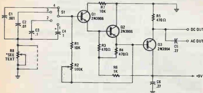
Fig. 1. The variable-frequency pulse generator produces narrow 7-volt positive-going pulses and has a frequency range of 2 Hz to over 50 kHz.
