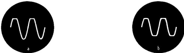
Fig. 1104. *Typical distorted waveforms. Note waveform a is clipped at top while waveform b is clipped top and bottom.*
