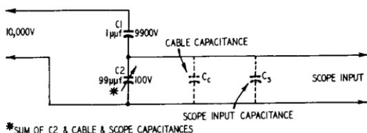
Fig. 607. Circuit showing voltage divider action of probe.
