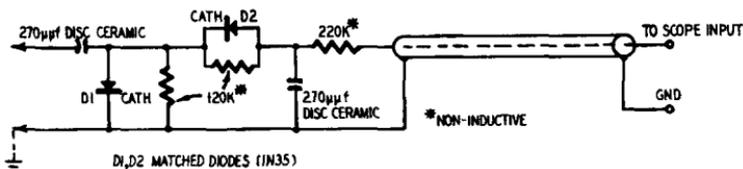
Fig. 301. Circuit diagram of voltage-doubler demodulator probe. This probe uses a pair of matched crystal diodes.
