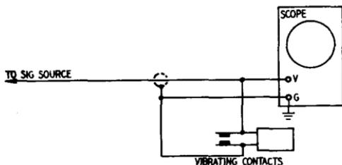
Fig. 409. Vibrating contacts intermittently short the vertical input of the scope.
