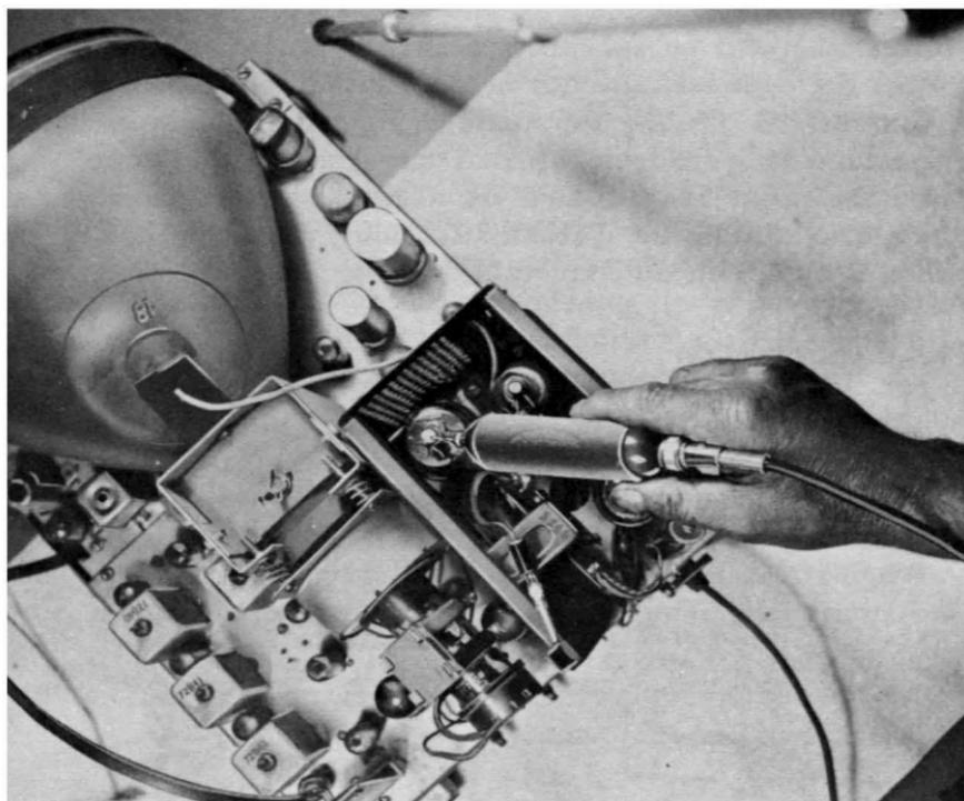
Fig. 602. Photo shows capacitance-divider probe being used to check high voltage waveforms.
