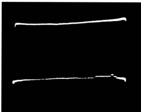
*Fig. 405. Curvature in the zero-volt reference line, sometimes noted during impedance checks of lead-ins and antennas, or front ends of TV receivers, is caused by 60-cycle pickup in the balanced crystal probe. Grounds should all be returned to a common point, and thence to a cold-water pipe. Ground all instrument cases.*
