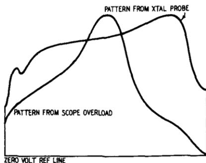
Fig. 218. Patterns obtained from crystal probe and from overloaded scope.
