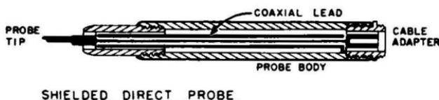
Fig. 709. Cross-sectional view of a shielded, direct probe.
