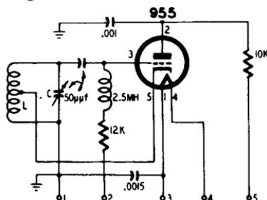
Fig. 1011. Circuit diagram of the grid-dip probe.
