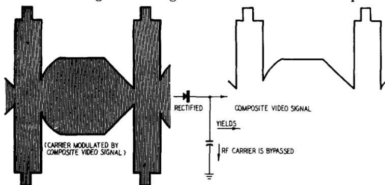
Fig. 201. The crystal in the probe removes one-half of the entire signal, consisting of the modulating signal and the r.f. carrier. The carrier is bypassed by the capacitor. The output is the original modulation voltage.
