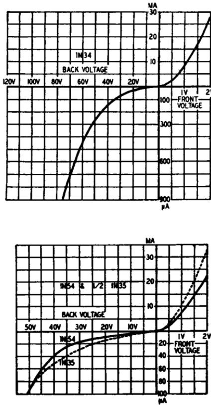
Fig. 213. Voltage-current relationships of three germanium crystal diodes.
