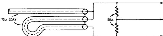
Fig. 419. The coaxial balun is simply cable bent back on itself as shown, and connected to the output cable of the generator. The balun gives a 4:1 impedance match.
