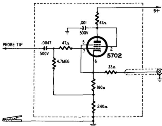
Fig. 824. Circuit diagram of the cathode-follower probe.
