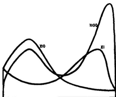
*Fig. 217. Example of attenuator resonances and partial rectification of r.f. signal by the vertical amplifier of a scope.*
