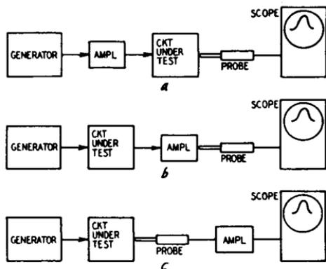
Fig. 923-a,-b,-c. In the drawings above we have three possible arrangements of the Chromatic Amplifier.
