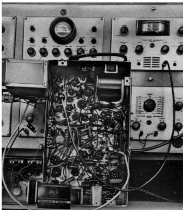
*Fig. 207. Visual alignment setup of a TV receiver. Improper impedance matching between test equipment and receiver can cause changes in the observed scope pattern when you touch the signal-generator cable.*
