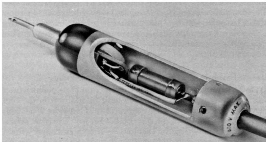
*Fig. 507. Cut-away view of the interior of a low-capacitance probe showing placement of parts.*
