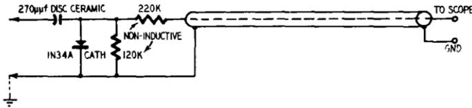
Fig. 103. Circuit of signal tracing demodulator probe.
