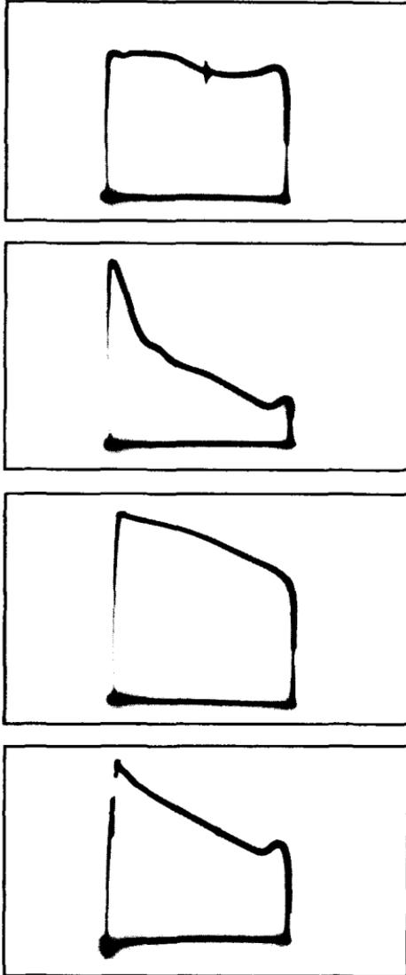
*Fig. 410. When an unsuitable demodulator probe is used to test the output from a sweep-frequency oscillator, or when the instrument is operating incorrectly, or if test conditions are unsuitable, typical patterns such as these will be observed as the instrument is tuned through its range.*
