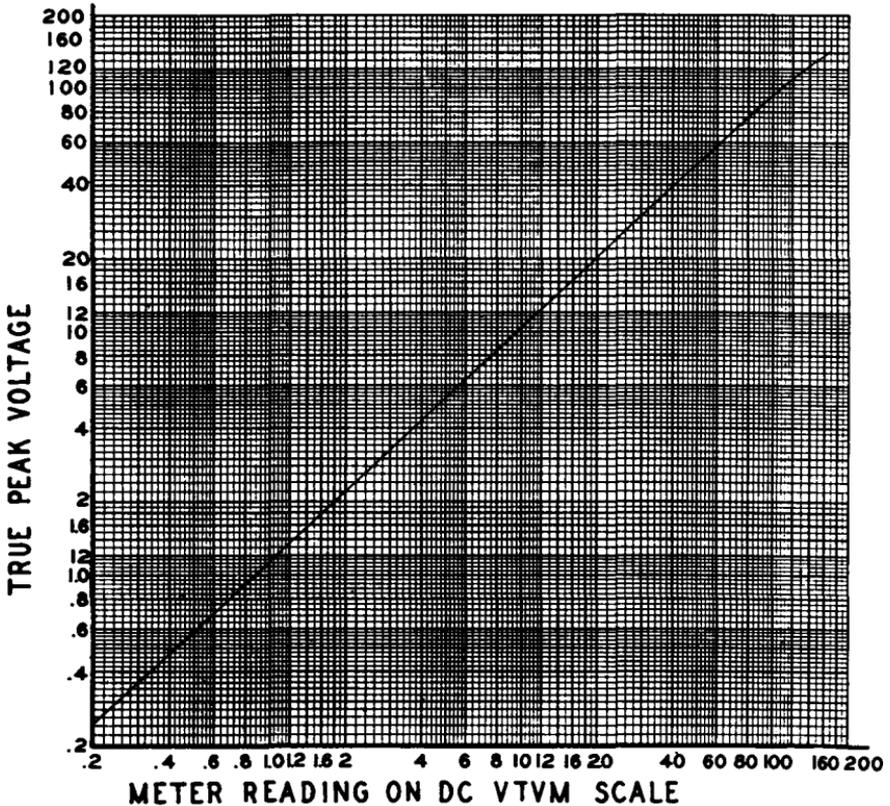
Fig. 1003. Graph shows relationship between peak voltage at test point and meter reading on your v.t.v.m.
