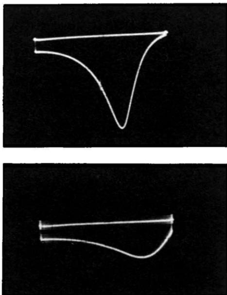
Fig. 220. Illustration at the top shows normal response curve. In the lower picture we see how the curve changes shape when sweep-generator tuning dial is touched.
