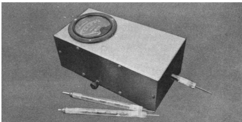
*Fig. 813. Photo of the trim-looking unit and the associated plug-in multiplier probes. The positioning of the meter is not critical and may be turned to suit your convenience. An inexpensive 0-1 ma meter is used.*
