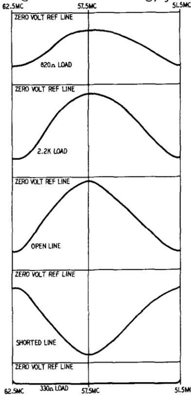
Fig. 403. The margin by which the standing wave pattern fails to contact the reference line measures the loss in the transmission line.
