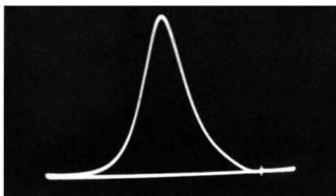
*Fig. 206. Sweep-signal trace produced in the output stages of an i.f. amplifier.*
