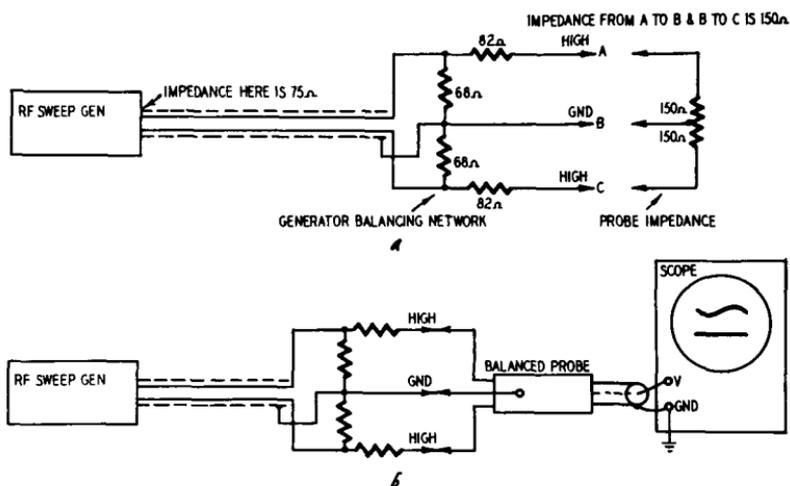
Fig. 407-a,-b. The balanced probe has a 300 ohm input, 75 ohm output. Since sweep generators have a 75 ohm output, a generator balancing network is needed to match the generator to the probe. This is shown in a, above. The technique for connecting the scope, balanced probe, matching network, and sweep generator is shown in the lower illustration, b.
