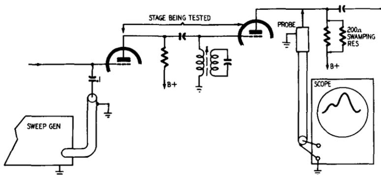
Fig. 211. Circuit diagram shows the use of a 200-ohm swamping resistor shunted across the plate load.
