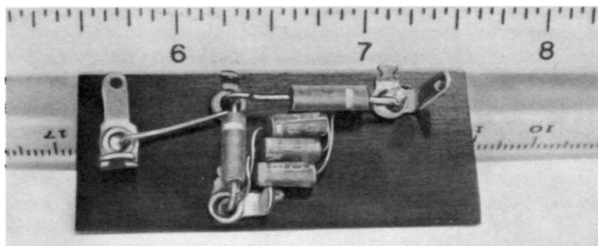
Fig. 902. Internal layout of the Chromatic Probe. The three crystals form a non-linear network. The output of the probe is the difference between the two signals that are applied to the probe input.
