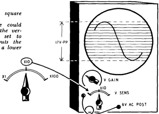
terminal. Advance the vertical gain control (vertical attenuator) until the sine waveform on the screen occupies 17 squares. Each square then represents 1 peak-to-peak volt.
