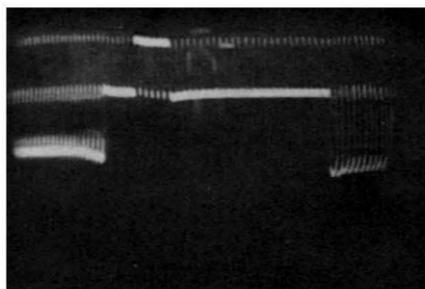
*Fig. 108. The vertical-blanking interval of Fig. 106 shown in greater detail.*
