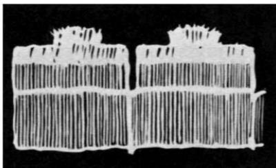
Fig. 519. *A correctly adjusted probe will produce this waveform.*
