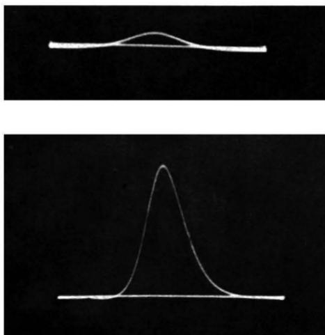
*Fig. 210. When using a crystal probe to trace a sweep signal through the i.f. amplifier, the pattern height increases from stage to stage, as shown above. The example shown indicates a gain of 10 which is typical for a conventional receiver.*
