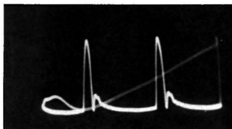
*Fig. 609. Normal sweep waveform at the plate of horizontal-output tube, seen with the aid of a 100-to-1 capacitance-divider probe. Diagonal line is scope retrace. Peaks are about 6,000 volts high.*
