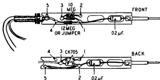
Fig. 303. Construction of a voltage-doubler probe. The parts are mounted on a terminal board. Front and back views are shown. The numbers, 1 to 5 inclusive, indicate connections made through brass soldering rivets.
