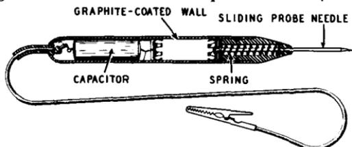
Fig. 804. *Cross-sectional view of capacitor-tester probe.*
