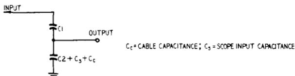
Fig. 608. Arrangement of various capacitances in the probe.
