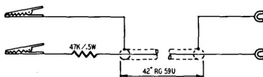
Fig. 704. Circuit of isolation probe for use with a scope. RG-62U has a smaller capacitance than the coaxial cable shown here.
