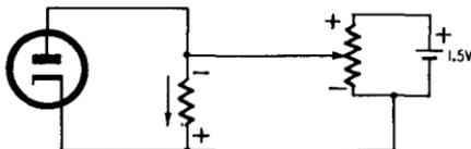
Fig. 1001. Basic circuit for overcoming the effect of contact potential.
