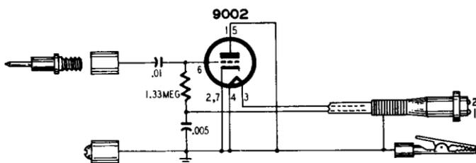
Fig. 1002. *Peak-indicating high-frequency probe (r.f. probe).
