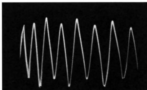
*Fig. 613. The voltage of successive peaks is not the same. This symptom is caused by the presence of a spurious low-frequency voltage in the circuit under test.*
