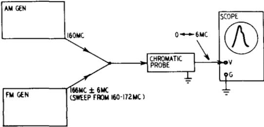
Fig. 904. To obtain a response curve in standard form it is necessary to develop one video sweep in each 1/120 second.
