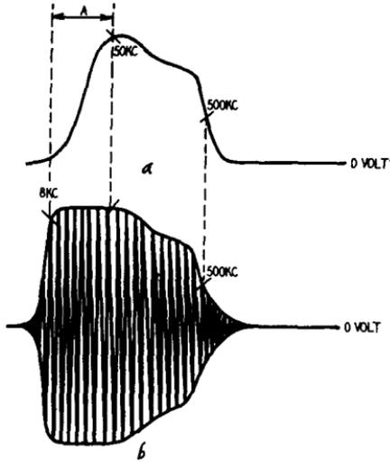
Fig. 915-a-b. Response curves: a, using demodulator probe; b, using low-capacitance probe. "A" is the area of low-frequency attenuation.
