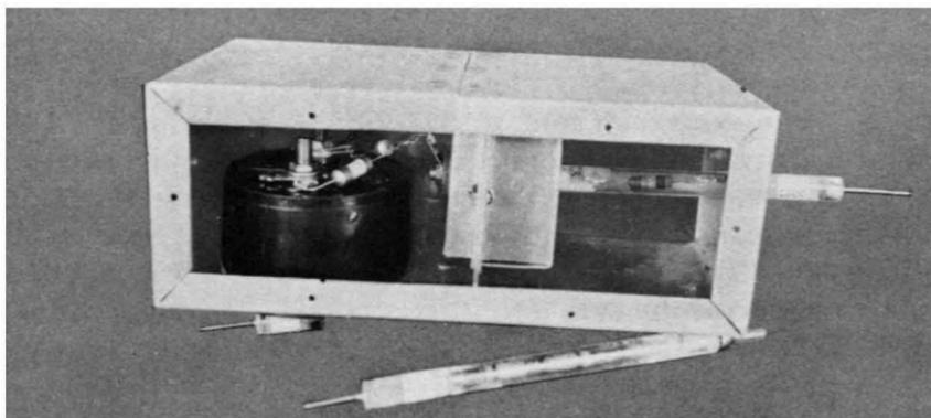
*Fig. 814. View of the inner construction showing placement of the components. The metal box consists of two shielded compartments. Both sides of the metal housing are held in place by self-tapping screws. The entire probe is readily accessible for any repairs or changes you might wish to make.*
