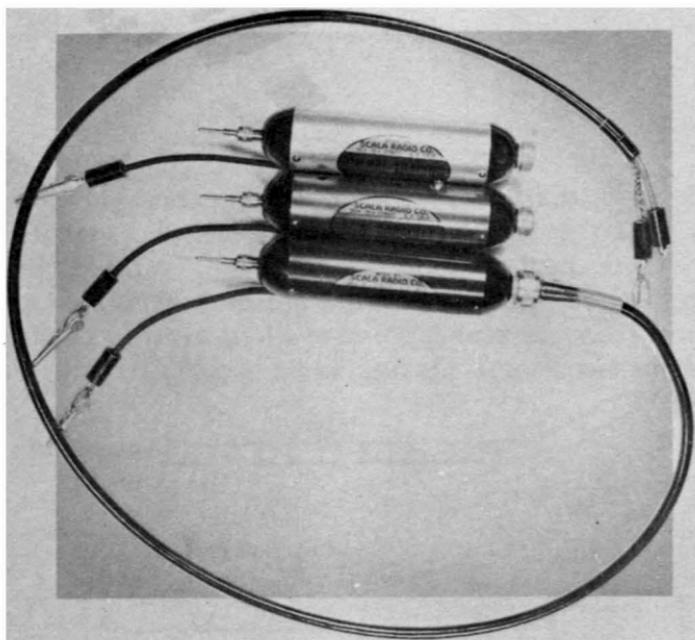
Fig. 305. Three types of scope probes used in TV test work. (Top) Crystal-demodulator signal-tracing probe; (center) low-capacitance high-impedance 10-1 voltage-divider probe; (bottom) 100-1 capacitance-divider high-voltage probe.
