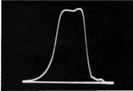
Fig. 909. Actual response curve in chrominance amplifier output circuit using Chromatic Probe.
