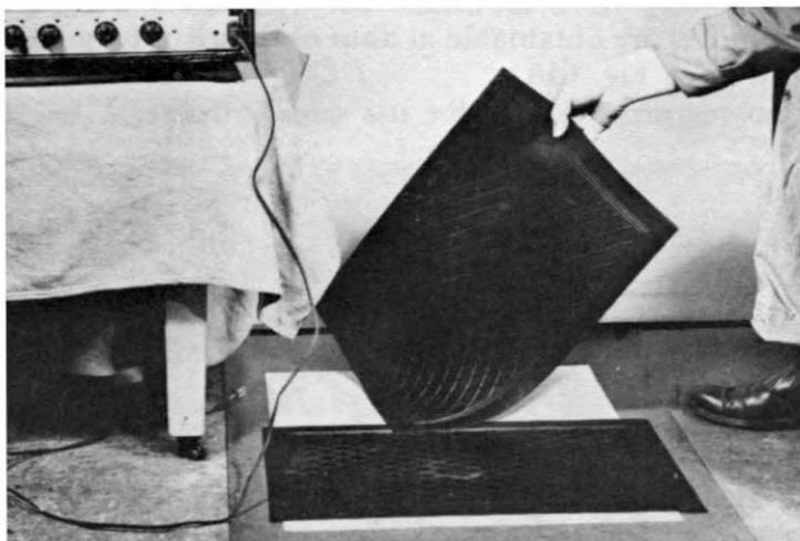
Fig. 618. A rubber mat is very inexpensive, high-voltage insurance.
