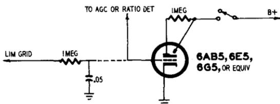
Fig. 818. Circuit diagram of magic-eye probe.
