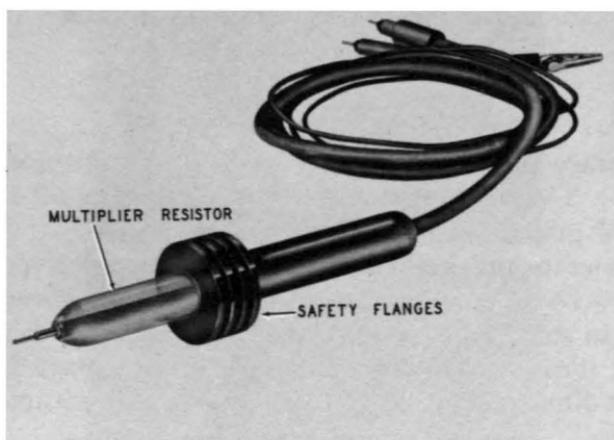
Fig. 615. Photo of typical high-voltage probe. Safety flanges present a long barrier to high voltage.
