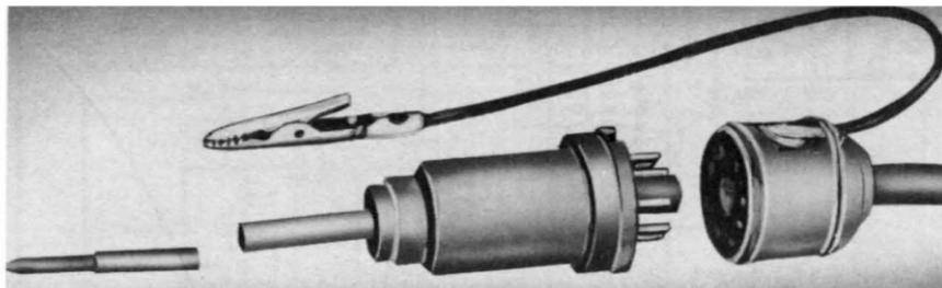
Fig. 1017. Photo of the vacuum-tube probe. The probe is very sensitive and can be used in very low r.f. signal voltage stages.
