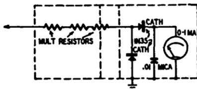
Fig. 815. Circuit diagram of the diode-type voltmeter.
