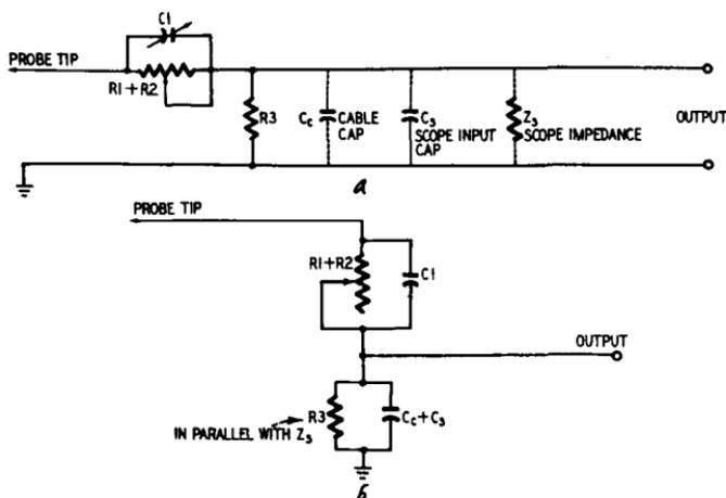
Fig. 502-a,b. Circuit factors involved in the design of a low-capacitance probe. The circuit, a, is rearranged as in b, to show divider action. See footnote for explanation of probe adjustment.
