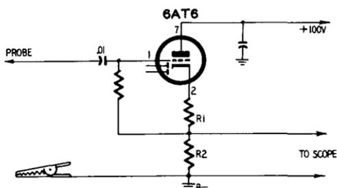
Fig. 1008. Circuit diagram of cathode-follower probe. The signal output is taken from across R2.
