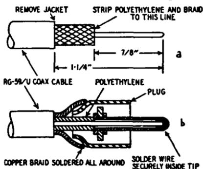
Fig. 821-a,-b. Illustration at top (a) shows preparation of coaxial cable while lower illustration (b) shows how to solder the cable to the plug.
