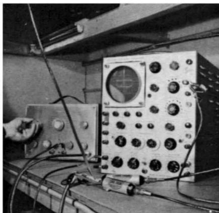
Fig. 412. Photo of test setup utilizing dual crystal probes instead of a balanced probe.
