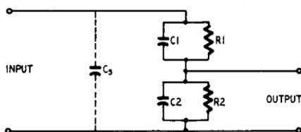
Fig. 805. *Electrical arrangement of the frequency-compensated probe.*
