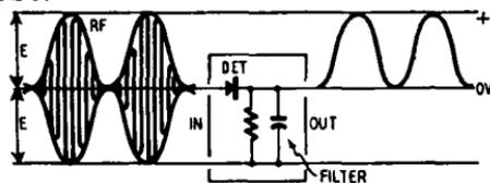
Fig. 101. A modulated wave can be rectified by a crystal-detector probe. The low-frequency wave can be seen on the scope.
