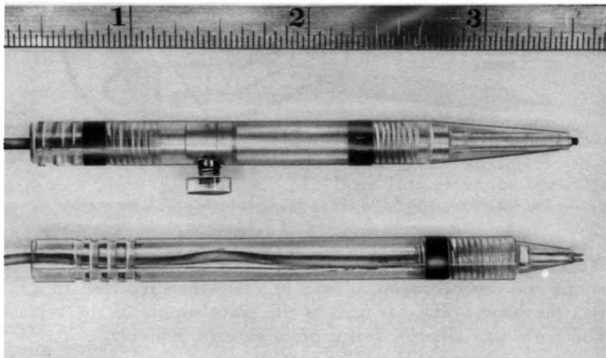
Fig. 810. Two types of miniature test probes. The ruler shown at the top of the photograph will give you some idea of the actual size of the probes.
