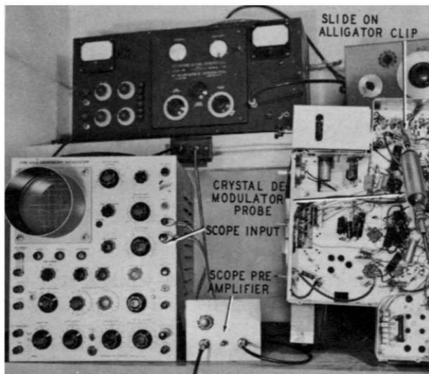
*Fig. 114. Even with high sensitivity lab scopes it is necessary to use a preamplifier when tracing weak signals in low level TV i.f. stages.*
