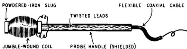
Fig. 802. This probe is very useful for tracking down sources of hum. Use any small diameter, insulated wire for the coil.
