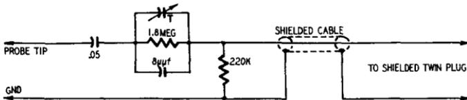
Fig. 504. The capacitor in series with the probe tip blocks d.c., permits passage of a.c. waveforms.
