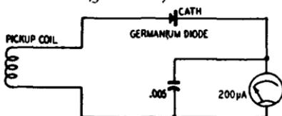
Fig. 812. R.f. detector probe circuit.
