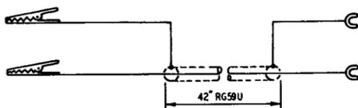
Fig. 710. A length of coaxial cable is easily converted into a direct probe.
