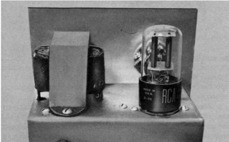
*Fig. 113. Top view of the preamplifier. Either an open- or shielded-type power transformer can be used. Amplifier uses but a single tube.*
