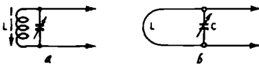
Fig. 805-a,b. Marker oscillator tank arrangements. Large inductors (a) may be trimmed by a slug or small inductors (b) may be formed like a hairpin with adjustable length.
