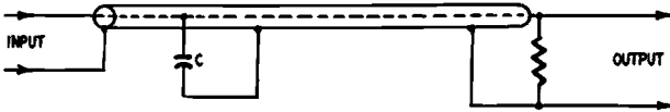
Fig. 309. The output of the generator should have a constant impedance to avoid reflections which cause lack of flatness. The capacitive reactance in the attenuator is represented here as a capacitor C shunted across an intermediate point of the cable.
