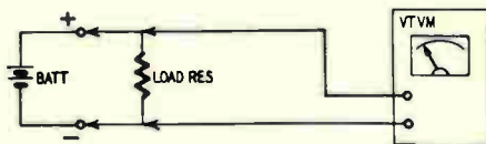
Fig. 1003. Method of testing battery voltage.
