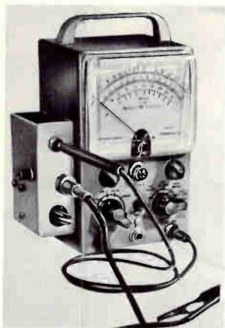
Fig. 1017. The preamplifier is attached to the case of the v.t.v.m.
