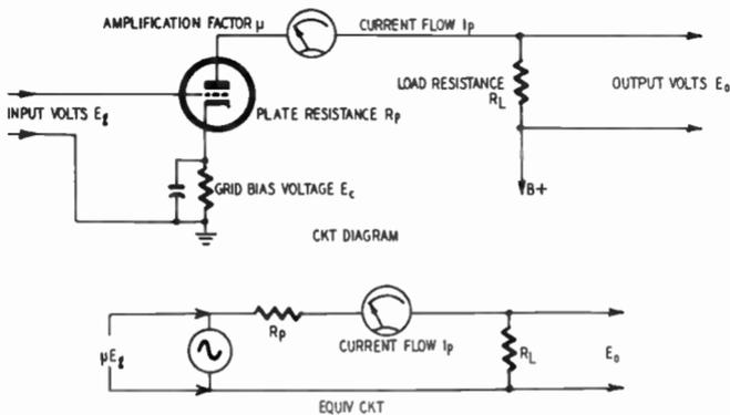
Fig. 325. The vacuum-tube amplifier can be simplified to an equivalent circuit.
