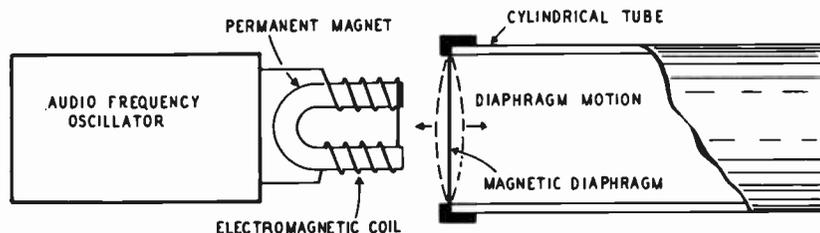
Fig. 702. *Movement of the diaphragm, caused by the varying current through the coil, produces sound.*
