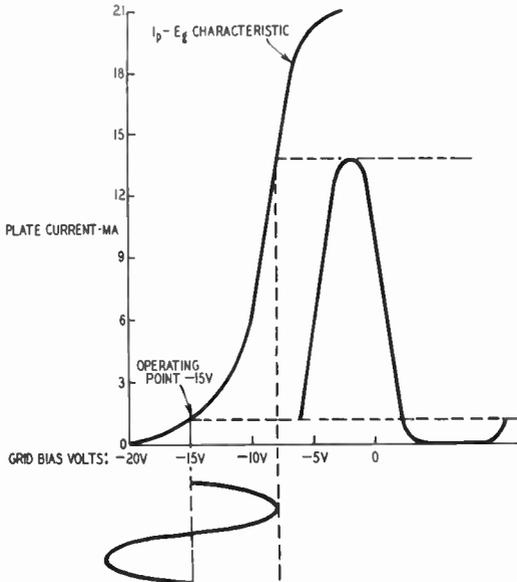
Fig. 303. Class-B operation uses more of the tube's characteristic curve, is more efficient, but produces more distortion than class A.
