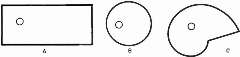
Fig. 704. *Irregularly shaped baffles and off-centering of speakers avoids a single cut-off frequency.*
