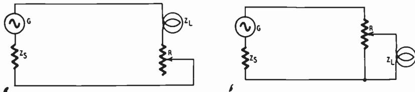
Fig. 607-a, b. *The variable attenuator at the left is not as suitable as that shown at the right.*
