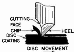
Fig. 906. Drawing at the left illustrates a cutting (or recording) stylus. These are generally made of sapphire while the best reproducing styli are diamond.
