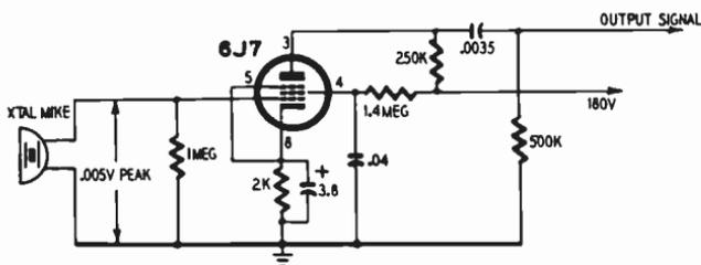
Fig. 326. Resistance-coupled audio amplifier. The design of this circuit is described in the text.
