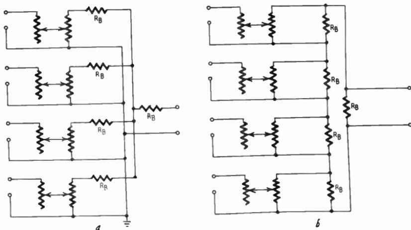
Fig. 610-a, -b. Circuit arrangements for mixer type attenuators.
