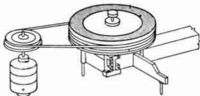
Fig. 903-c. In the illustration at the left we have a simplified drawing of a belt-driven turntable. The advantage of such an arrangement is that the motor is isolated from the turntable.
