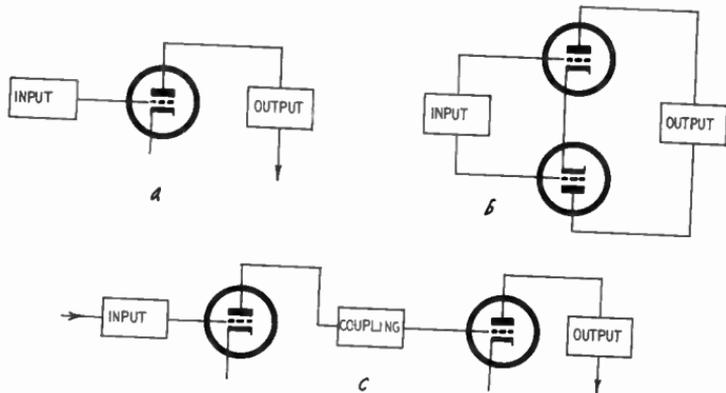
Fig. 307-a, b, c. The circuits shown in a and b provide only a single stage of amplification. In c we have a cascade arrangement of two stages of amplification.
