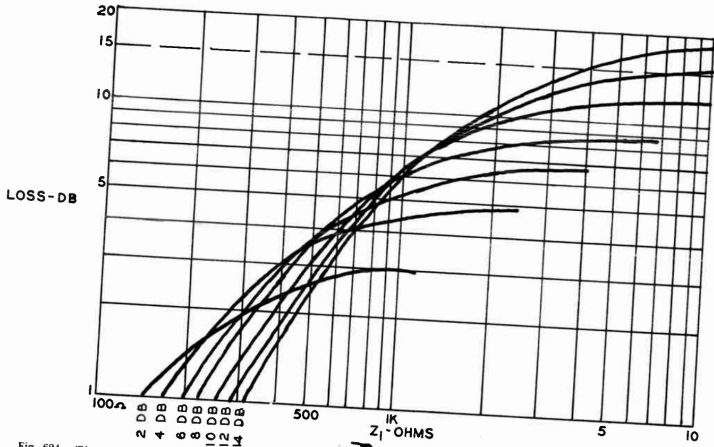
Fig. 624. The curves shown in the illustration above can be used to aid in the solution of equalizer design problems.
