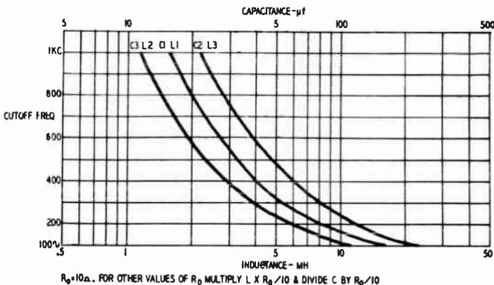
Fig. 723. Design curves based on the networks of Fig. 722.
