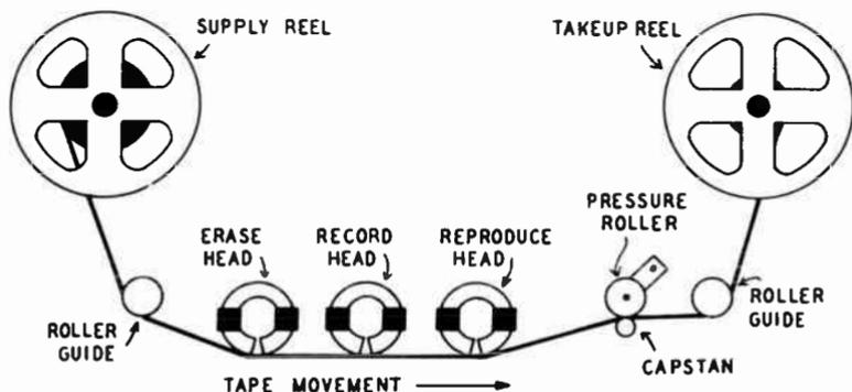
Fig. 923. Major components of a tape recording system.
