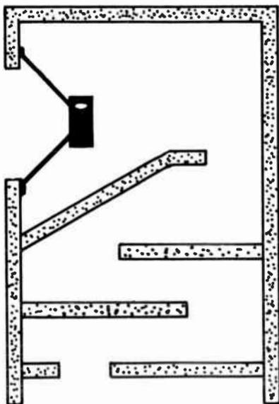
Fig. 707. *Cross-sectional view of an acoustic labyrinth.*
