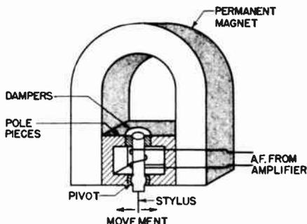
Fig. 909. Chief components of a magnetic cutter.
