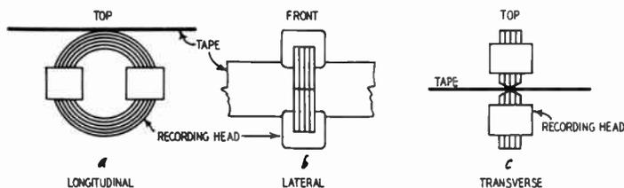
Fig. 929-a. -b. -c. *Longitudinal, lateral, and transverse magnetization.*
