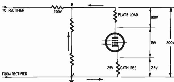
Fig. 412. The cathode resistor, tube, and plate load form a voltage divider across the output of the power supply.
