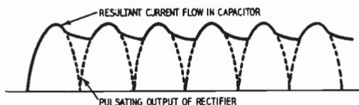
Fig. 408. The filter changes the output of the rectifier from pulsating d.c. to a somewhat smoother voltage.
