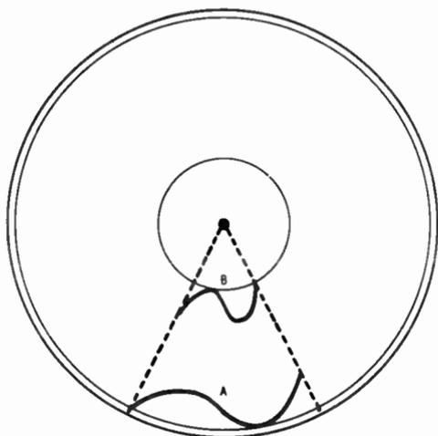
Fig. 913. *The angular distance of groove A is identical with that of groove B.*
