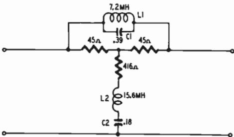
Fig. 626. Here we have the final circuit of the equalizer whose design was calculated and described for you in the text.
