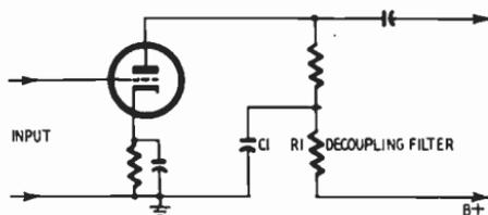
Fig. 317. A decoupling filter consists of a resistor and a capacitor.
