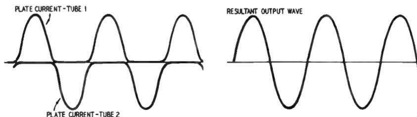
Fig. 304. The distortion of class-B operation can be largely overcome through the use of a push-pull circuit.
