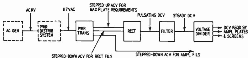
Fig. 402. Block diagram of a power supply. Almost all supplies follow this same general pattern.
