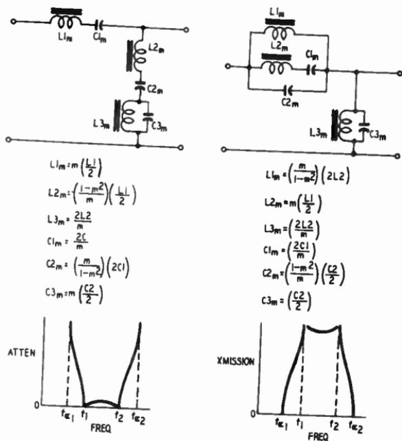
Fig. 619. *M*-derived half section used as a bandpass filter.
