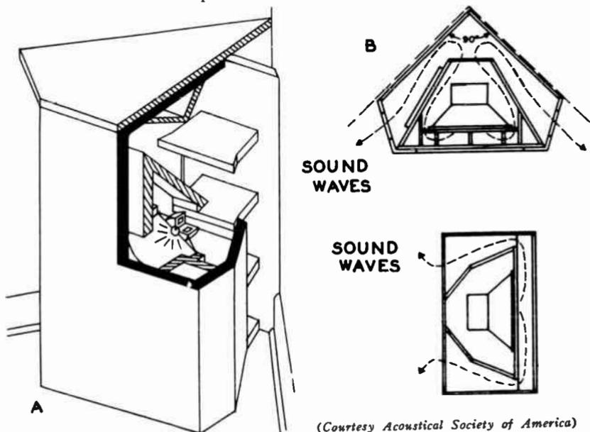
Fig. 711-a,-b. Example of the construction of a folded horn.
