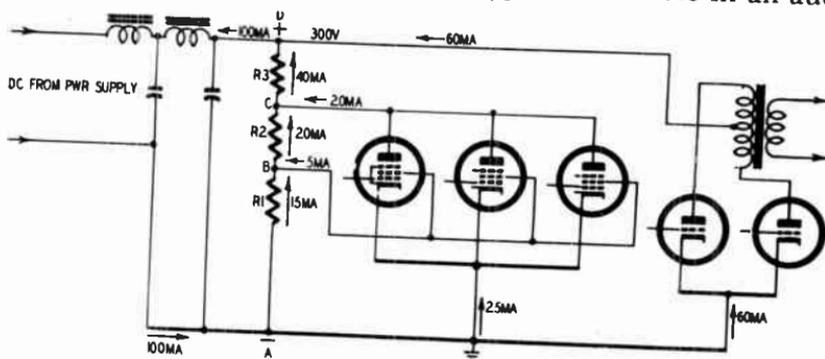
Fig. 411. The power supply furnishes plate and screen voltages for the tubes. The tubes may be considered as a load in parallel with the output of the power supply.
