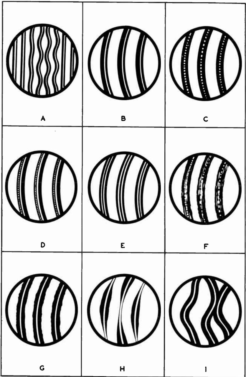
Fig. 920. Typical faults revealed by microscopic examination of the grooves of a record.
