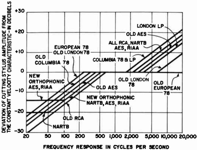
Fig. 912. *Typical recording characteristics.*
