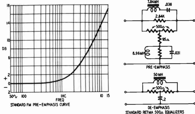
Fig. 621. Typical pre-emphasis and de-emphasis networks. The pre-emphasis curve is used for FM broadcasting.
