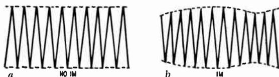
Fig. 503-a,-b. Undistorted waveform (a) shows intermodulation distortion (b).
