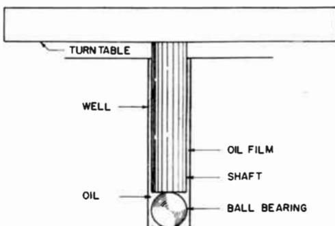
Fig. 902. *Turntable shaft rests on a ball bearing.*
