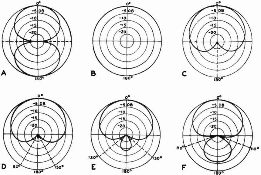
Fig. 811. These illustrations (a to f inclusive) show the varying response characteristics that can be obtained with a modern microphone.
