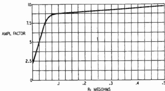
Fig. 315. The gain of an audio circuit increases as the resistance or impedance of the load is raised.
