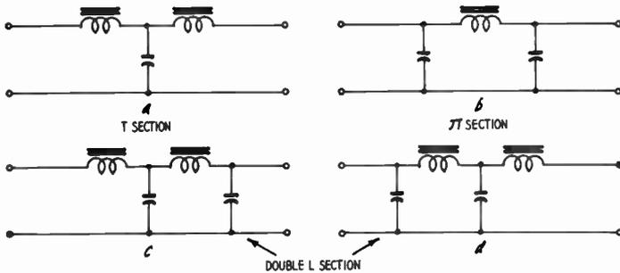
Fig. 410-a, b, c, d. Various types of power supply filters.
