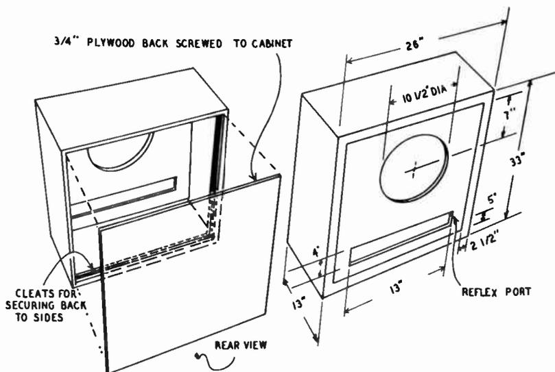
Fig. 706. Constructional details of a bass-reflex enclosure.
