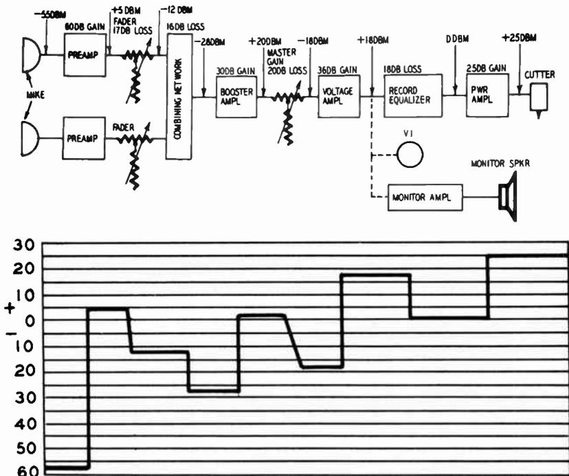
Fig. 205. Block diagram of an audio-amplifier system. The graph indicates the loss or gain of the various units in the system.
