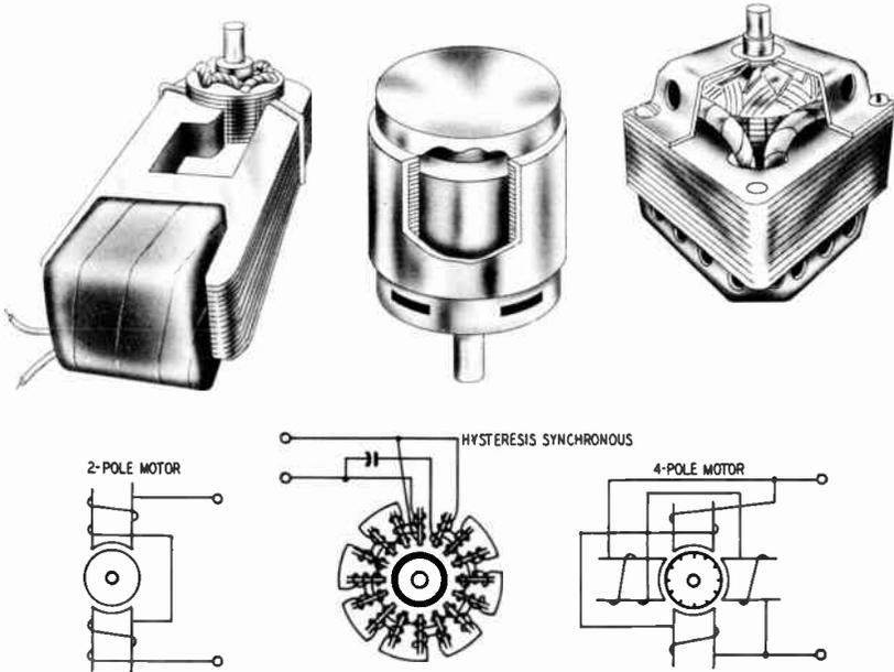
Fig. 901. Typical turntable motors and their electrical circuits.
