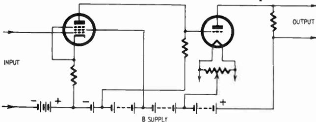
Fig. 309. Circuit of a direct-coupled amplifier. The capacitor between the plate of the first tube and the control grid of the following tube is eliminated.
