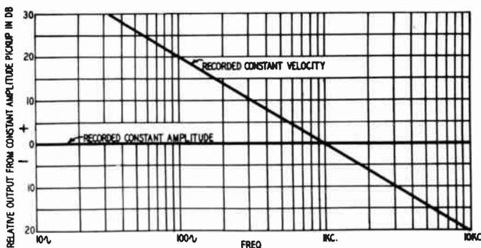
Fig. 910. Output of constant-velocity reproducer decreases 6 db per octave when used with a record made under conditions of constant amplitude.
