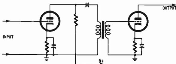
Fig. 316. The capacitor connected between the plate of the first tube and the primary of the transformer permits passage of the signal, but blocks d.c. from the audio transformer.
