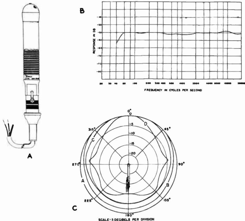
Fig. 805-a, -b, -c. Dynamic microphone (a) has excellent frequency response (b). The graph (c) shows the directivity pattern.
