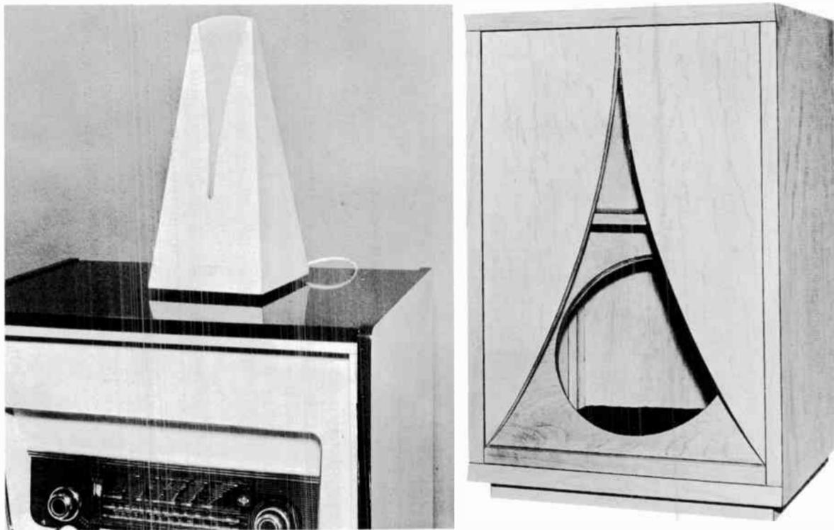
Fig. 709. The unfinished cabinet on the right shows the speaker board mounted behind the tapered slot. A port is behind the narrow end of the slot. On the left a miniature version using the same principle boasts a smooth response from 80 cycles to beyond 15 kc with a 4-watt, 5-inch, 8-ohm speaker. This 4-pound unit may also be hung on the wall in an inverted position. (Karlson Associates, Inc.)
