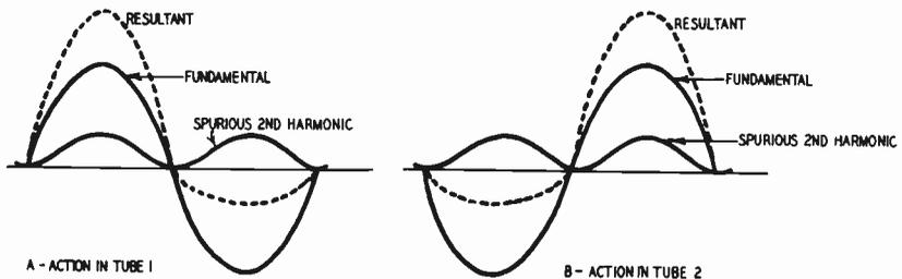
Fig. 319-a-b. Waveforms in the output of a push-pull circuit.
