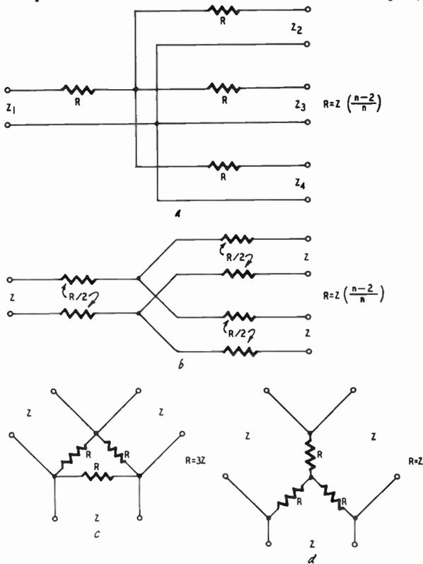
Fig. 606-a, -b, -c, -d. Attenuators can be used to divide the signal.
