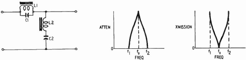
Fig. 615. Band elimination filter and its characteristics.
