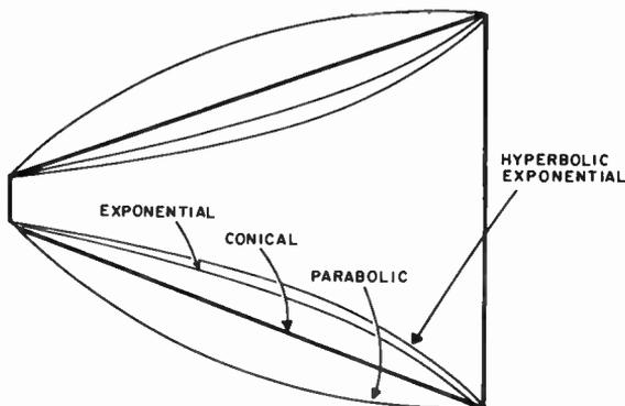
Fig. 714. This illustration shows shapes of typical horns.
