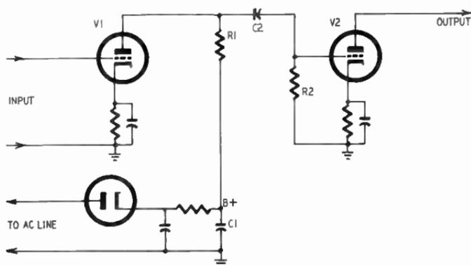
Fig. 310. Elementary audio-amplifier system. Triodes are used here for the sake of simplicity.
