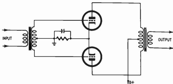
Fig. 318. *Fundamental diagram of a push-pull circuit. Center-tapped transformers are used.*
