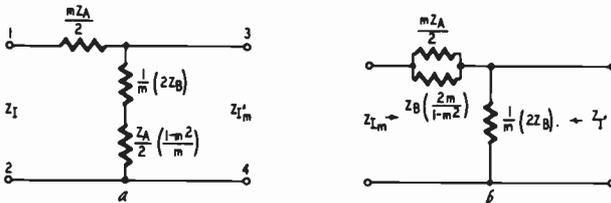
Fig. 616-a, -b. Basic series  $m$ -derived half section.
