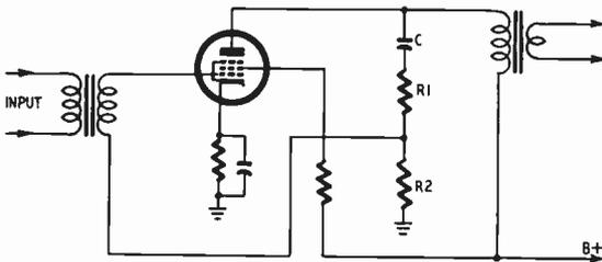
Fig. 321. Typical negative-feedback arrangement. Frequency response improves at expense of gain.
