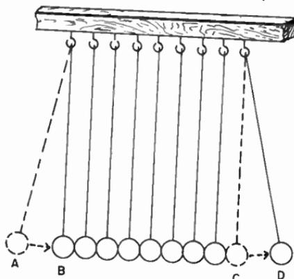
Fig. 701. Mechanical illustration of the transmission of sound in air.
