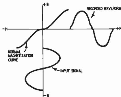
Fig. 925. *Distortion produced in recorded waveform.*
