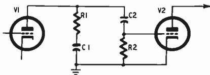
Fig. 311. This is the same circuit as that shown in Fig. 310. The power supply has been omitted.
