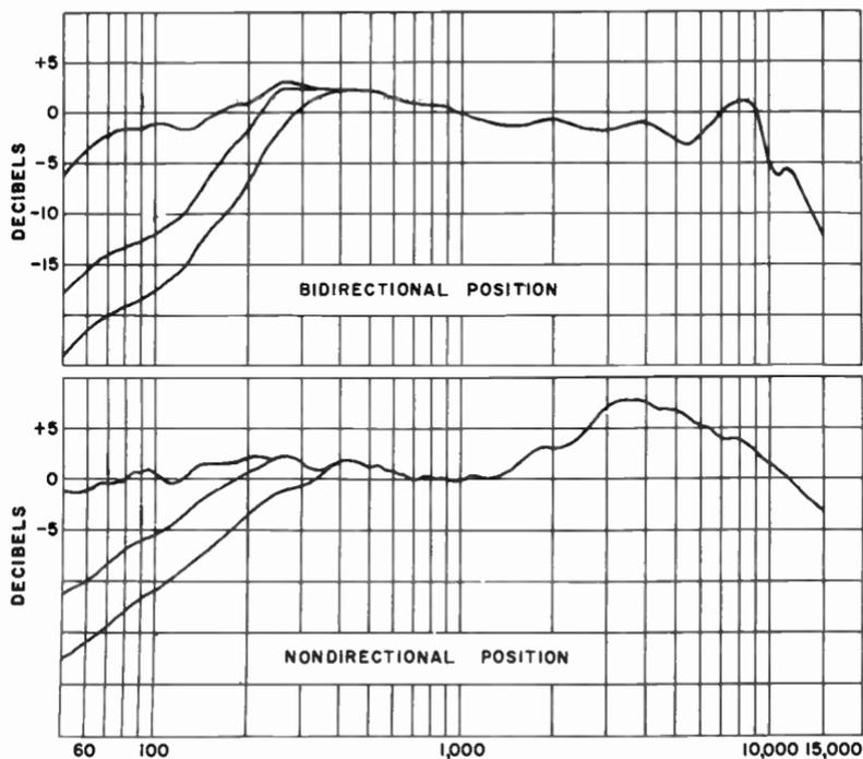
Fig. 810. Several of the frequency response characteristics of the microphone illustrated in Fig. 809.
