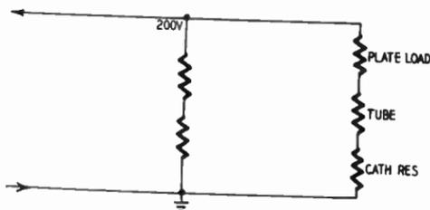
Fig. 413. The circuit of Fig. 412 becomes simplified if we consider the tube as a resistor.
