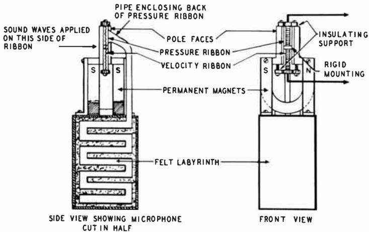
Fig. 809. Modern microphone shown in cross section.
