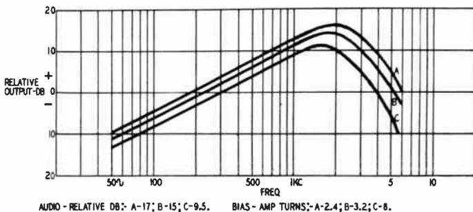
Fig. 927. Relationship between bias and frequency response.
