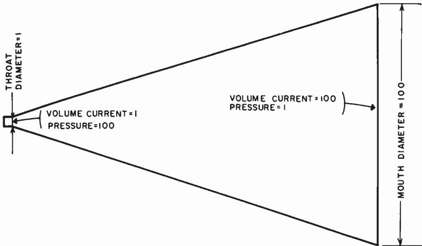
Fig. 713. *Relationship of throat and mouth pressures in a horn.*
