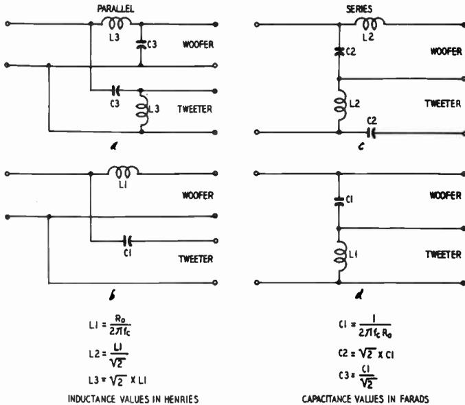
Fig. 722-a, -b, -c, -d. Constant-resistance dividing networks.
