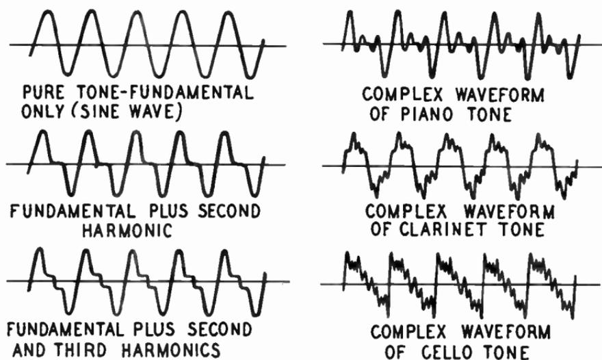
Fig. 104. The three curves at the left show the formation of a complex waveform through the combination of a pure tone and its harmonics. Representative waveforms of various instruments are shown at the right.
