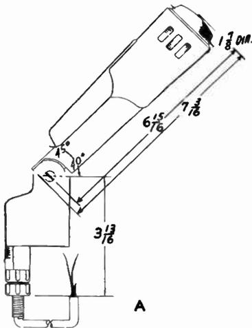
Fig. 813. This microphone (a) has openings in the case arranged in such a manner that a cardioid characteristic (b) is obtained.
