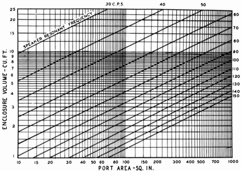
Fig. 705. This chart gives the relationship between the volume, resonant frequency and port area of a bass-reflex enclosure.
