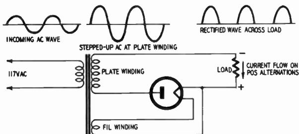
Fig. 405. The line voltage is stepped up by the transformer and is rectified by the diode. The output consists of pulses.
