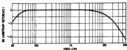
Fig. 501. *Frequency-response curve of a typical audio amplifier system.*
