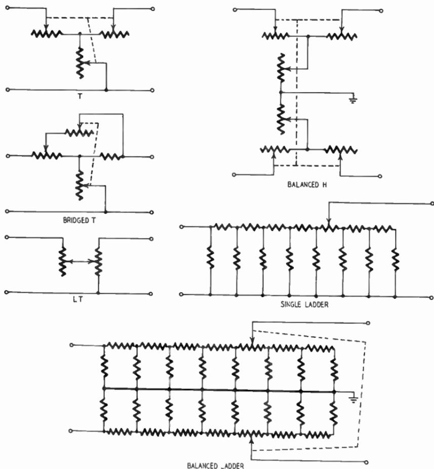
Fig. 608. Typical attenuating networks are shown above.
