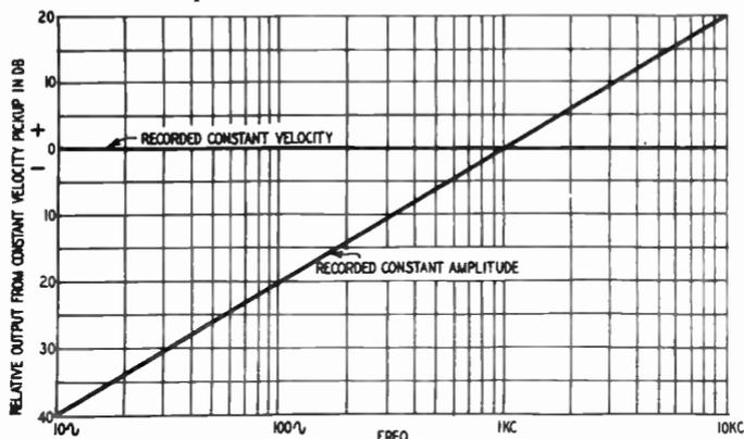
Fig. 911. This curve also shows a 6 db slope per octave. Compare this with Fig. 910.
