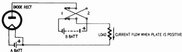
Fig. 404. Current will flow through the diode only when the plate is positive with respect to the filament (or cathode). The diode behaves like a valve.
