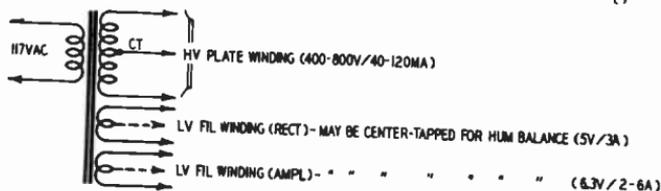
Fig. 403. Typical power transformer circuit. The size of the transformer will be determined by the amount of power to be delivered by it.
