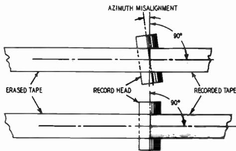
Fig. 930. Angular displacement of the record head will produce distortion.
