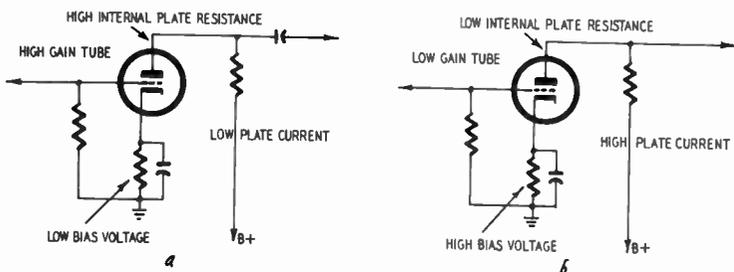
Fig. 308-a,b. The circuit at the left is a voltage amplifier; that at the right is a power amplifier. The circuits are drawn the same way, but component values and type of operation differ.
