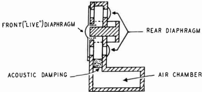
Fig. 812. In this microphone the acoustic air chamber is below the microphone.
