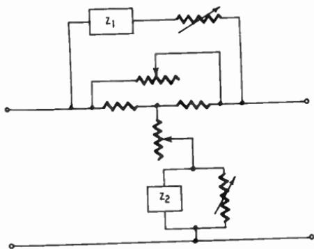
Fig. 628. Basic arrangement of a constant-B equalizer circuit.
