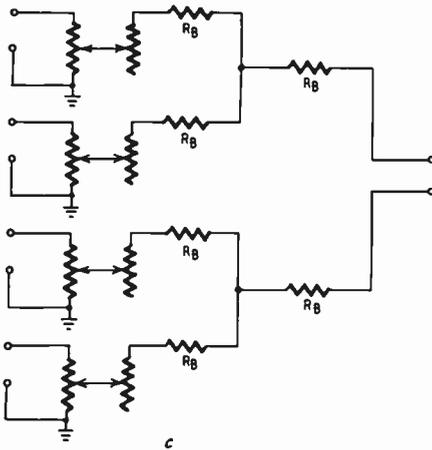
Fig. 610-c. *Series-parallel mixer circuit.*
