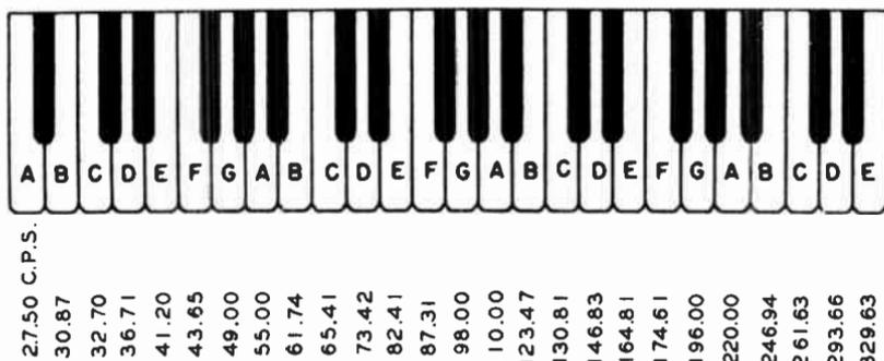
Fig. 103. This illustration shows a standard 88-note piano keyboard. The figures placed below each key indicate the frequency in cycles per second of each corresponding note. Middle A on the piano has been fairly well standardized at 440 cycles per second (c.p.s.). The piano, in common with all other musical instruments, produces complex tones. These tones consist of sine waves plus a number
