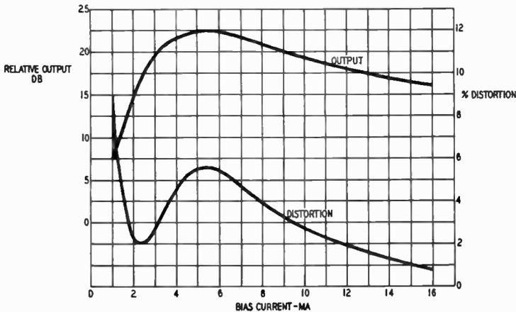
Fig. 928. Effect of bias current on output and distortion.
