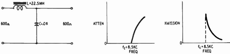
Fig. 612. Single constant- $k$   $L$  section showing attenuation and transmission characteristics.
