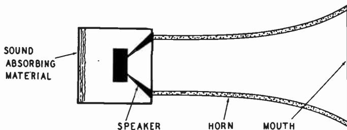
Fig. 710. Typical horn-type loudspeaker.
