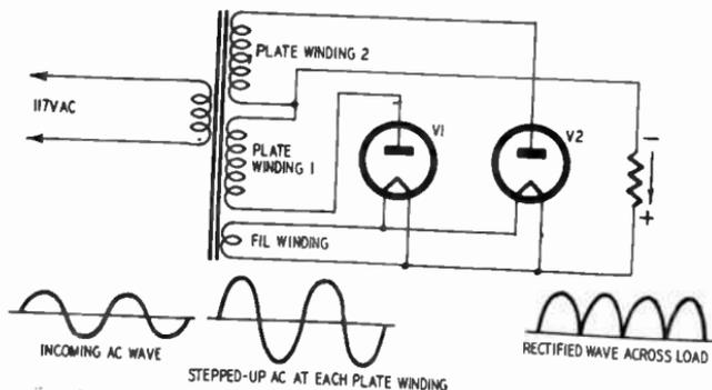
Fig. 406. The action here is the same as that shown in Fig. 405 except that we have more pulses in the output. This type of supply is more desirable for audio work.
