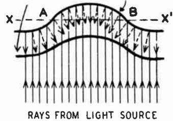
Fig. 918. The drawing at the right helps explain the reason for the reflected light patterns of Fig. 917. The greatest angle between the rays from the light source and those that are reflected will occur at the steepest groove curvature.
