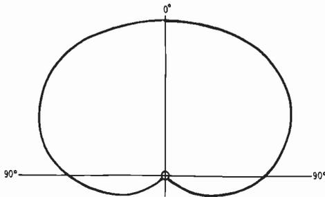
Fig. 808. Graph of a cardioid characteristic.
