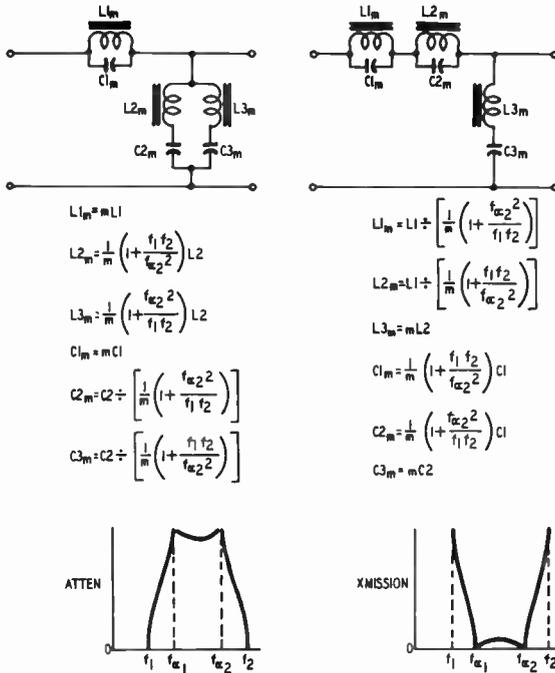
Fig. 620. *M*-derived half section used as a band elimination filter.
