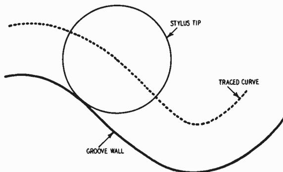
Fig. 914. *The pickup cannot always follow the exact curve of the recording stylus.*
