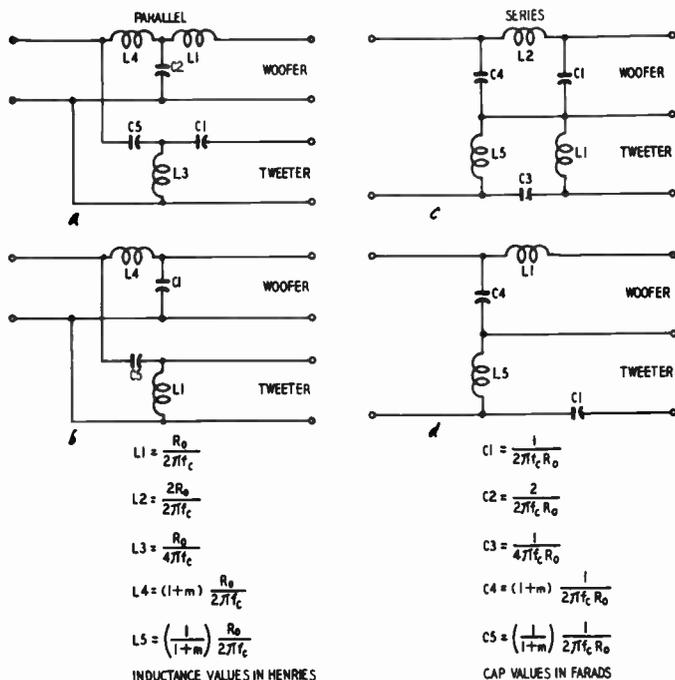
Fig. 720-a, -b, -c, -d. Design circuits and formulas for crossover networks.
