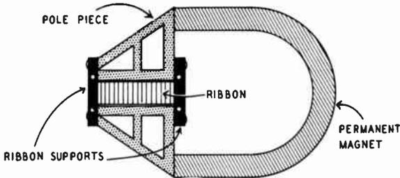
Fig. 806. *Velocity or pressure-gradient microphone.*
