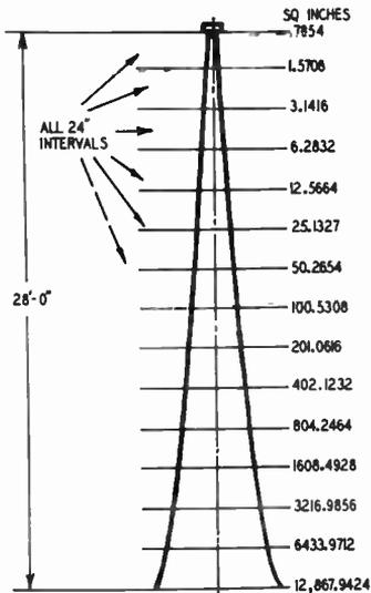
Fig. 716. Design of a horn.
