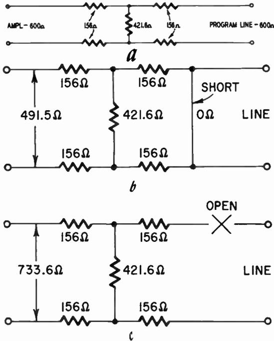
Fig. 605-a, -b, -c. Attenuators can be used as isolation networks.
