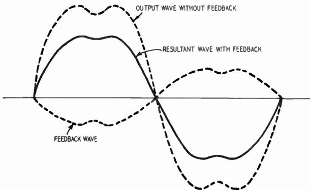
Fig. 322. *The effect of feedback is to reduce the gain and improve the waveform*
