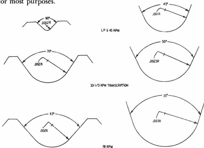
Fig. 907. Record groove dimensions (left) and stylus dimensions (right). These drawings are not to scale, and are exaggerated for the sake of clarity.
