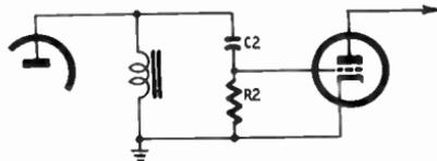
Fig. 313. An iron-core coil can be substituted for resistor  $R_1$ .
