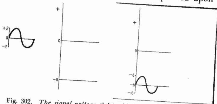
Fig. 302. The signal voltage (left) added to the d.c. bias (center) gives us an a.c. wave with a d.c. component, (right).
