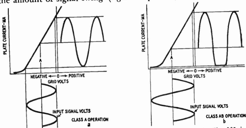
Fig. 306-a,-b. The drawing for class AB operation illustrated in Fig. 305 is repeated here so that you may compare it with class A (shown at the left). The letter A is directly below the operating point.
