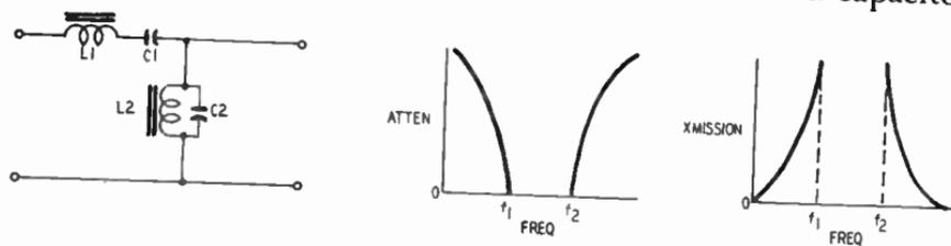
Fig. 614. Bandpass filter contains series and parallel (fixed-tuned) circuits.
