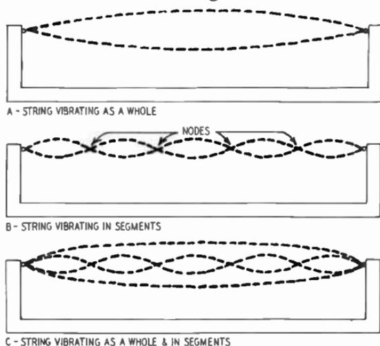
Fig. 106. *This illustration shows the characteristics of a vibrating string.*
