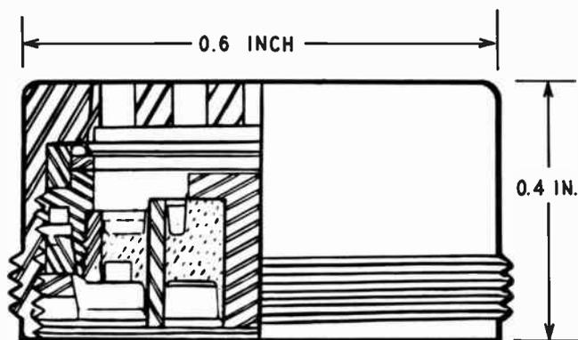
Fig. 814. *Extremely small size is unique feature of this condenser microphone.*
