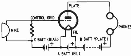
Fig. 401. *There are three voltage supplies in this circuit. The A battery furnishes filament voltage, the B battery is for plate voltage while the C battery biases the control grid.*
