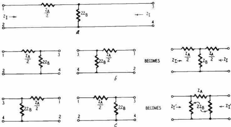
Fig. 611-a, -b, -c. The L-pad can be used to build a T- or pi attenuator.
