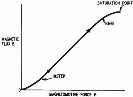
Fig. 921. Normal magnetization curve.
