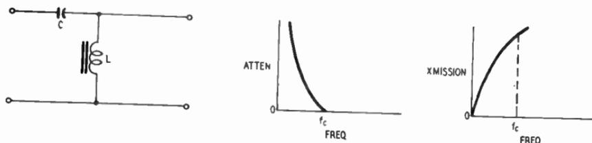
Fig. 613. Single constant- $k$  high-pass filter network.
