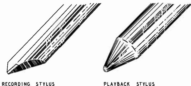
Fig. 905. Difference in construction between recording and playback styli.
