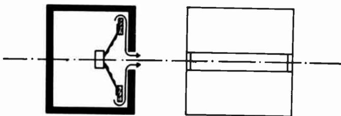
Fig. 708. *The Helmholtz resonator has a strong resonance point.*
