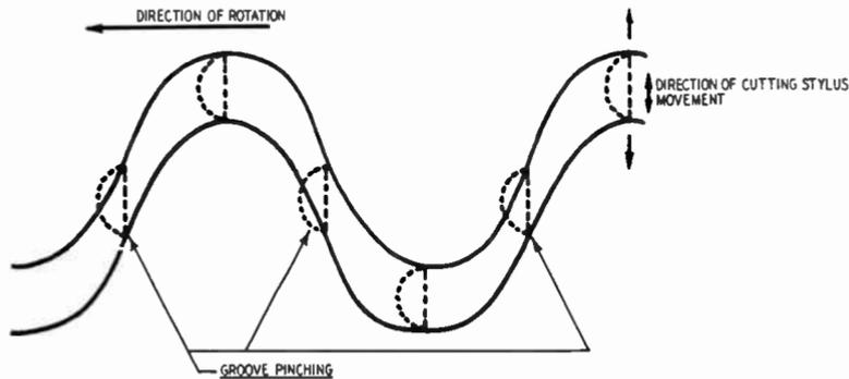
Fig. 915. Illustration of pinch effect.
