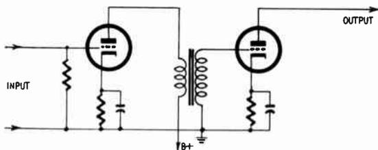
Fig. 314. *Transformer-coupled audio amplifier.*
