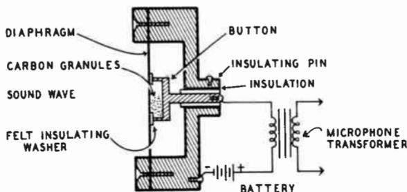
Fig. 801. *Cross-sectional view of carbon microphone.*
