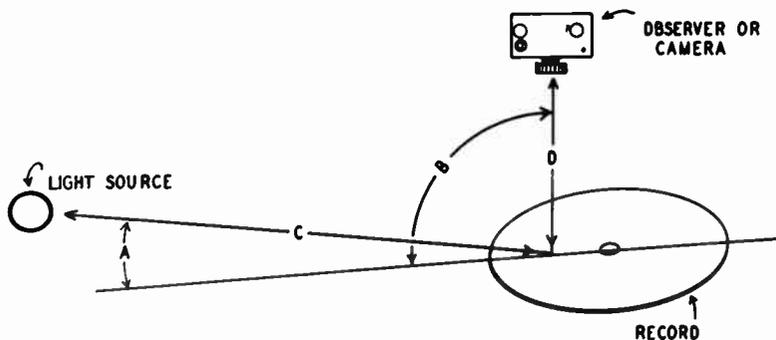
Fig. 916. Setup for visual groove inspection.
