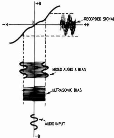
Fig. 926. Effect of mixing ultrasonic bias and the audio signal.
