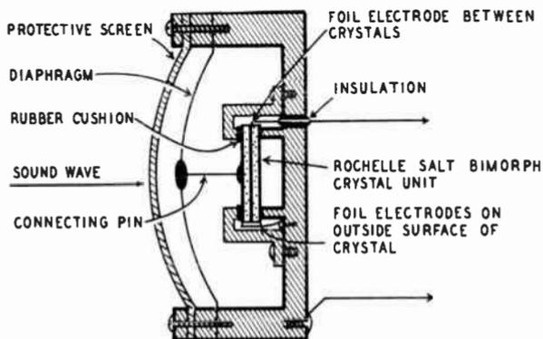
Fig. 803. *Crystal microphone in cross section.*
