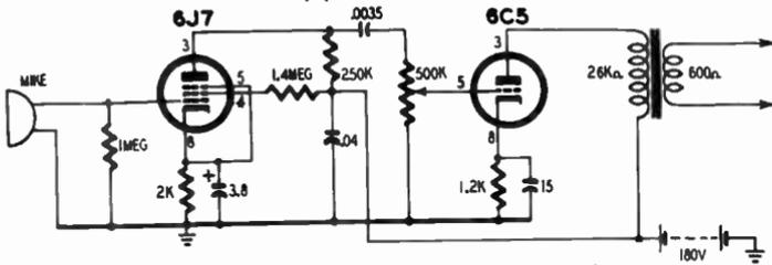
Fig. 328. The final design of the amplifier.
