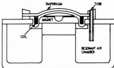
Fig. 804. *Dynamic or moving-coil microphone.*
