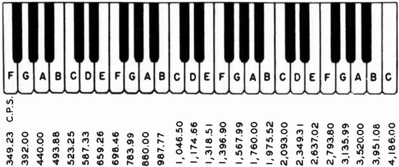
*of harmonics. The fundamental sine wave combines with the harmonics to produce complex waveforms. It is the presence of these harmonics which gives the piano its particular tone. Frequencies other than harmonics are produced when a key is struck, but the harmonics are the most important. This means that an audio system must be able to pass a wide range of frequencies.*
