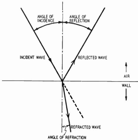
Fig. 101. Sound, striking a wall, is reflected by it. Some of the sound is absorbed by the wall and a portion of the sound is transmitted by it.
