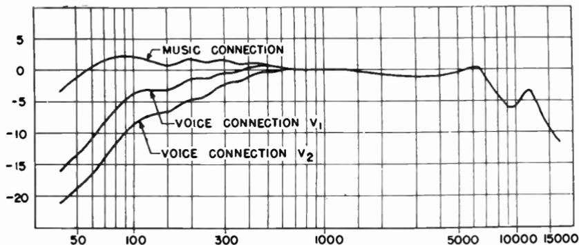
Fig. 807. Frequency response curves of a typical velocity microphone.
