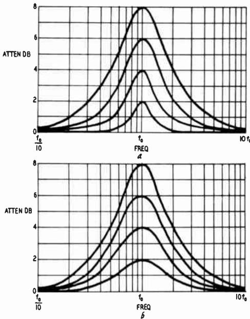
Fig. 627-a, -b. Families of curves for equalizer circuits.
