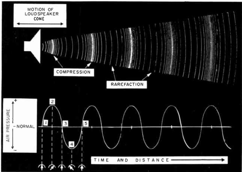
Fig. 102. *The motion of the cone of a loudspeaker produces changes in the pressure of the air surrounding the cone.*
