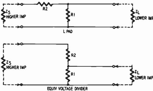
Fig. 604. The L-pad is a voltage divider.
