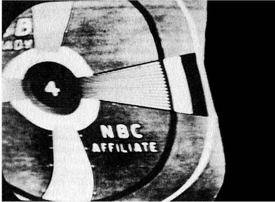
Fig. 510. Horizontal jitter or weaving. The trouble in this case was due to a short between cathode and heater of a sync clipper-amplifier tube.
