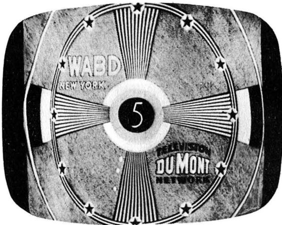
Fig. 305. Photo of test pattern indicates insufficient width.
