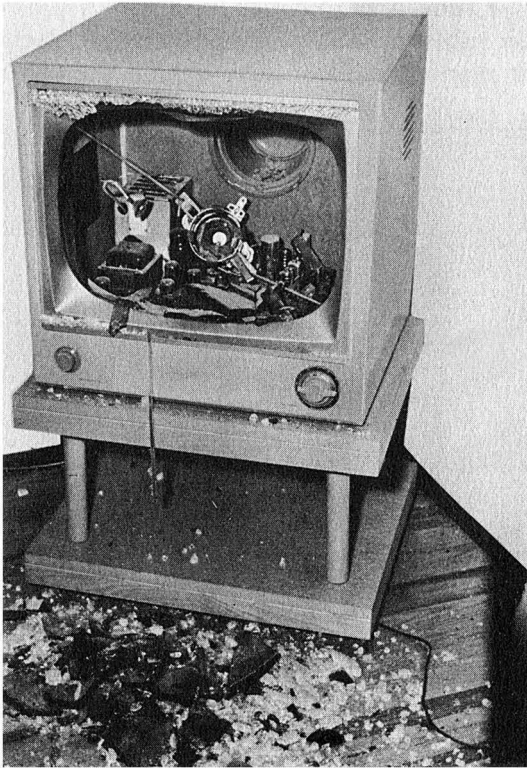
Fig. 102. Result of a cathode-ray implosion due to inadequate safety precautions.
