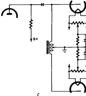
Fig. 301-c. Inductive phase inverter using a center-tapped choke.
