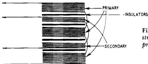
Fig. 604. Special method of constructing a transformer in which the primary and secondary windings are interleaved.
