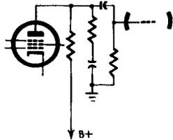
the intermediate stage a narrower response than the other two, the phase shifts of the various stages will occur at different frequencies. Although the final response may not be as wide as one would have hoped for, the somewhat narrower response may permit a degree
