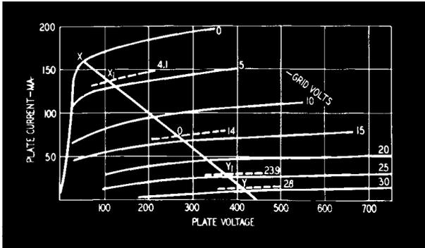
Fig. 205. Plate-voltage-current curves of the 6L6 showing load line and operating conditions.
