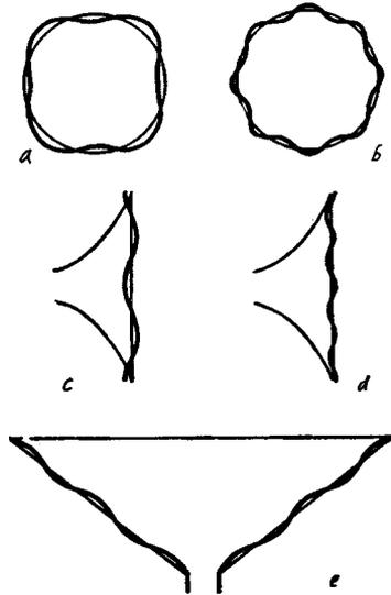
Fig. 1003. *Types of cone deformation causing distortion: a, -b) typical nodes formed in a straight-sided conical diaphragm; c, -d) exponential diaphragms displaying axial nodes; e) wave motion along the surface of the cone.*
