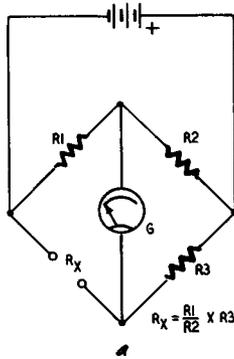
Fig. 1103-a. *Wheatstone bridge for measurement of dc resistances.*
