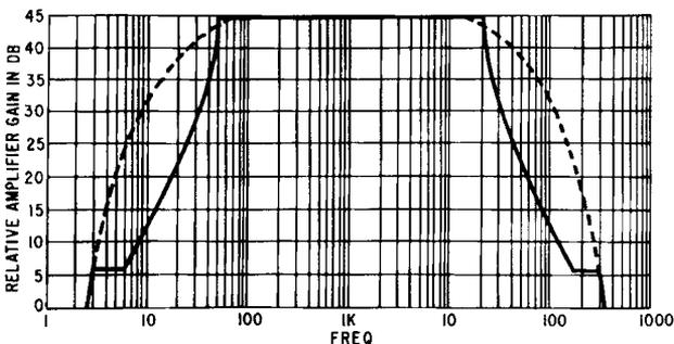
Fig. 715. Ideal response of a stable feedback amplifier.
