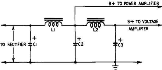
Fig. 907. Two-stage capacitor-input filter.
