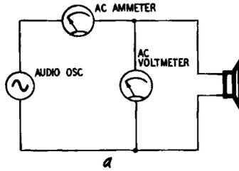
Fig. 1006-a. *Determining speaker impedance by using an ammeter and voltmeter.*
