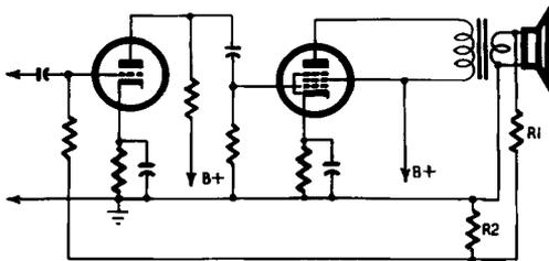
Fig. 708. The secondary of the output transformer is part of the feedback loop.
