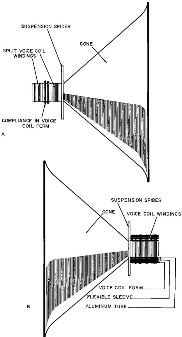
Figs. 1203-a,-b. *Two methods of introducing a compliance into a voice coil; a) split voice coil on a form with center compliance; b) compound voice coil with intermediate compliance.*
