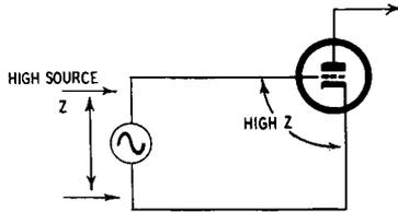
Fig. 401. Source and grid-to-cathode impedances are generally high.
