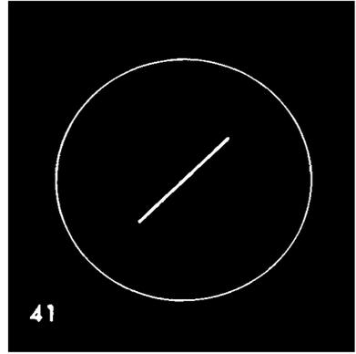
Trace 40) *Parasitic oscillation revealed by square wave*; Trace 41) *Two voltages in phase*; Trace 42) *Two voltages 30° or 330° out of phase*; Trace 43) *Two voltages 60° or 300° out of phase*; Trace 44) *Two voltages 90° or 270° out of phase*.
