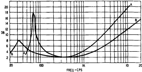
Fig. 1005. Impedance curves of dynamic speakers: AA) curve of a conventional design with cone surround resonance at 70 cps; BB) curve of speaker with free-edge cone. Voice coil, cone compliance and rear suspension (spider washer) resonance of 32 cps.
