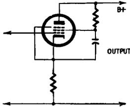
Fig. 703. Method of connecting a series feed resistor.
