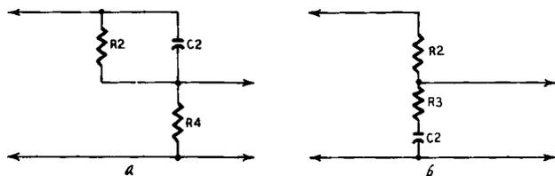
Figs. 805-a,-b. Tone control circuits: a) bass cut; b) treble cut.
