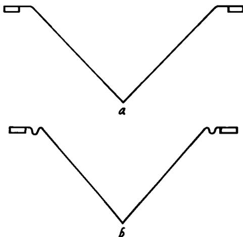
*Figs. 1202-a-b. Free edge suspension: a) usual type consisting of a flat felt, woven cloth, thin or sponge rubber ring. Movement is rather restricted; b) free edge suspension permitting rotary motion arising from tangential arm spider. Incorrect material or its application will result in cone drooping.*
