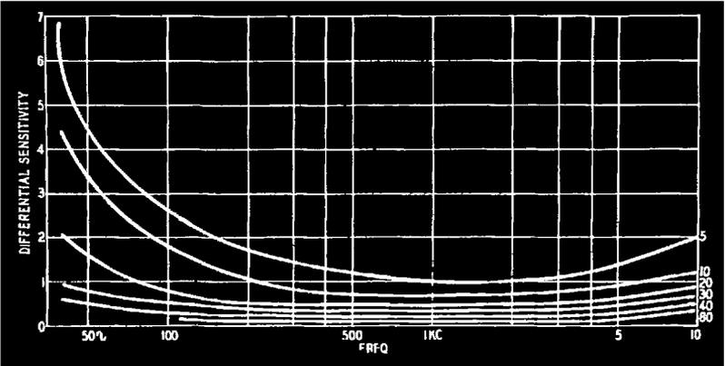
Fig. 103. Variation of frequency response of the ear at various volume levels. The figures shown at the right-hand ends of the curves are in db.
