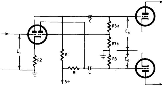
This table includes double triodes normally used as voltage amplifiers. Other tubes can also be used; e.g. the double triodes listed in Table 8, where the operating conditions listed in that table should be used. C is selected to give 0.9  $E_o$ , at 50 cps.
