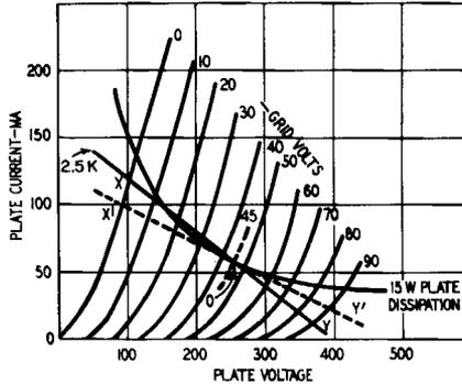
Fig. 204. Plate-voltage–plate-current curves of the 2A3 showing load line and operating conditions.
