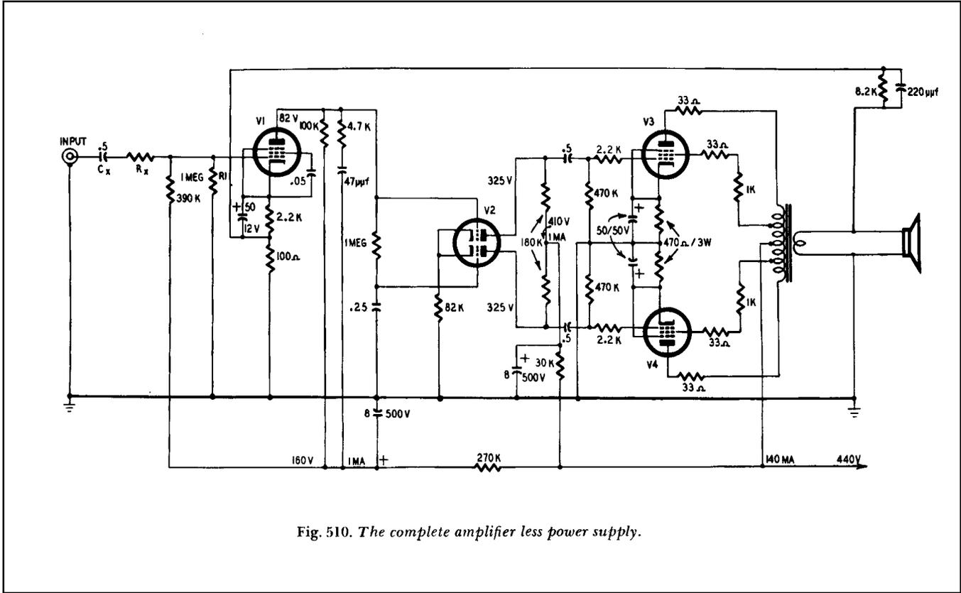
Fig. 510. The complete amplifier less power supply.
