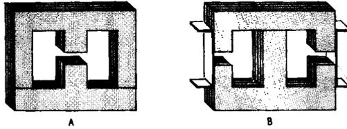
Fig. 911. Several possible arrangements of laminated-iron cores.
