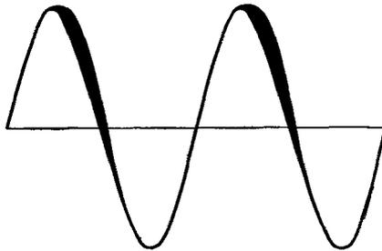
Fig. 607. Spreading of the sine wave indicates oscillation.
