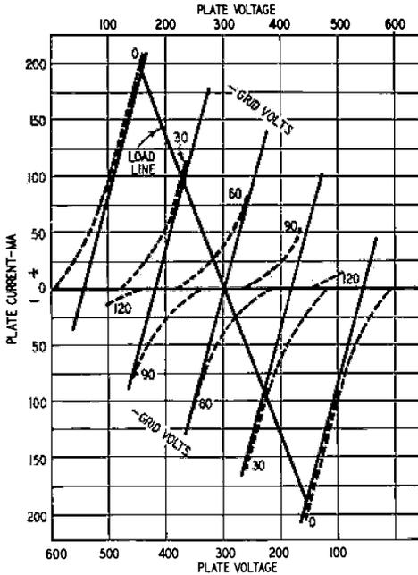
Fig. 206. Combined characteristics of two 2A3 tubes in push-pull.
