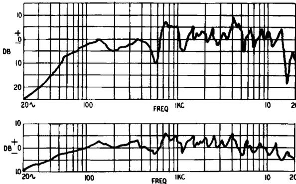
Fig. 1001. Frequency response curves of a speaker with 4 volts input (upper curve) and with 1 volt input (lower curve).
