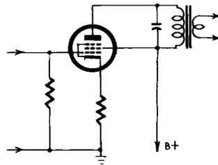
Fig. 710. A capacitive shunt is sometimes placed across the primary of the output transformer.
