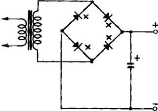
Fig. 904. Metal rectifier bridge connection.
