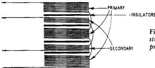
Fig. 604. Special method of constructing a transformer in which the primary and secondary windings are interleaved.
