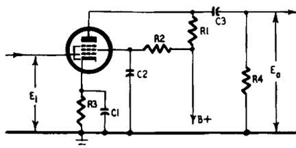
C1, C2, C3 adjusted to give 0.7 E<sub>o</sub> at 50 cps.
