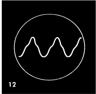
Trace 11) 30% 3rd harmonic in phase; Trace 12) 30% 3rd harmonic  $-90^\circ$  out of phase.
