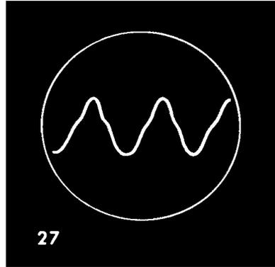
Trace 26) 5% 3rd harmonic 180° out of phase and 5% 5th harmonic in phase; Trace 27) 5% 3rd harmonic 180° out of phase and 5% 5th harmonic 180° out of phase; Trace 28) waveform when amplifier is set to maximum undistorted output; Trace 29) slight overloading; Trace 30) more overloading.
