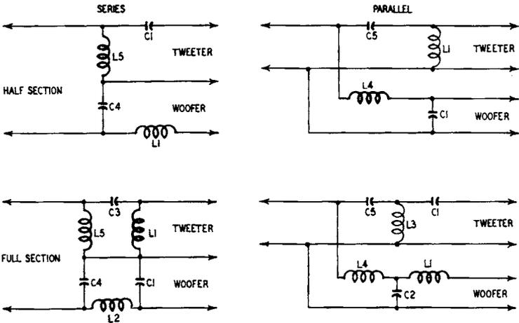
$$L1 = R/\omega \quad L2 = 2R/\omega \quad L3 = R/2\omega \quad L4 = 1.6R/\omega \quad L5 = 0.63R/\omega$$
