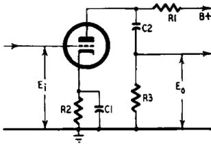
C1 and C2 adjusted to give 0.8  $E_o$  at 50 cps.
