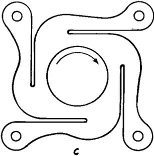
Fig. 1201-c. Tangential arm spider producing rotary cone motion when used with a free edge suspension.
