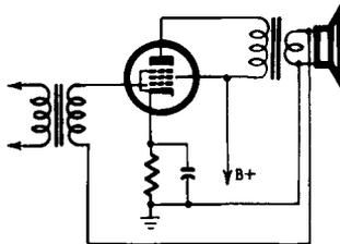
Fig. 706. Applying feedback across the output stage and output transformer.
