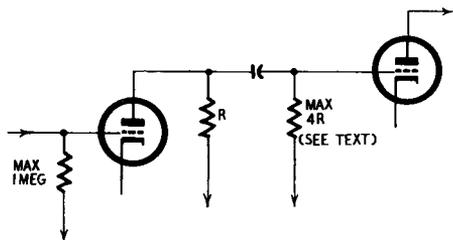
Fig. 402. *Relative values of plate and grid resistors.*
