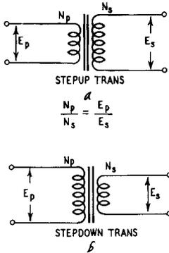
Fig. 601. Relationship between primary and secondary windings of a transformer: a) stepup transformer; b) stepdown transformer.
