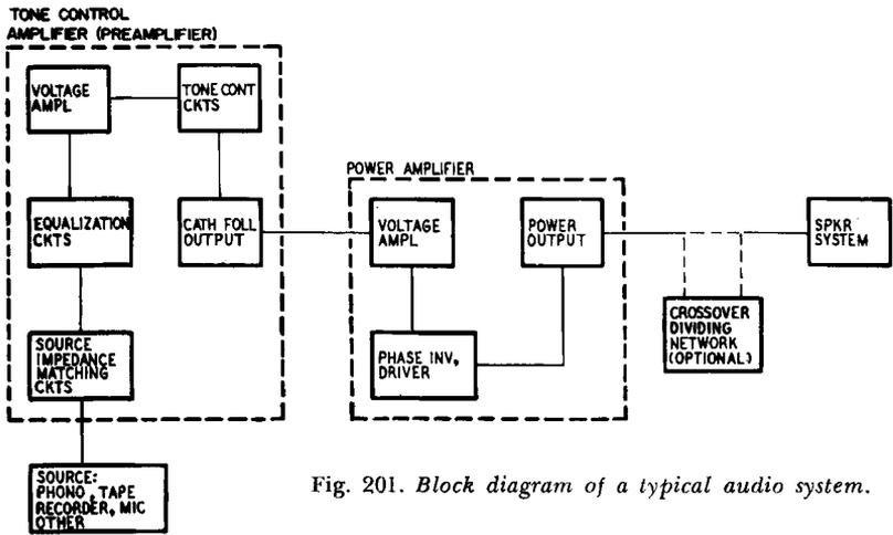
Fig. 201. Block diagram of a typical audio system.
