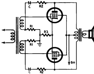
Fig. 705. Applying feedback across a push-pull output stage.
