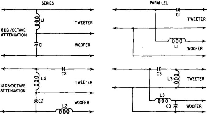
$$L1 = R/\omega \quad L2 = R/\sqrt{2}\omega \quad L3 = \sqrt{2}R/\omega$$
