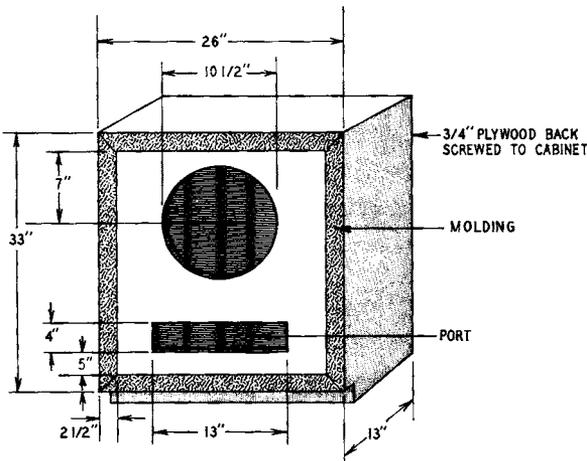
Fig. 1009. *External view of a typical bass-reflex enclosure.*
