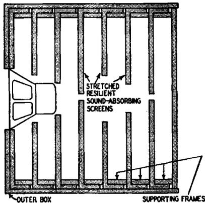
Fig. 1207. *The Hartley Baffle. Each set of four sound absorbing screens forms an acoustic filter, the example shown comprising a 2-stage filter. Note that sound absorbing material is nipped between the screen frames and sides of the box to damp out resonances in the box sides and adding the frame thickness to the box wall thickness.*
