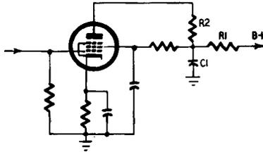
Fig. 406.  $R_1$  and  $C_1$  form a decoupling network.
