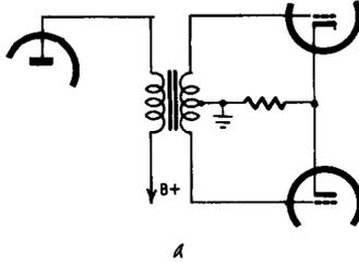
Fig. 301-a. Inductive phase inverter using center-tapped transformer.
