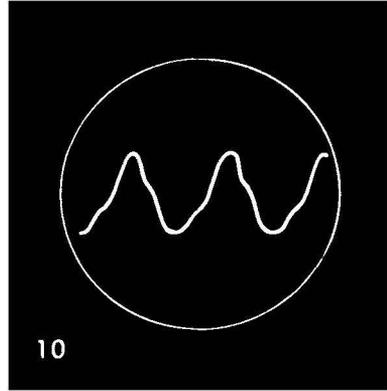
Trace 9) 15% 3rd harmonic  $+90^\circ$  out of phase; Trace 10) 15% 3rd harmonic  $-90^\circ$  out of phase.
