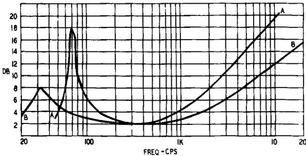
Fig. 1005. *Impedance curves of dynamic speakers: AA) curve of a conventional design with cone surround resonance at 70 cps; BB) curve of speaker with free-edge cone. Voice coil, cone compliance and rear suspension (spider washer) resonance of 32 cps.*
