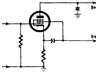
Fig. 709.  $R_f$  bypass to ground in an early stage increases stability in feedback amplifiers.
