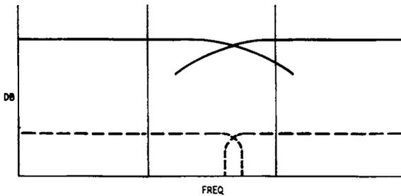
Fig. 1010. Response curve of a typical dividing network.
