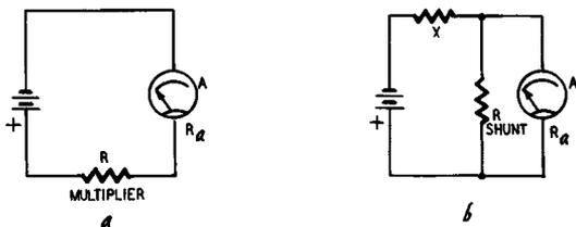
Fig. 1101-a, -b. To use the ammeter as a voltmeter (left) a series resistor is inserted. The meter range is extended (right) through the use of a shunt resistor.
