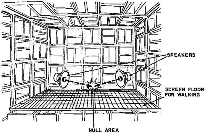
Fig. 104. Mutual interference of sound waves: a—(above) two speakers working at the same level and frequency in an anechoic chamber; b—(below) null areas produced by the tines of a tuning fork.
