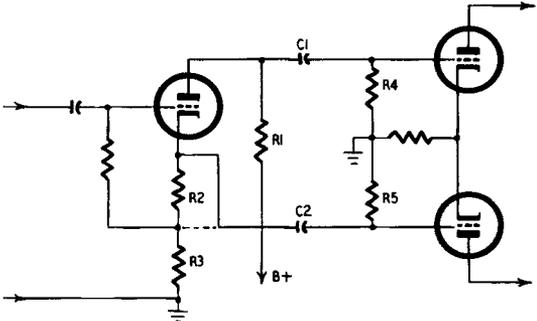
Fig. 305. Split-load phase inverter.
