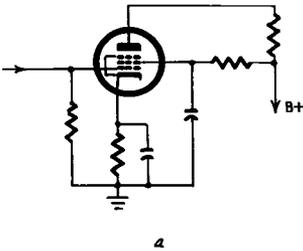
Fig. 404-a. Usual method of applying screen voltage.
