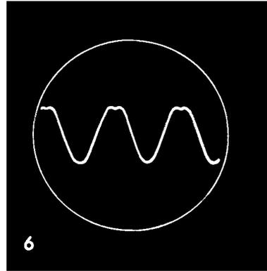
Trace 5) 30% 2nd harmonic  $180^\circ$  out of phase; Trace 6) 30% 2nd harmonic  $+90^\circ$  out of phase.
