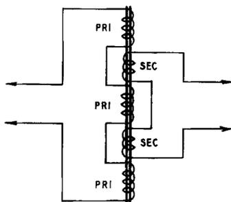
Fig. 603. Method of alternating primary and secondary windings to reduce leakage inductance.
