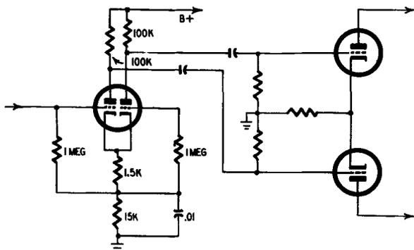
Fig. 304. *Self-balancing phase inverter (Schmitt).*
