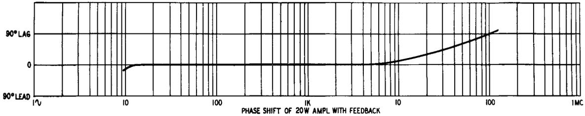
Fig. 511. Performance curves for the amplifier of Fig. 510.
