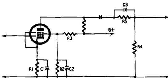
Fig. 712. Bass cut filter for feedback amplifiers.
