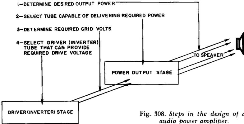
Fig. 308. Steps in the design of an audio power amplifier.
