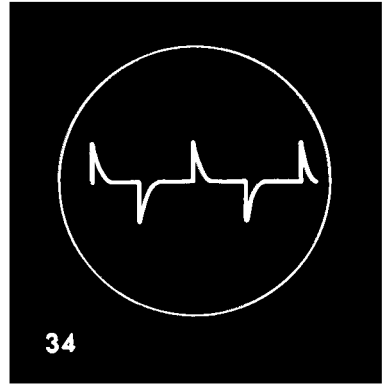
Trace 33) Effect of long time constant on a square wave; Trace 34) Effect of short time constant on a square wave.
