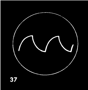
Trace 37) Effect of an amplifier (with treble attenuation) on a square wave, typical of an amplifier without negative feedback, at 3,000 cps.
