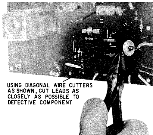
Fig. P-10. When removing parts, cut as closely to the body of the component as possible. (Courtesy Admiral Corp.)
