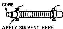
Fig. S-6. If the ferrite core is cemented into position, a few drops of solvent will loosen it enough to permit core adjustment.
