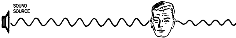
Fig. 204. Effect of interposition of the head upon amplitude of sound at each ear.
