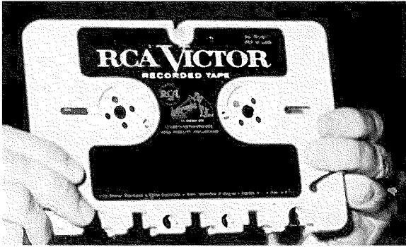
Fig. 612. The RCA magazine for use with tapes recorded by their method contains up to 1 hour of music.
