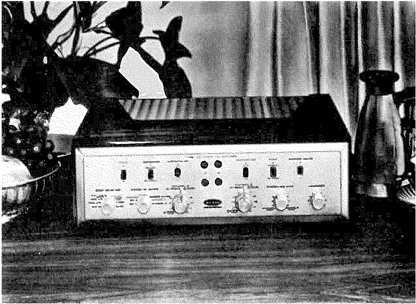
Fig. 1004. A stereo control amplifier which contains facilities for handling all types of program material. (Courtesy H. H. Scott, Inc.)
