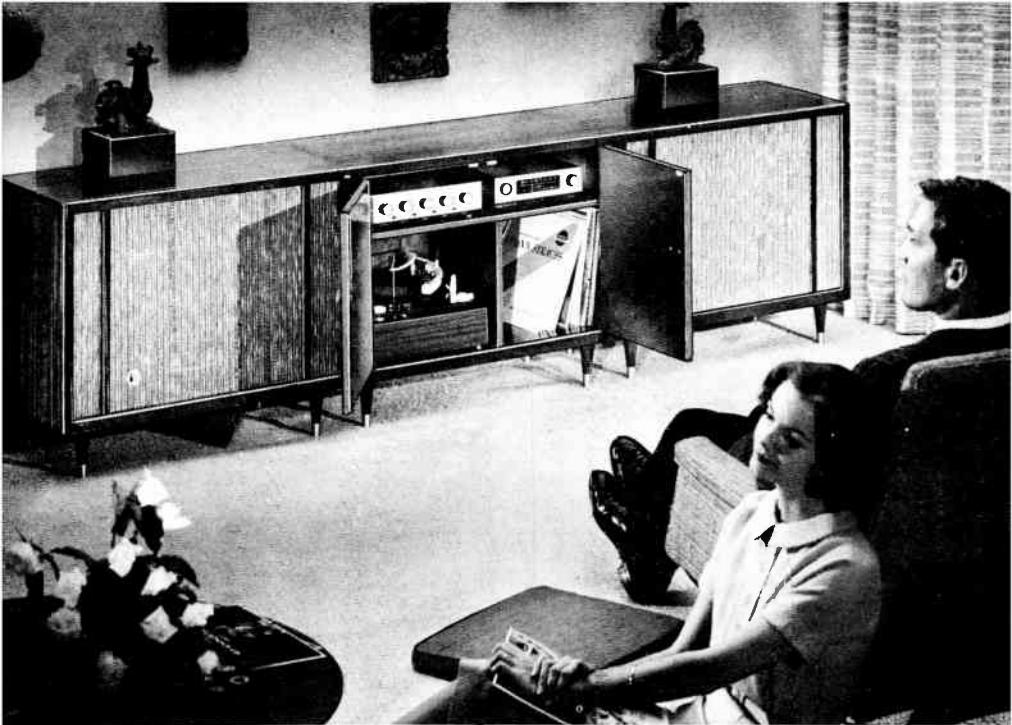
Fig. 103. Basic stereo system consists of stereo program source, dual control amplifier, power amplifiers and two speaker systems. More speakers may be used, but placement is critical. (Photo: Allied Radio Corp.)
