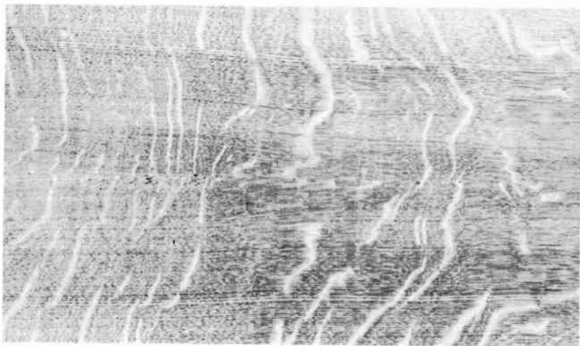
Fig. 1209. Quartered oak displays one of the most beautiful and complex graining figures to be found in wood. (Hardwood Plywood Institute.)
