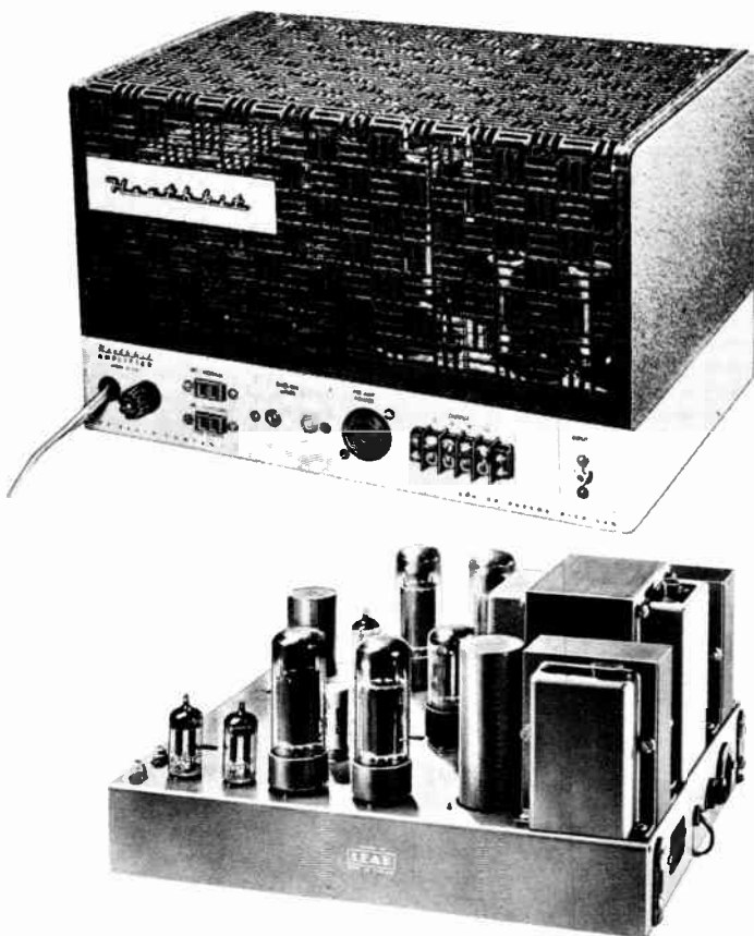
Fig. 412. The power amplifier is your hi-fi system's workhorse: (a) a typical single-channel amplifier and (b) a stereo power amplifier. Both units must be used with appropriate preamplifiers. (Upper photo: Heath Co. Lower photo: British Industries Corp.)
