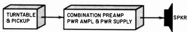
Fig. 401. The simplest form of a single-channel high-fidelity system contains just three components: the record player, the preamp-amplifier combination and the speaker system. For many installations, this is all that will be required.
