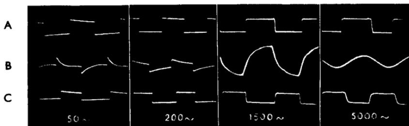
FIG. S/4A. Square waves at 50, 200, 1,500 and 5,000 c/s.
