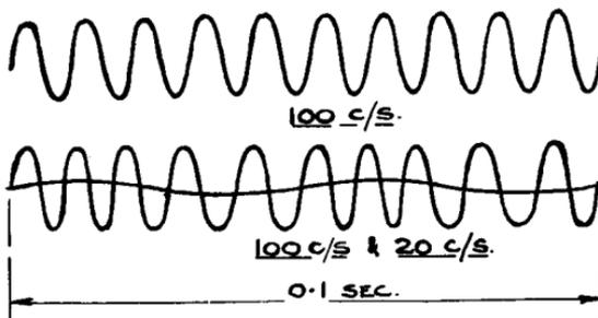
FIG. F/3. *Effect of 20 cycle flutter on 100 c/s pure tone.*
