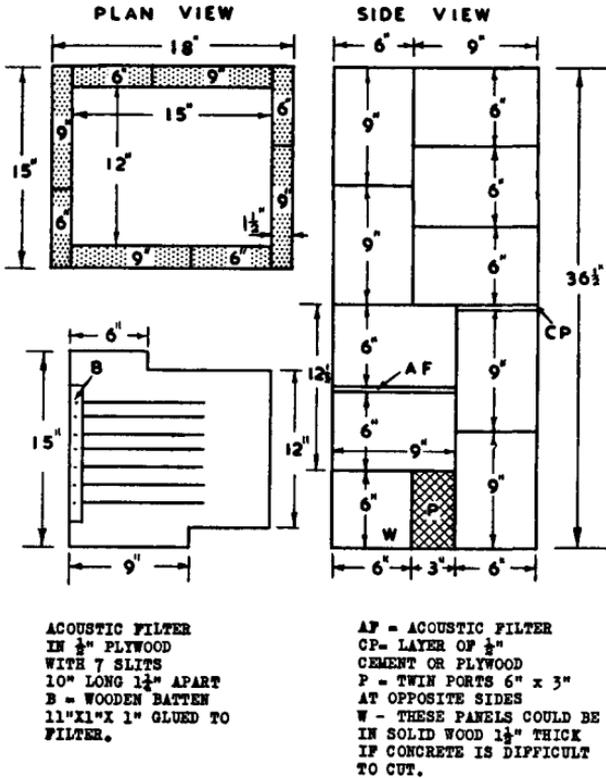
FIG. C/8. Concrete column, 4 cu.ft., using slabs 9" x 6" x  $1\frac{1}{2}$ " and suitable for 8" and 10" units.
