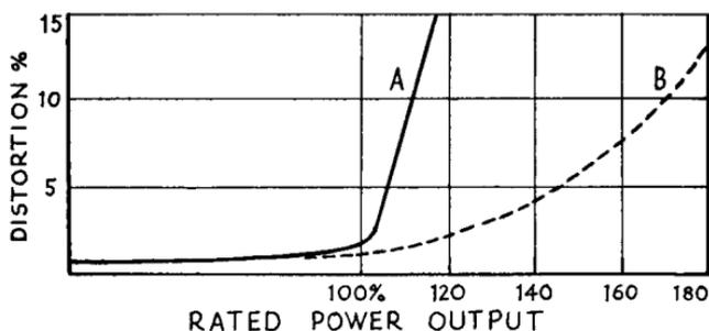
FIG. O/4. Amplifiers with different overload characteristics.
