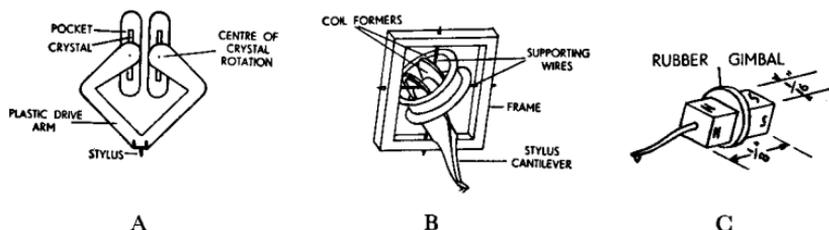
FIG. C/1. Cantilevers in stereo pickups.
