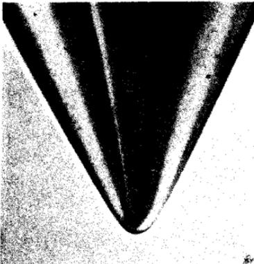
FIG. S/9. *First-class diamond LP stylus with excellent polish. Mag. 250x.*
