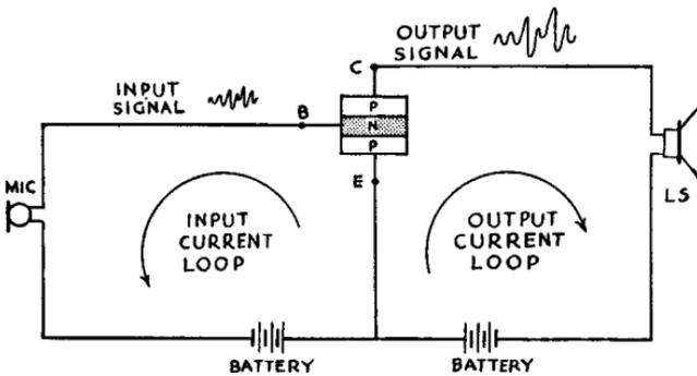
FIG. T/12. The transistor as an amplifier.
