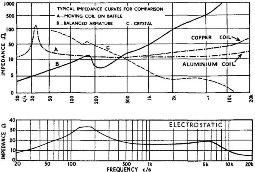
FIG. I/1. Typical impedance curves.
