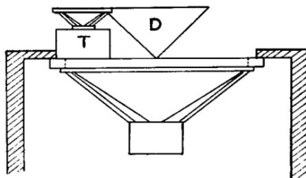
Column mounting is suitable for the home constructor; results with 8" and 10" units can be very good, and the cost with concrete models is extremely low. It should however be pointed out that these columns do not give the pure bass down to 30 c/s which is possible with 12" roll surround units in specially designed enclosures of about 2 cu. ft.
