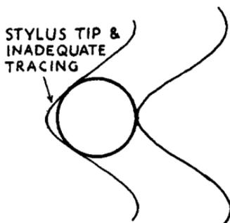
The use of  $\frac{1}{2}$  mil points has greatly reduced the incidence of inner groove distortion.
