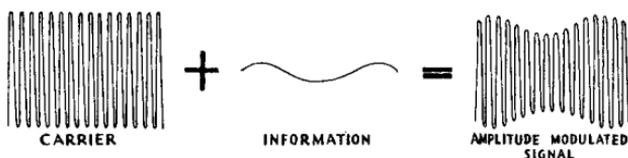
FIG. A/1. *Amplitude modulation.*
