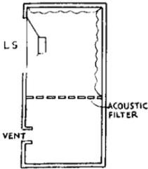
FIG. A/5. *Reflex enclosure with Acoustic Filter. Ordinary saw-cuts  $1\frac{1}{2}$ " apart make suitable slits. Absorbent lining in upper section only.*
