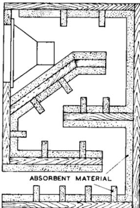
FIG. A/6. *Typical acoustic labyrinth.*
