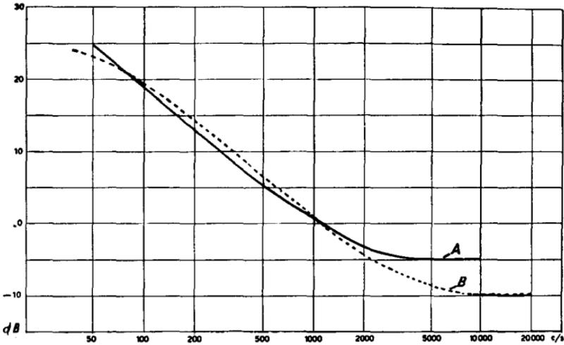
FIG. T/3. Standard replay characteristics for 7½" tapes
