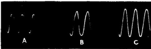
FIG. N/1. *Non-linearity at A and B at 40 c/s with 1 watt input to 10" unit.*
