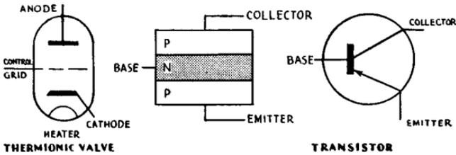
FIG. T/11. Valve and Transistor symbols.
